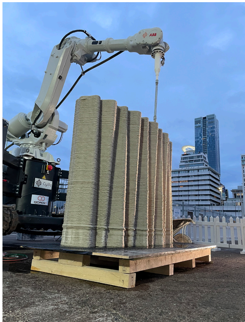
An example of a wall which can be achieved using the QOROX™ 3D Printed Concrete Wall System.
