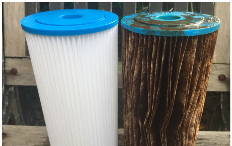
A new 20 micron water filter (left) and the used filter it is replacing after 4 months' use.
