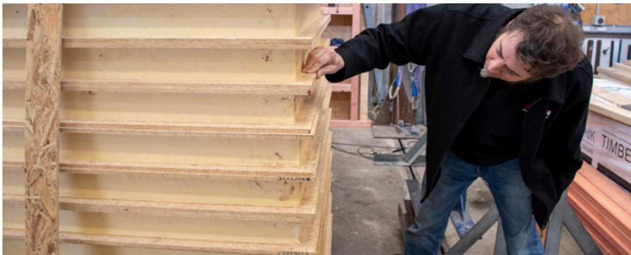
Prefabricated building systems are becoming more prevalent in New Zealand in an effort to provide resilient buildings that are high quality, affordable and can be quickly constructed. Structural insulated panel (SIP) systems have been used worldwide for many decades. They provide excellent insulation performance, which can improve energy efficiency and include a high degree of off-site prefabrication.
