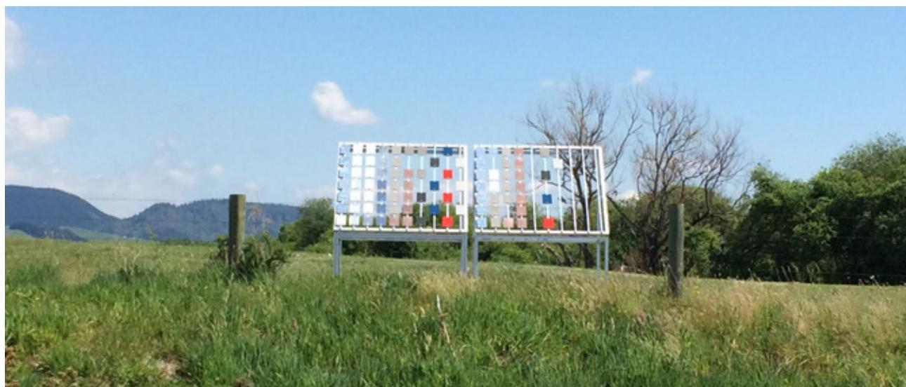
BRANZ has established over 100 outdoor exposure testing sites across New Zealand. These sites are used to evaluate the environmental performance of metals, plastics and timbers to meet specific research or consultancy needs. Exposure testing and other forms of monitoring provide well-grounded baseline data. The monitoring data informs material durability assessment, required by the New Zealand Building Code, and methodology development for testing materials.
