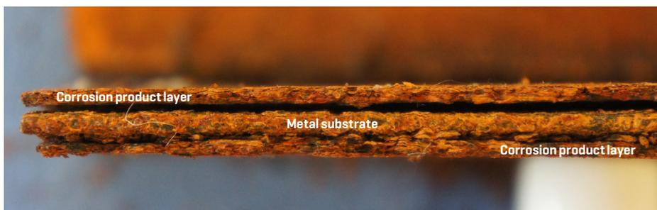
Figure 3. Corrosion products on the mild steel sample exposed at the wastewater treatment plant site for 1 year.
