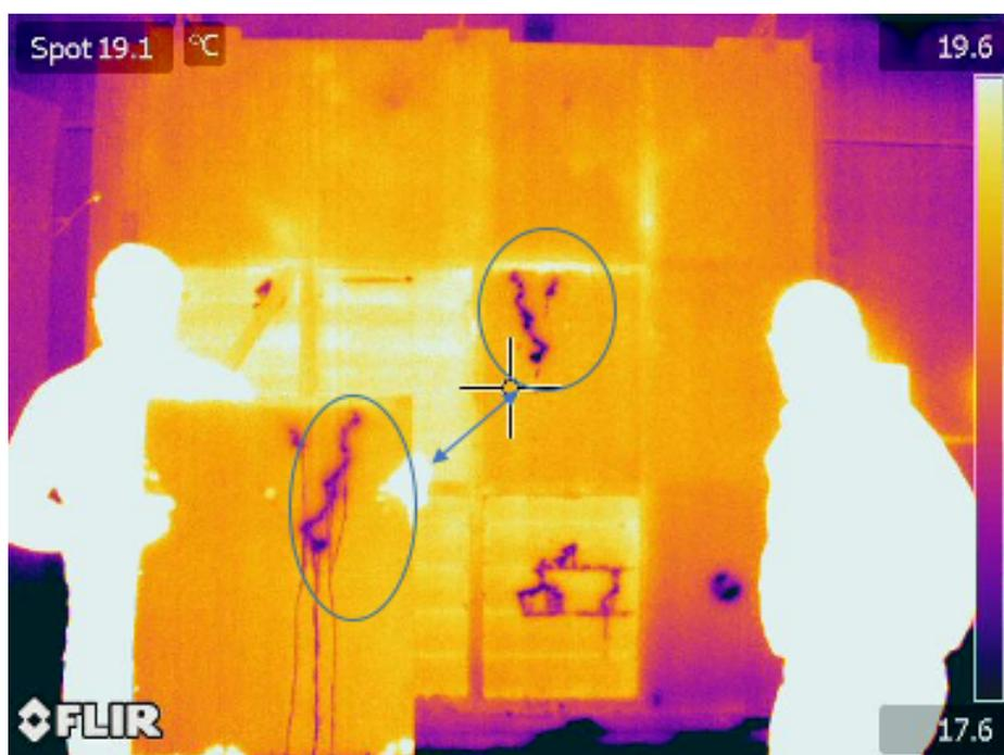
Figure 2. Disassembly of a wall where water transfer has occurred. The pattern of water on the back of the lining being held up matches the pattern on the surface of the insulation.
