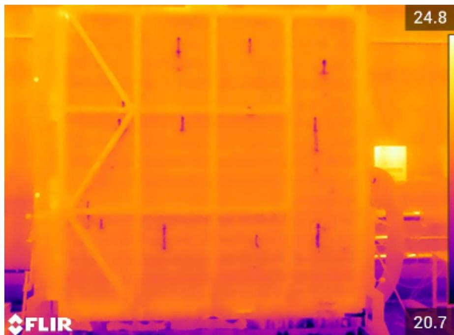
Figure 1. The baseline case – an uninsulated wall without lining.
