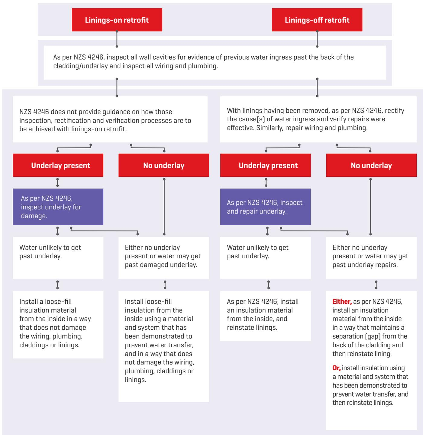
Figure 3. Decision tree for retrofitting wall insulation
