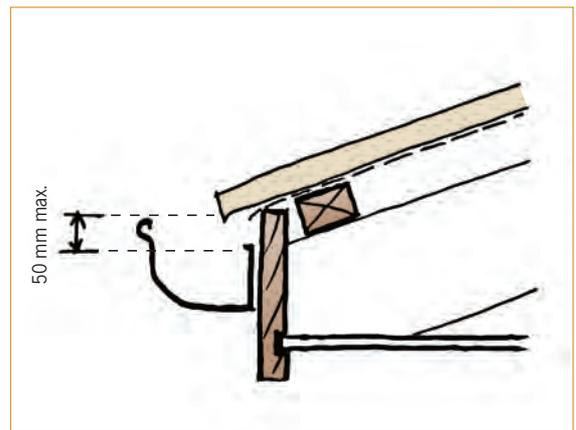
Figure 2. External gutter.
