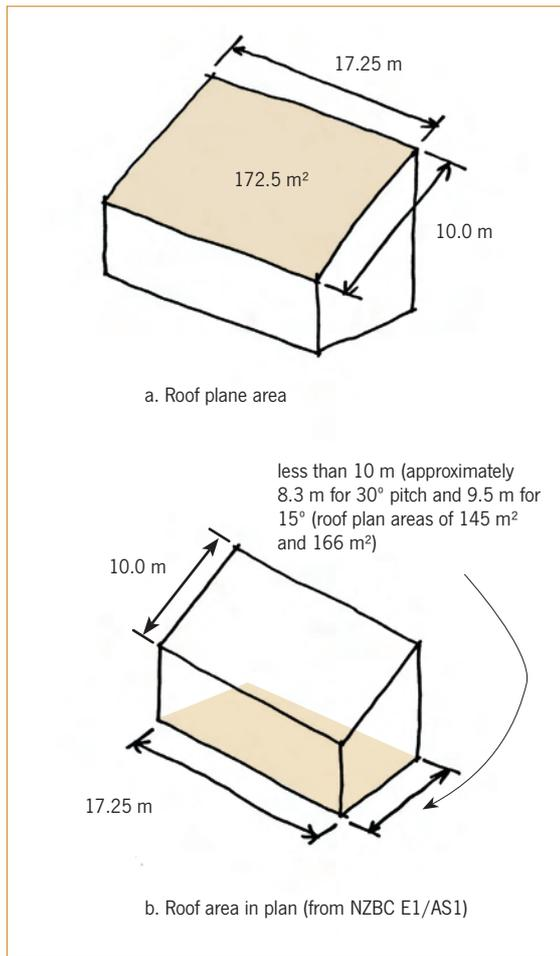
Figure 1. Roof area calculation.
