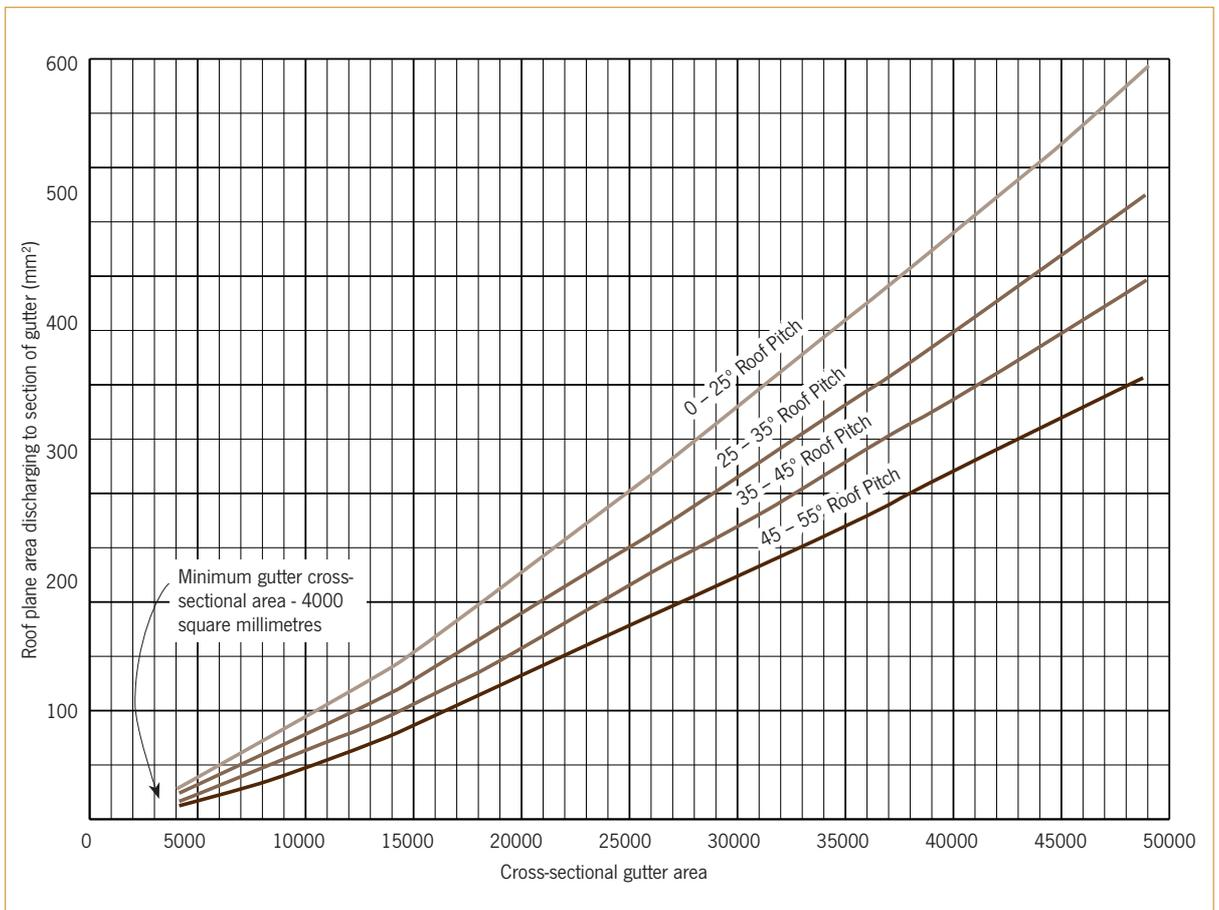
Figure 4. Cross-sectional area of external gutter (mm<sup>2</sup>). Based on rainfall intensity of 100mm/hr)adjusted for roof plane area. (Adapted from E1/AS1.)
