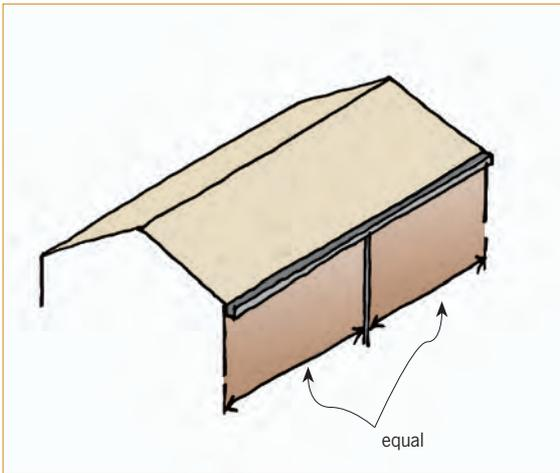
Figure 3. Centrally positioned outlet.
