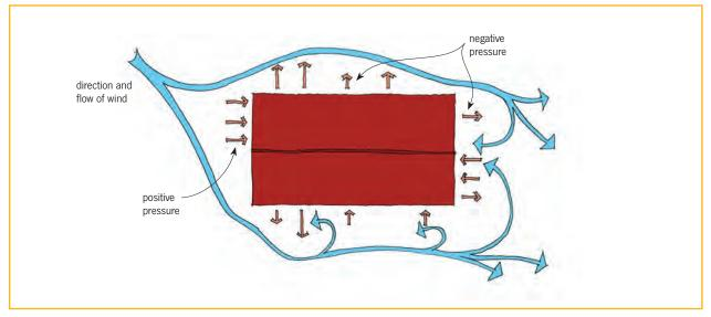
Figure 3. Wind pressure acting on walls.
