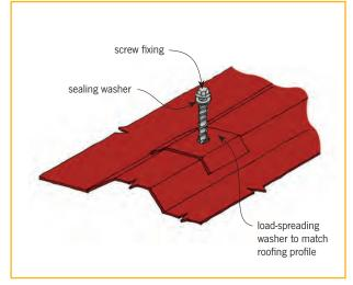
Figure 4. Load-spreading washer to metal roofing.
