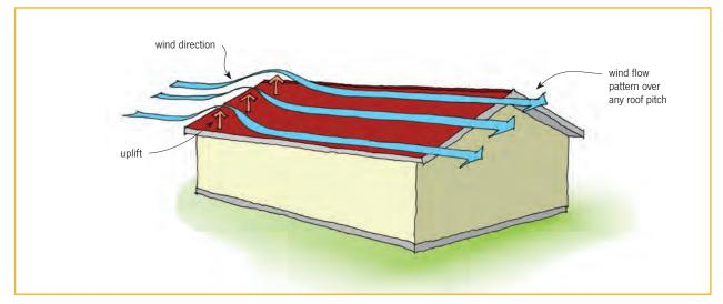
Figure 1. Wind parallel to ridge.
