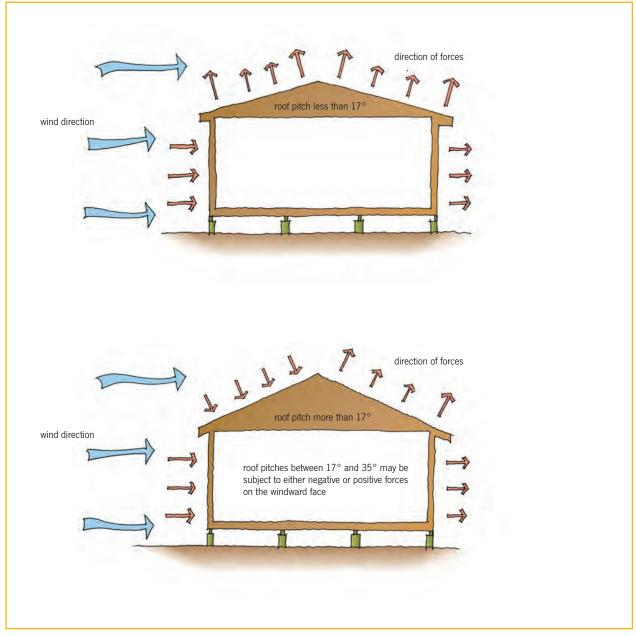
Figure 2. Wind at right angles to ridge.
