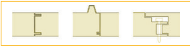
Figure 2 Examples of edge-jointing details – the dark line is the metal skin outline
