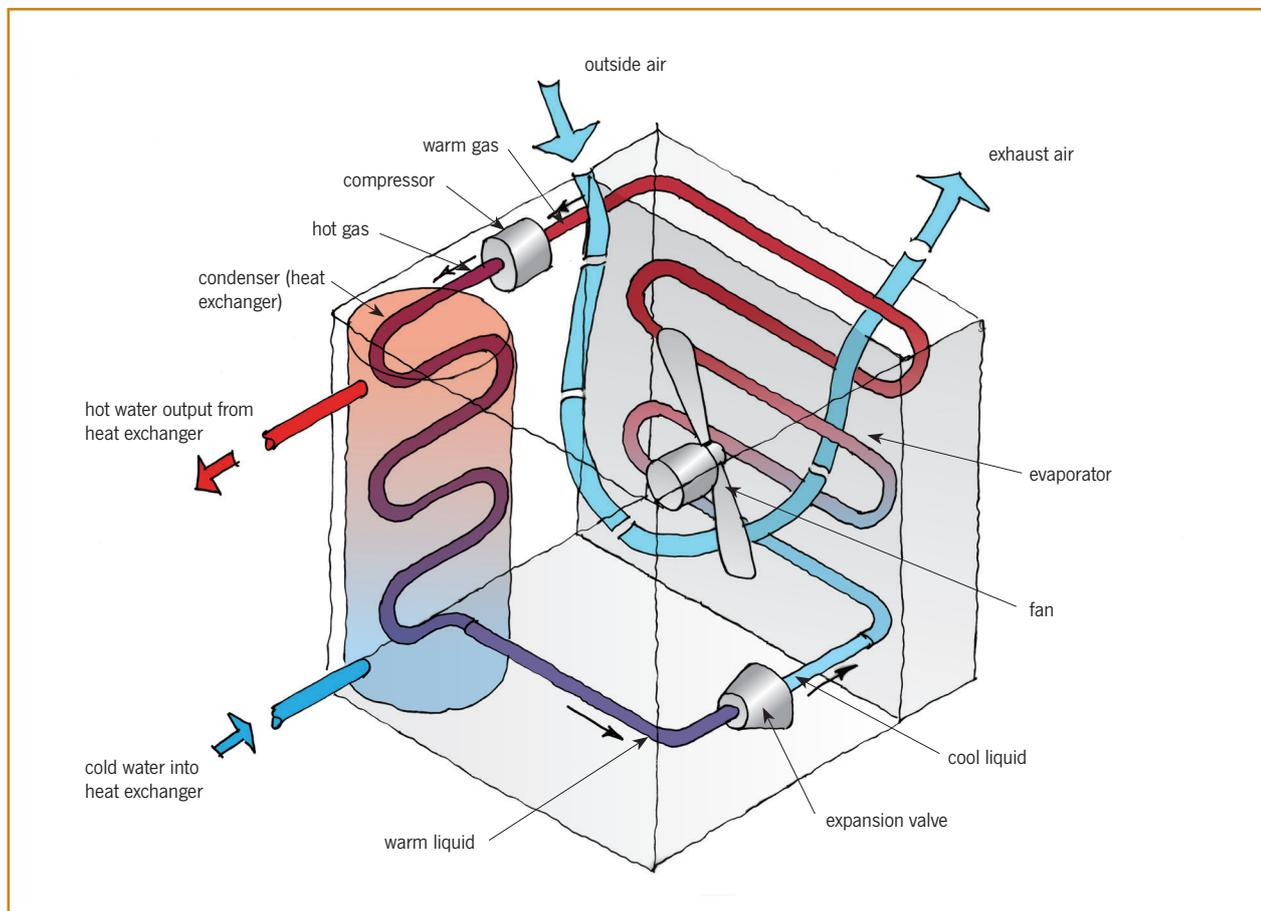
Figure 1. Air-source heat pump water heater cycle.
