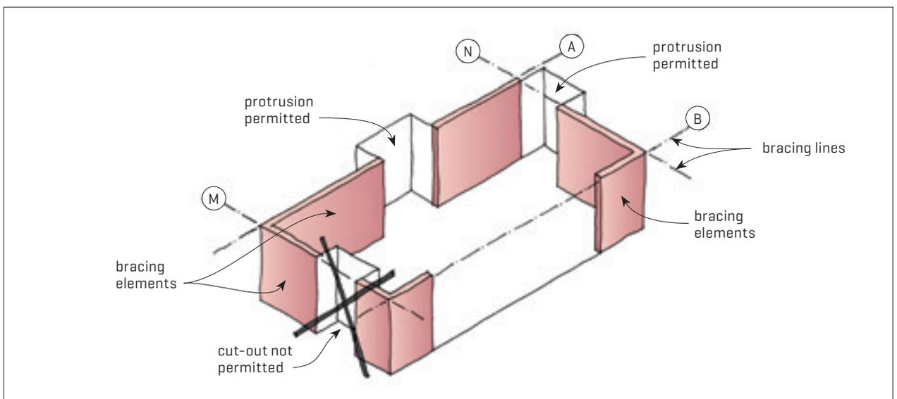
Figure 6. Ceiling diaphragm protrusions and cut-outs.
