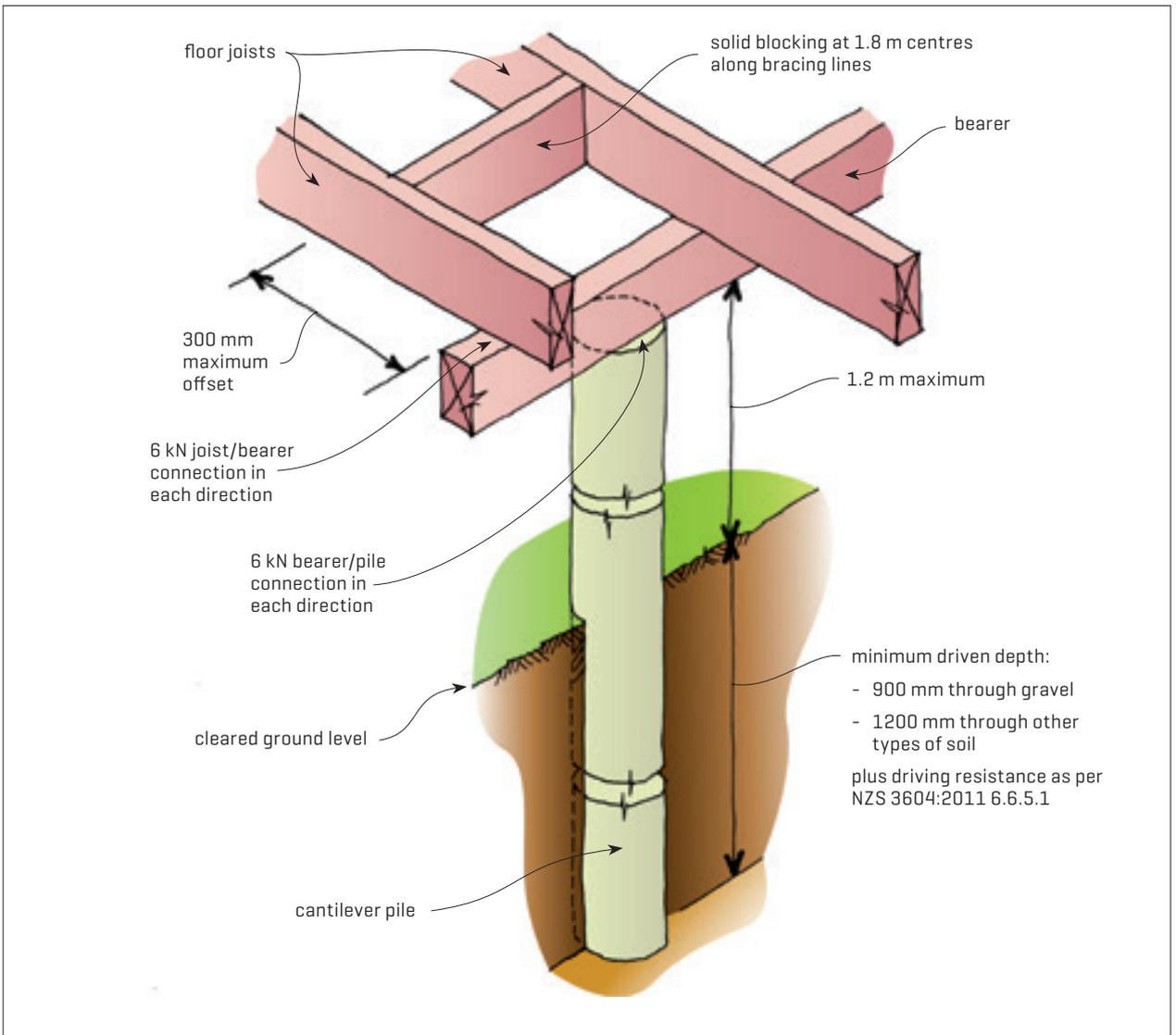
Figure 2. Cantilever piles.
