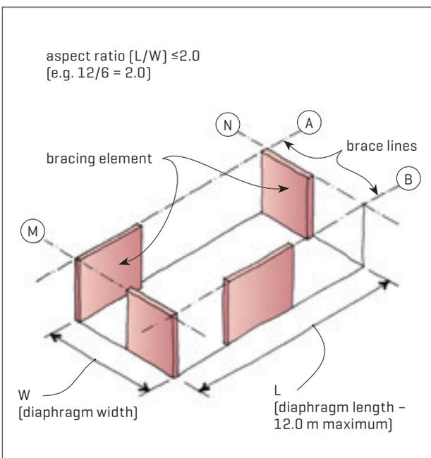
Figure 3. Bracing lines supporting diaphragms.
