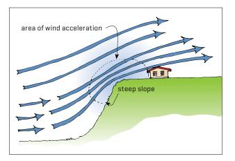
Figure 2. Wind speed over an escarpment. (An escarpment is a slope of 35% (19° or 1 in 3) or steeper over a vertical distance of 6 metres or more that separates two more gently sloping or flat areas.)
