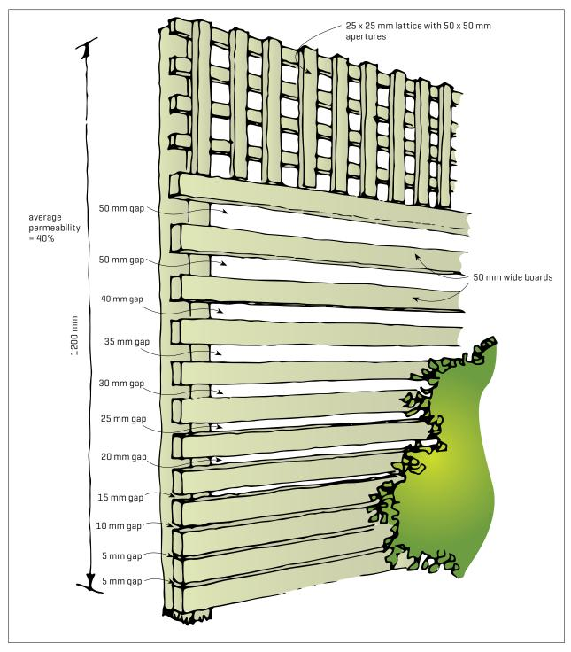
Figure 9. Fencing designed for maximum shelter.
