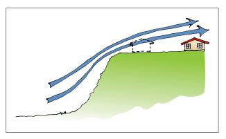
Figure 5. Locating the building back from the edge of a slope.
