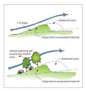
Figure 15. Earth mounding to provide shelter. The imported material can also improve the ground conditions to get the shelter planting established as well as acting as a wind management tool.
