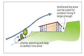
Figure 14. Wind protection by excavating the site.
