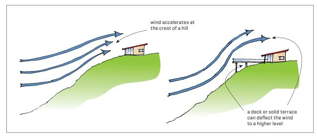
Figure 13. Using a terrace or deck to deflect wind.
