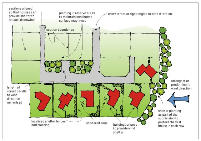
Figure 4. Site planning to reduce wind effects. Screens can manage wind and provide sheltered outdoor living environments.
