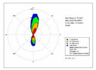
Figure 3. Wind rose (direction, strength and frequency) diagram for Kelburn, Wellington, which shows that strong winds generally blow in a northwest to north or southerly direction. (Source: NIWA.)
