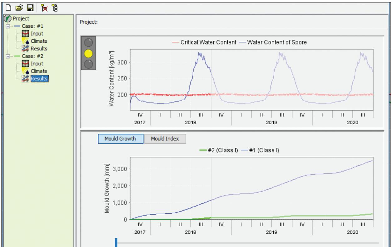
Figure 3. Example output from WUFIBio.
