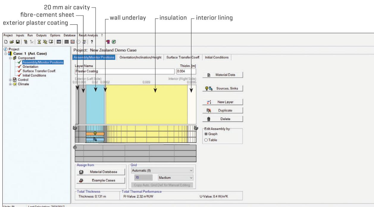
Figure 2. WUFI model of 20 mm cavity wall.
