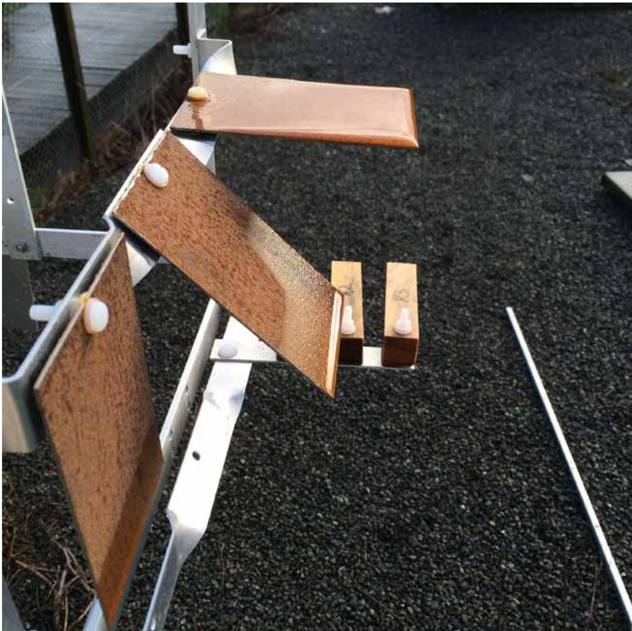
Mild steel coupons were installed in an exposed location away from the BRANZ test house.
