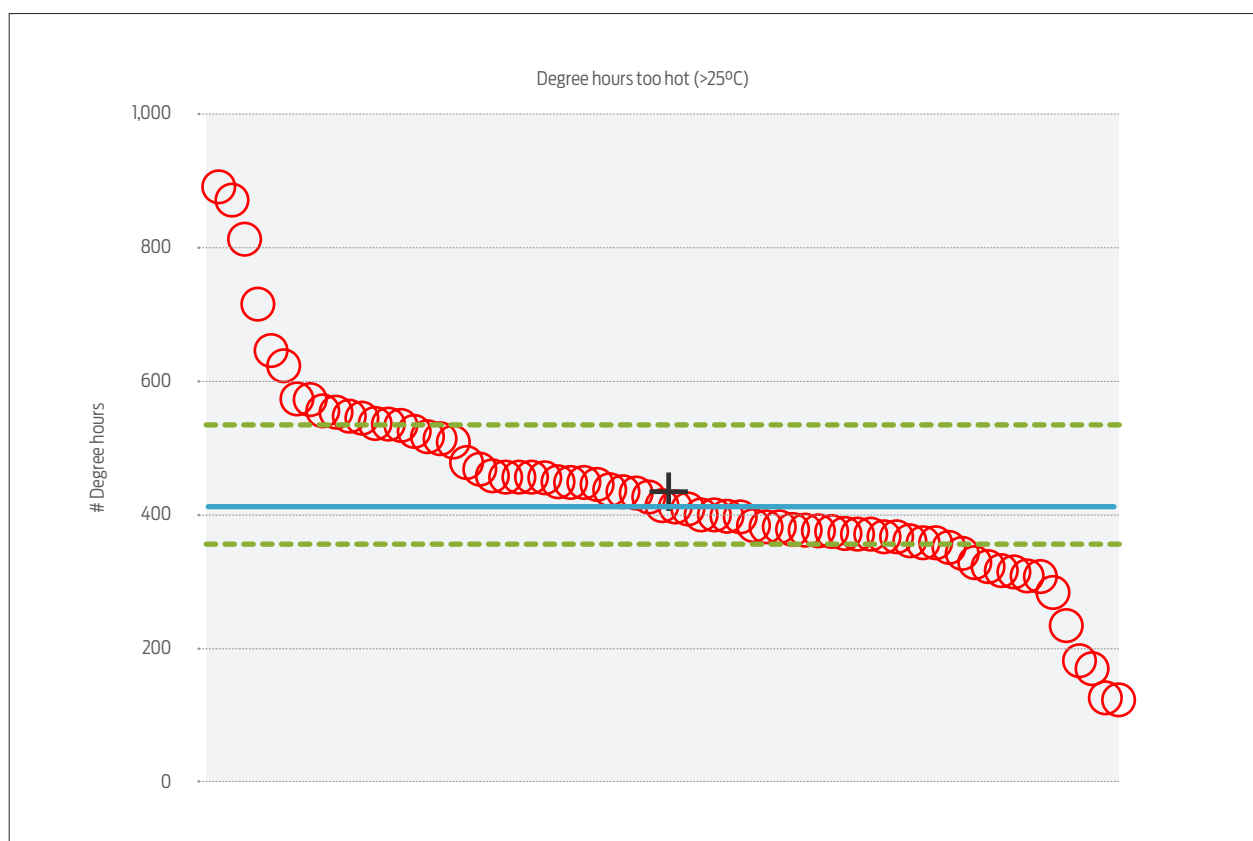
Figure 2. Overheating severity in the main living room for 70 new Christchurch houses [assessed through computer modelling].
