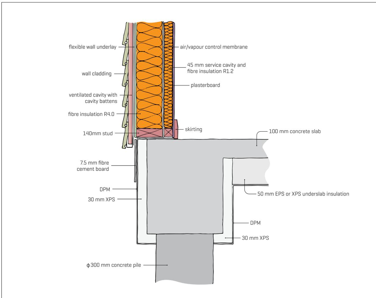
Figure 3. Concrete pile to insulated slab on ground.
