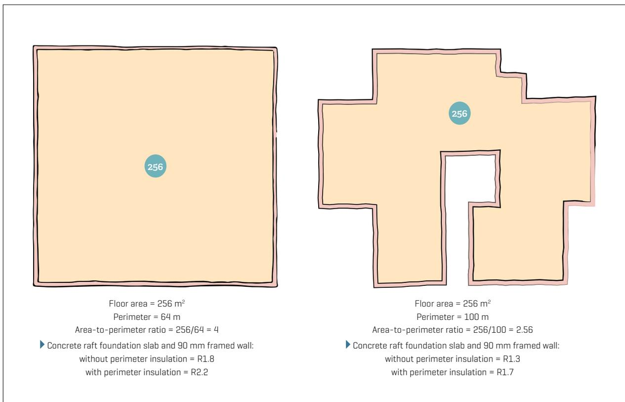
Figure 1. Slab area-to-perimeter ratio.
