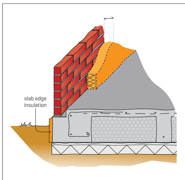
Figure 4. Slab edge insulation.
