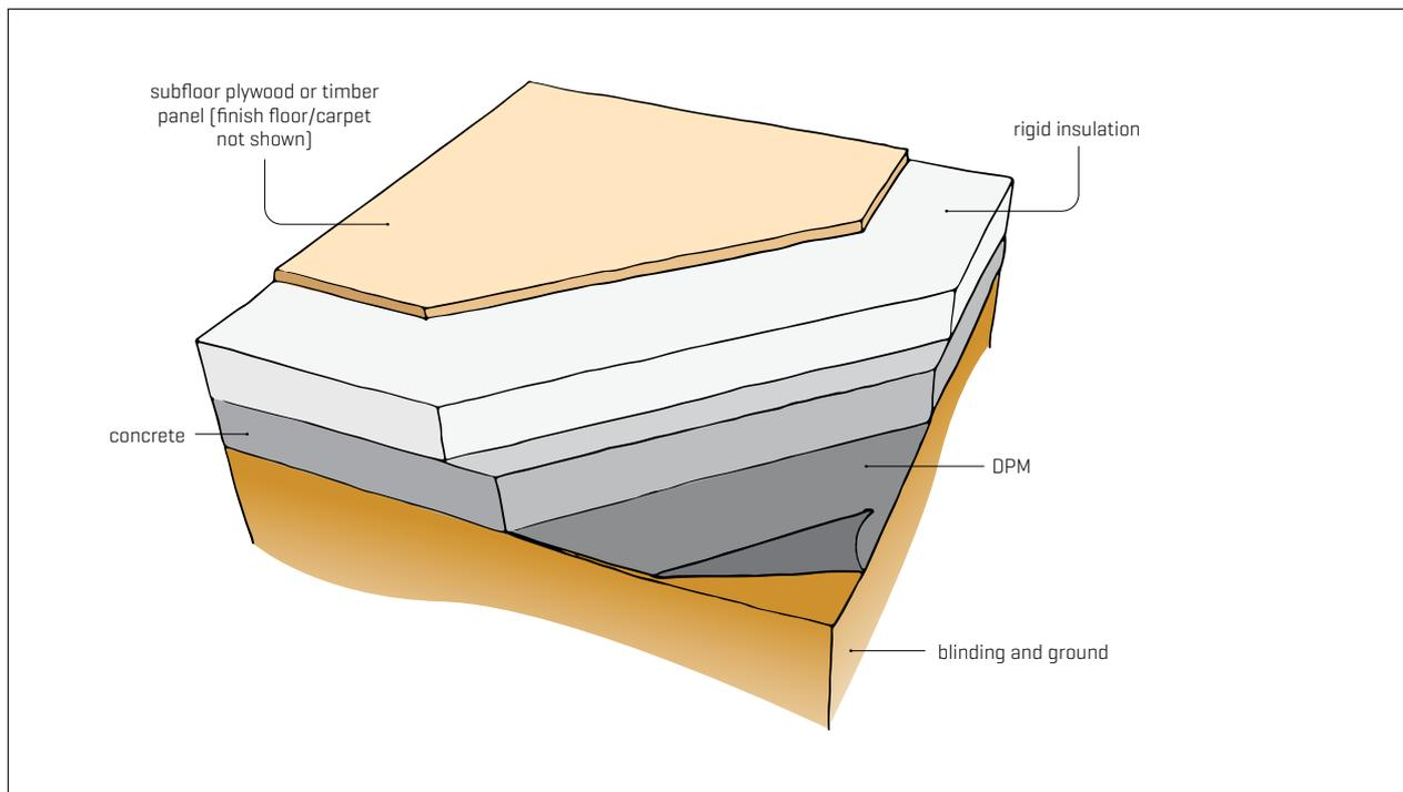
Figure 5. Insulation above the slab with rigid sheet material above the insulation.
