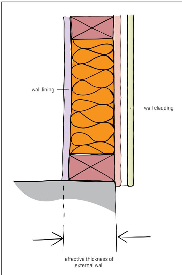
Figure 2. Effective thickness of an external wall.
