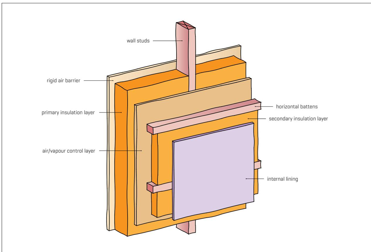
Figure 2. A 45 mm thick interior batten fixed over an air/vapour control layer creates space for a secondary insulated cavity.
