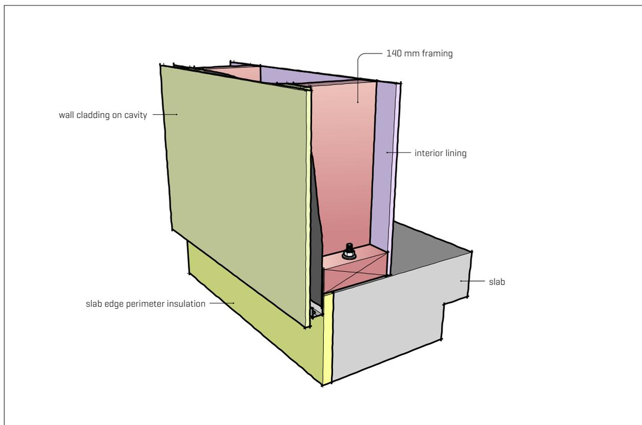
Figure 1. Using 140 mm timber framing reduces the difficulty of fixing bottom plates to the edge of the floor slab and enables a deeper bottom plate overhang to better accommodate vertical slab edge insulation.
