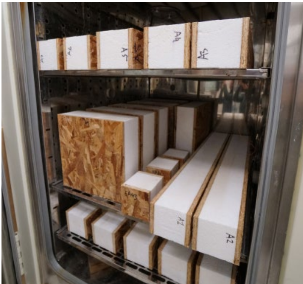
Small-scale SIP samples in indoor climate chambers for accelerated ageing.
