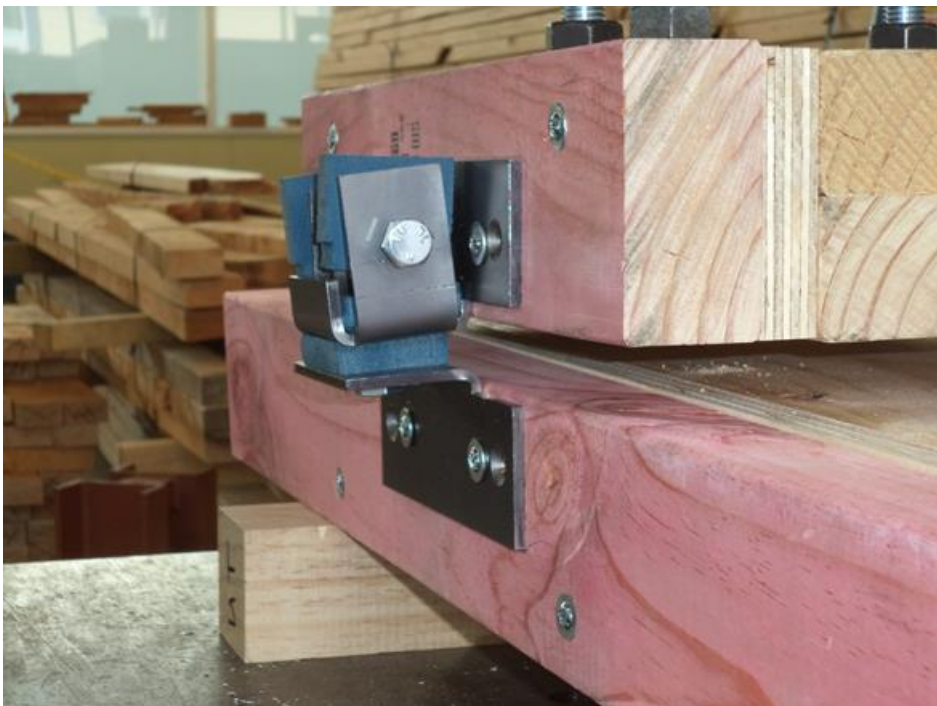
Figure 50. Final distortion of brackets after axial compression/tension test.
