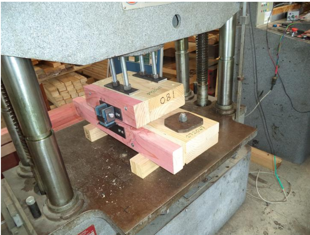
Figure 46. Across-plate connector shear load test.
