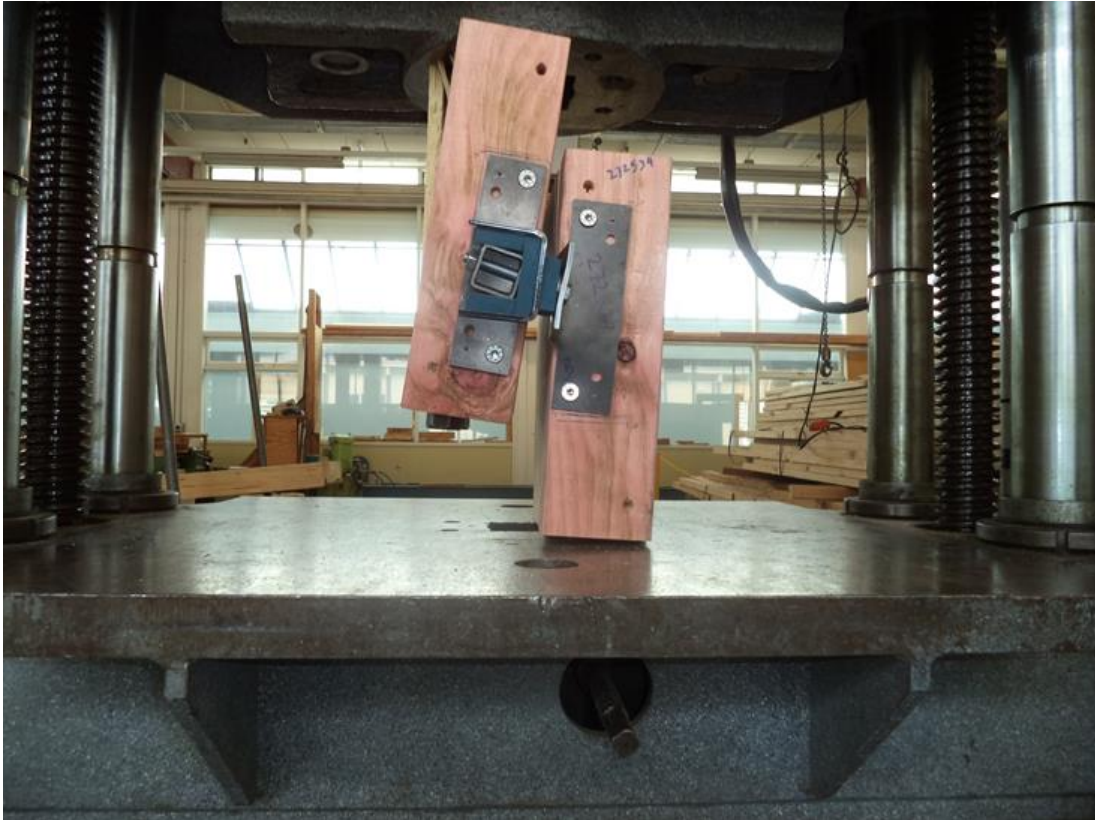
Figure 35. Final failure mode in axial tension – failure is due to splitting of the timber, the connector still holds and the screws are still connected to the joist sections.
