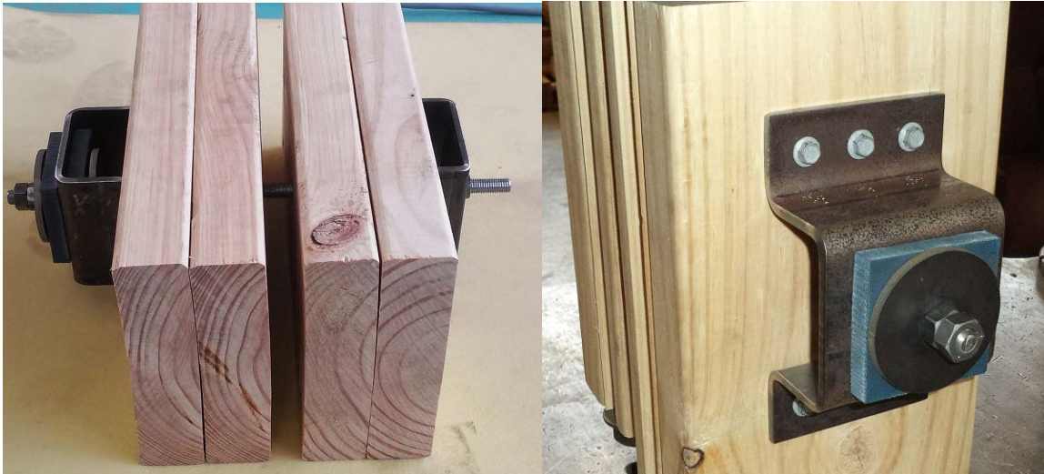
Figure 39. Through-joist connector prototype.
