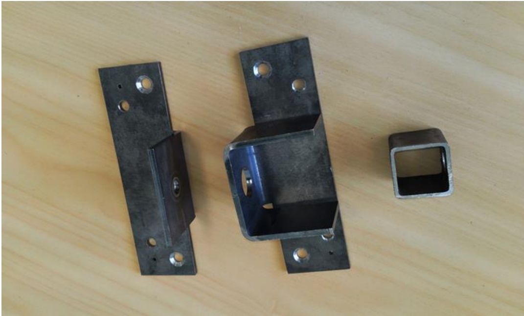
Figure 10. Steel parts (from left to right), L bracket, Cup Bracket, Square insert.
