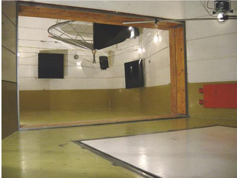
Figure 21. The acoustic chambers without our test wall. Clearly showing the aperture with its wooden collar.
