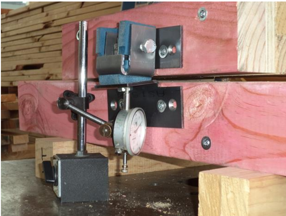
Figure 49. Distortion of brackets under axial compression load (about 6kN)
