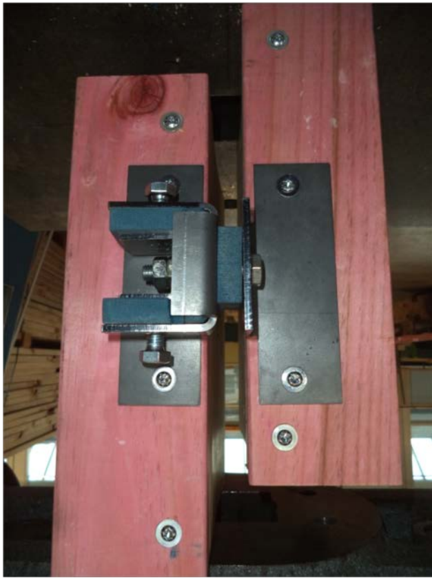
Figure 46. Across-plate connector shear load test.
