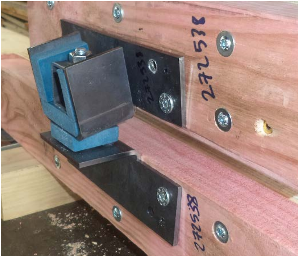
Figure 33. Axial cyclic loading test showing flexure of brackets at 15mm tension displacement. Note that the part of the brackets which are faced to the timber are flexing as well as rotating.
