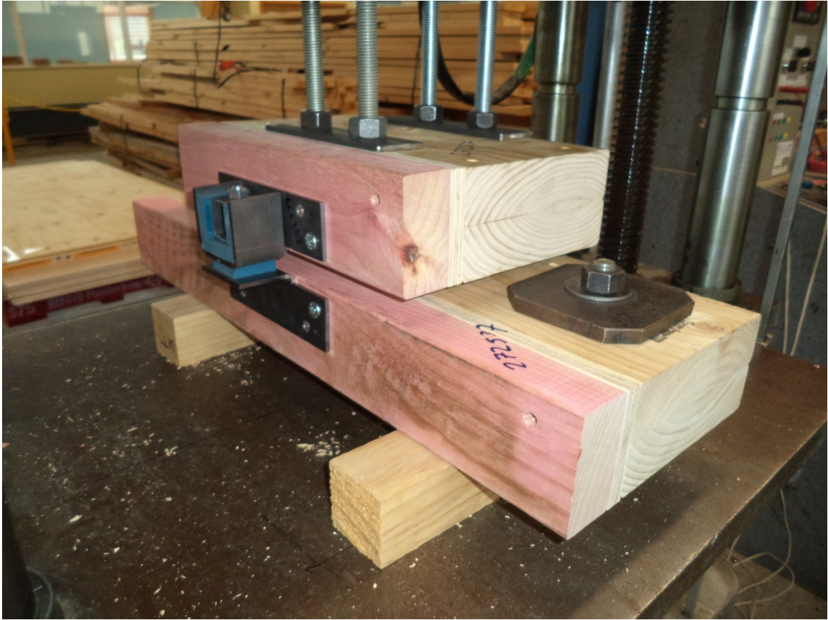
Figure 26. Across-plate connector axial load test.
