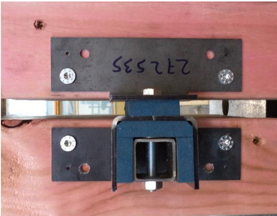
Figure 8. Across-plate connector design prototype as screwed on to bottom plates. Two pairs of screw holes are provided each side, but only one pair is expected to be used to penetrate middle of edge joists (and only these were counter sunk).
