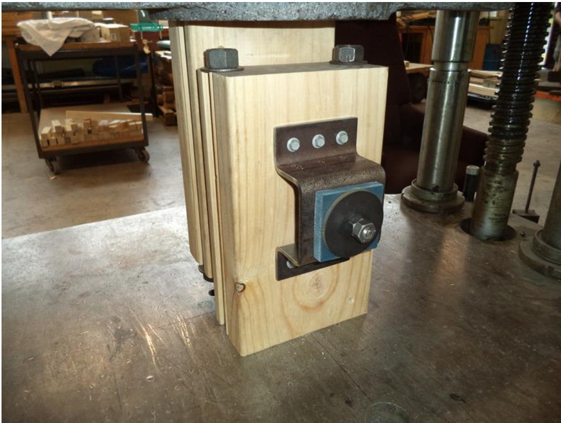
Figure 44. Through-joist connector shear load test.
