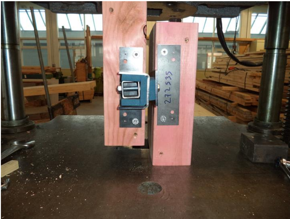
Figure 30. Shear cyclic test showing movement of SHS within bracket.
