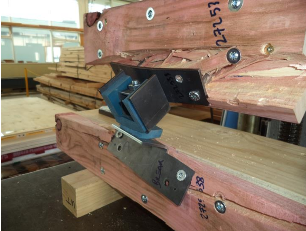
Figure 37. Final failure mode in axial tension – failure is due to splitting of the timber, the connector still holds and the screws are still connected to the joist sections.
