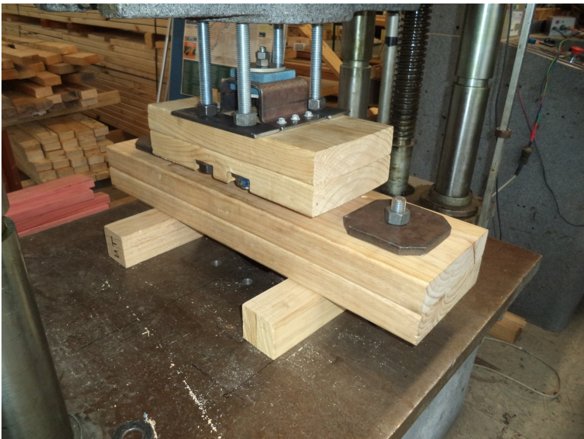
Figure 44. Through-joist connector shear load test.
