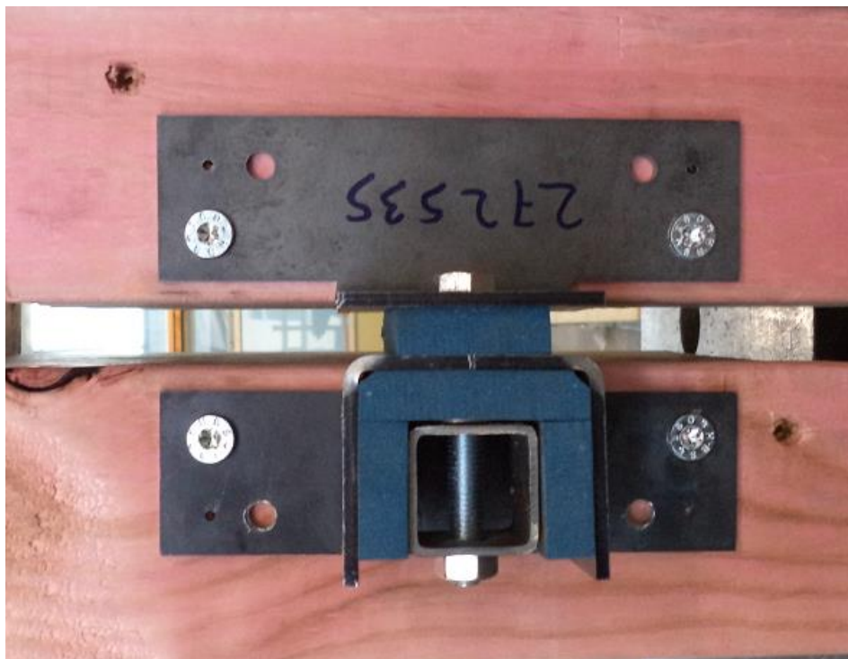
Figure 1. Across-plate connector design prototype screwed on to bottom plates, through flooring and into the edge joist.
