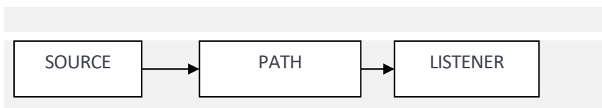
Figure 8: Simplified block diagram representing the transmission of noise from a sound source along one or more transmission paths to a listener
