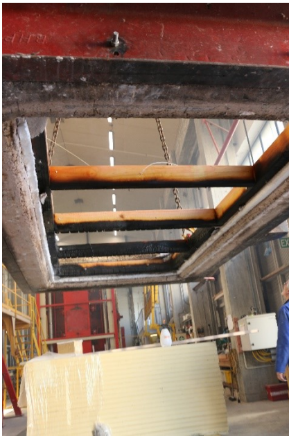
Evaluating lining encapsulation robustness with furnace tests
