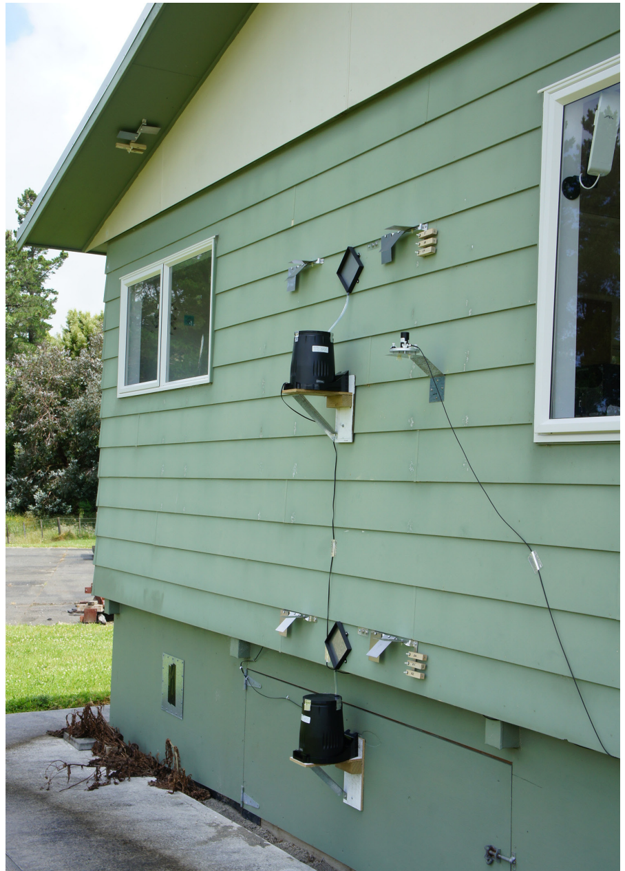
Figure 2. Measuring equipment installed on the BRANZ test building at Judgeford (semi-rural environment).
