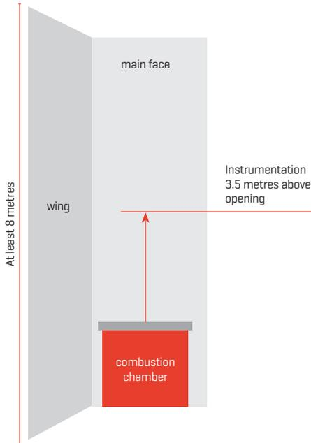
Figure 2. Schematic of BS 8414 test specimen
