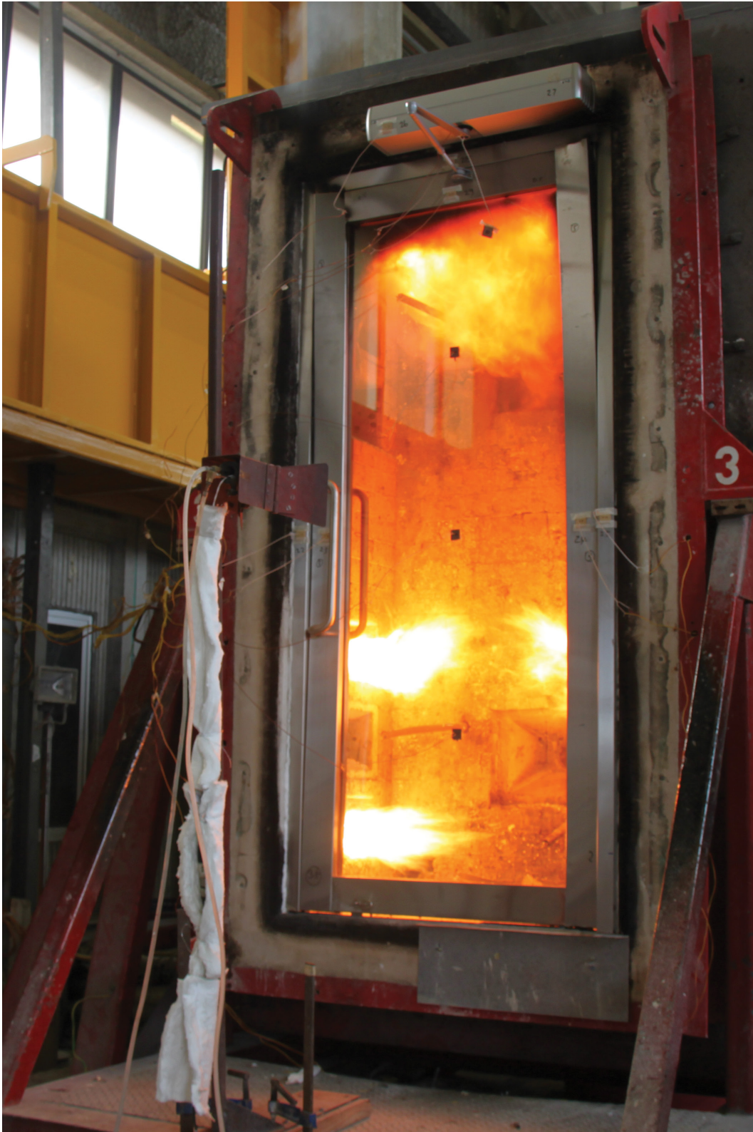
Pilot fire resistance furnace 2 m high × 1 m wide
