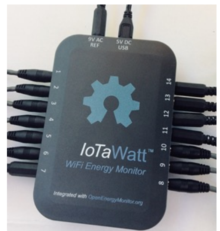
The IoTaWatt™ measures the energy used on individual circuits.
