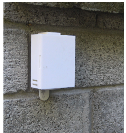
Wireless tags are contained inside a small box and mounted to an exterior wall.
