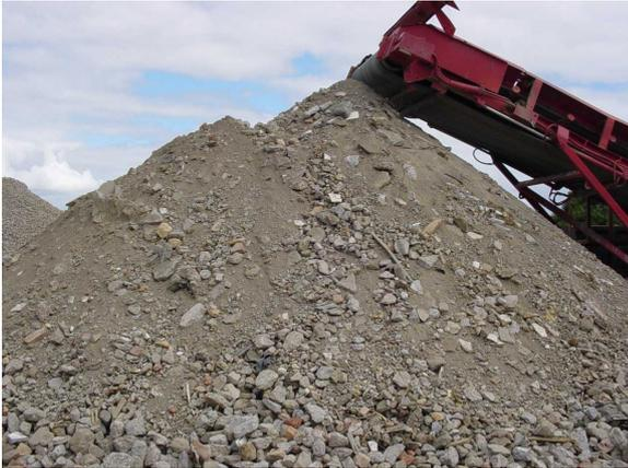
Locate plant for processing where you want the stockpiles to be located to save moving stockpiles later. As the pile reaches the height of the conveyor, the plant will need to be moved to the next stockpile location.
