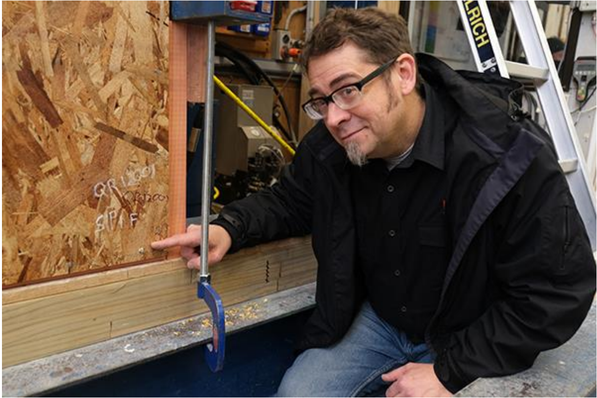
BRANZ structural engineer Dr David Carradine checks a SIPs panel undergoing laboratory testing for earthquake resilience (photo credit: Niall Harkin)
