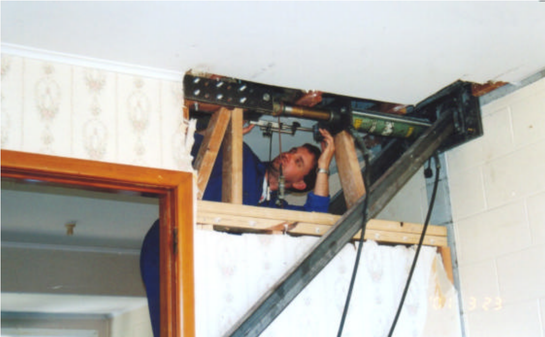
Figure 29: Reaction frame and loading ram at top floor ceiling level
