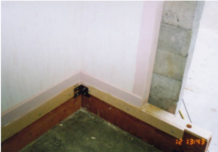
Figure 3: Simulation of concrete foundation (bottom plate coach screwed to foundation beam and flooring beneath skirting board)
