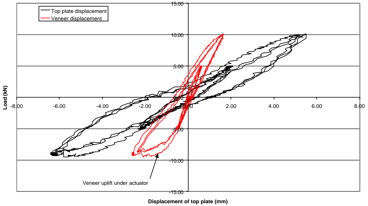
Figure 21: Comparison of top plate displacement and veneer displacement against load – cycles to 10 kN.
