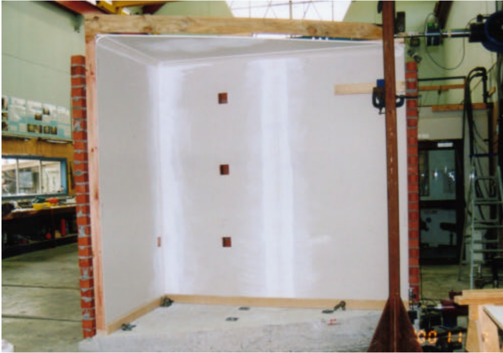
Figure 20: Interior view of the brick veneer test specimen
