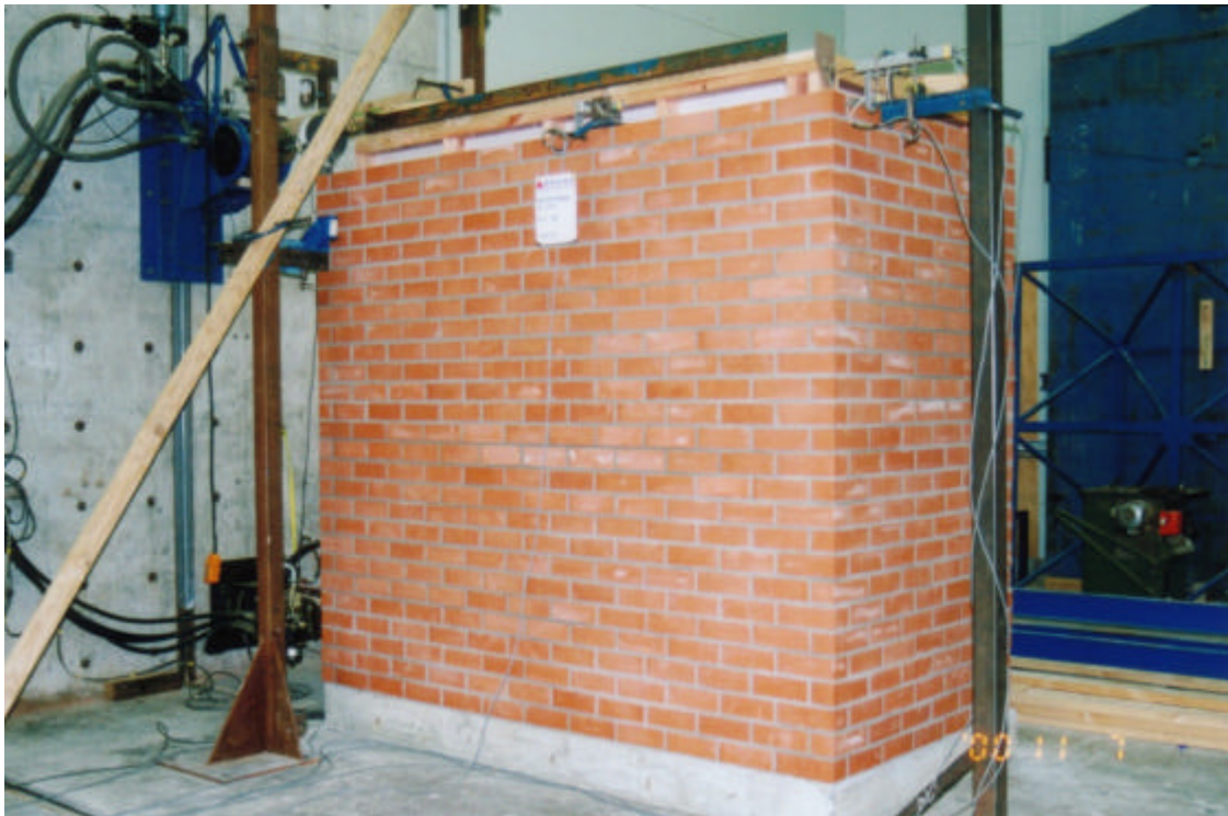
Figure 19: Exterior view of the brick veneer test specimen
