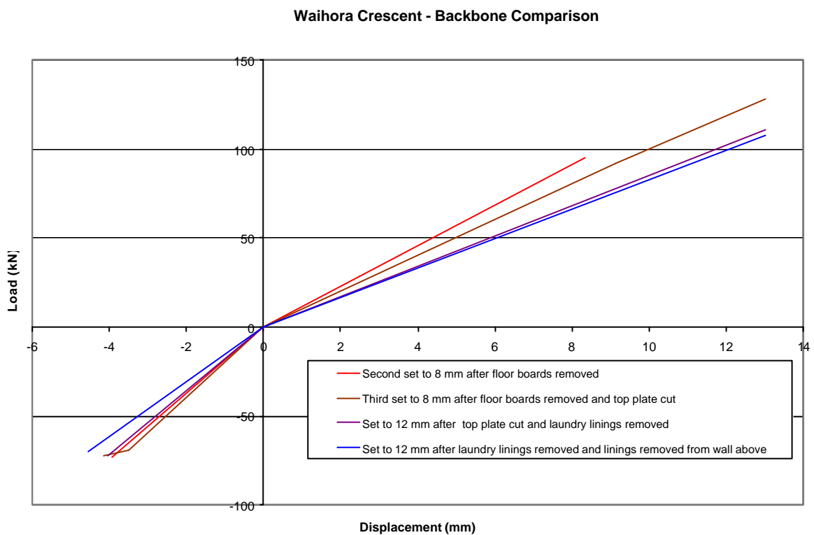
Figure 42: Comparison of backbone curves as potential load transferring elements successively removed
