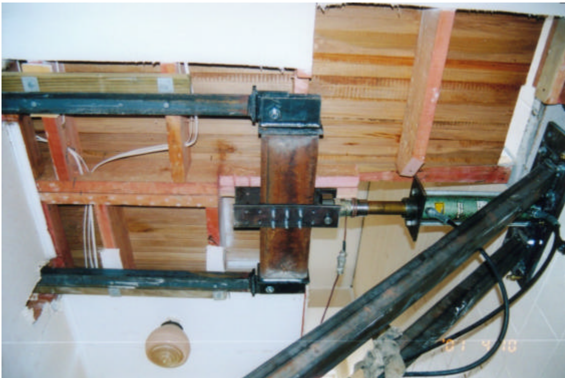
Figure 36: Details of the load application rig (load was applied via the spreader beam in the centre of the photograph to the two beams fixed to the underside of the joists)
