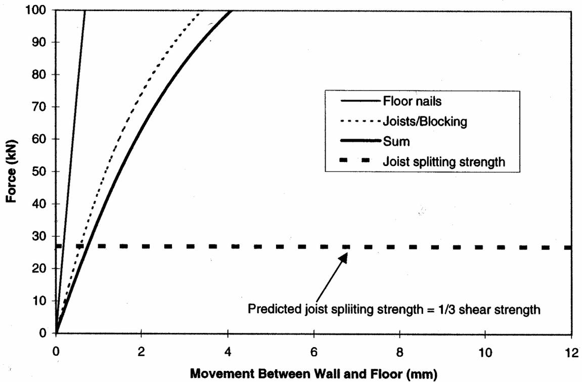
Figure A.9: Relationship Between Force and Movement – Force Perpendicular to Stringers.
