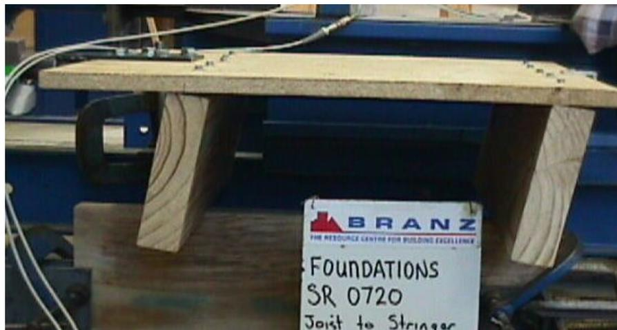
**Figure A.4: Load Parallel to Stringer Without Blocking.**
