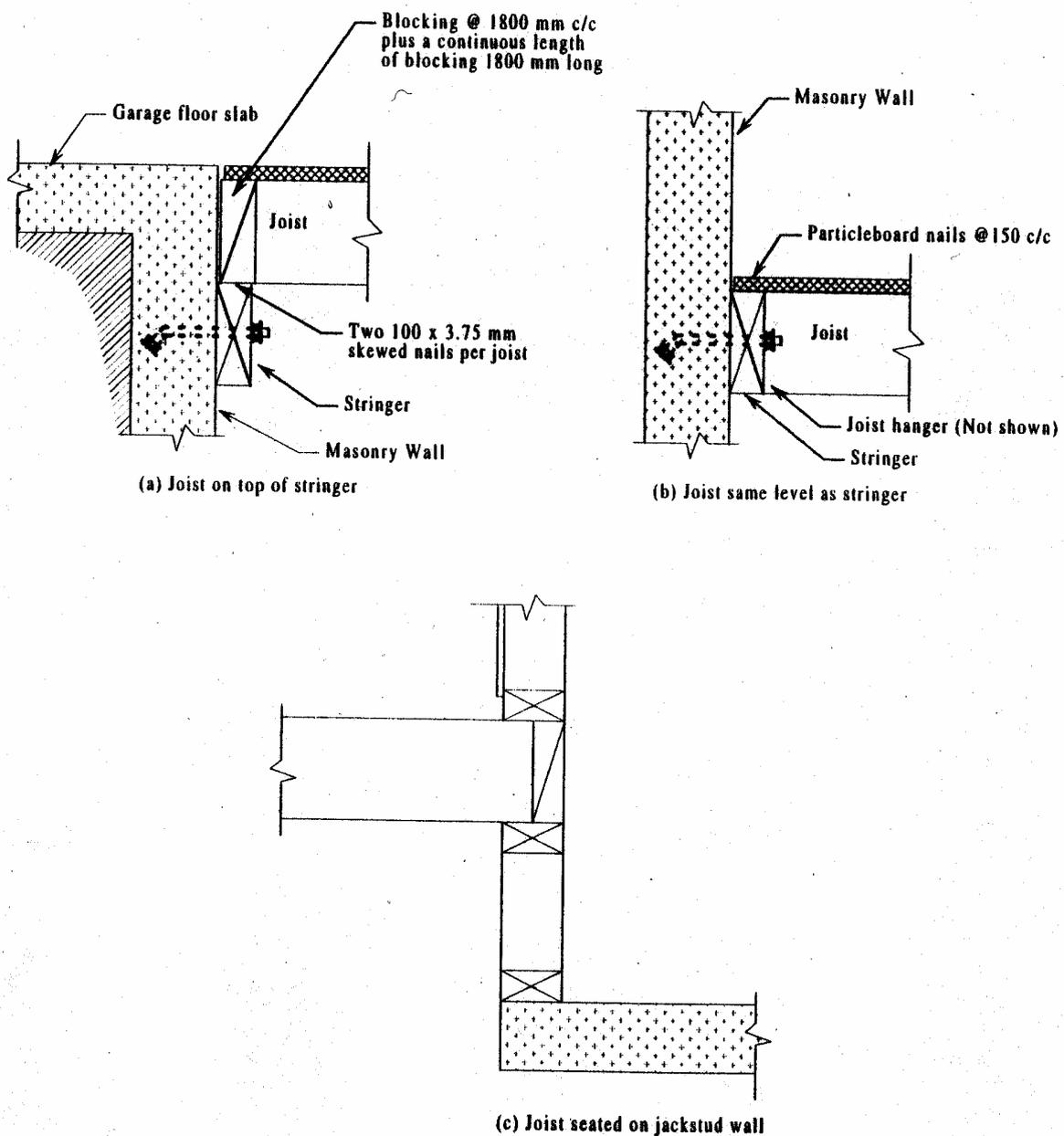
**Figure 3. Fixings at junction of house floor on piles and garage**
