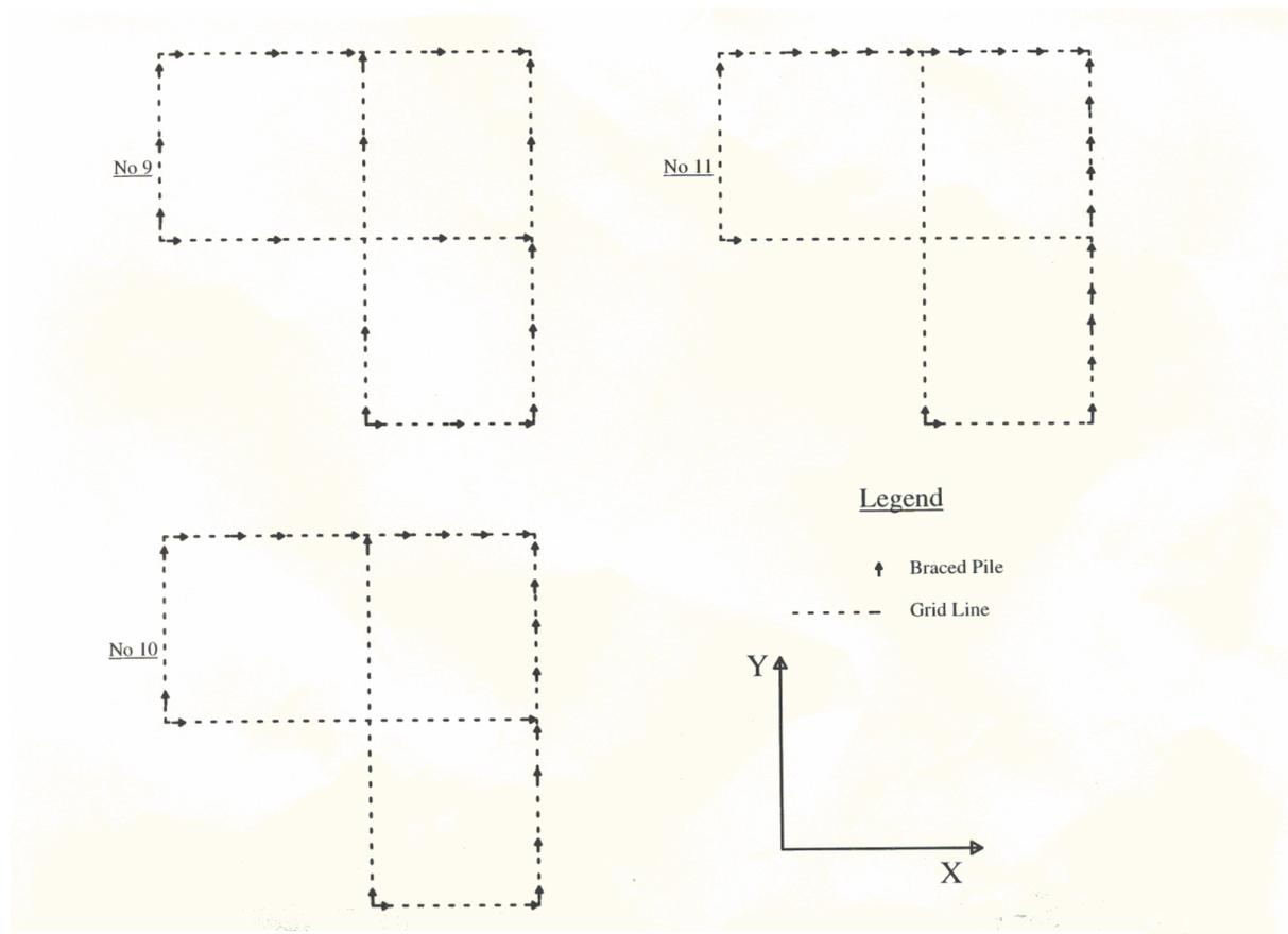
**Figure 8. Pile configurations analysed for 'L' shaped house**
