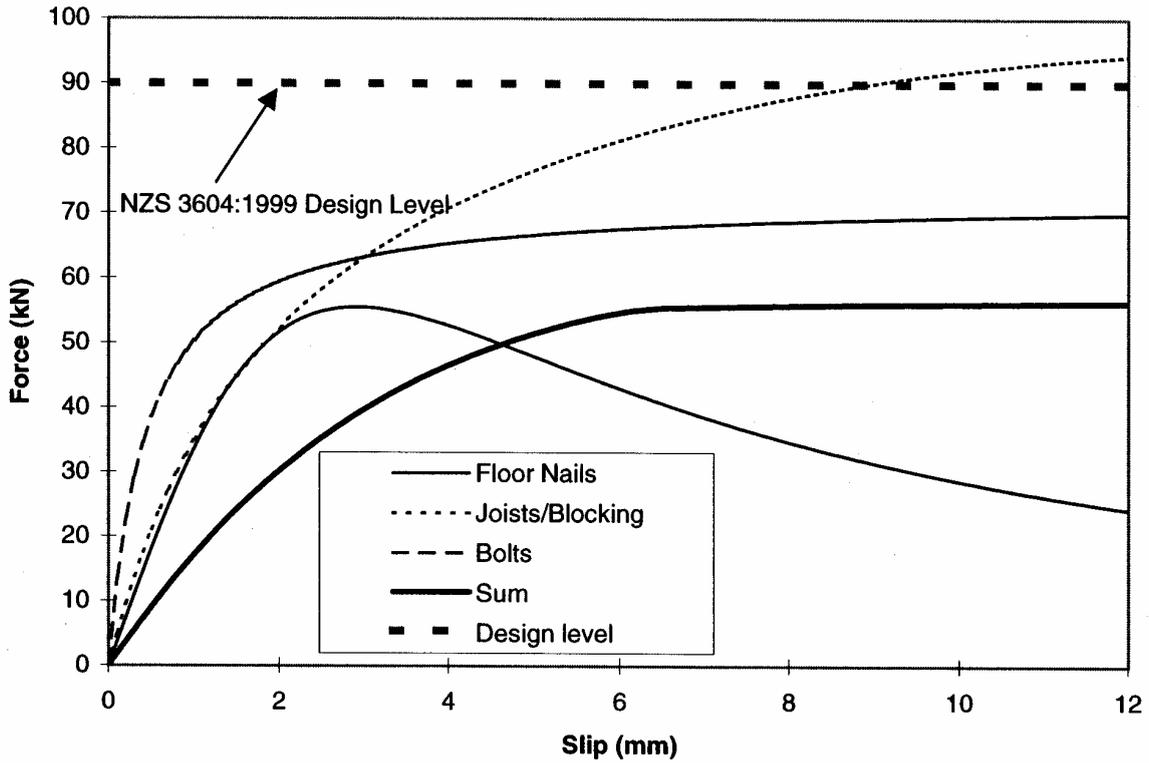
Figure A.8: Movement Between Wall and Floor – Force Parallel to Stringers
