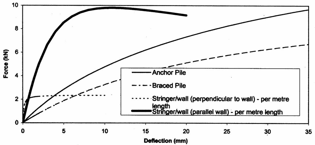
Figure 1. Plot of foundation element load versus slip relationship as defined by Table 1.
