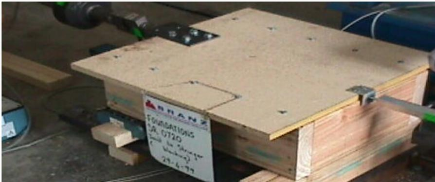
**Figure A.3: Load Perpendicular to Stringer With Blocking.**
