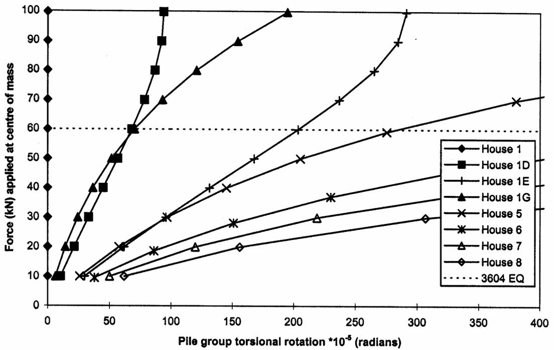
Figure 7. Floor rotation versus Y force – rectangular pile configuration
