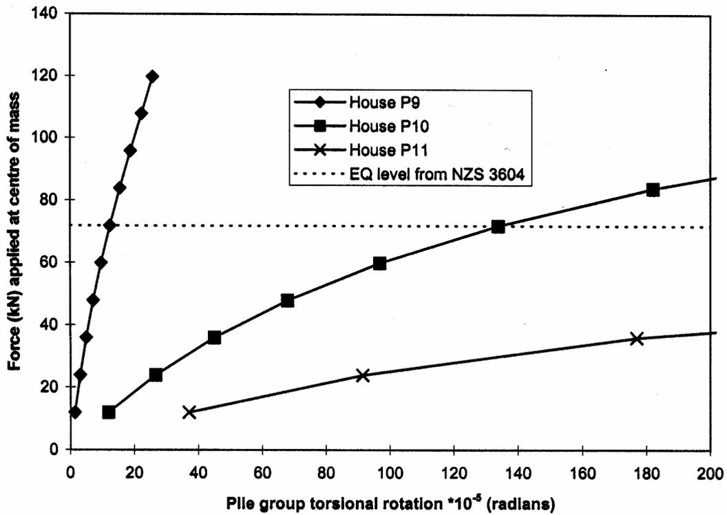
Figure 10. Floor rotation versus X force – “L” shaped house
