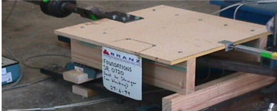
**Figure A.2: Load Perpendicular to Stringer Without Blocking**
