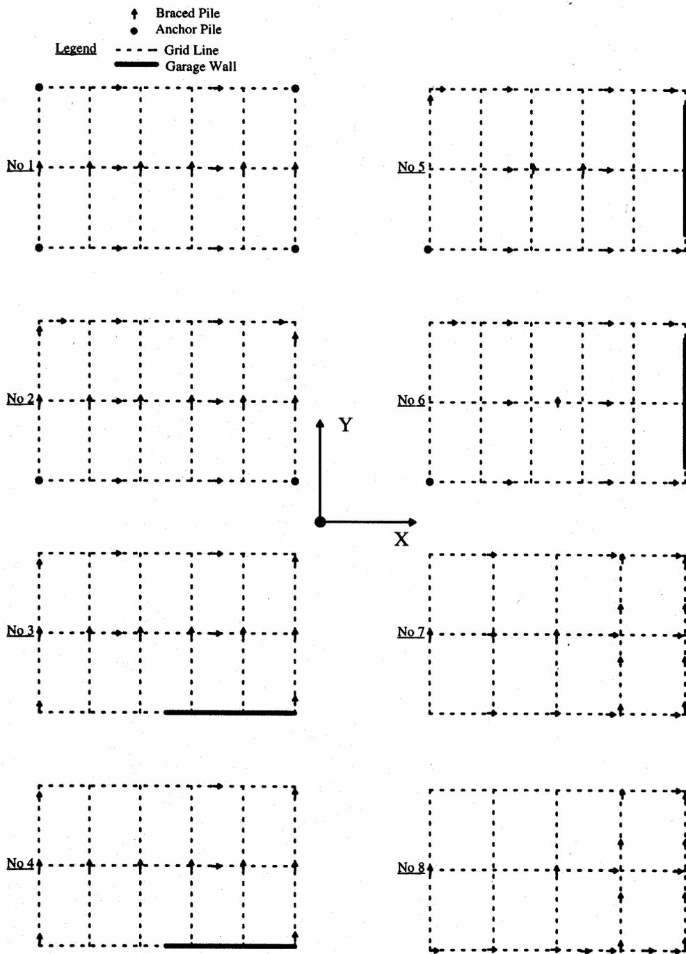
Figure 2. Pile configurations analysed for rectangular house
