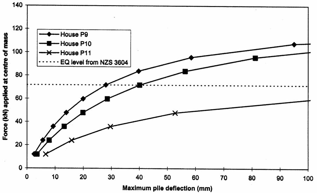
Figure 9. Maximum pile deflections versus X force – “L” shaped house
