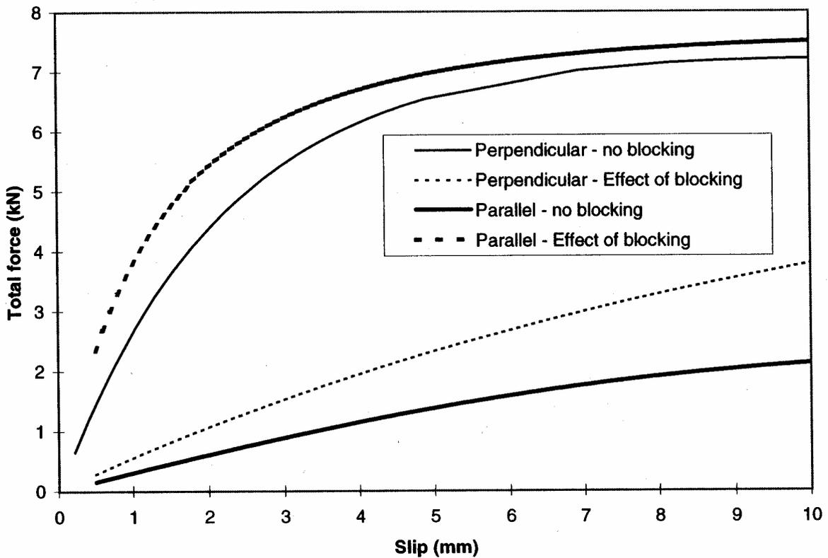
Figure A.7: Load Versus Deflection for Joists Perpendicular
