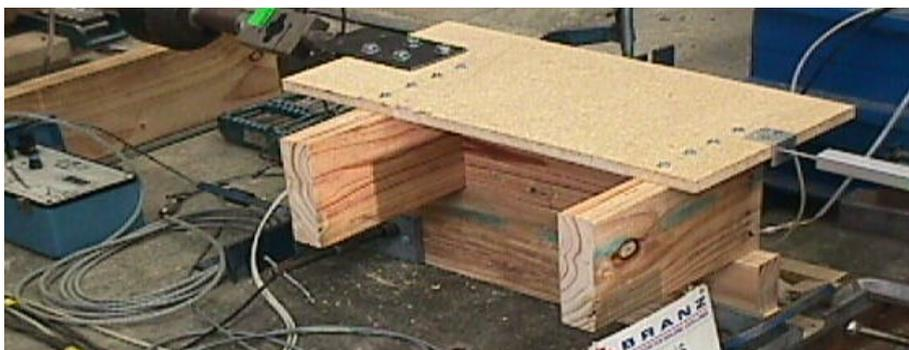
**Figure A.5 Load Parallel to Stringer With Blocking.**
