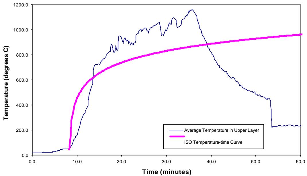
**Figure 8: Graph of room fire curve vs ISO Standard temperature-time**
