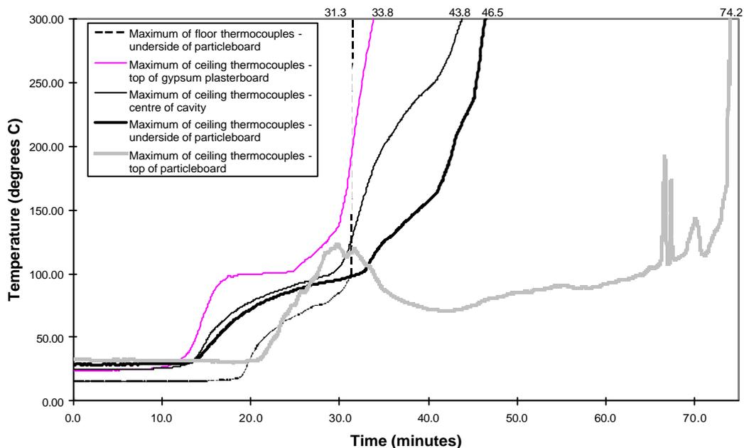
**Figure 14: Maximum thermocouple readings, time to exceed 300°C**
