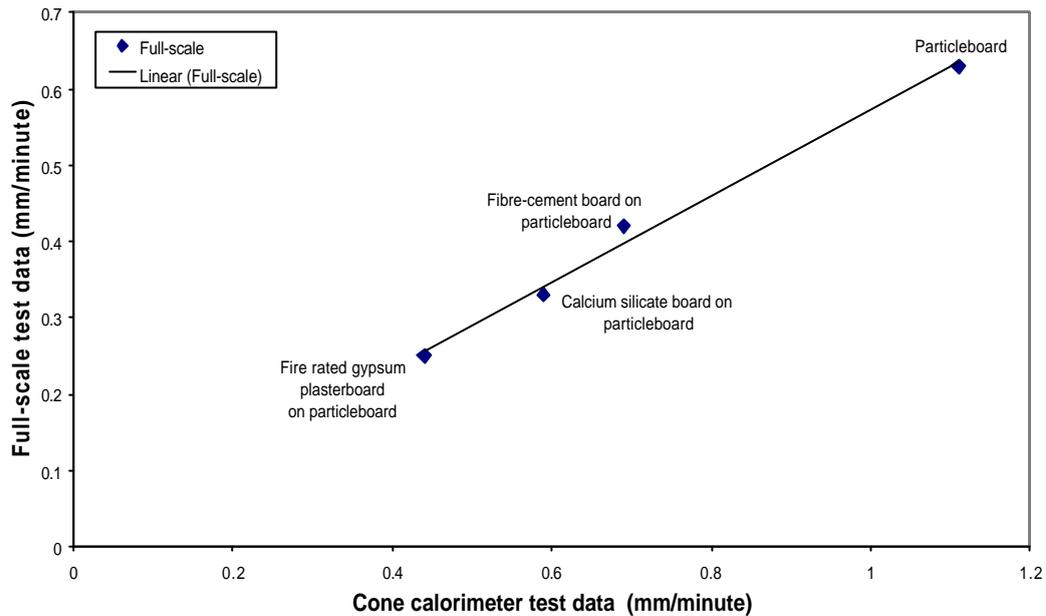
**Figure 15: Correlation between the effective charring rates determined from the cone calorimeter and the full-scale furnace tests, taking into account the initial delay time to reach 300 °C on the exposed surface**
