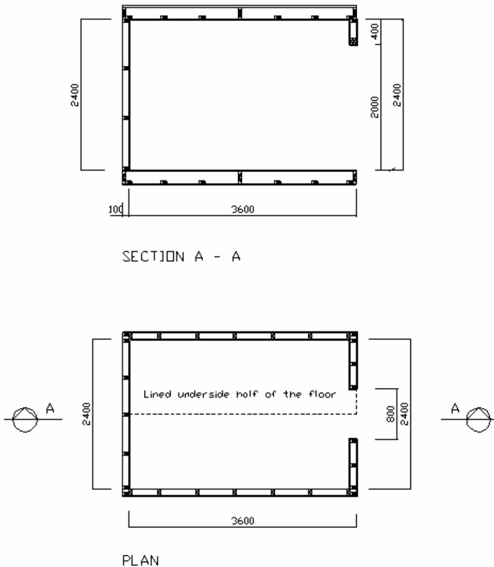
**Figure 1: Plan and section drawings of the room construction**
