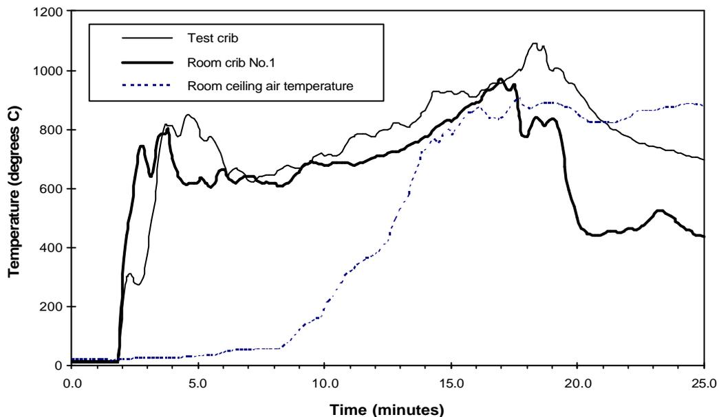
**Figure 10: Temperature-time curves comparing test crib temperatures with those for the first crib ignited in the full-scale room test, Crib No. 1**
