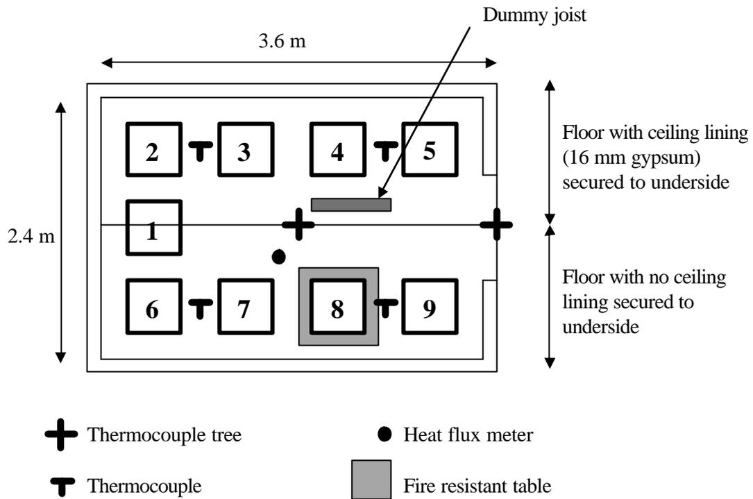
**Figure 3: Diagrammatic layout of the room**
