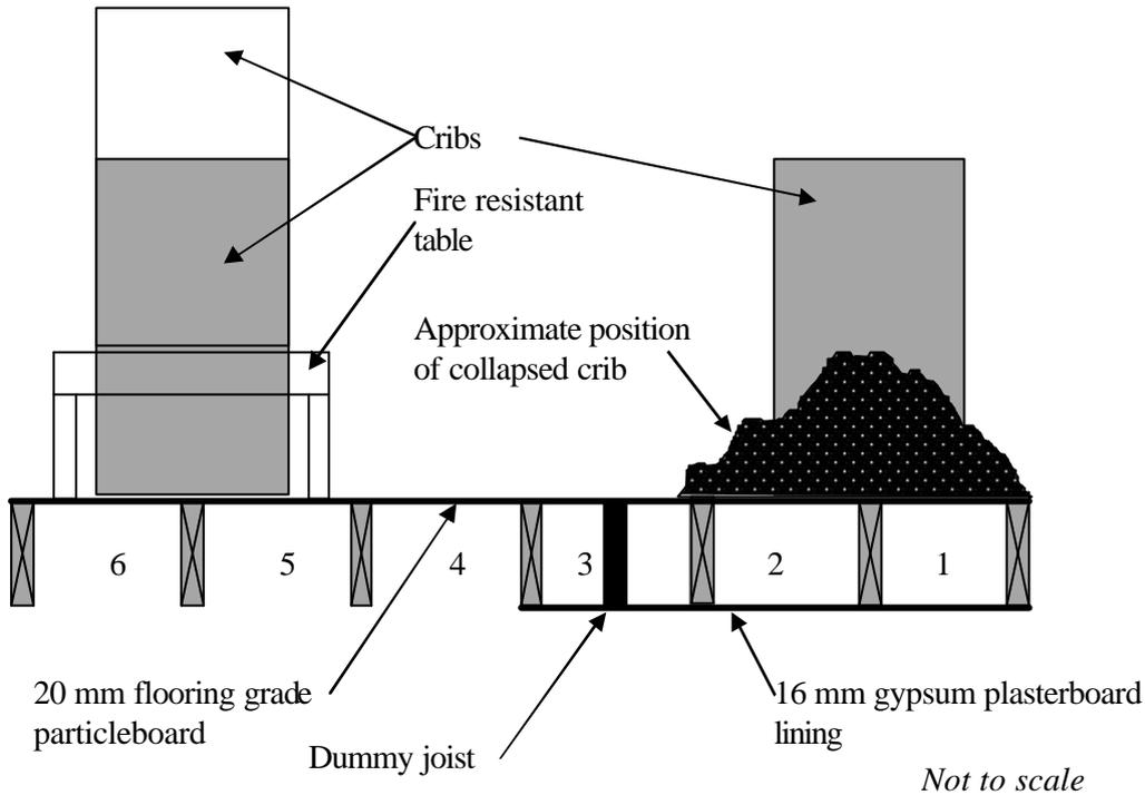
**Figure 12: Diagrammatic section through room**
