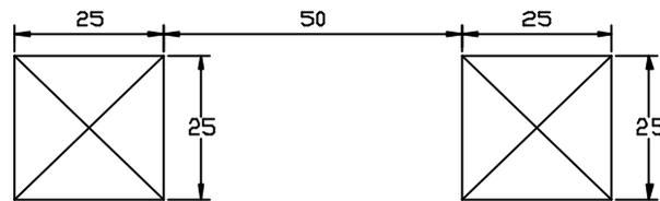
**Figure 2: Crib stick dimensions and spacings**
