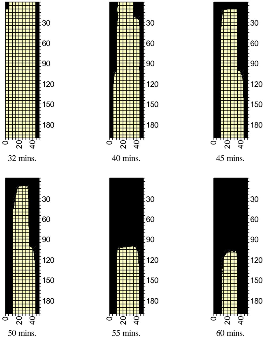
**Figure 13: Dummy joist char diagrams**
