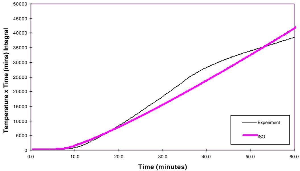
**Figure 9: Comparison of the temperature-time integral for the room fire curve with the ISO Standard temperature-time curve**
