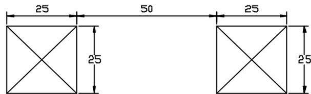
**Figure 2: Crib stick dimensions and spacings**
