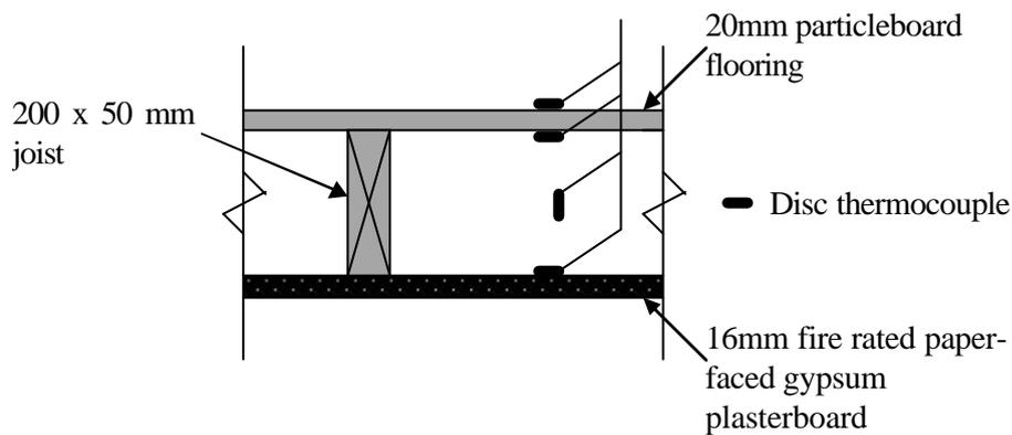
**Figure 5: Room ceiling instrumentation layout**
