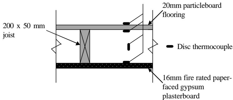
**Figure 5: Room ceiling instrumentation layout**
