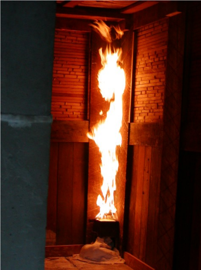
Figure 10-7: Fire test 20 seconds after ignition
