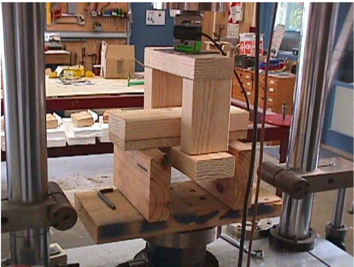
Figure 39. Test setup used to measure bottom plate to timber foundation beam tension strength.
