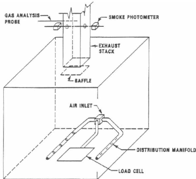
**Figure 59: A schematic of the layout used for testing armchairs in a room calorimeter. Extracted from (Schuhmann & Hartzell 1989).**
