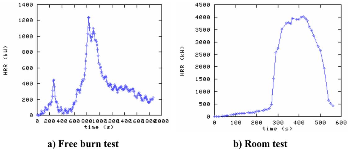
**Figure 44: Heat release rate profiles of a bedroom with plywood wall linings. Note the change in scale. Extract taken from (Lee 1985).**
