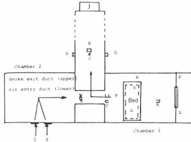
**Figure 45: Room-corridor arrangement used in the experiments by Paul. Extracted from (Paul 1989).**
