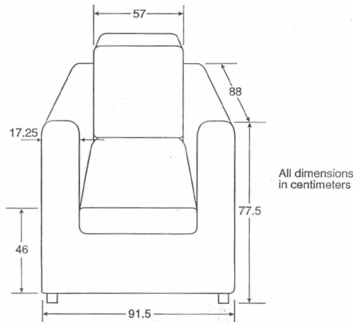
**Figure 60: Configuration of the full-scale chairs. Extracted from (Ohlemiller & Villa 1992).**
