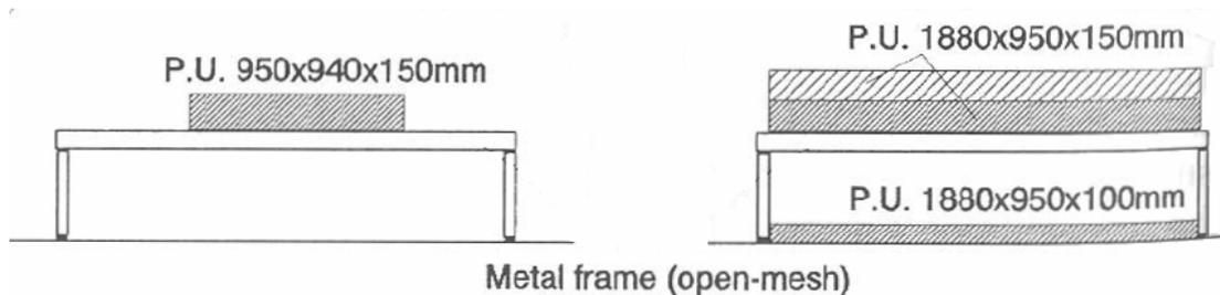
**Figure 48: Fuel configuration used by Luo and Beck. Extracted from (Luo & Beck 1996).**
