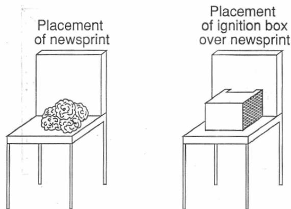
**Figure 61: TB 133 Ignition Source 1. Extracted from (Ohlemiller & Villa 1992).**
