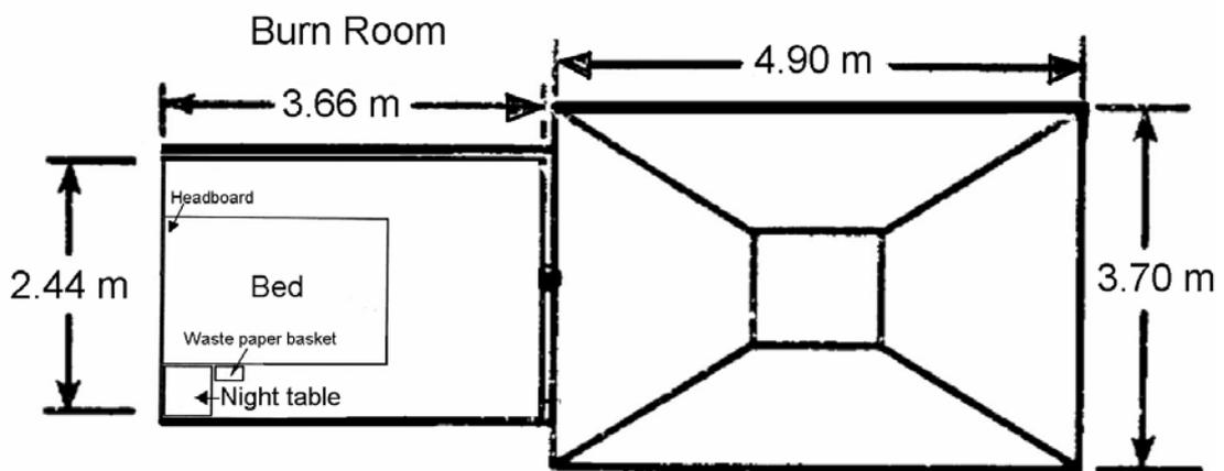
**Figure 43: Schematic of the set-up for the room tests conducted by Lee (Lee 1985).**
