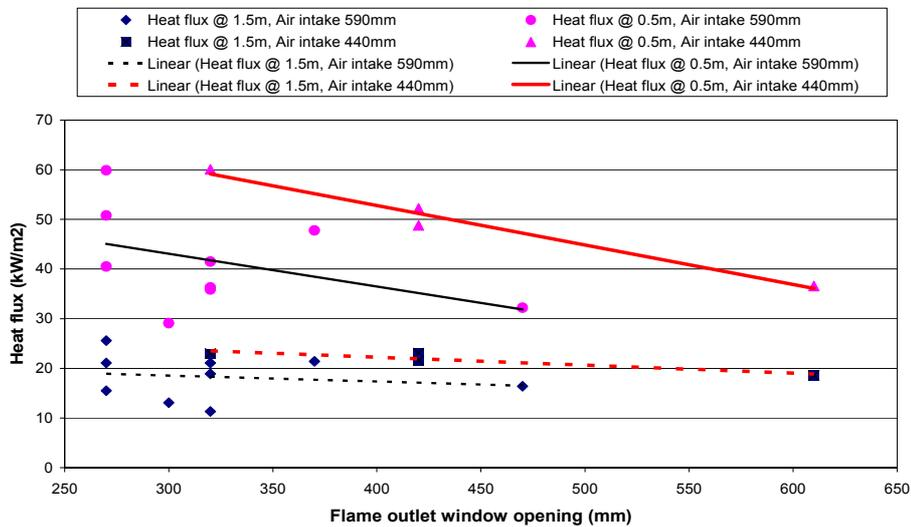
**Figure 4-2: Graph of heat flux vs flame outlet window opening height for two air intake opening heights.**
