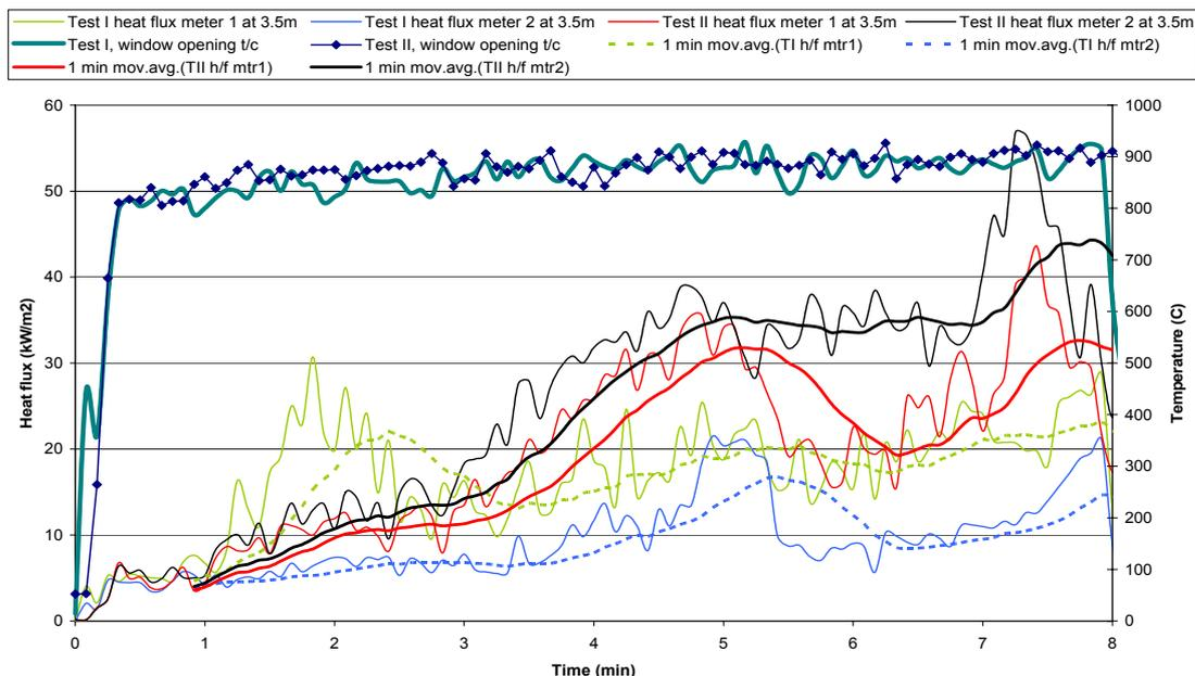
**Figure 7-4: Heat flux measurements from Plywood Tests I and II**
