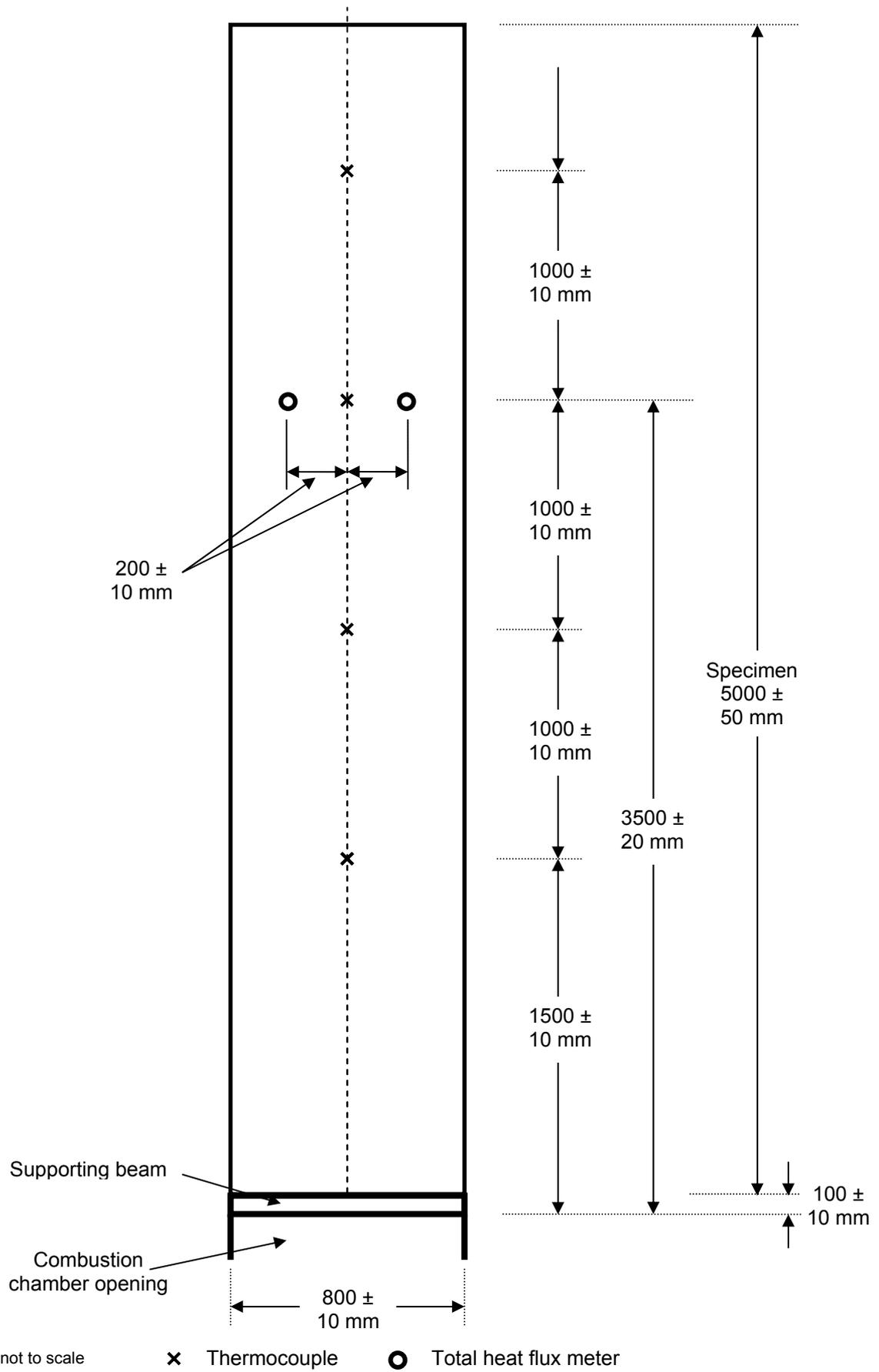
**Figure 11-6: Specimen dimensions and instrumentation layout – proposed by BRANZ**
