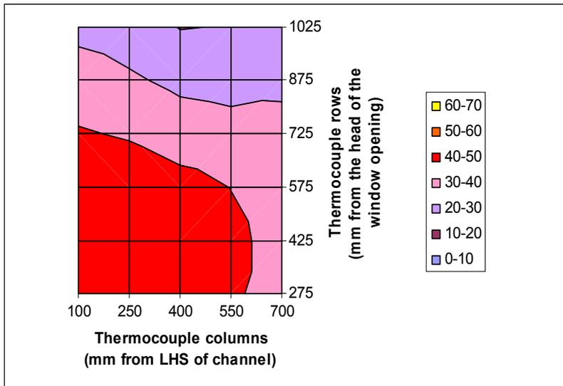
**Figure 5-7: Plate heat flux meter exposure plot after 1200 seconds, Calibration Test 2.**
