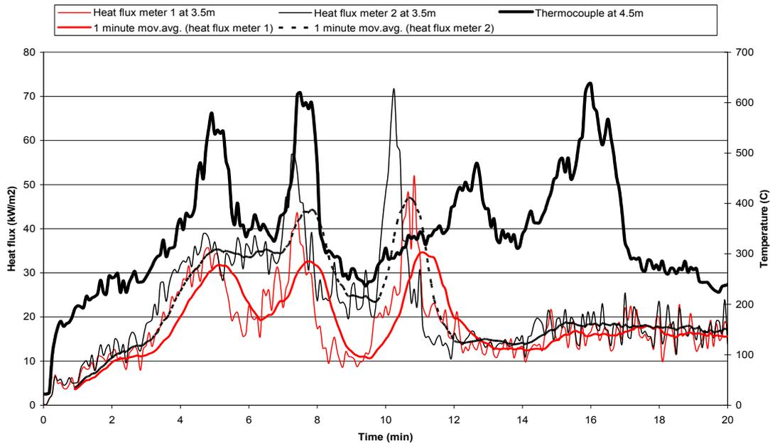
**Figure 7-3: Plywood Test II heat flux at 3.5 m and temperature at 4.5 m (channel height 5000 mm).**
