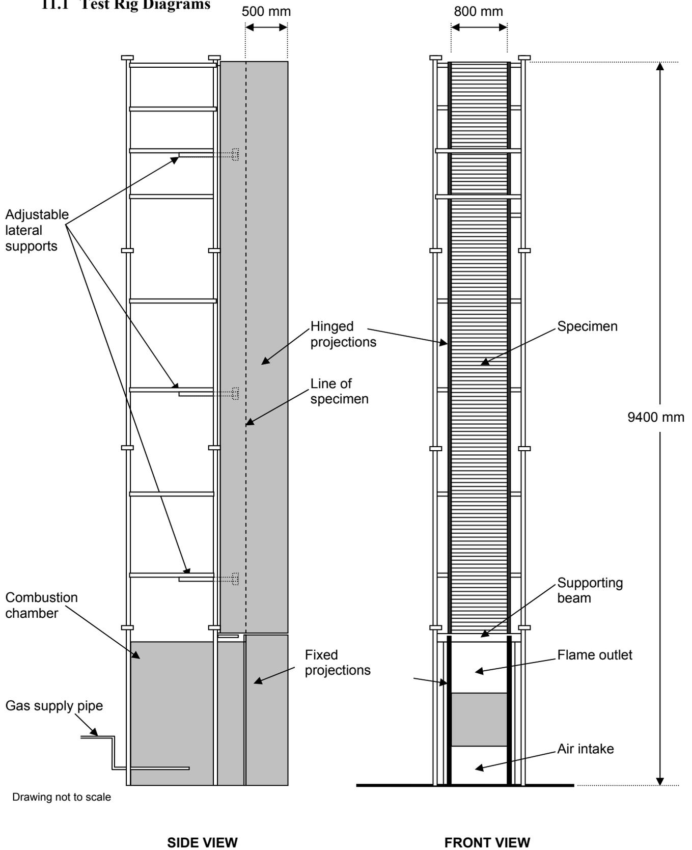
Figure 11-1: Test apparatus – original (ASTM, 1992)
