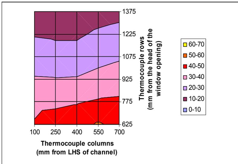
**Figure 5-9: Plate heat flux meter exposure plot after 1200 seconds, Calibration Test 1**
