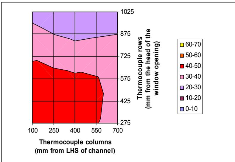
**Figure 5-6: Plate heat flux meter exposure plot after 900 seconds, Calibration Test 2.**
