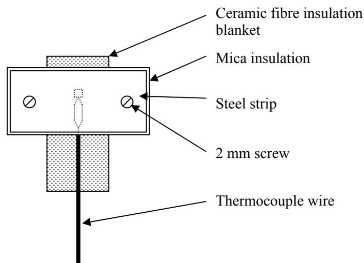
Figure 5-1: Typical plate thermocouple attachment (Dillon, 1998).
