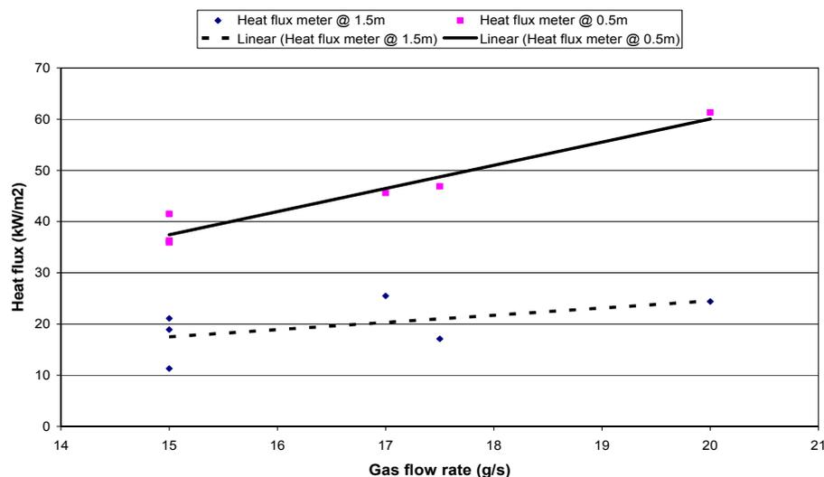
Figure 4-1: Graph of heat flux vs gas flow rate for fixed ventilation conditions.
