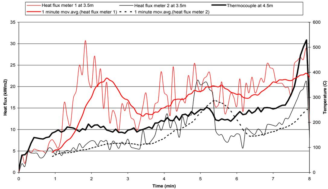
**Figure 7-2: Plywood Test I heat flux at 3.5 m and temperature at 4.5 m (channel height 7320 mm).**
