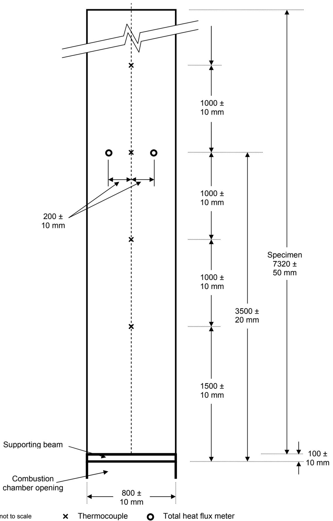
**Figure 11-5: Specimen dimensions and instrumentation layout – original (ASTM, 1992)**
