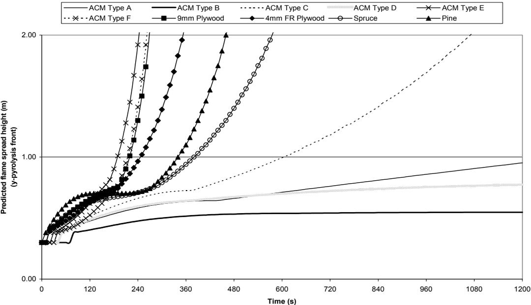
Figure 6-1: Predicted flame spread rates for several façade materials using the BRANZfire based model.
