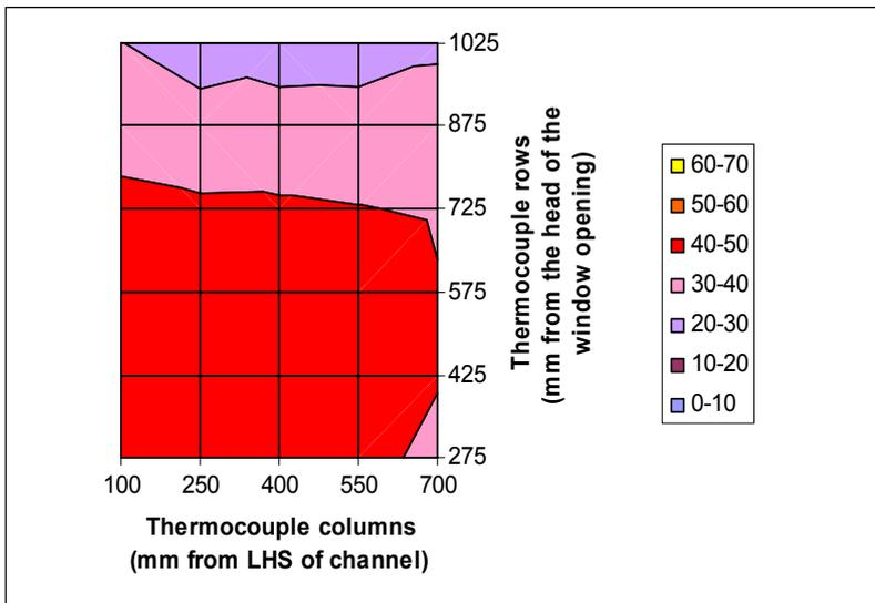
**Figure 5-4: Plate heat flux meter exposure plot after 300 seconds, Calibration Test 2.**
