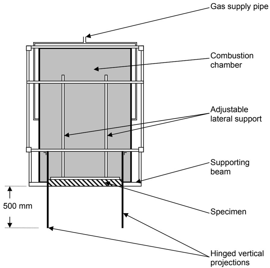
**Figure 11-3: Horizontal cross-section above combustion chamber (ASTM, 1992)**
