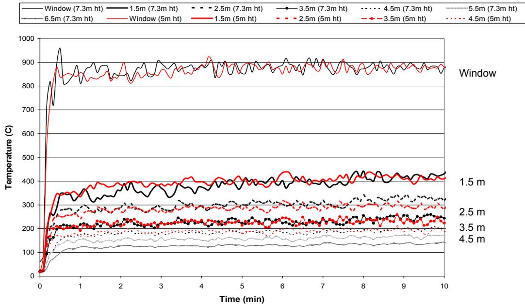
**Figure 7-1: Comparison of calibration tests thermocouple data for 7320 mm and 5000 mm channel heights.**
