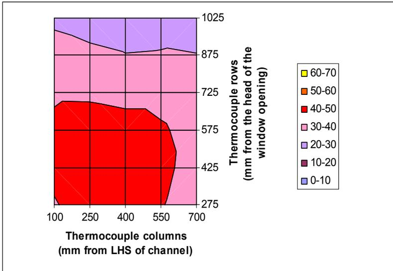
**Figure 5-5: Plate heat flux meter exposure plot after 600 seconds, Calibration Test 2.**
