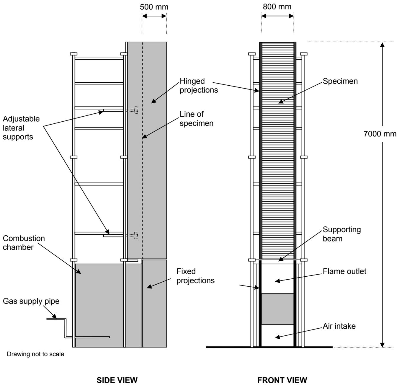
**Figure 11-2: Test apparatus – proposed by BRANZ**
