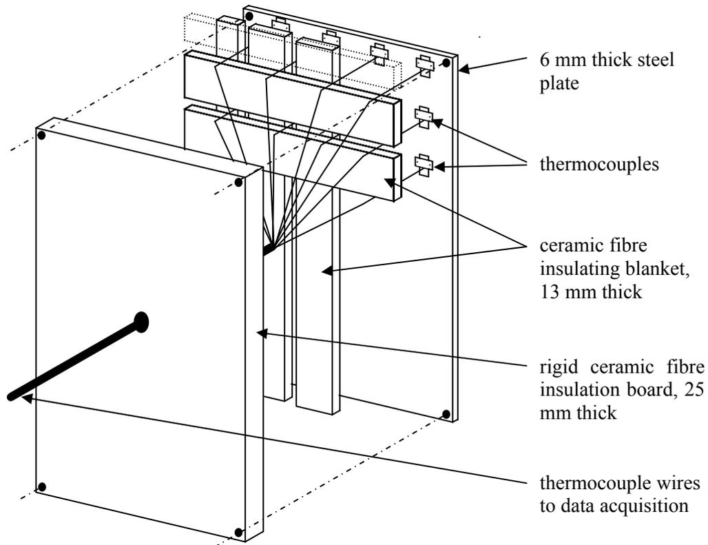
**Figure 5-2: Heat flux plate assembly (Dillon, 1998).**
