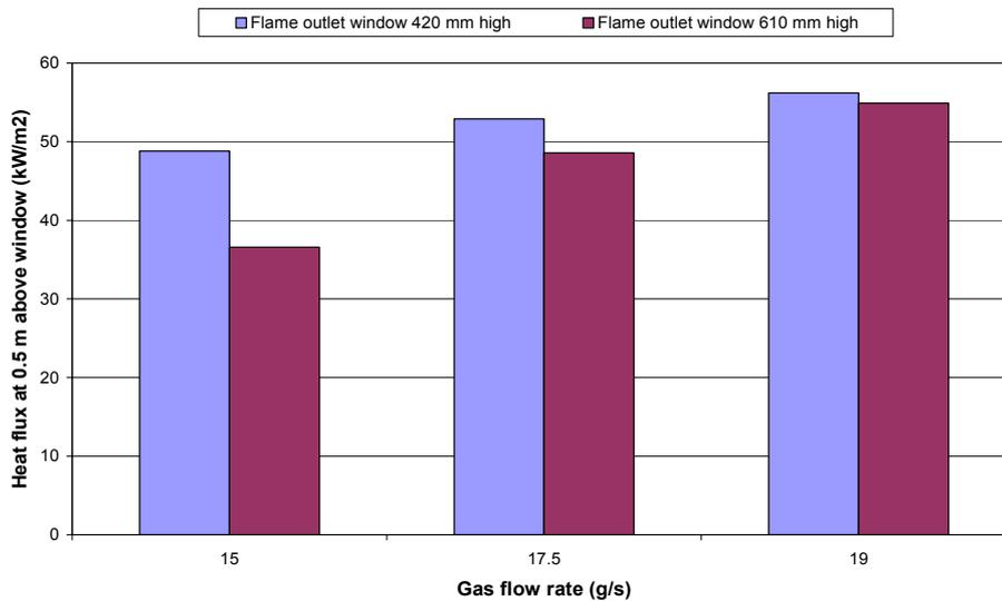
**Figure 4-4: Received heat flux vs gas flow rate for two heights of flame outlet window with 800 mm wide outlet and 440 mm high air intake.**
