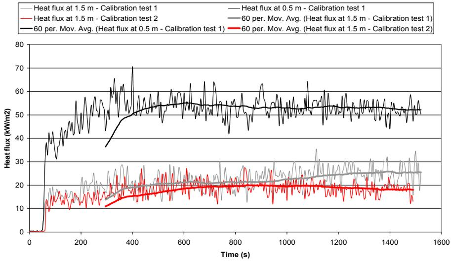
**Figure 5-3: Medtherm heat flux meter measurements during calibration testing of the plate heat flux meter.**
