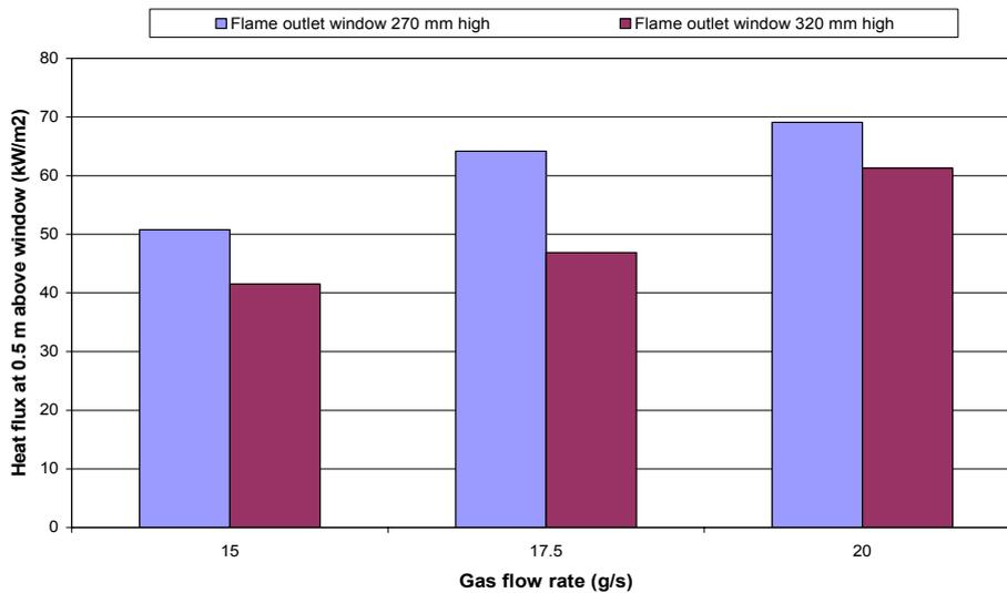
**Figure 4-3: Received heat flux vs gas flow rate for two flame outlet window heights with 800 mm wide outlet and 590 mm high air intake.**
