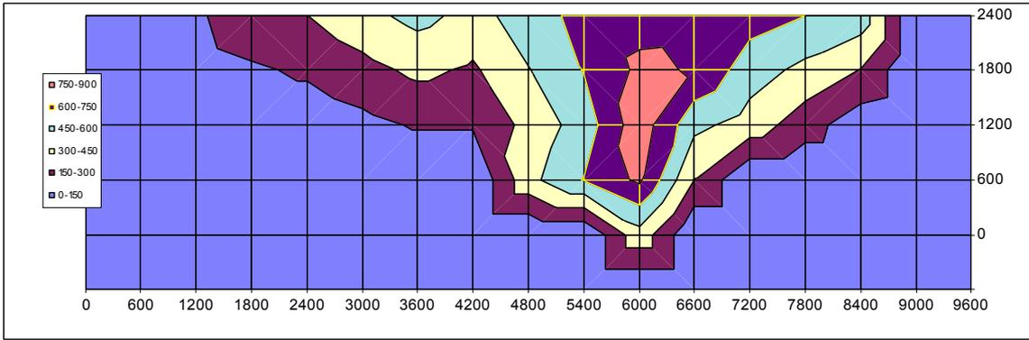
**Figure 26: Temperature contours in walls of test PIP 2 at end of test 11:51**
