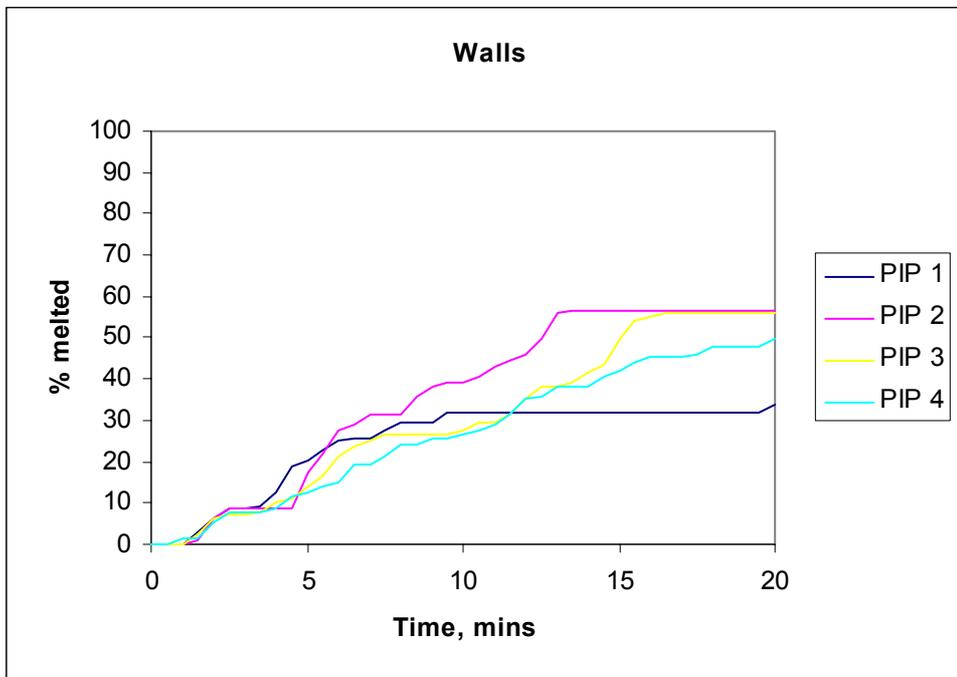
**Figure 9: Percentage melted EPS in wall cavities**
