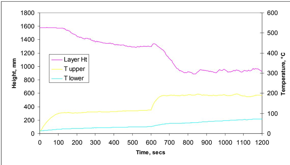
**Figure 44: Fire conditions in room space in PIP 4**
