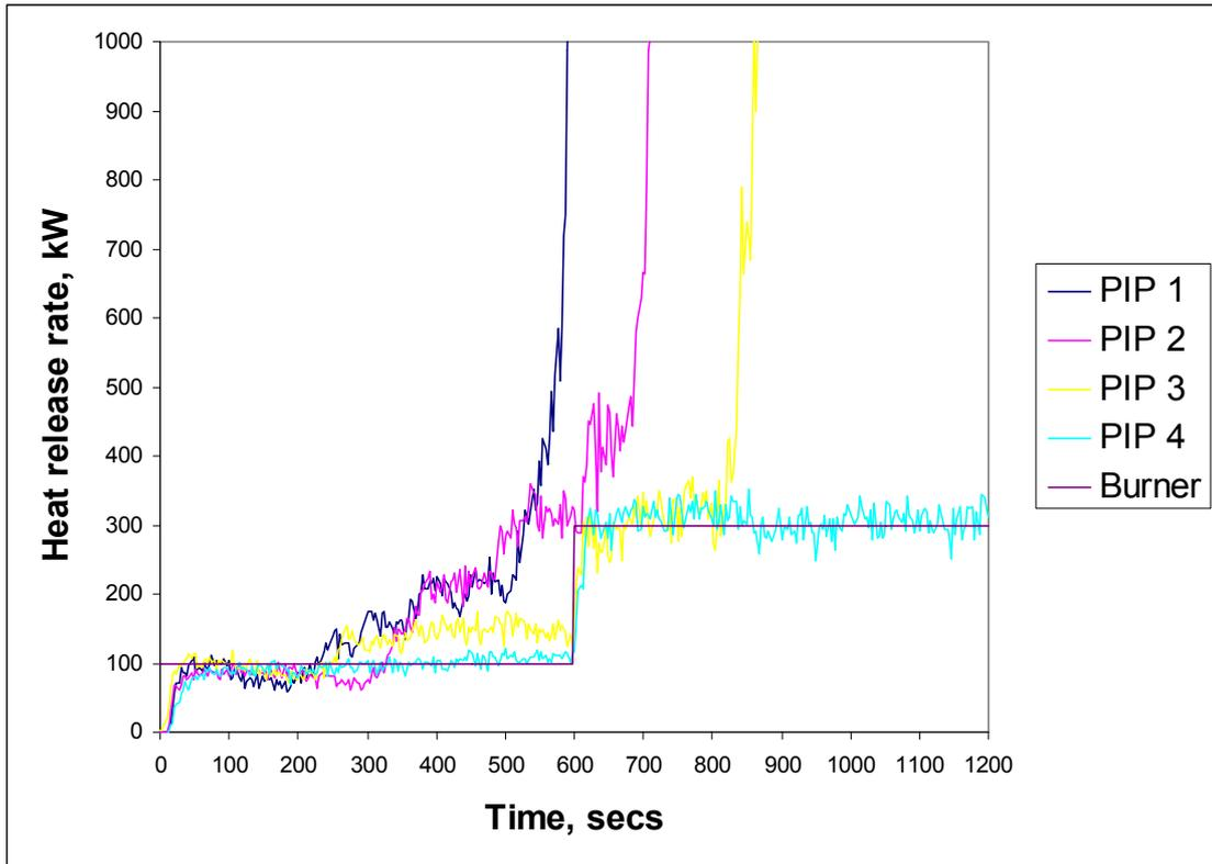
**Figure 4: Heat release rates of each test**
