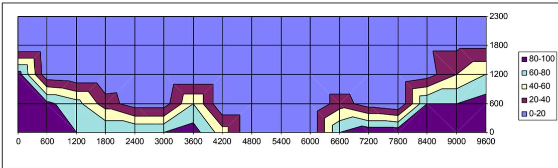
**Figure 17: Depth of foam at end of test PIP 3 after 15 minutes**
