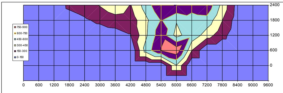
**Figure 25: Temperature contours in walls of test PIP 2 at 10 minutes**
