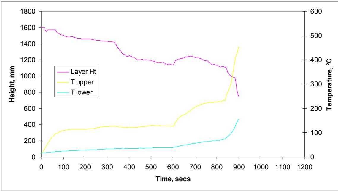
**Figure 43: Fire conditions in room space in PIP 3**
