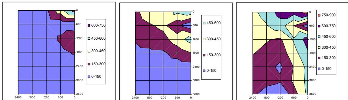
**Figure 33: Temperature contours in ceiling of test PIP 3 at 5 minutes**
