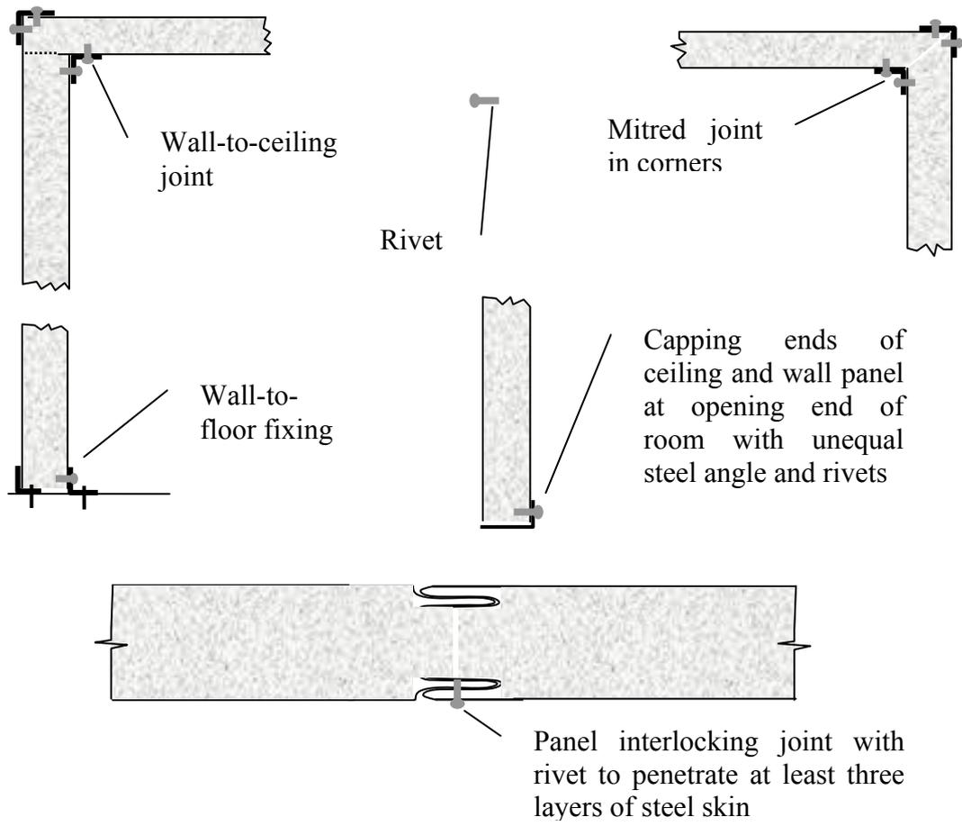
**Figure 3: Panel assembly details**
