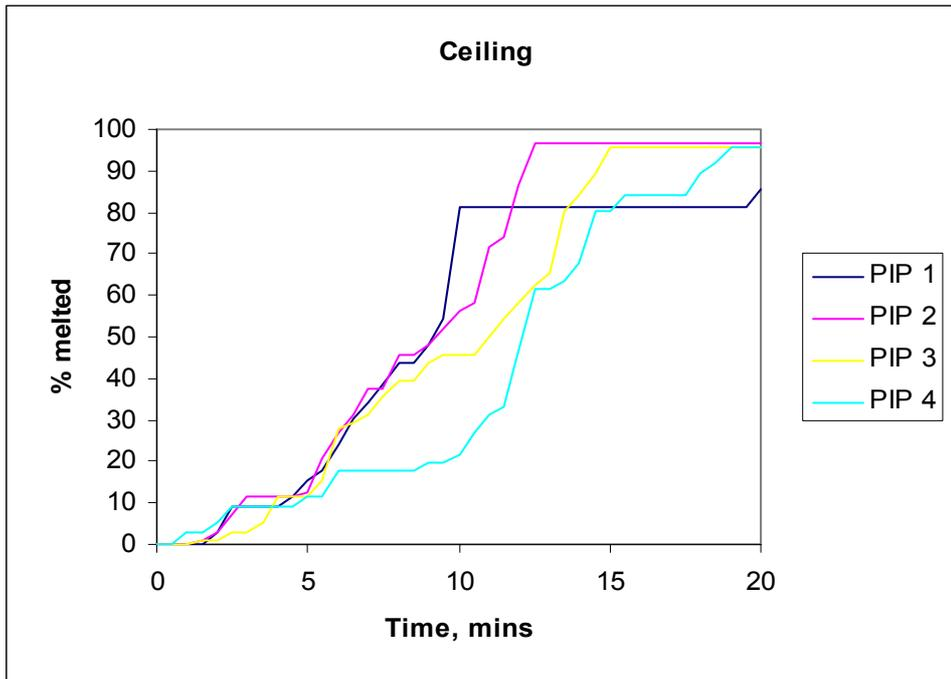
**Figure 10: Percentage melted EPS in ceiling cavity**
