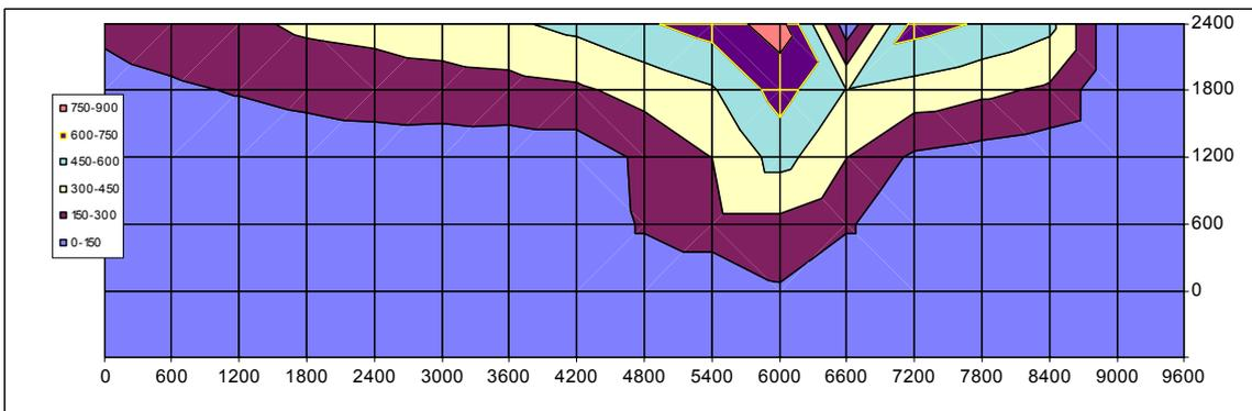
**Figure 31: Temperature contours in walls of test PIP 3 at end of test 14:21**
