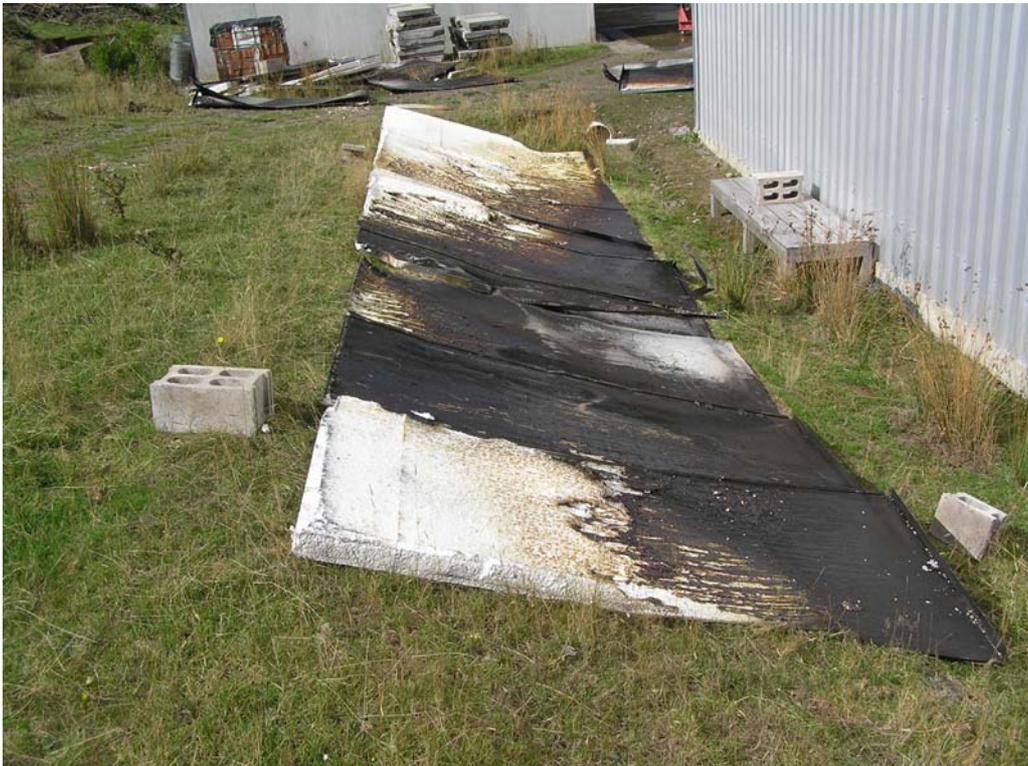
**Figure 27: EPS core in walls remaining at the end of test PIP 2**
