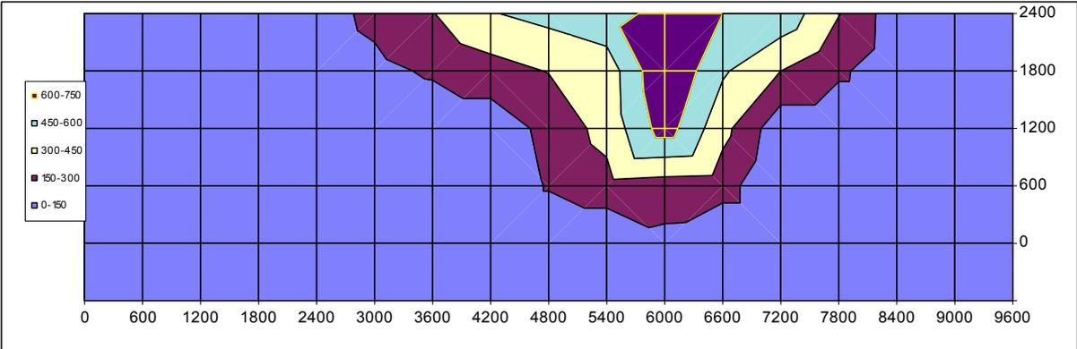
Figure 20: Temperature contours in walls of test PIP 1 at 10 minutes
