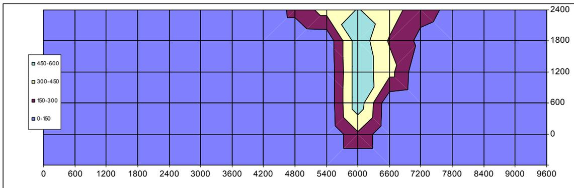
**Figure 34: Temperature contours in walls of test PIP 4 at 5 minutes**
