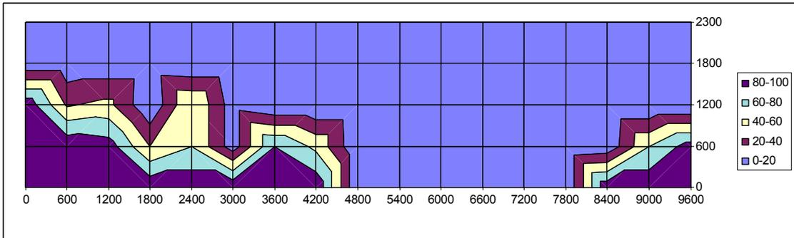
**Figure 16: Depth of foam at end of test PIP 2 after 12 minutes**
