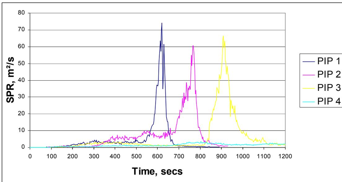
**Figure 5: Smoke production rate**
