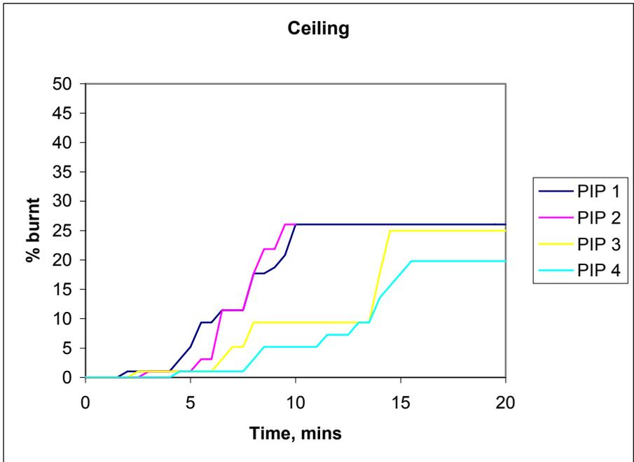
Figure 12: Percentage core burnt in ceiling
