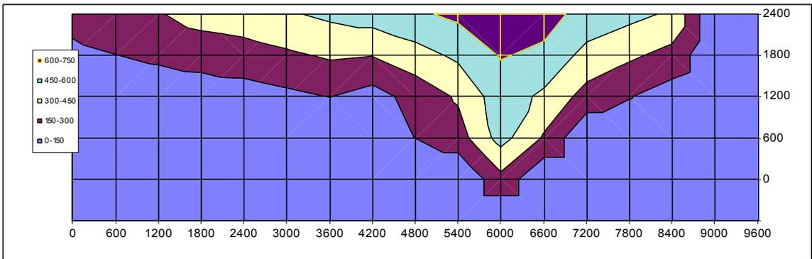
**Figure 37: Temperature contours in walls of test PIP 4 at 20 minutes**
