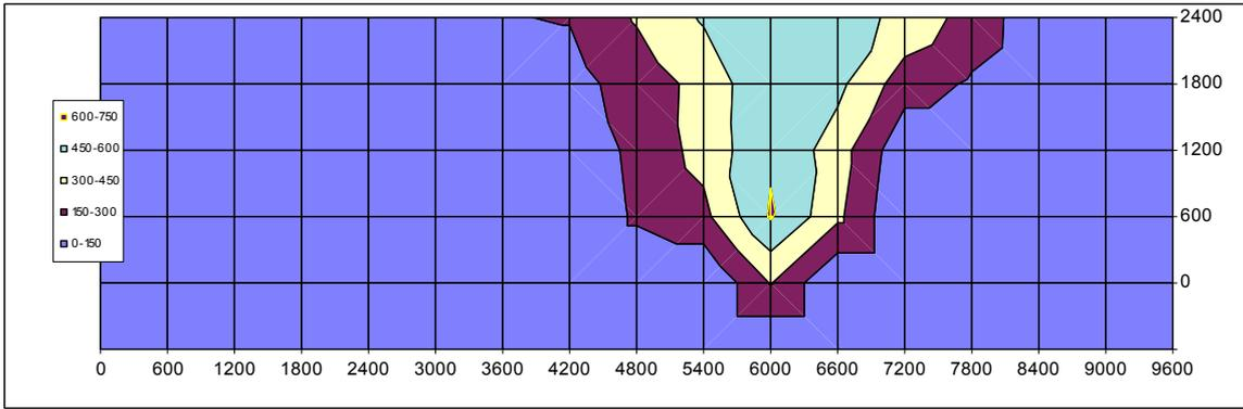
**Figure 35: Temperature contours in walls of test PIP 4 at 10 minutes**
