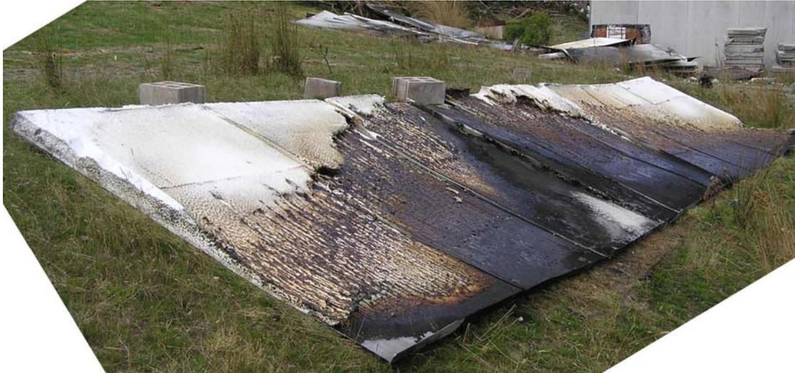
**Figure 32: EPS core in walls remaining at the end of test PIP 3**
