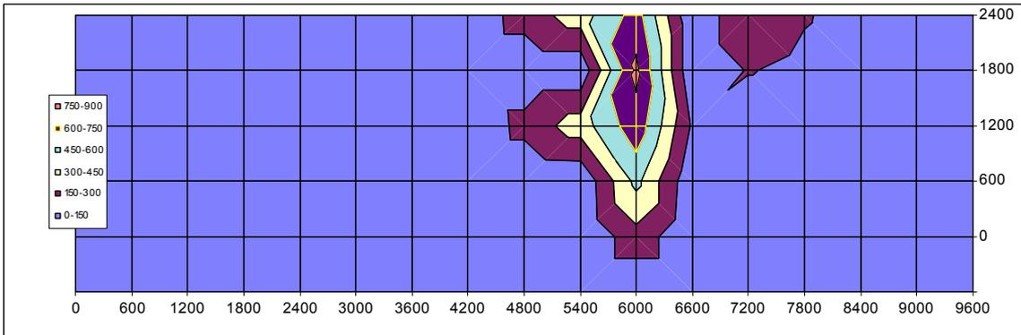
**Figure 29: Temperature contours in walls of test PIP 3 at 5 minutes**
