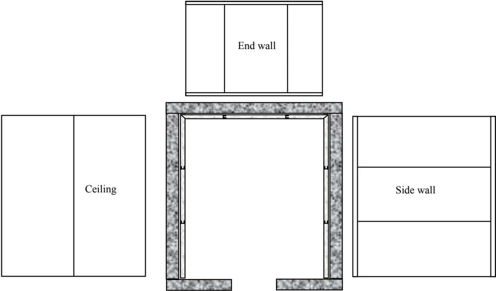
Figure 2: Assembly of test specimen, layout of panels
