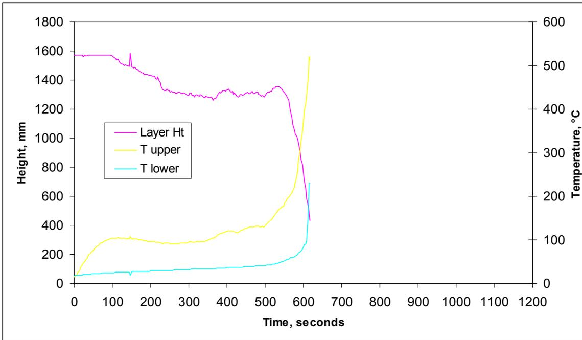
**Figure 41: Fire conditions in room space in PIP 1**
