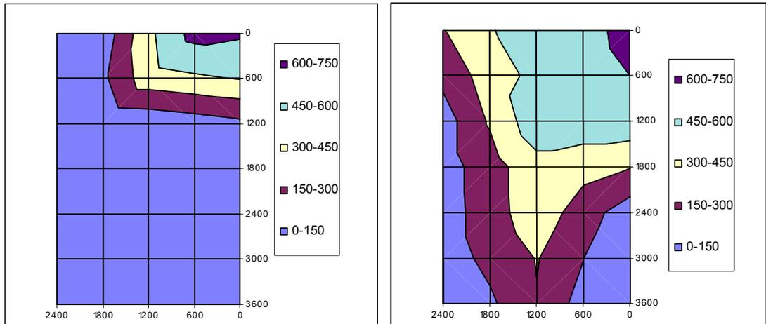
**Figure 22: Temperature contours in ceiling of test PIP 1 at 5 and 10 minutes**
