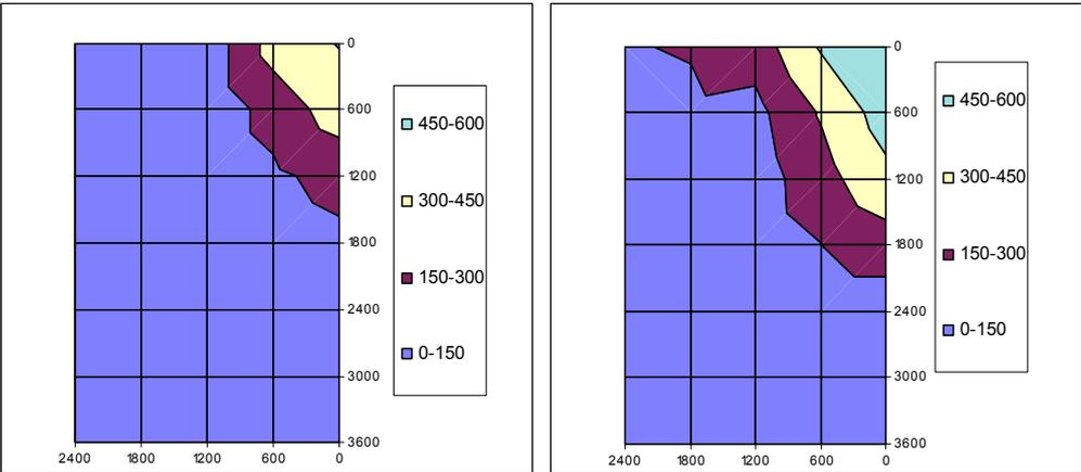
**Figure 39: Temperature contours in ceiling of test PIP 4 at 5 and 10 minutes**
