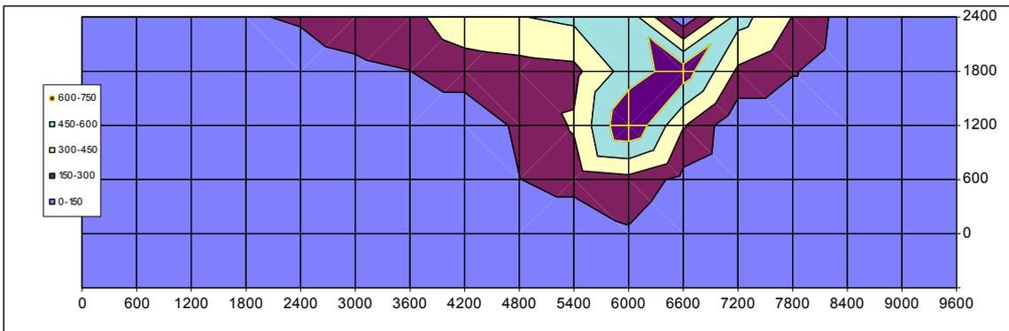
**Figure 30: Temperature contours in walls of test PIP 3 at 10 minutes**
