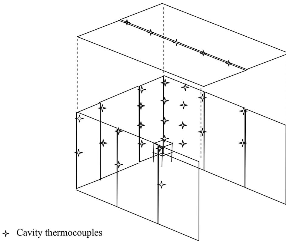
**Figure 8: Cavity thermocouples**
