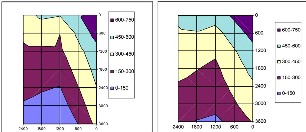
Figure 40: Temperature contours in ceiling of test PIP 4 at 15 and 20 minutes
