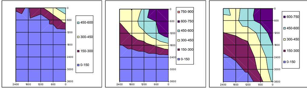
**Figure 28: Temperature contours in ceiling of test 2 at 5, 10 minutes and end of test**
