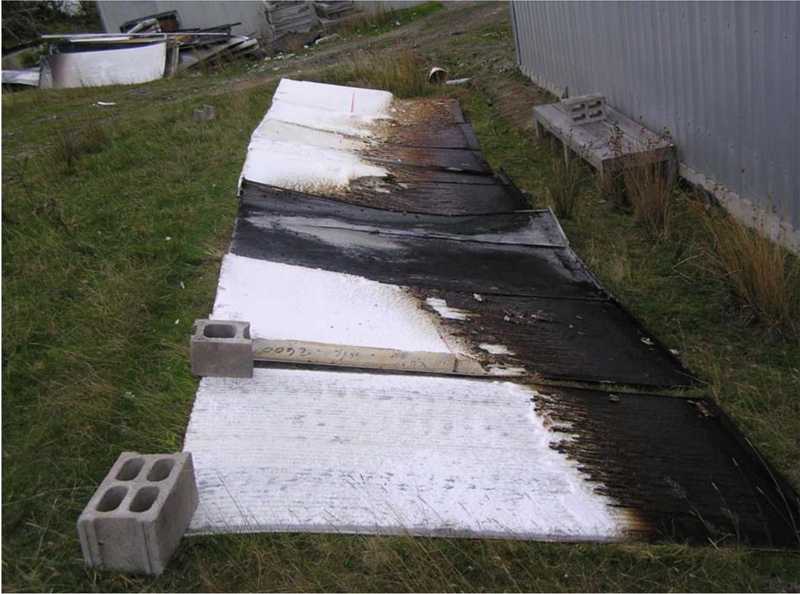
**Figure 38: EPS core in walls remaining at the end of test PIP 4**
