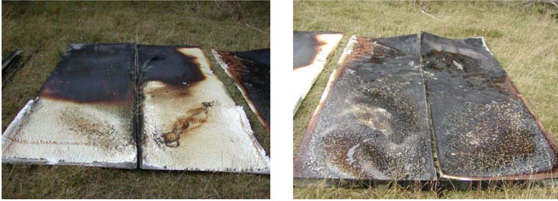
**Figure 23: EPS core remaining in the ceiling at end of test PIP 1, upper steel skins on left and lower fire exposed skins on right**
