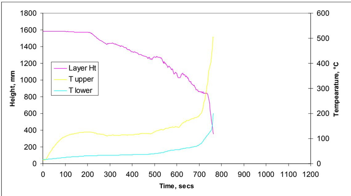
**Figure 42: Fire conditions in room space in PIP 2**
