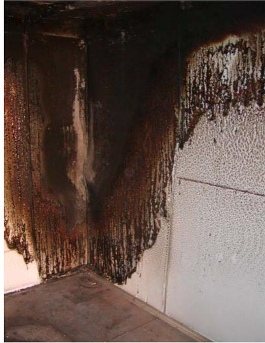
**Figure 21: EPS core remaining in the burner corner after test PIP 1, with exposed skins removed**
