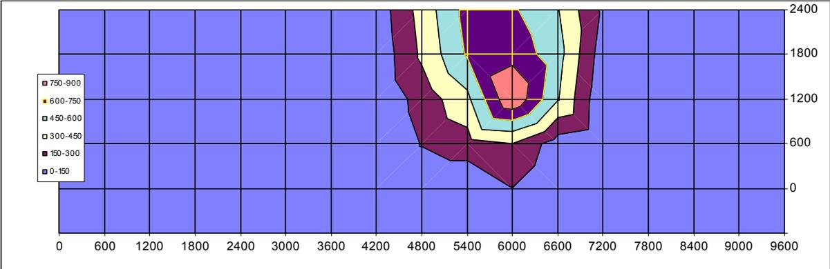
Figure 19: Temperature contours in walls of test PIP 1 at 5 minutes
