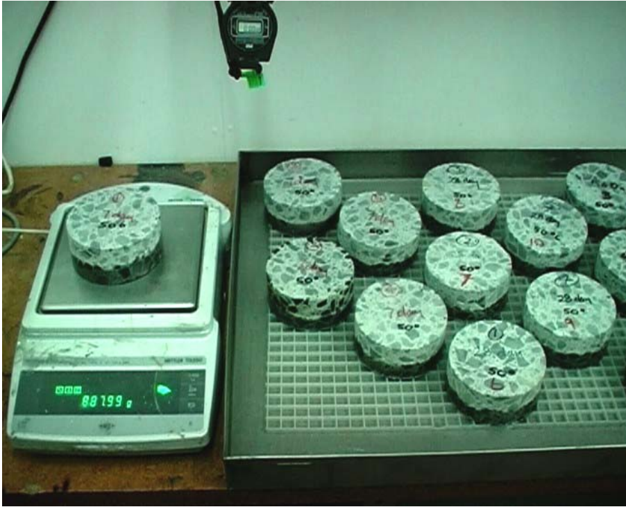
Figure 30: Sorptivity testing in practice
