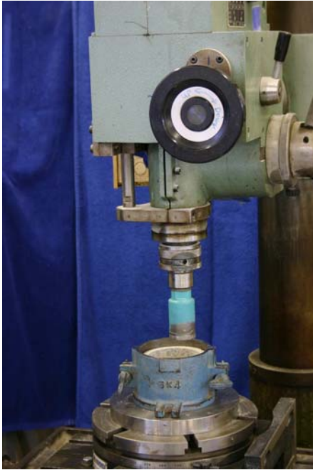
Figure 4: Profile grinding of a concrete core using a vertical mill
