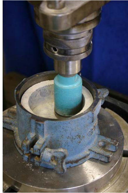
Figure 4: Profile grinding of a concrete core using a vertical mill
