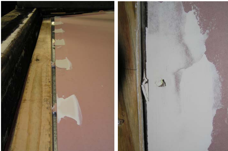
Figure 40: FR3362F displacement of side studs at 40 mm drift
