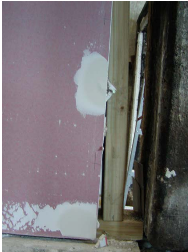
Figure 30: Racking of wall FR3362B
