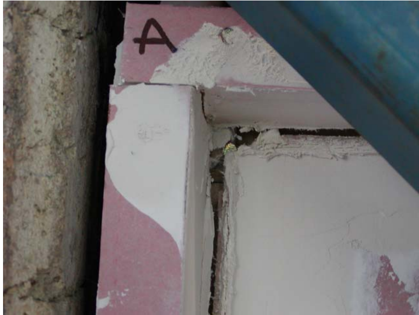
Figure 33: Lining separation in corner at maximum drift
