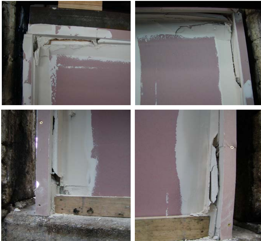
Figure 38: Damage to corners of exposed side of FR3362E
