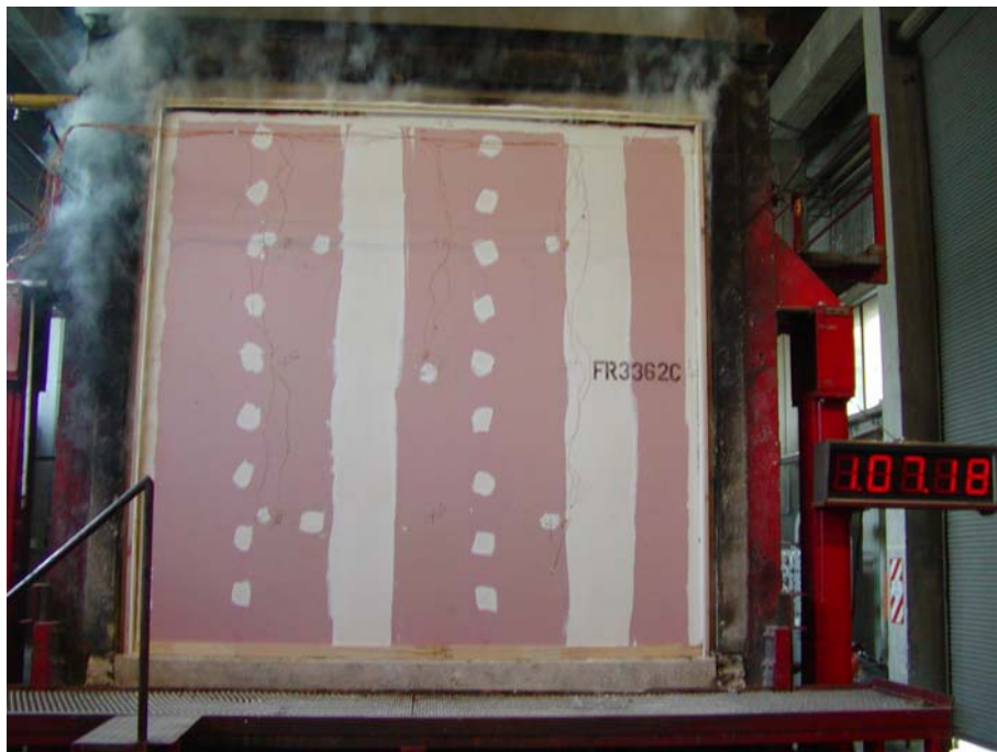
Figure 53: FR3362C at 67 minutes, the time of insulation failure
