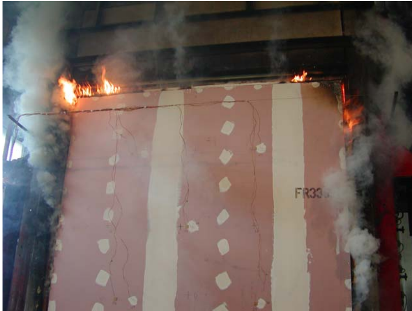
Figure 50: Flaming at top edge FR3362B 60 minutes, previously failed at bottom corner 34 minutes
