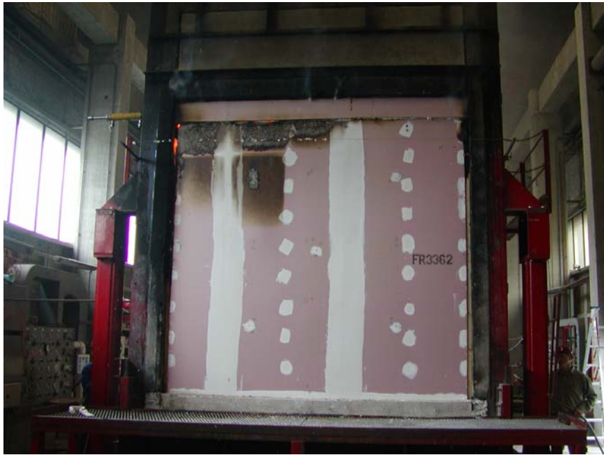
Figure 47: Non-exposed face of FR3362A at conclusion of test 53 minutes
