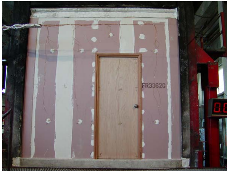
Figure 67: FR3362G at start of test
