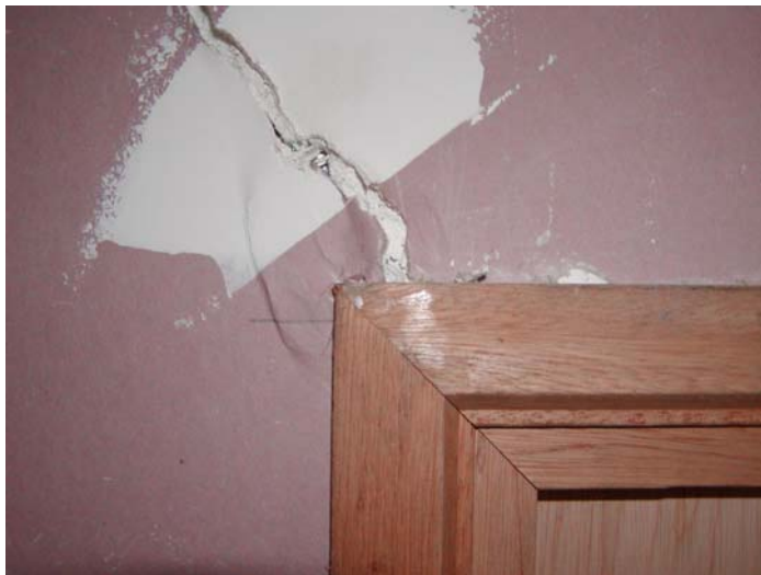
Figure 43: Racking of wall and door FR3362G door frame corner non-fire exposed side
