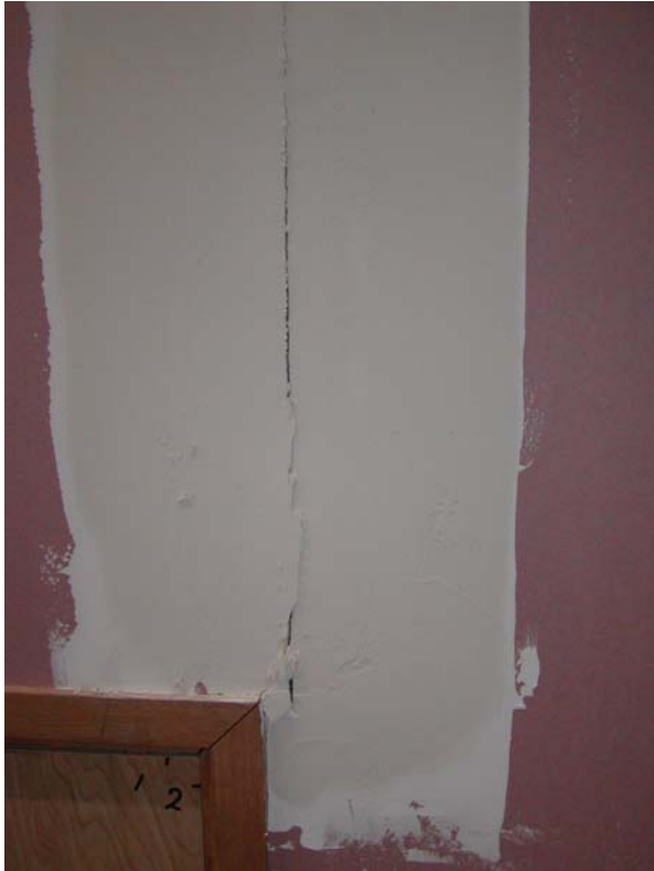
Figure 42: Racking of wall and door FR3362G door frame corner fire exposed side
