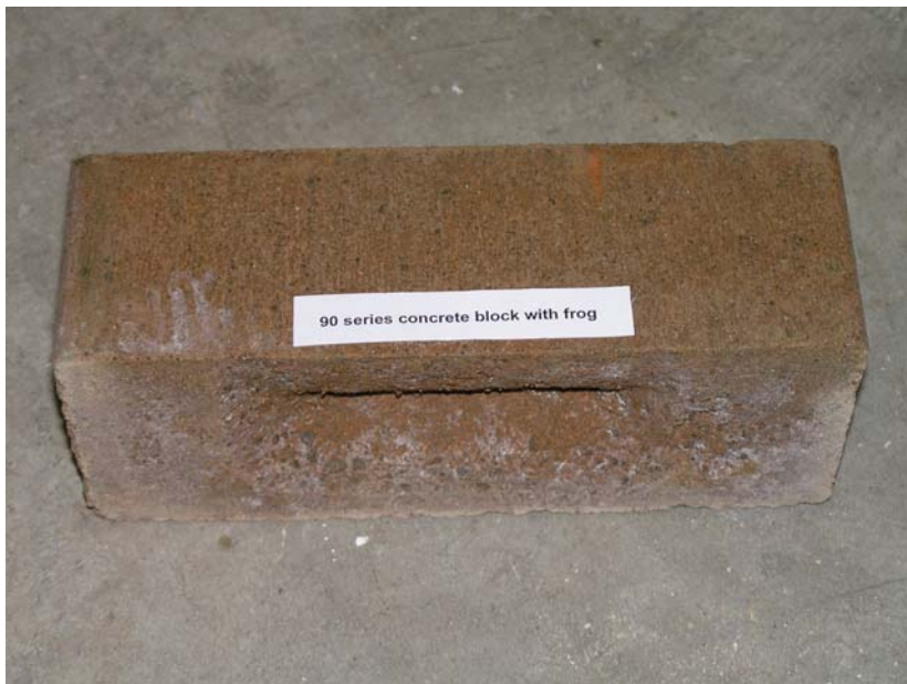
Figure 5:. 90 series concrete block with “frog”
