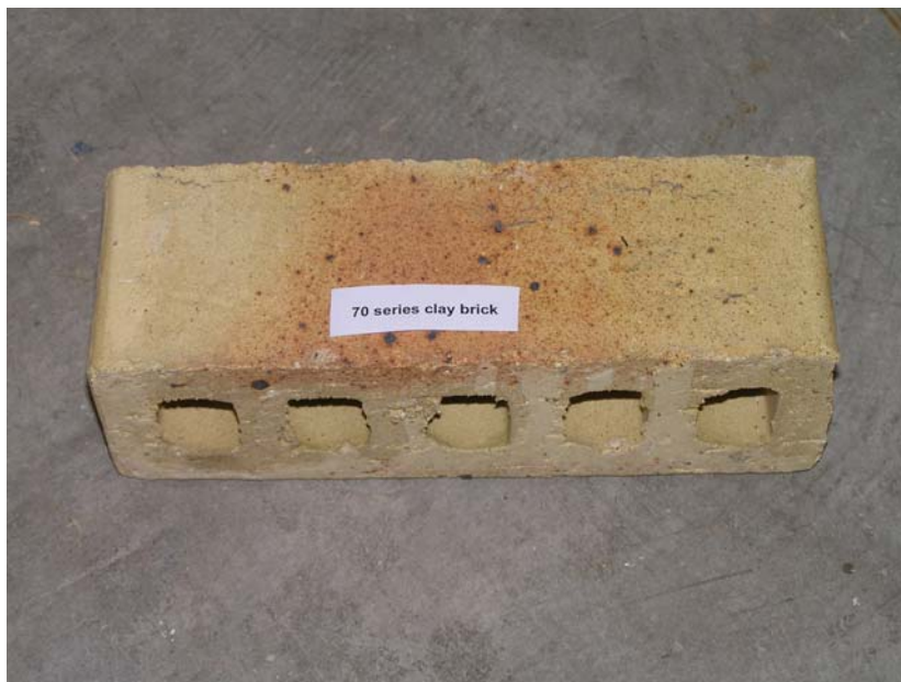
Figure 1: 70 series clay brick with holes
