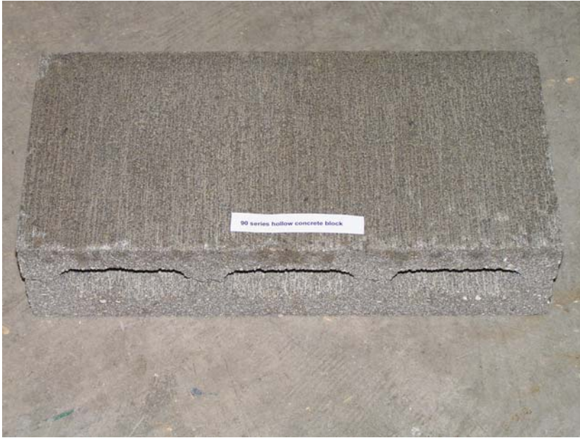
Figure 6: 90 series concrete block with slots
