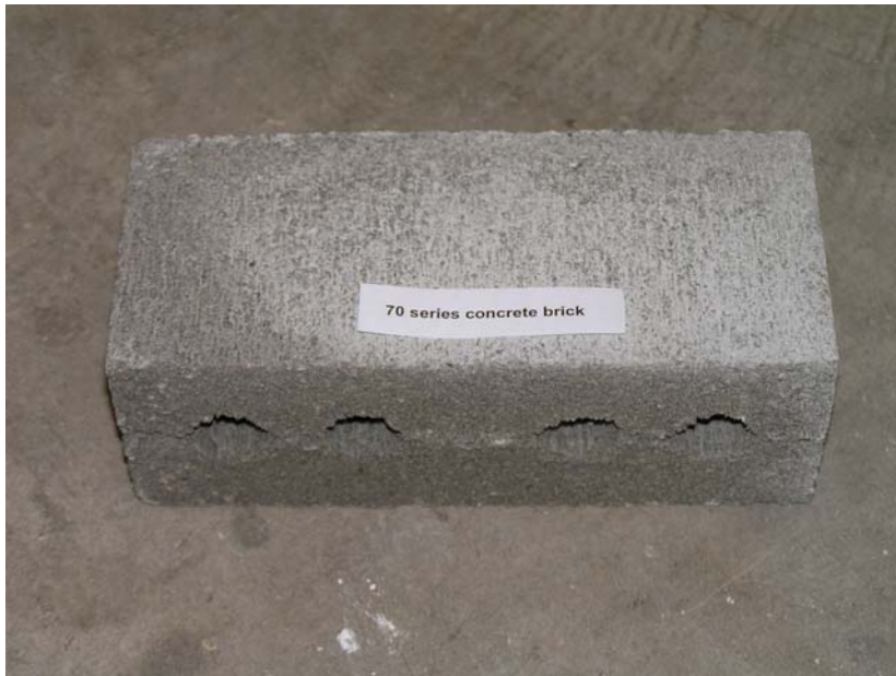
Figure 2: 70 series concrete block with holes
