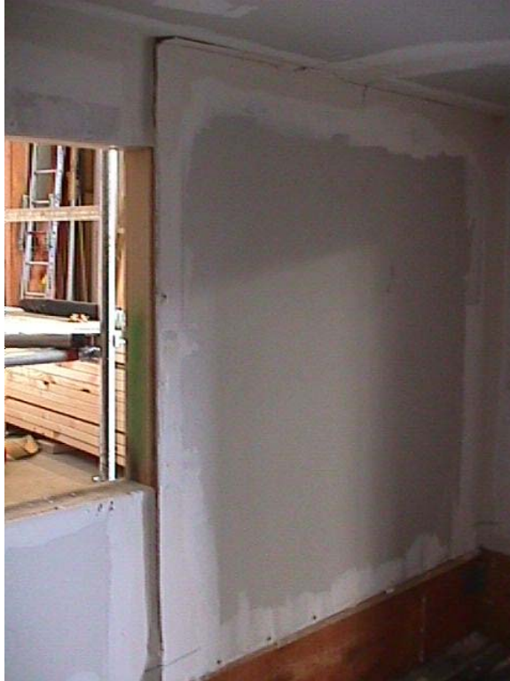
Figure 39. Room R2 – movement at wall long side doorway opening near test completion
