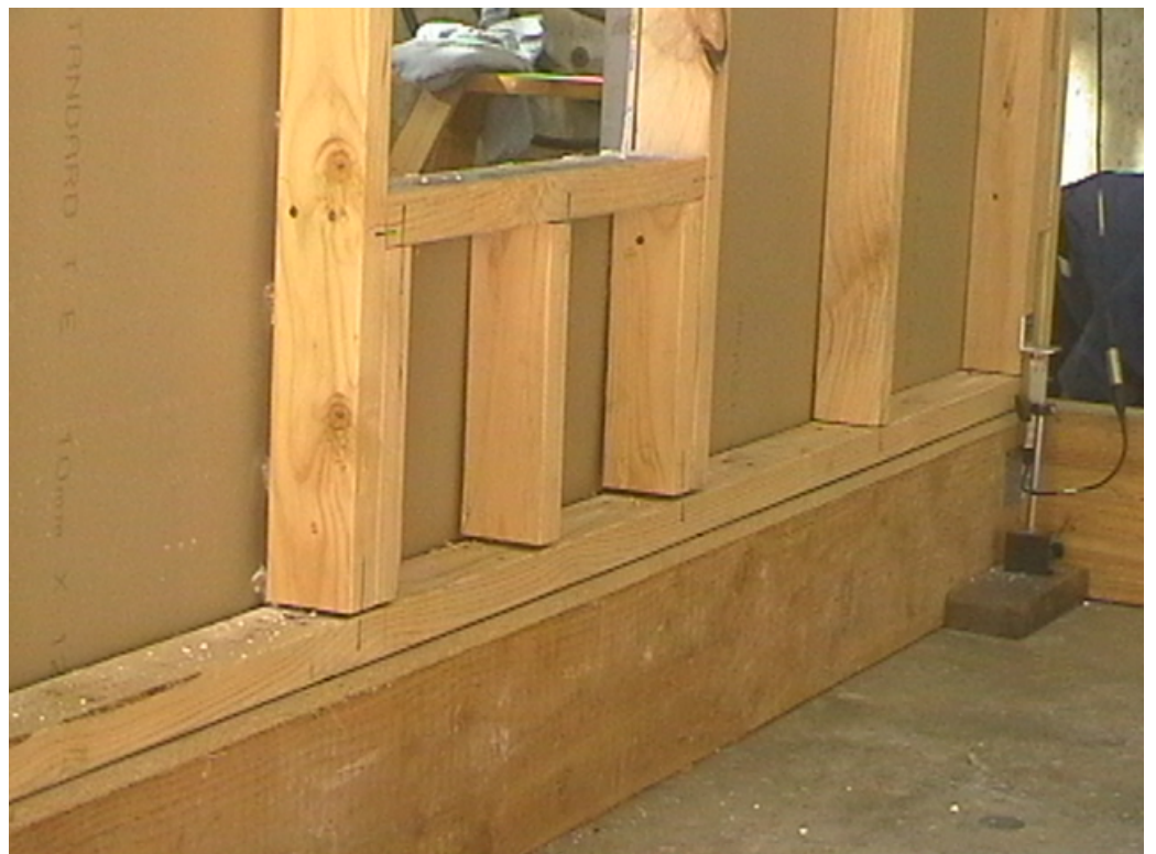
Figure 40. Room R2 – stud uplift on long side walls
