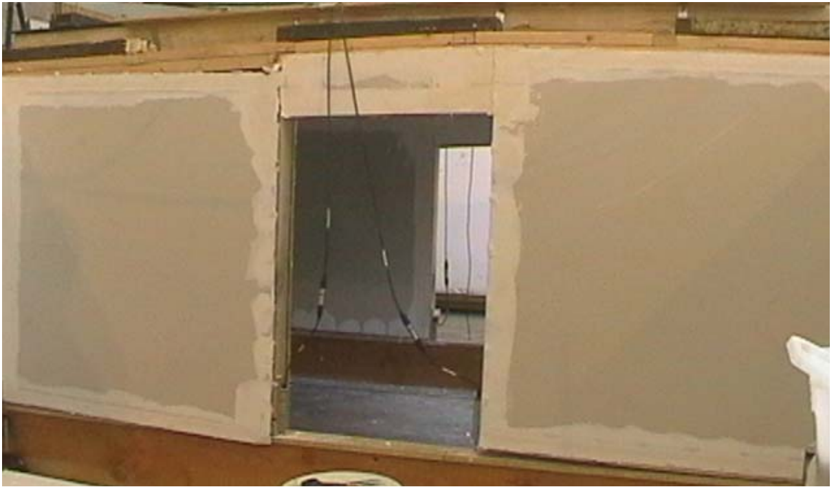
Figure 41. Room R5 – photograph of vertical movement at wall long side doorway openings
