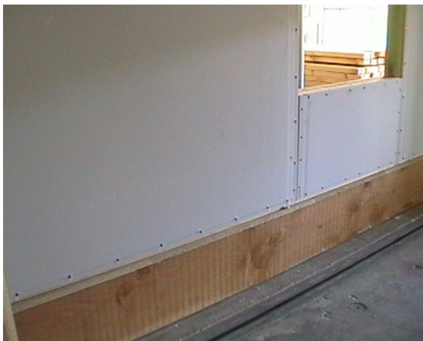
Figure 38. Room R1 – photograph of damage to the interior plasterboard screw fixings at 7 mm wall deflection on the room long sides at the window openings
