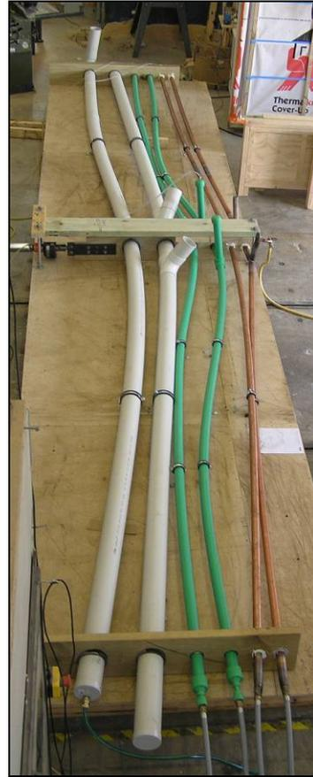
**Figure 19. Significant deformation at  $\pm 270$  mm in plan view.**
