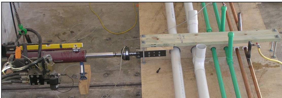
**Figure 9.  $\pm 300$  mm stroke and 10 tonnes actuator used in the test.**
