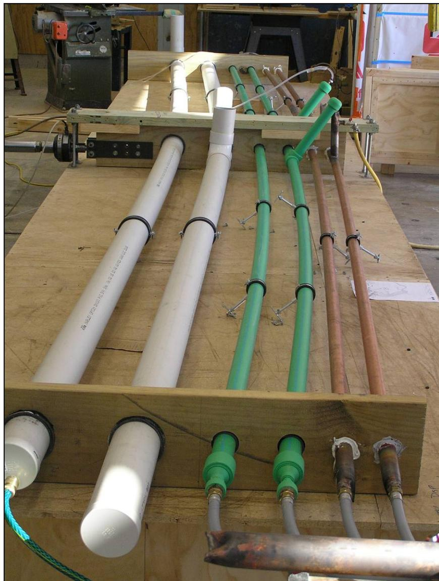
**Figure 12.  $\pm 150$  mm displacement without pipe clamps.**
