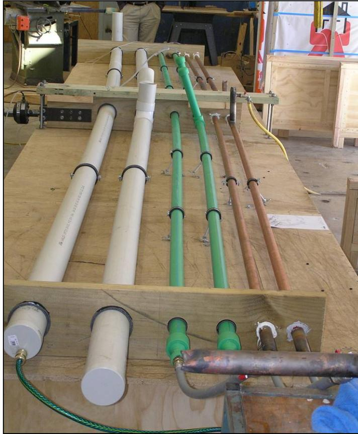
**Figure 10. Start of test at  $\pm 20$  mm displacement.**
