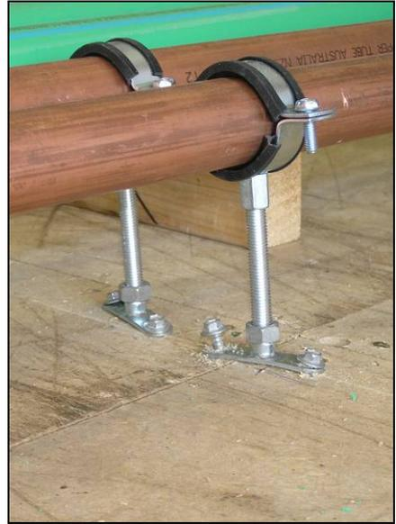
**Figure 15. Onset of the pipe clamp loosening.**
