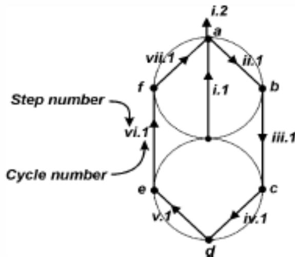
Figure 3. Horizontal plane displacement orbit for performing drift-controlled bi-directional loading tests.
