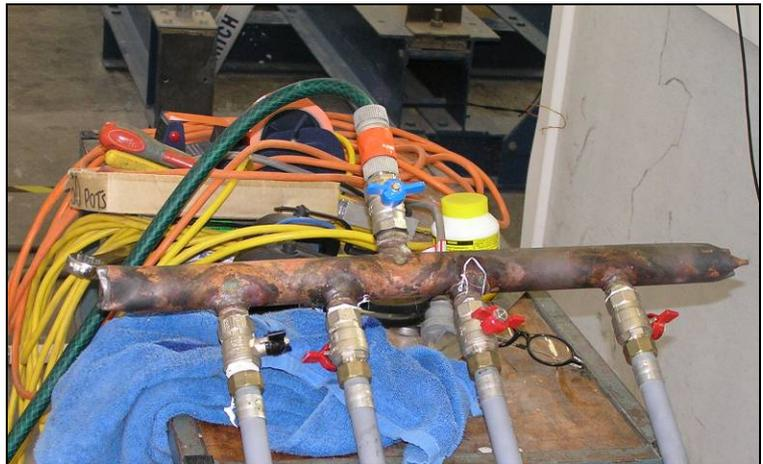
**Figure 5. Valves controlling main pressure.**
