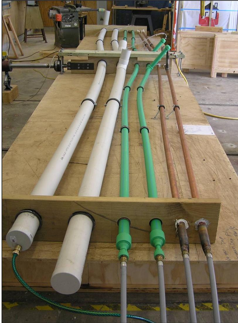
**Figure 16. Bending of pipes and the pipe clamps at  $\pm 150$  mm.**
