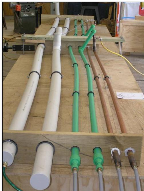
**Figure 14. Ultimate limit state inter-storey deflection of  $\pm 85$  mm with introduced pipe clamps.**
