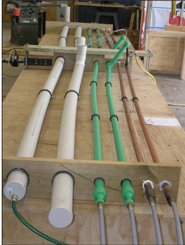
**Figure 13. Test set-up with pipe clamps.**
