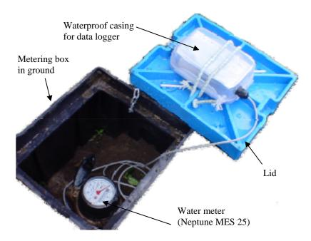
Before entering the house, the logging equipment was installed in the metering box (see Figure 16) and the logger started to capture the flow data. After the audit was complete, the logger was removed to download the signature trace data and replaced with an empty logger, which would collect data for the next month.
