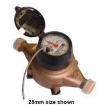
The MESM series nutating disc positive displacement flowmeters are fitted with a non-resetable mechanical totaliser sealed counter c/w a reed switch contact closure output. The pulse output delivers a high rate of pulses per volume making these meters ideal for precision data logging and batching applications. The volt free contact allows use in remote areas where no power source is available.
