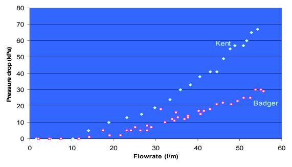
Figure 3: Pressure loss curves of water meters
