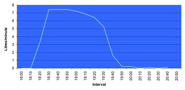
Figure 8: Flow profile of toilet flush
