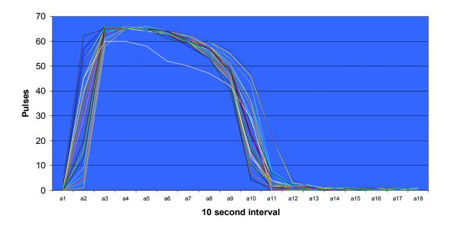
Figure 9: Multiple toilet flushes superimposed
