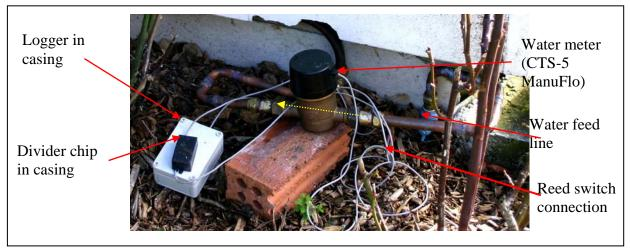
Figure 6: Monitoring arrangement of equipment
