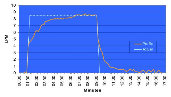
Figure 14: Gravity fed shower (header tank)
