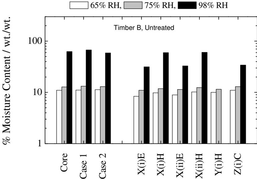
Figure 40. Comparison of oven-dry and meter moisture content methodologies at 65%, 75% and 98% relative humidity for Timber B (untreated), 'Position 5'.
