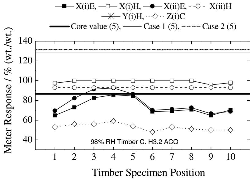
Figure 31. Distribution of moisture content across the length of Timber C (H3.2 ACQ) at 98% relative humidity – presented as a function of analysis methodology.
