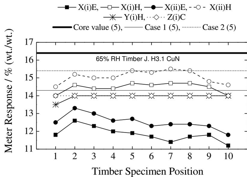
Figure 18. Distribution of moisture content across the length of Timber J (H3.1 LOSP CuN) at 65% relative humidity – presented as a function of analysis methodology.
