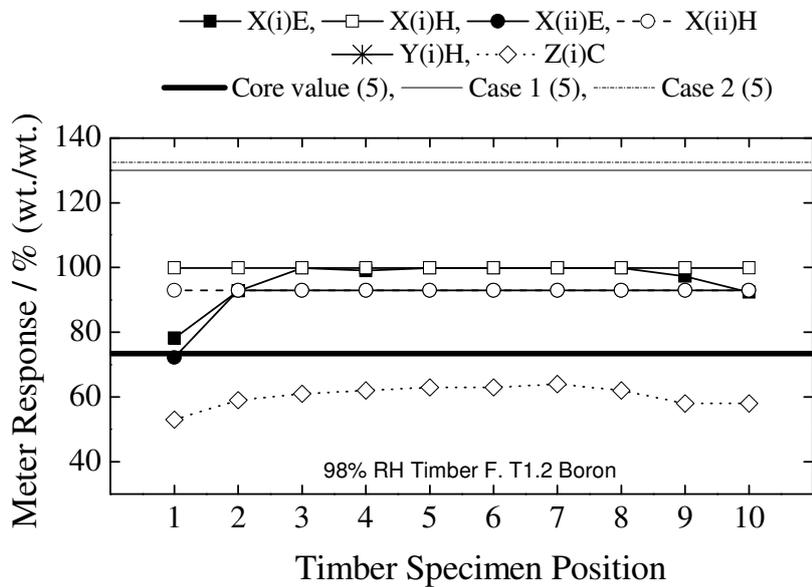
Figure 34. Distribution of moisture content across the length of Timber F (T1.2 boron) at 98% relative humidity – presented as a function of analysis methodology.
