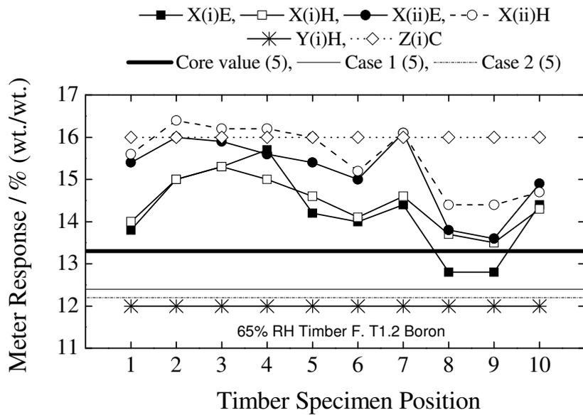
Figure 14. Distribution of moisture content across the length of Timber F (T1.2 boron) at 65% relative humidity – presented as a function of analysis methodology.
