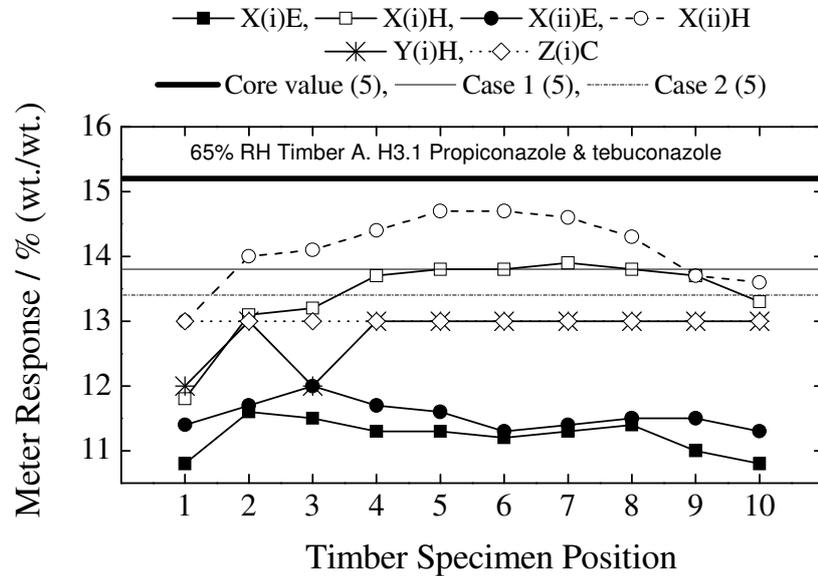
Figure 9. Distribution of moisture content across the length of Timber A (H3.1 propiconazole and tebuconazole) at 65% relative humidity – presented as a function of analysis methodology.
