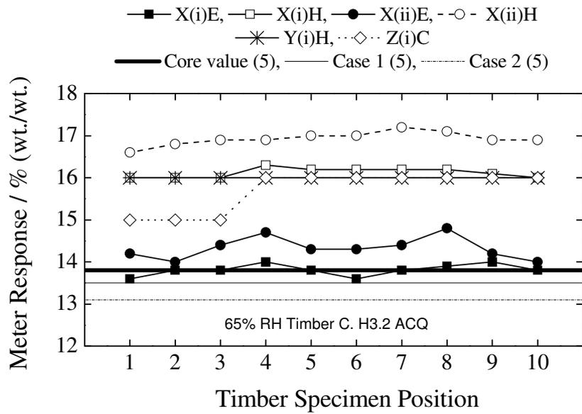
Figure 11. Distribution of moisture content across the length of Timber C (H3.2 ACQ) at 65% relative humidity – presented as a function of analysis methodology.
