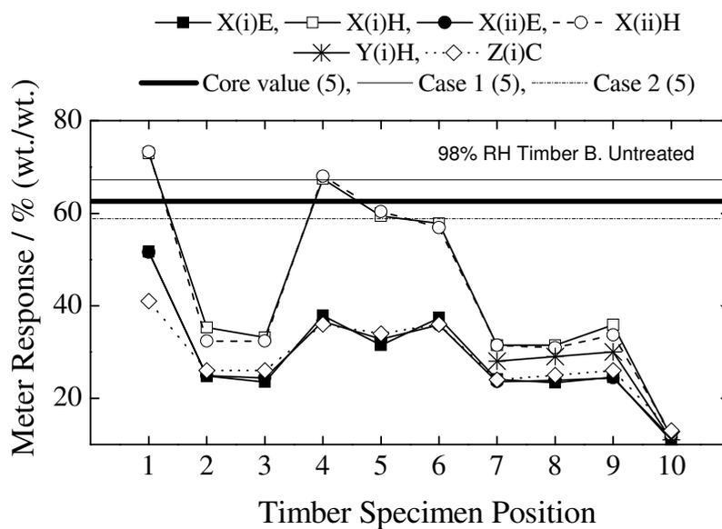
Figure 30. Distribution of moisture content across the length of Timber B (untreated) at 98% relative humidity – presented as a function of analysis methodology.
