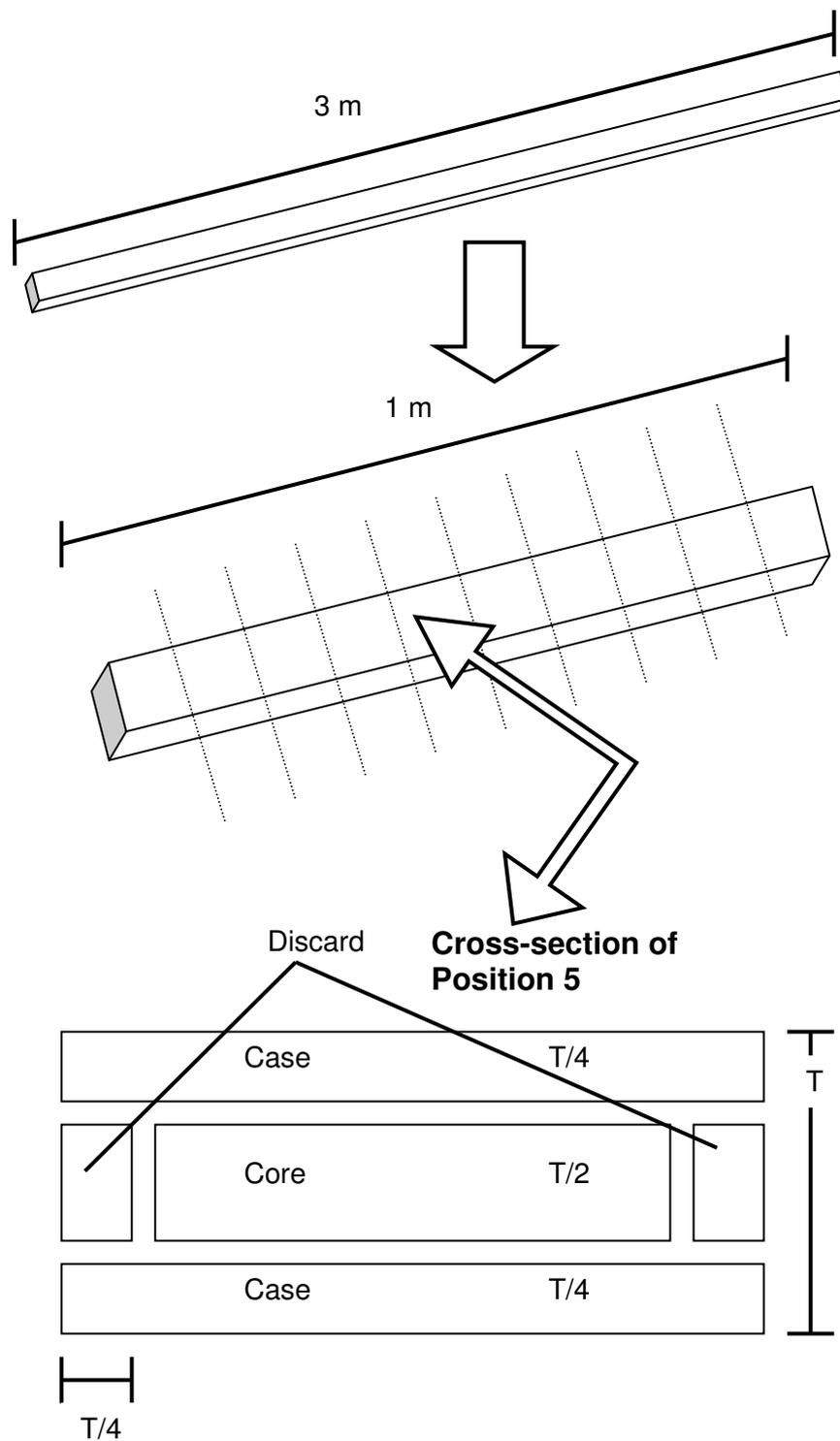
Figure 2. Cutting and sequencing of the timber specimens according to Cutting Pattern (a) as described in AS/NZS 1080.1 (Standard 1997). T = 45 mm (drawing not to scale).
