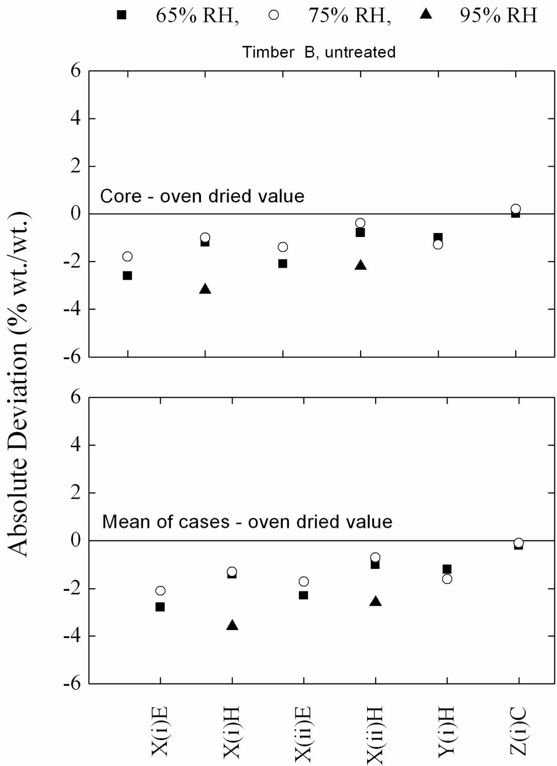
**Figure 7. Timber B (untreated). Values of absolute deviation of each moisture meter reading at Position 5 (uncorrected) from values measured using the AS/NZS 1080.1 oven-dried method (core and mean of cases).**
