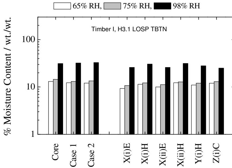
Figure 47. Comparison of oven-dry and meter moisture content methodologies at 65%, 75% and 98% relative humidity for Timber I (H3.1 LO SP TBTN), 'Position 5'.
