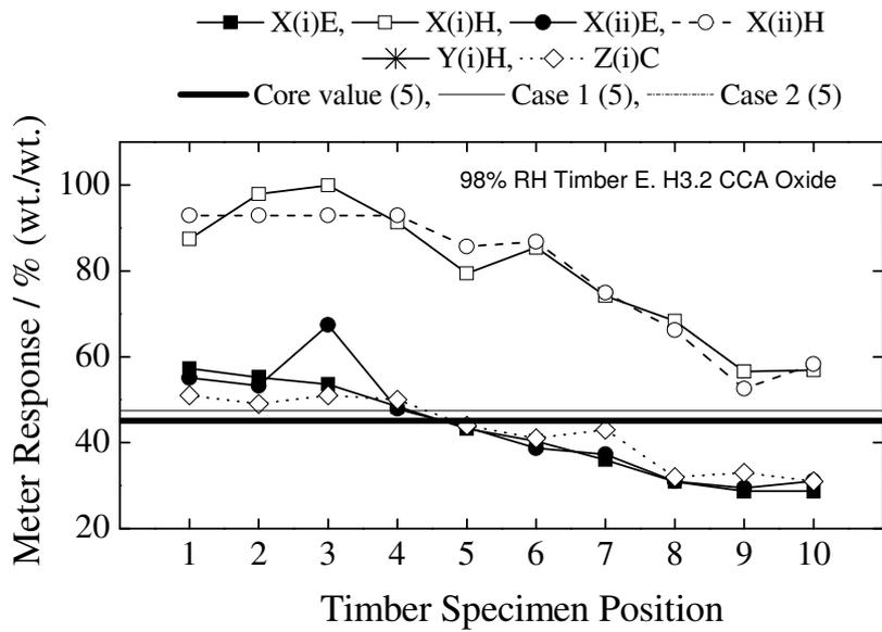
Figure 33. Distribution of moisture content across the length of Timber E (H3.2 CCA) at 98% relative humidity – presented as a function of analysis methodology.
