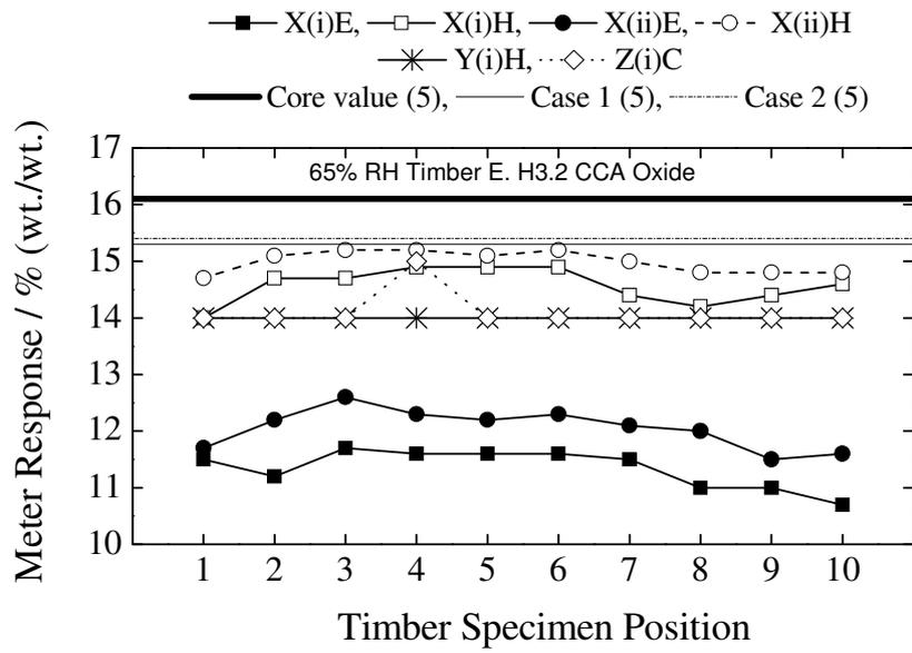
Figure 13. Distribution of moisture content across the length of Timber E (H3.2 CCA) at 65% relative humidity – presented as a function of analysis methodology.
