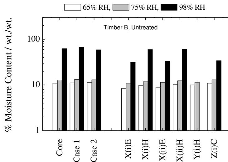
**Figure 5. Comparison of oven-dry and meter moisture content methodologies at 65%, 75% and 98% relative humidity for Timber B (untreated), 'Position 5'.**
