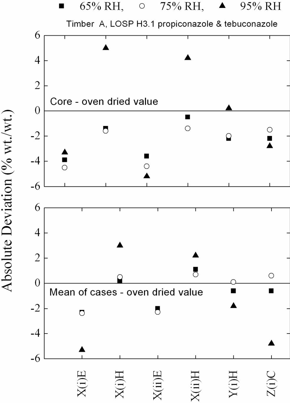
Figure 49. Timber Sample A (LOSP H3.1 propiconazole and tebuconazole). Values of absolute deviation of each moisture meter reading at Position 5 (uncorrected) from values measured using the AS/NZS 1080.1 oven-dried method (core and mean of cases).
