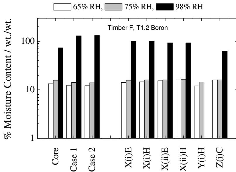
Figure 44. Comparison of oven-dry and meter moisture content methodologies at 65%, 75% and 98% relative humidity for Timber F (T1.2 boron), 'Position 5'.
