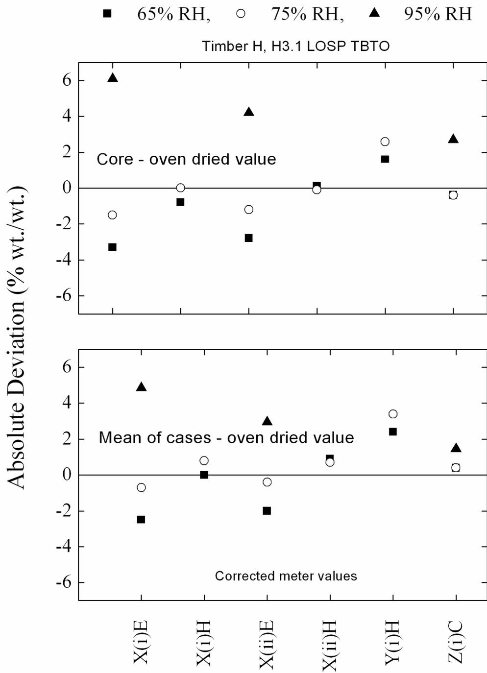
**Figure 66. Corrected (see Table 9 for guide only) absolute values of meter deviation for Timber Sample H (H3.1 LOSP TBTO). Values of absolute deviation of each moisture meter reading at Position 5 (corrected) from values measured using the AS/NZS 1080.1 oven-dried method (core and mean of cases).**
