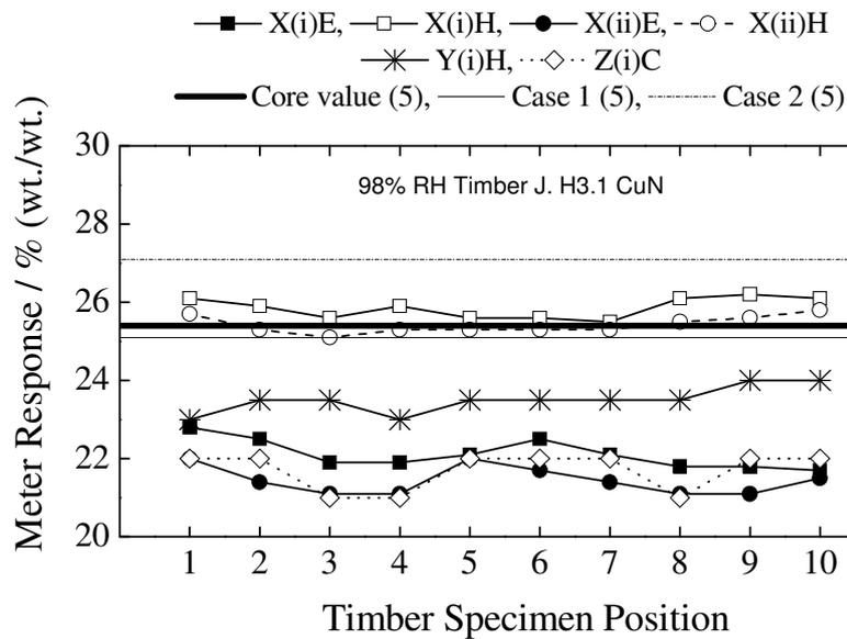
Figure 38. Distribution of moisture content across the length of Timber J (H3.1 LOSP CuN) at 98% relative humidity – presented as a function of analysis methodology.
