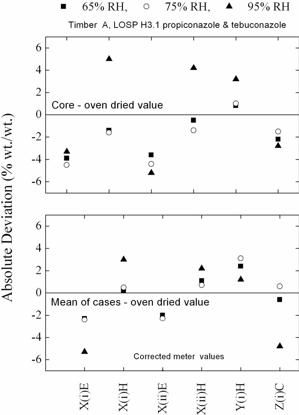
**Figure 59. Corrected (see Table 9 for guide only) absolute values of meter deviation for Timber Sample A (LOSP H3.1 propiconazole and tebuconazole). Values of absolute deviation of each moisture meter reading at Position 5 (corrected) from values measured using the AS/NZS 1080.1 oven-dried method (core and mean of cases).**
