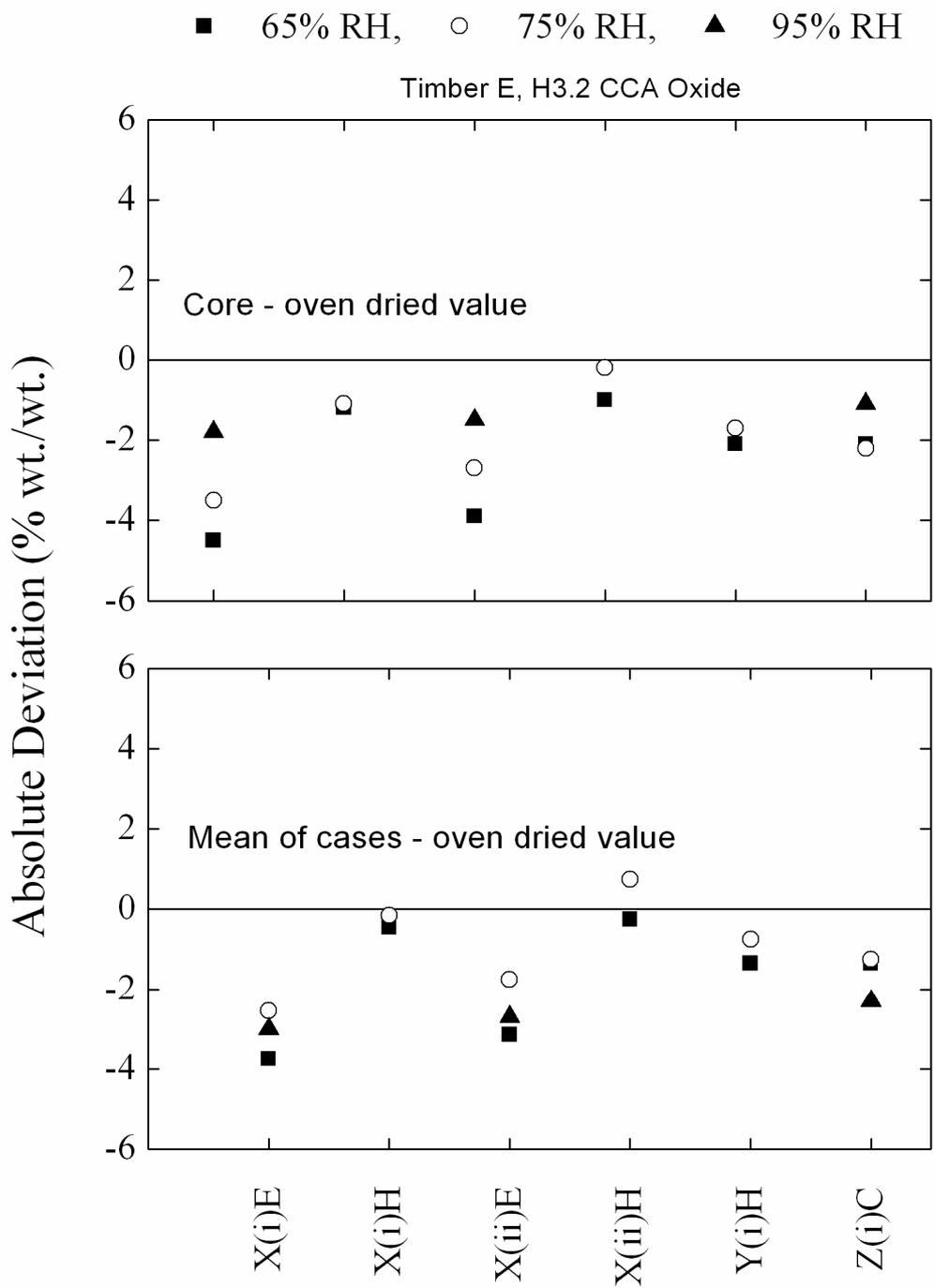
**Figure 53. Timber Sample E (H3.2 CCA oxide). Values of absolute deviation of each moisture meter reading at Position 5 (uncorrected) from values measured using the AS/NZS 1080.1 oven-dried method (core and mean of cases).**
