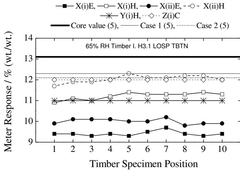
Figure 17. Distribution of moisture content across the length of Timber I (H3.1 LOSP TBTN) at 65% relative humidity – presented as a function of analysis methodology.
