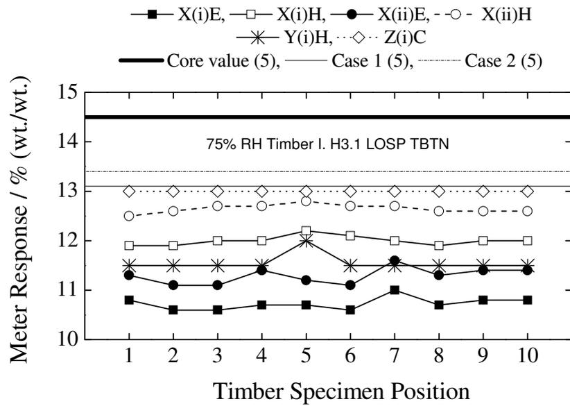
Figure 27. Distribution of moisture content across the length of Timber I (H3.1 LOSP TBTN) at 75% relative humidity – presented as a function of analysis methodology.
