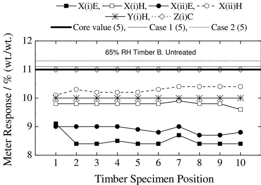
Figure 3. Distribution of moisture content across the length of Timber B (untreated) at 65% relative humidity – presented as a function of analysis methodology.
