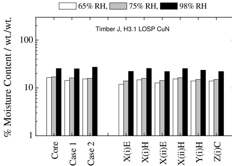
Figure 48. Comparison of oven-dry and meter moisture content methodologies at 65%, 75% and 98% relative humidity for Timber J (H3.1 LO SP CuN), 'Position 5'.
