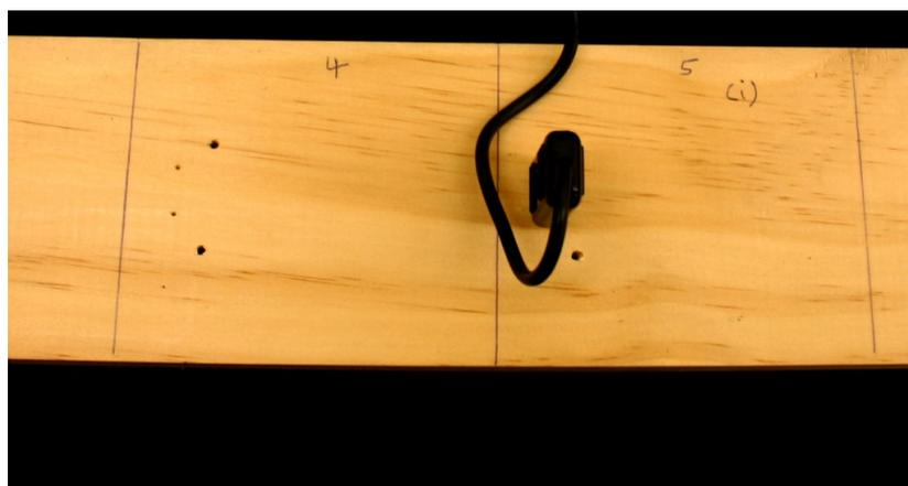
**Figure 1. Test Positions 4 and 5 as shown for the untreated timber specimen (the hand-held probe is shown which relates to meter conditions X(i)E and X(ii)E). Note that to this point, as shown, only meter conditions X(i)E and X(i)H have been used in this sample – the difference in electrode tip separation and electrode width can be clearly seen via the holes left within the timber.**
