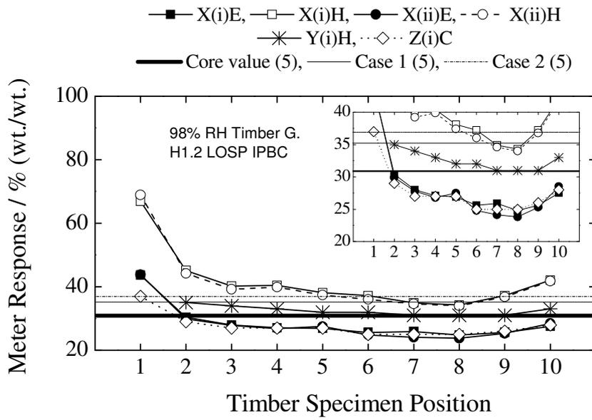
Figure 35. Distribution of moisture content across the length of Timber G (H1.2 LOSP IPBC) at 98% relative humidity – presented as a function of analysis methodology.
