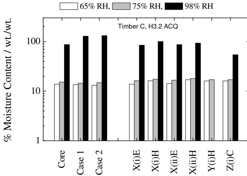
Figure 41. Comparison of oven-dry and meter moisture content methodologies at 65%, 75% and 98% relative humidity for Timber C (H3.2 ACQ), 'Position 5'.
