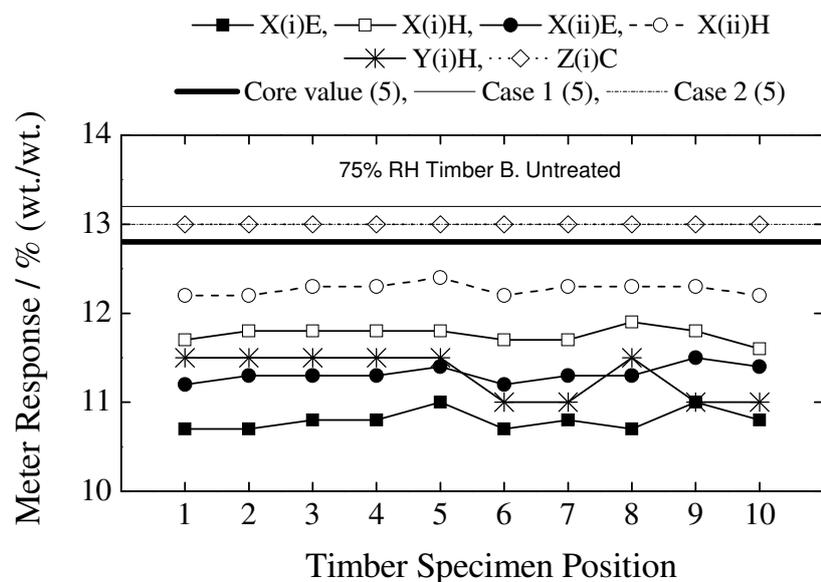
Figure 20. Distribution of moisture content across the length of Timber B (untreated) at 75% relative humidity – presented as a function of analysis methodology.
