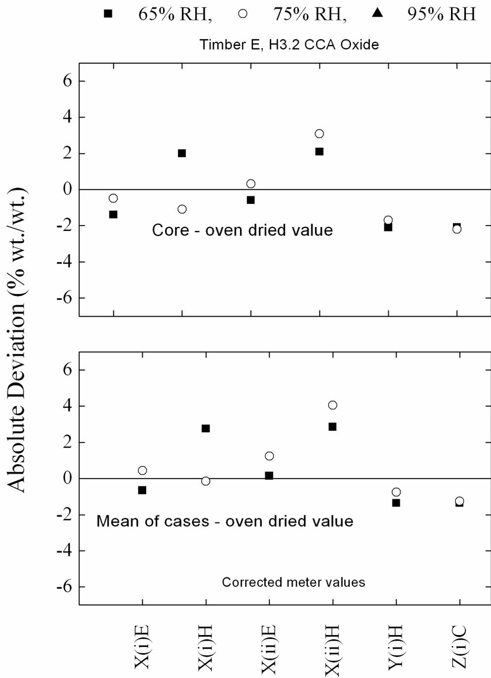
**Figure 63. Corrected (see Table 9 for guide only) absolute values of meter deviation for Timber Sample E (H3.2 CCA oxide). Values of absolute deviation of each moisture meter reading at Position 5 (corrected) from values measured using the AS/NZS 1080.1 oven-dried method (core and mean of cases).**
