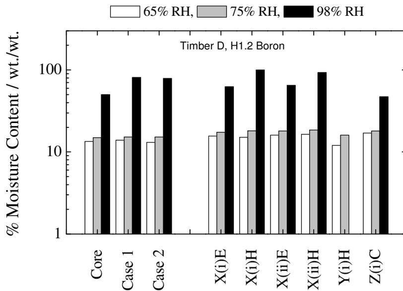
Figure 42. Comparison of oven-dry and meter moisture content methodologies at 65%, 75% and 98% relative humidity for Timber D (H1.2 boron), 'Position 5'.
