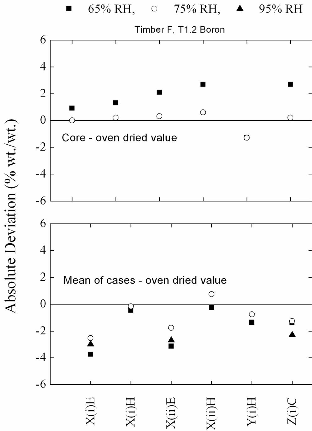
**Figure 54. Timber Sample F (T1.2 boron). Values of absolute deviation of each moisture meter reading at Position 5 (uncorrected) from values measured using the AS/NZS 1080.1 oven-dried method (core and mean of cases).**
