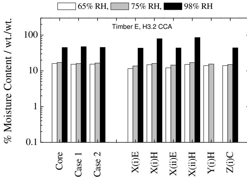
Figure 43. Comparison of oven-dry and meter moisture content methodologies at 65%, 75% and 98% relative humidity for Timber E (H3.2 CCA), 'Position 5'.
