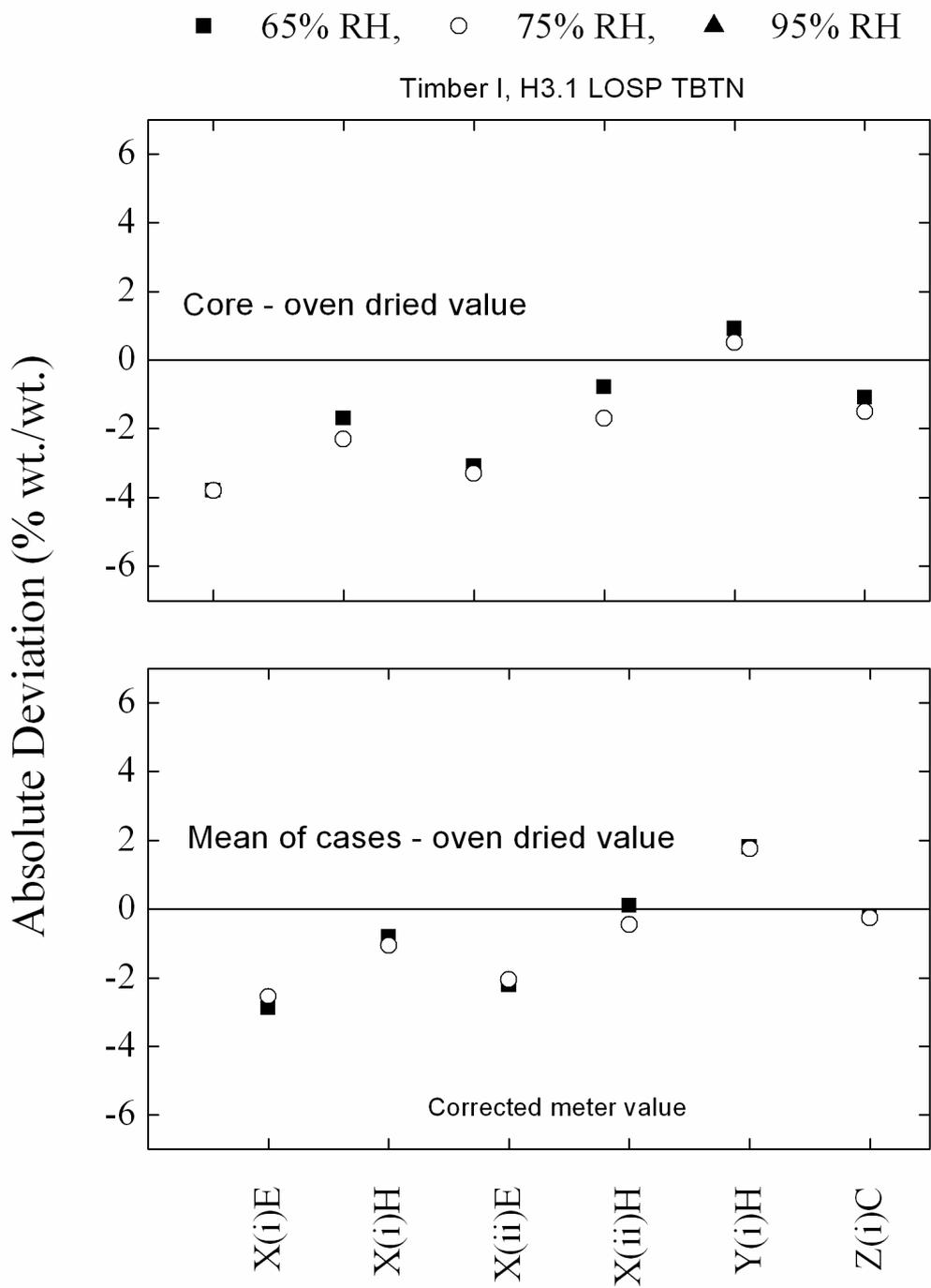
**Figure 67. Corrected (see Table 9 for guide only) absolute values of meter deviation for Timber Sample I (H3.1 LO SP TBTN). Values of absolute deviation of each moisture meter reading at Position 5 (corrected) from values measured using the AS/NZS 1080.1 oven-dried method (core and mean of cases).**
