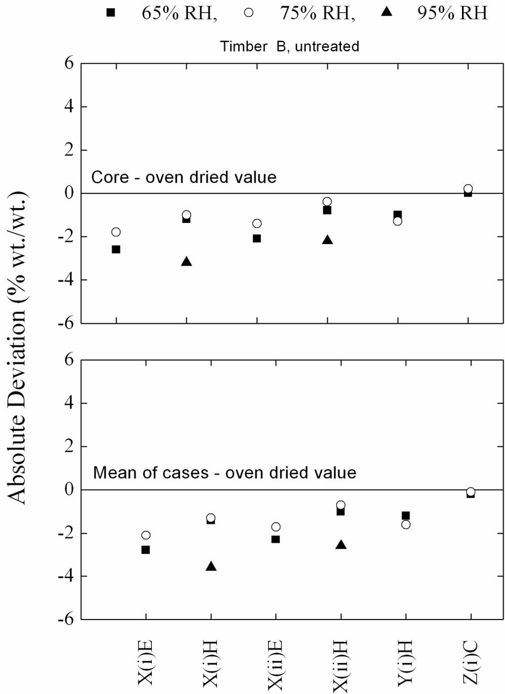
**Figure 50. Timber Sample B (untreated). Values of absolute deviation of each moisture meter reading at Position 5 (uncorrected) from values measured using the AS/NZS 1080.1 oven-dried method (core and mean of cases).**
