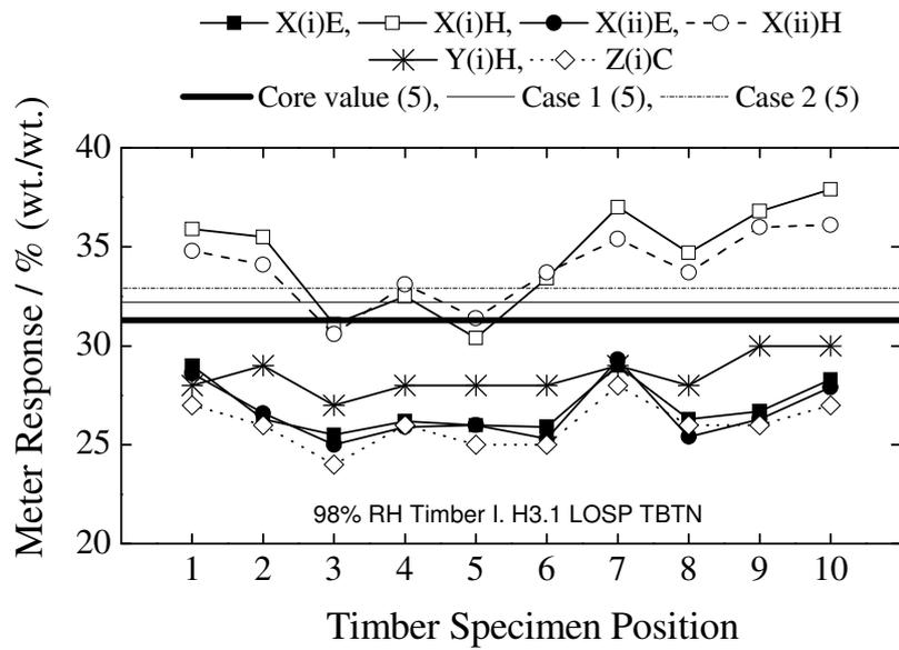
Figure 37. Distribution of moisture content across the length of Timber I (H3.1 LOSP TBTN) at 98% relative humidity – presented as a function of analysis methodology.
