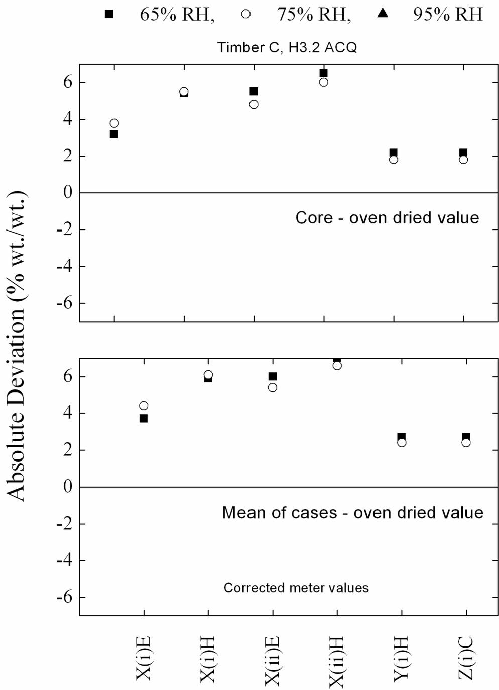
**Figure 61. Corrected (see Table 9 for guide only) absolute values of meter deviation for Timber Sample C (H3.2 ACQ). Values of absolute deviation of each moisture meter reading at Position 5 (corrected) from values measured using the AS/NZS 1080.1 oven-dried method (core and mean of cases).**
