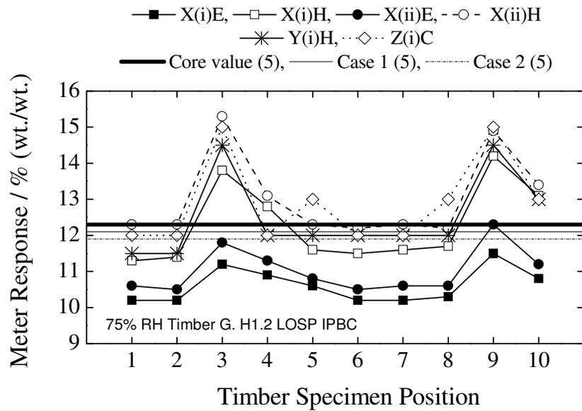
Figure 25. Distribution of moisture content across the length of Timber G (H1.2 LOSP IPBC) at 75% relative humidity – presented as a function of analysis methodology.
