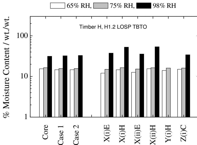
Figure 46. Comparison of oven-dry and meter moisture content methodologies at 65%, 75% and 98% relative humidity for Timber H (H1.2 LOSP TBTO), 'Position 5'.
