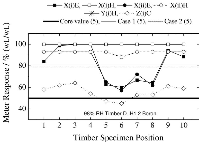
Figure 32. Distribution of moisture content across the length of Timber D (H1.2 boron) at 98% relative humidity – presented as a function of analysis methodology.
