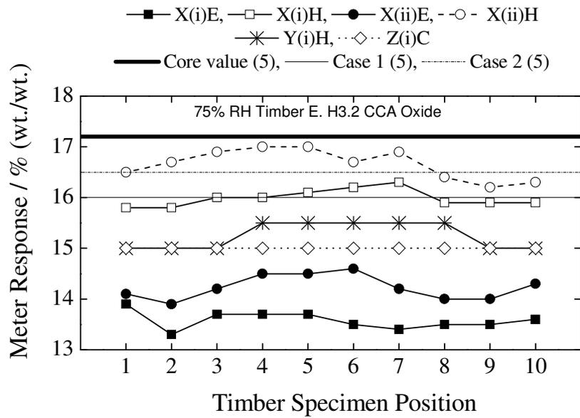
Figure 23. Distribution of moisture content across the length of Timber E (H3.2 CCA) at 75% relative humidity – presented as a function of analysis methodology.
