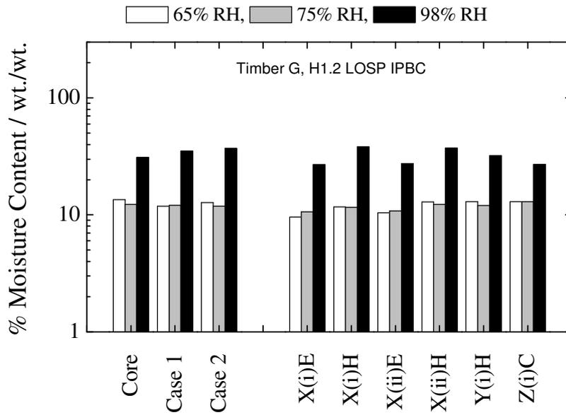
Figure 45. Comparison of oven-dry and meter moisture content methodologies at 65%, 75% and 98% relative humidity for Timber G (T1.2 LOSP IPBC), 'Position 5'.
