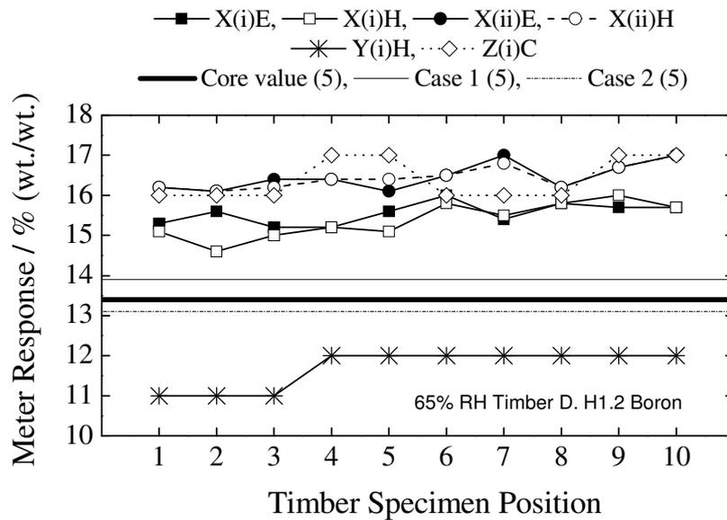
Figure 12. Distribution of moisture content across the length of Timber D (H1.2 boron) at 65% relative humidity – presented as a function of analysis methodology.
