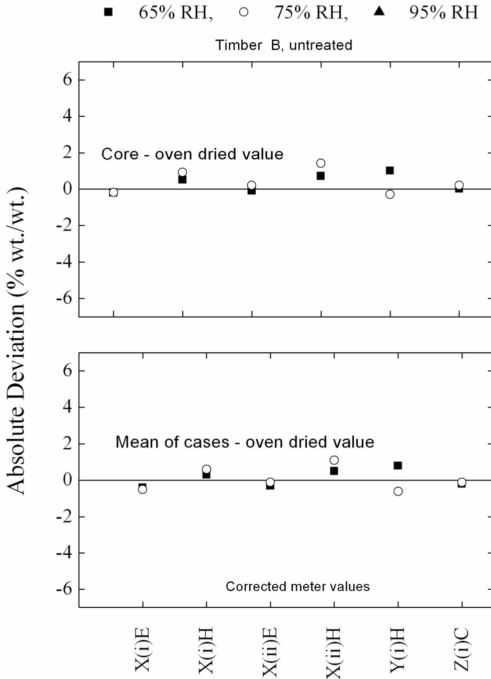
**Figure 8. Corrected (see Table 9 for guide only) absolute values of meter deviation for Timber Sample B (untreated). Values of absolute deviation of each moisture meter reading at Position 5 (corrected) from values measured using the AS/NZS 1080.1 oven-dried method (core and mean of cases).**
