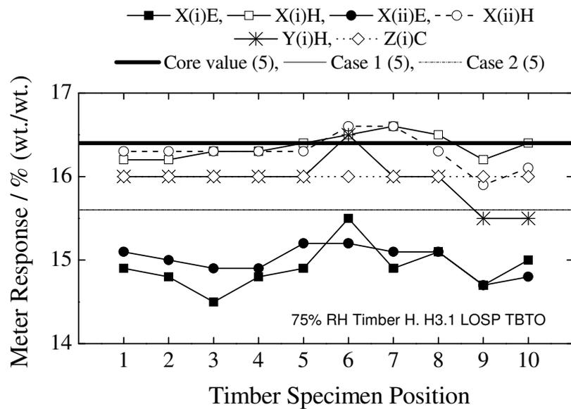
Figure 26. Distribution of moisture content across the length of Timber H (H3.1 LOSP TBTO) at 75% relative humidity – presented as a function of analysis methodology.
