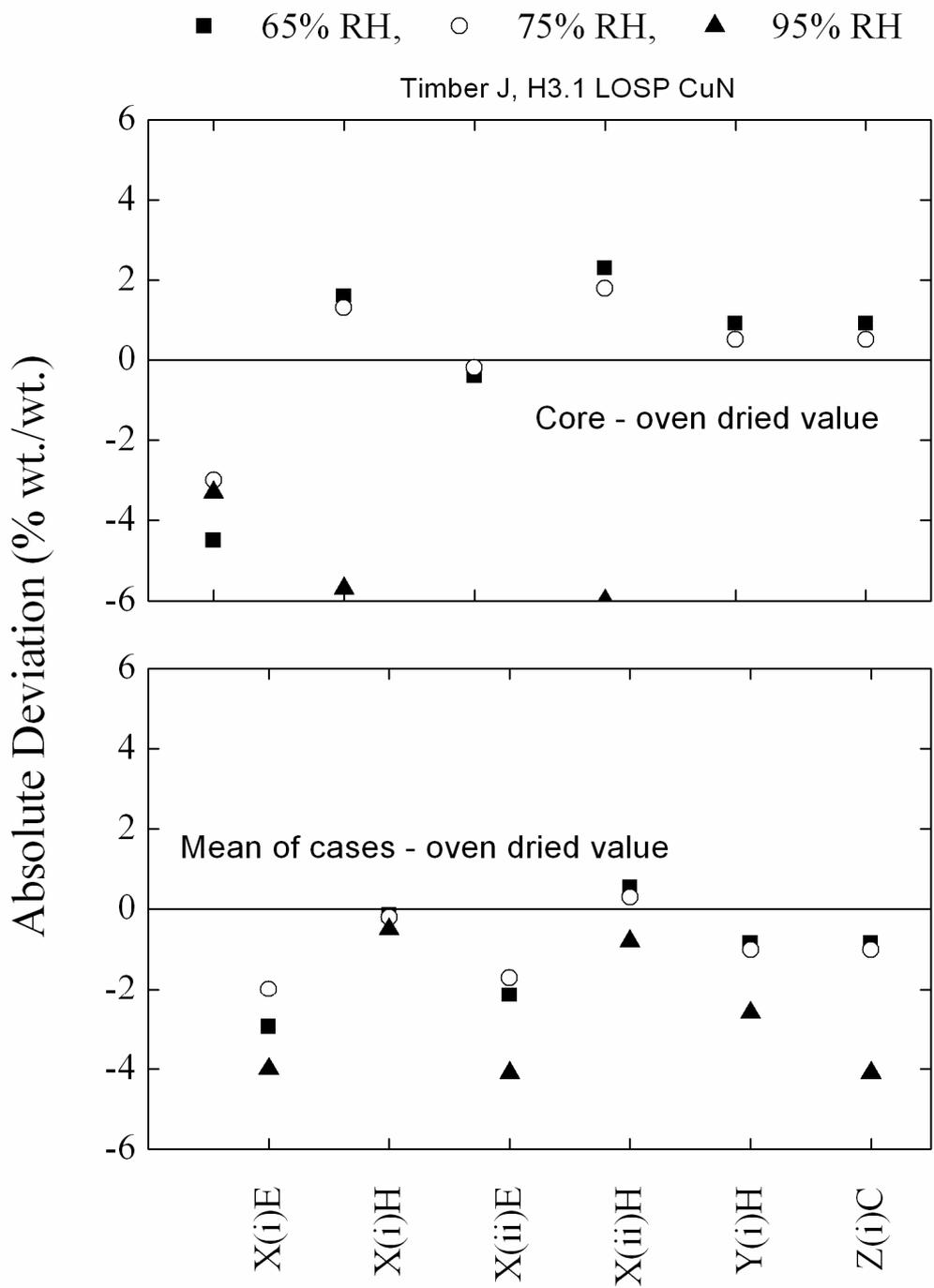
**Figure 58. Timber Sample J (H3.1 LOSP CuN). Values of absolute deviation of each moisture meter reading at Position 5 (uncorrected) from values measured using the AS/NZS 1080.1 oven-dried method (core and mean of cases).**
