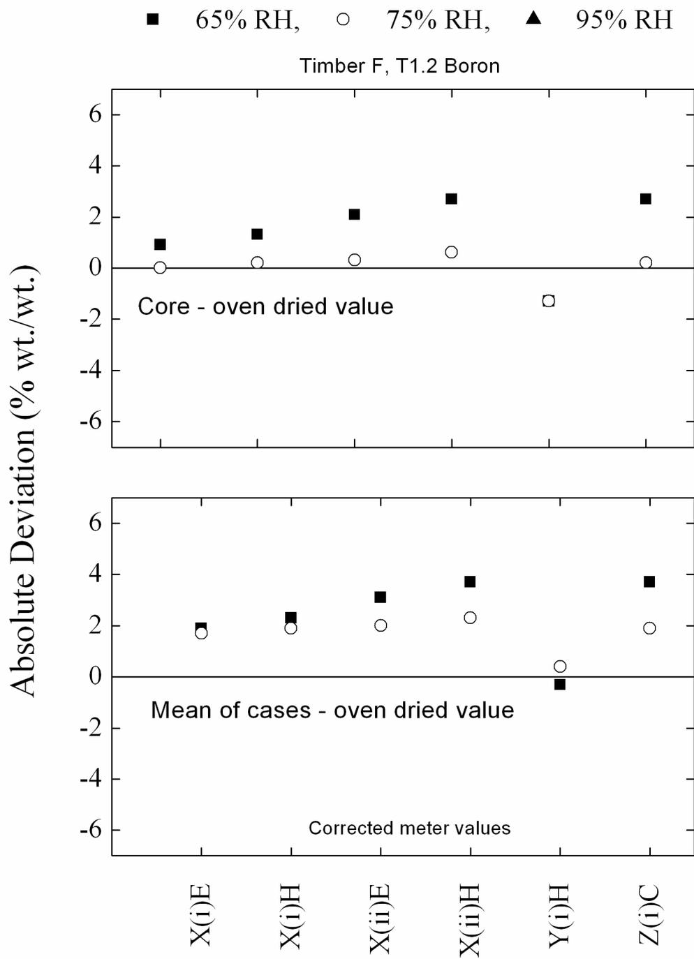
**Figure 64. Corrected (see Table 9 for guide only) absolute values of meter deviation for Timber Sample F (T1.2 boron). Values of absolute deviation of each moisture meter reading at Position 5 (corrected) from values measured using the AS/NZS 1080.1 oven-dried method (core and mean of cases).**
