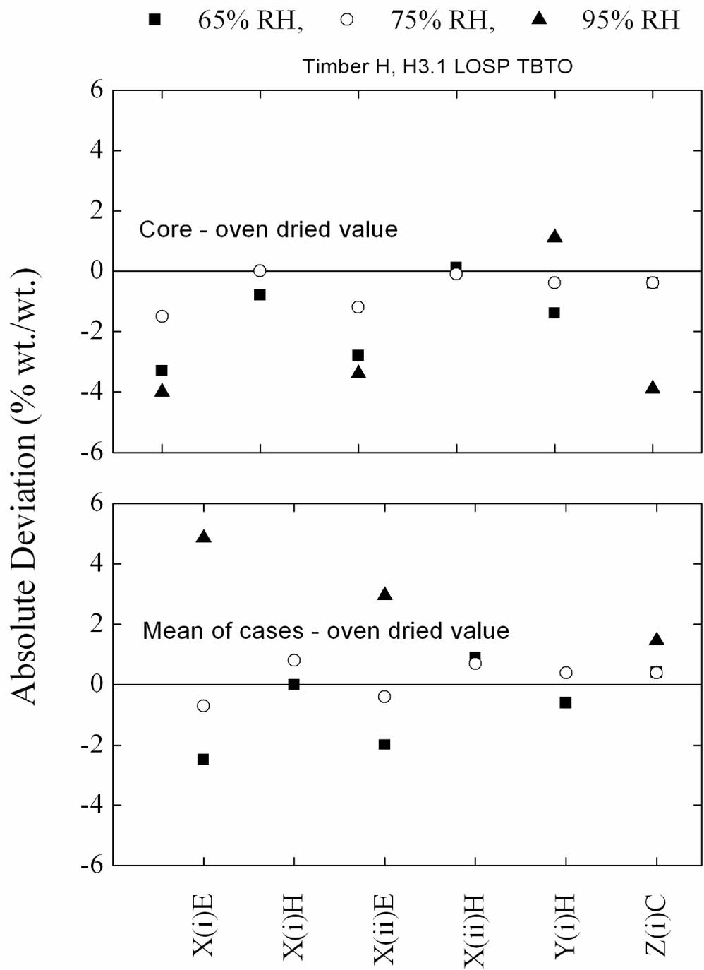
**Figure 56. Timber Sample H (H3.1 LOSP TBTO). Values of absolute deviation of each moisture meter reading at Position 5 (uncorrected) from values measured using the AS/NZS 1080.1 oven-dried method (core and mean of cases).**
