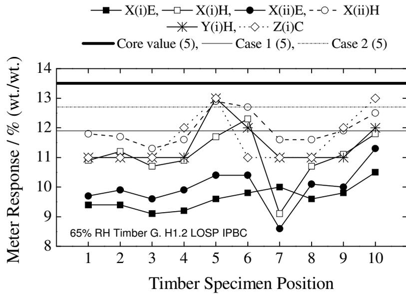
Figure 15. Distribution of moisture content across the length of Timber G (H1.2 LOSP IPBC) at 65% relative humidity – presented as a function of analysis methodology.
