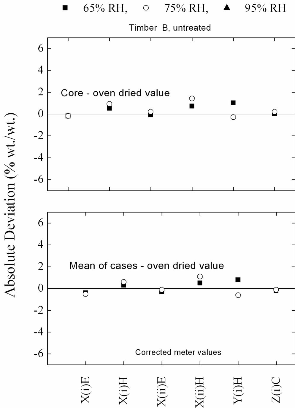
**Figure 60. Corrected (see Table 9 for guide only) absolute values of meter deviation for Timber Sample B (untreated). Values of absolute deviation of each moisture meter reading at Position 5 (corrected) from values measured using the AS/NZS 1080.1 oven-dried method (core and mean of cases).**
