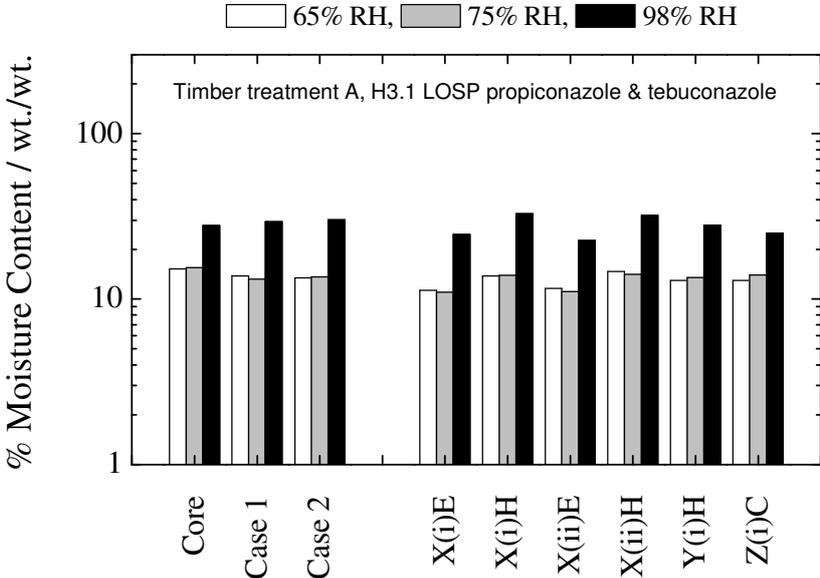
Figure 39. Comparison of oven-dry and meter moisture content methodologies at 65%, 75% and 98% relative humidity for Timber A (H3.1 LOSP propiconazole and tebuconazole), 'Position 5'.
