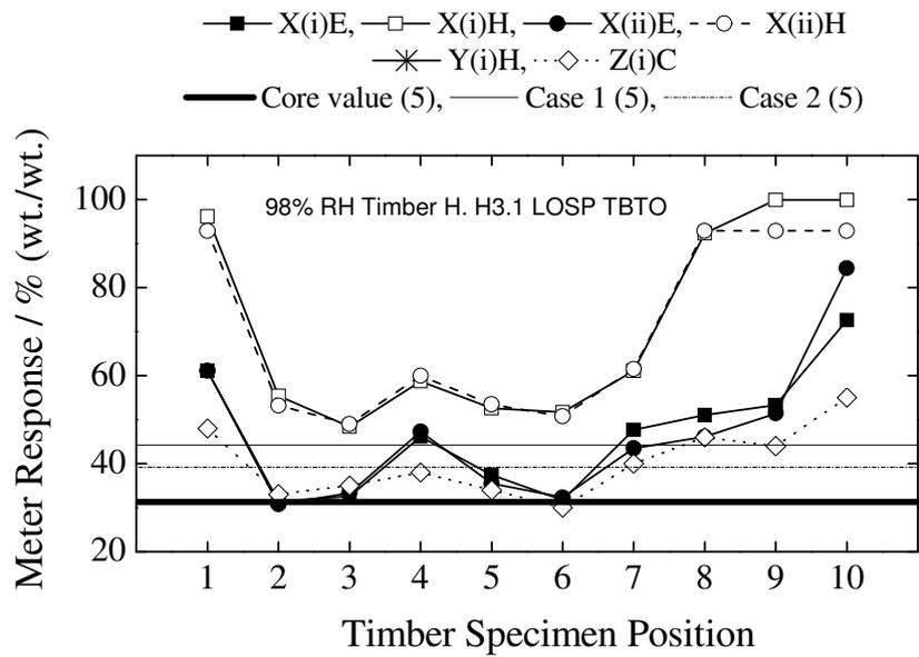
Figure 36. Distribution of moisture content across the length of Timber H (H3.1 LOSP TBTO) at 98% relative humidity – presented as a function of analysis methodology.
