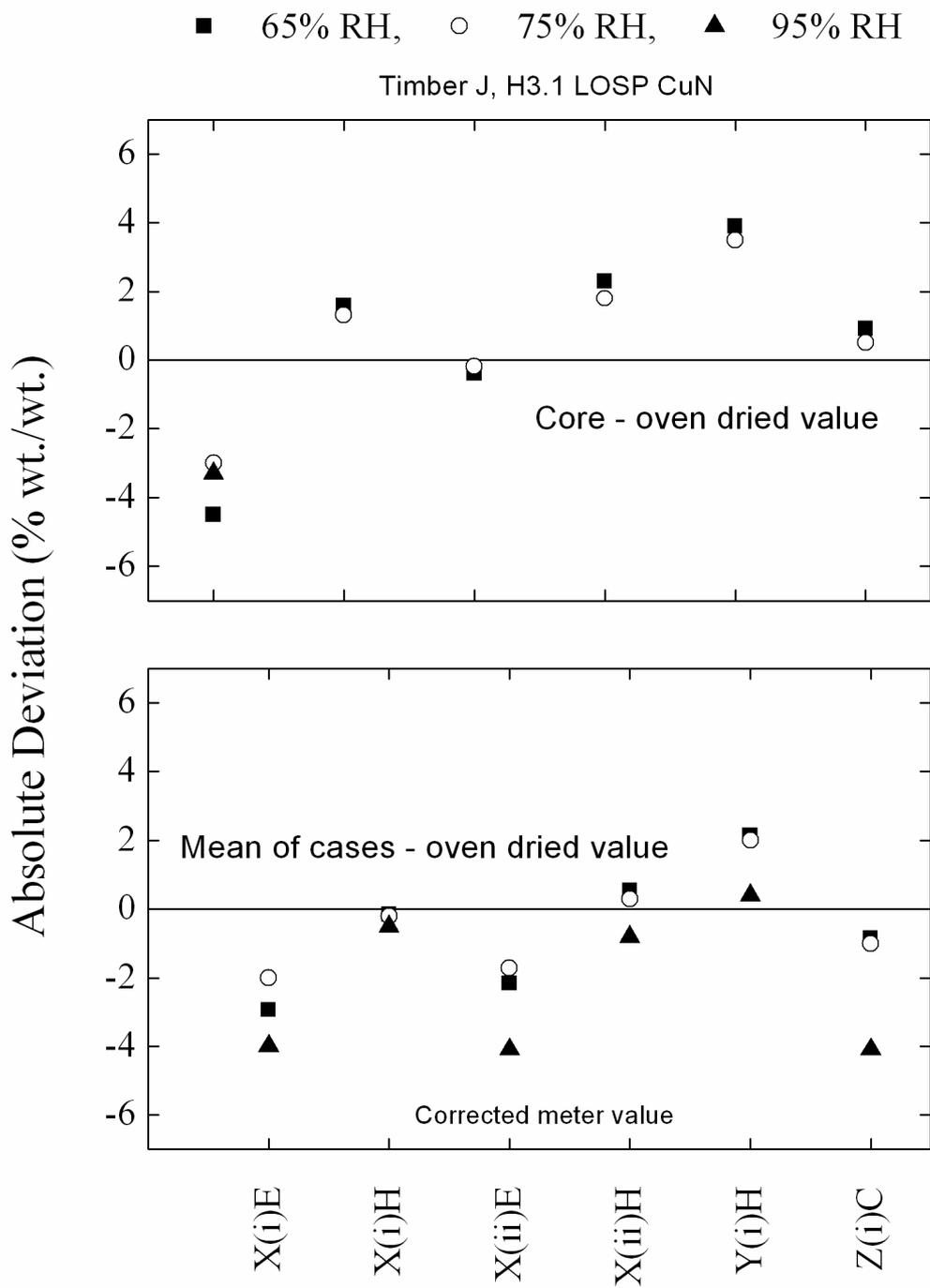
**Figure 68. Corrected (see Table 9 for guide only) absolute values of meter deviation for Timber Sample J (H3.1 LOSP CuN). Values of absolute deviation of each moisture meter reading at Position 5 (corrected) from values measured using the AS/NZS 1080.1 oven-dried method (core and mean of cases).**
