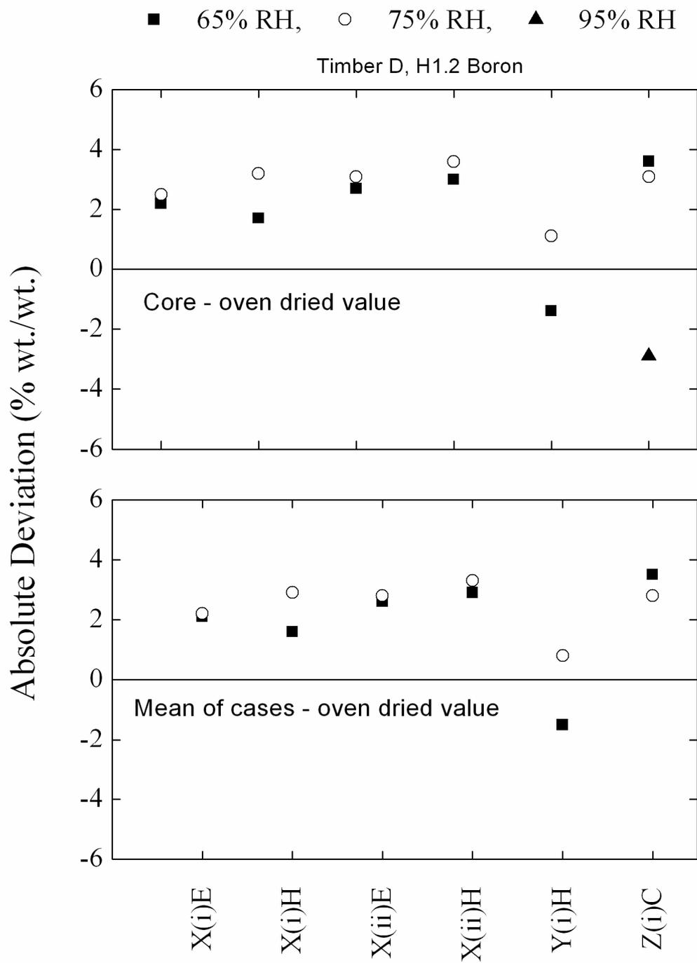
**Figure 52. Timber Sample D (H1.2 boron). Values of absolute deviation of each moisture meter reading at Position 5 (uncorrected) from values measured using the AS/NZS 1080.1 oven-dried method (core and mean of cases).**
