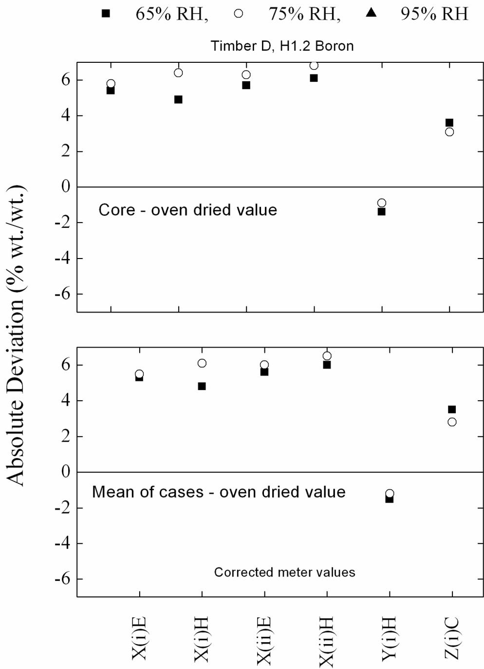
**Figure 62. Corrected (see Table 9 for guide only) absolute values of meter deviation for Timber Sample D (H1.2 boron). Values of absolute deviation of each moisture meter reading at Position 5 (corrected) from values measured using the AS/NZS 1080.1 oven-dried method (core and mean of cases).**
