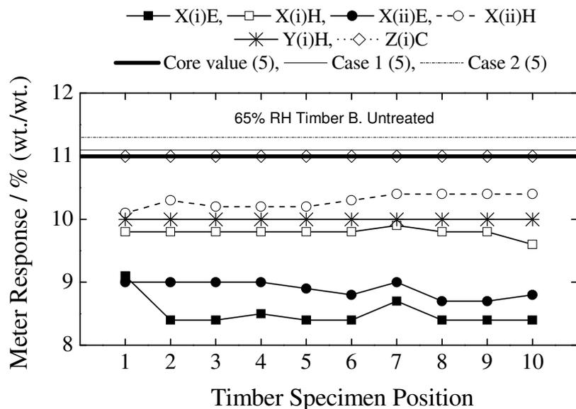
Figure 10. Distribution of moisture content across the length of Timber B (untreated) at 65% relative humidity – presented as a function of analysis methodology.
