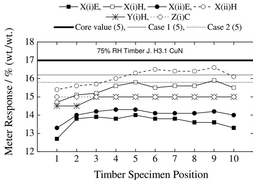
Figure 28. Distribution of moisture content across the length of Timber J (H3.1 LOSP CuN) at 75% relative humidity – presented as a function of analysis methodology.
