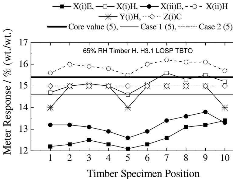
Figure 16. Distribution of moisture content across the length of Timber H (H3.1 LOSP TBTO) at 65% relative humidity – presented as a function of analysis methodology.
