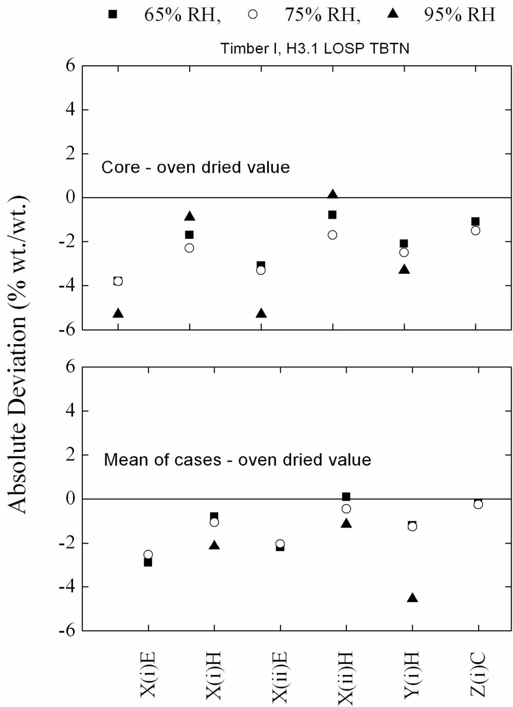
**Figure 57. Timber Sample I (H3.1 LO SP TBTN). Values of absolute deviation of each moisture meter reading at Position 5 (uncorrected) from values measured using the AS/NZS 1080.1 oven-dried method (core and mean of cases).**
