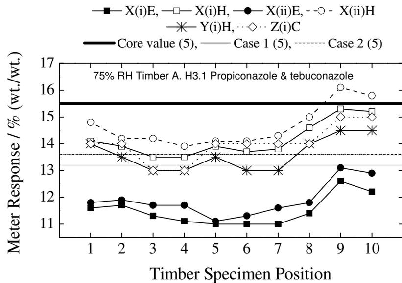
Figure 19. Distribution of moisture content across the length of Timber A (H3.1 propiconazole and tebuconazole) at 75% relative humidity – presented as a function of analysis methodology.
