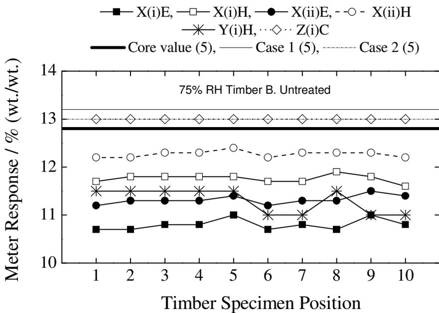
Figure 4. Distribution of moisture content across the length of Timber B (untreated) at 75% relative humidity – presented as a function of analysis methodology.
