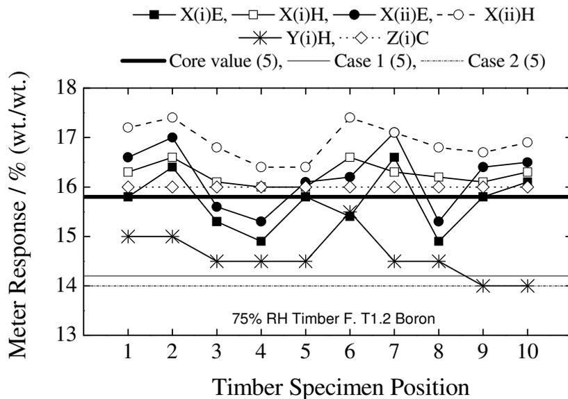
Figure 24. Distribution of moisture content across the length of Timber F (T1.2 boron) at 75% relative humidity – presented as a function of analysis methodology.
