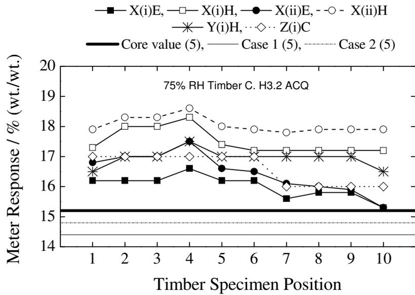
Figure 21. Distribution of moisture content across the length of Timber C (H3.2 ACQ) at 75% relative humidity – presented as a function of analysis methodology.
