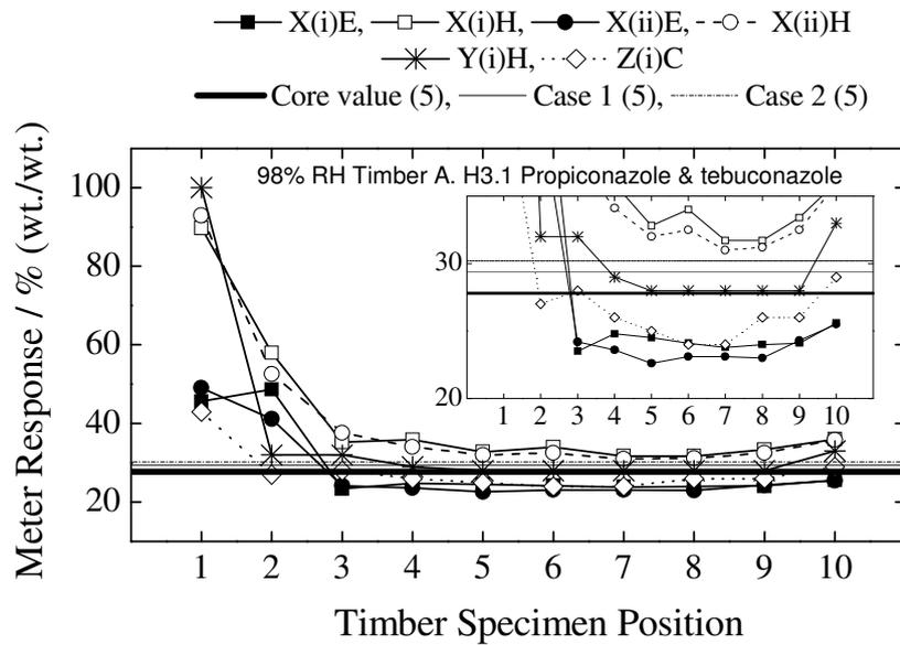
Figure 29. Distribution of moisture content across the length of Timber A (H3.1 propiconazole and tebuconazole) at 98% relative humidity – presented as a function of analysis methodology.
