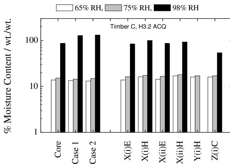
**Figure 6. Comparison of oven-dry and meter moisture content methodologies at 65%, 75% and 98% relative humidity for Timber C (H3.2 ACQ), 'Position 5'.**
