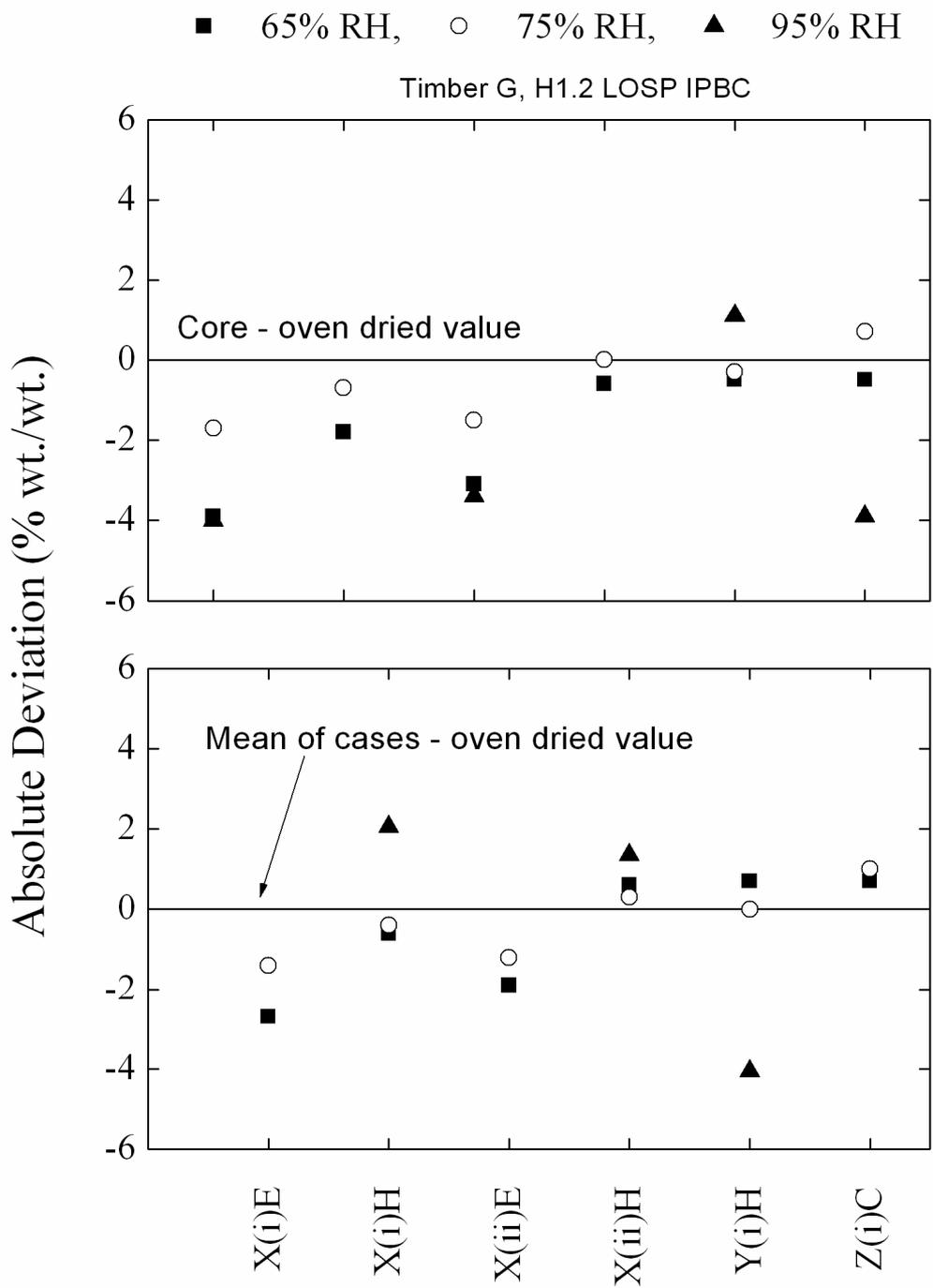
**Figure 55. Timber Sample G (H1.2 LOSP IPBC). Values of absolute deviation of each moisture meter reading at Position 5 (uncorrected) from values measured using the AS/NZS 1080.1 oven-dried method (core and mean of cases).**
