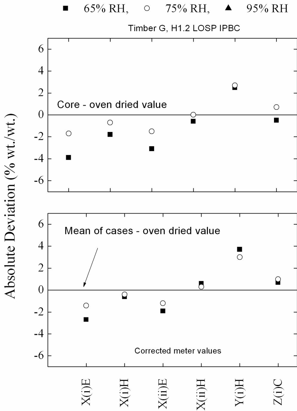
**Figure 65. Corrected (see Table 9 for guide only) absolute values of meter deviation for Timber Sample G (H1.2 LOSP IPBC). Values of absolute deviation of each moisture meter reading at Position 5 (corrected) from values measured using the AS/NZS 1080.1 oven-dried method (core and mean of cases).**
