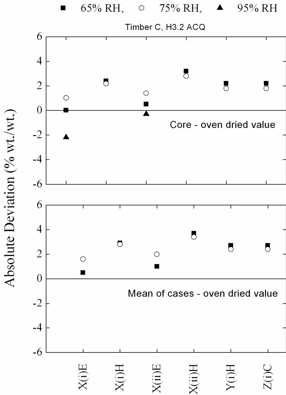
**Figure 51. Timber Sample C (H3.2 ACQ). Values of absolute deviation of each moisture meter reading at Position 5 (uncorrected) from values measured using the AS/NZS 1080.1 oven-dried method (core and mean of cases).**
