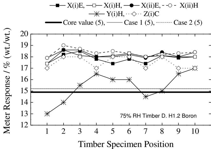
Figure 22. Distribution of moisture content across the length of Timber D (H1.2 boron) at 75% relative humidity – presented as a function of analysis methodology.
