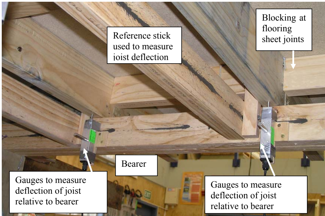
Figure 14. Measurement of vertical deflection of joist relative to bearer during Stage IV.
