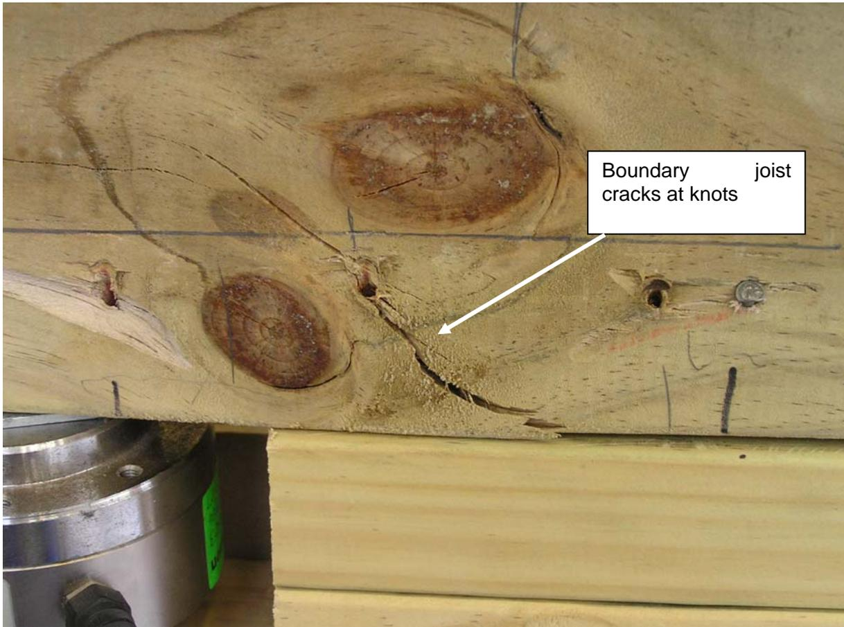
Figure 58. Crack at knots in End 2 boundary joist late in Test 2 of Stage II
