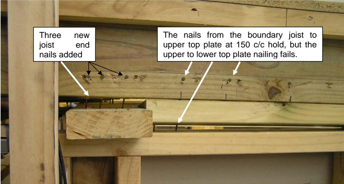
Figure 54. End 2 boundary joist uplift at other end in latter stages of Stage III Test 1
