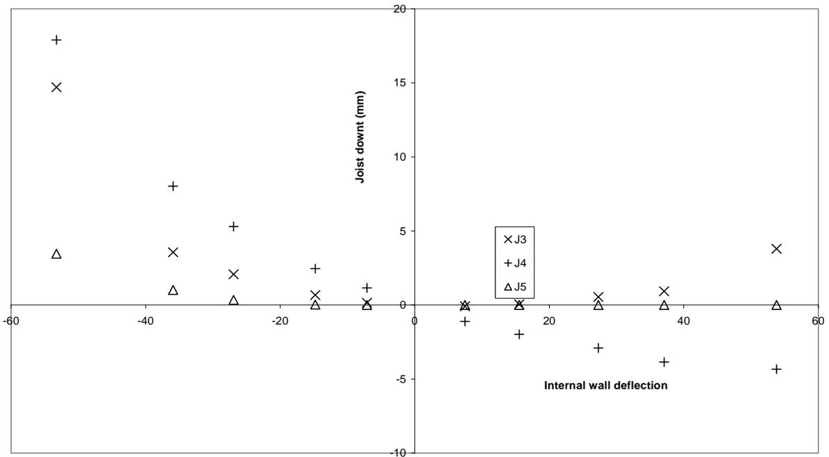
Figure 65. Joist deflection at Z2 at the internal wall for Test 1 of Stage III
