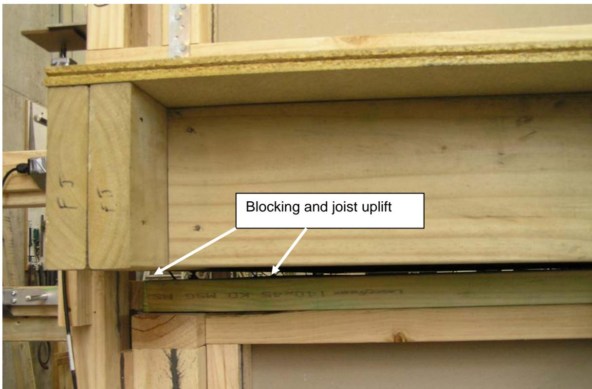
Figure 17. Boundary joist uplift from wall below at Side 1 End 1 due to actuator malfunction prior to Test 2 of Stage I
