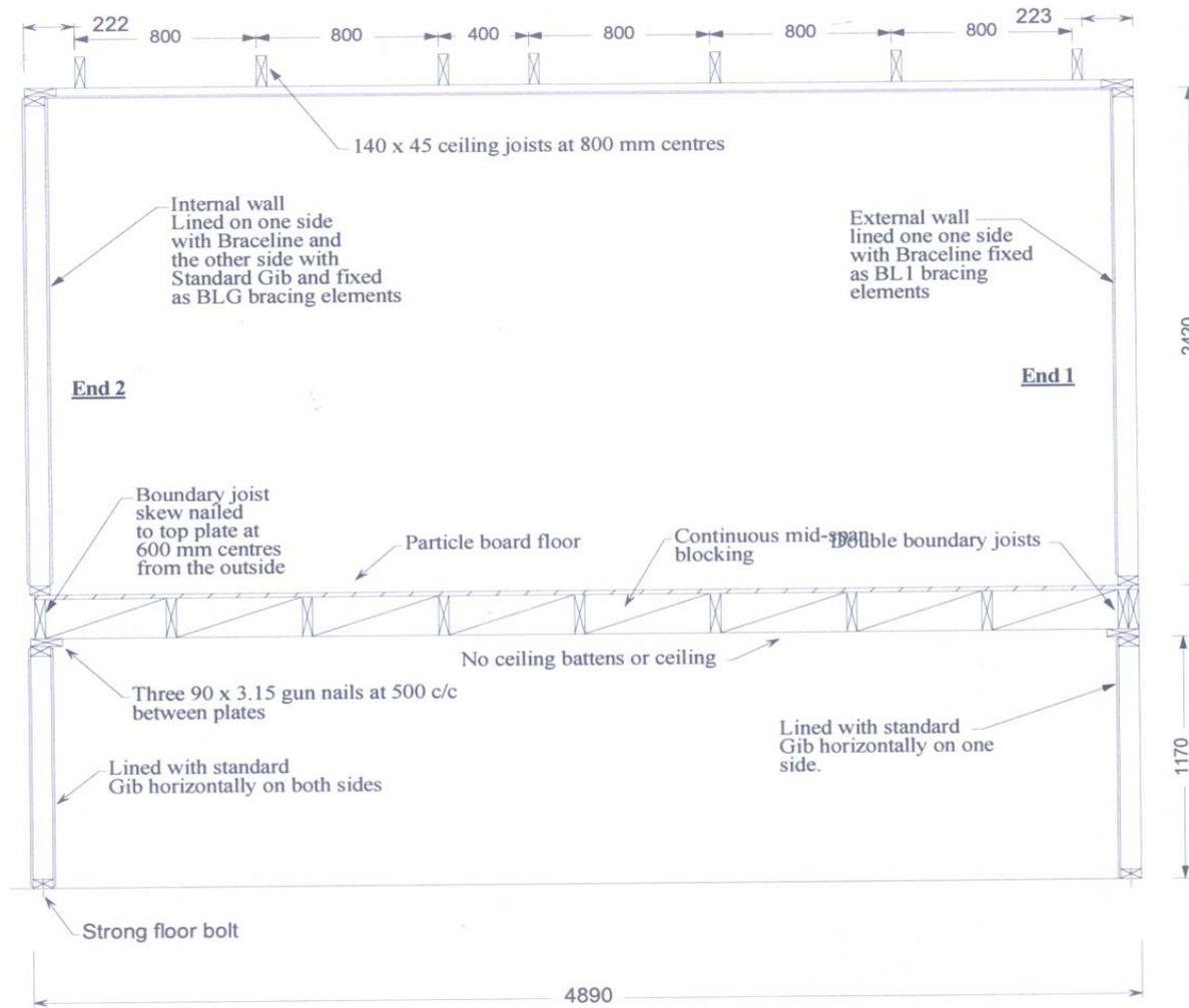
Figure 3. Cross-section of Room 2 looking towards Side 1
