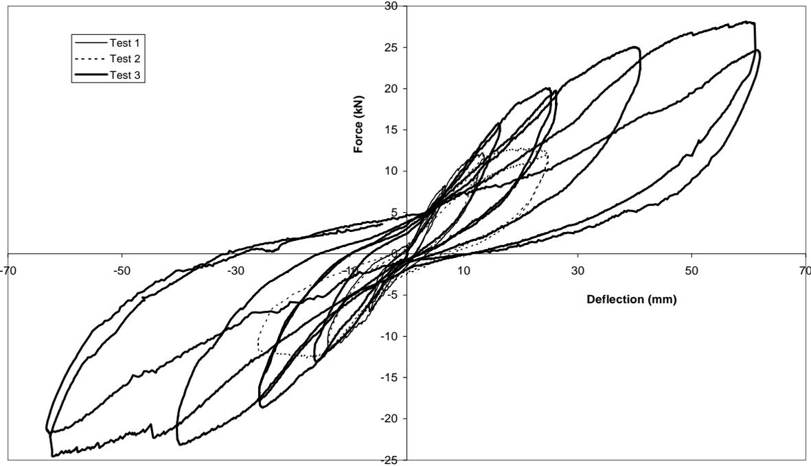
**Figure 41. Total racking force versus average deflection for Stage II**
