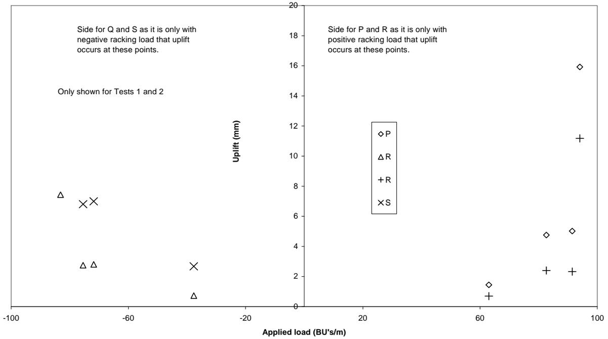
**Figure 44. Uplift of upper storey studs from lower storey studs versus racking load at End 1 for Stage II**
