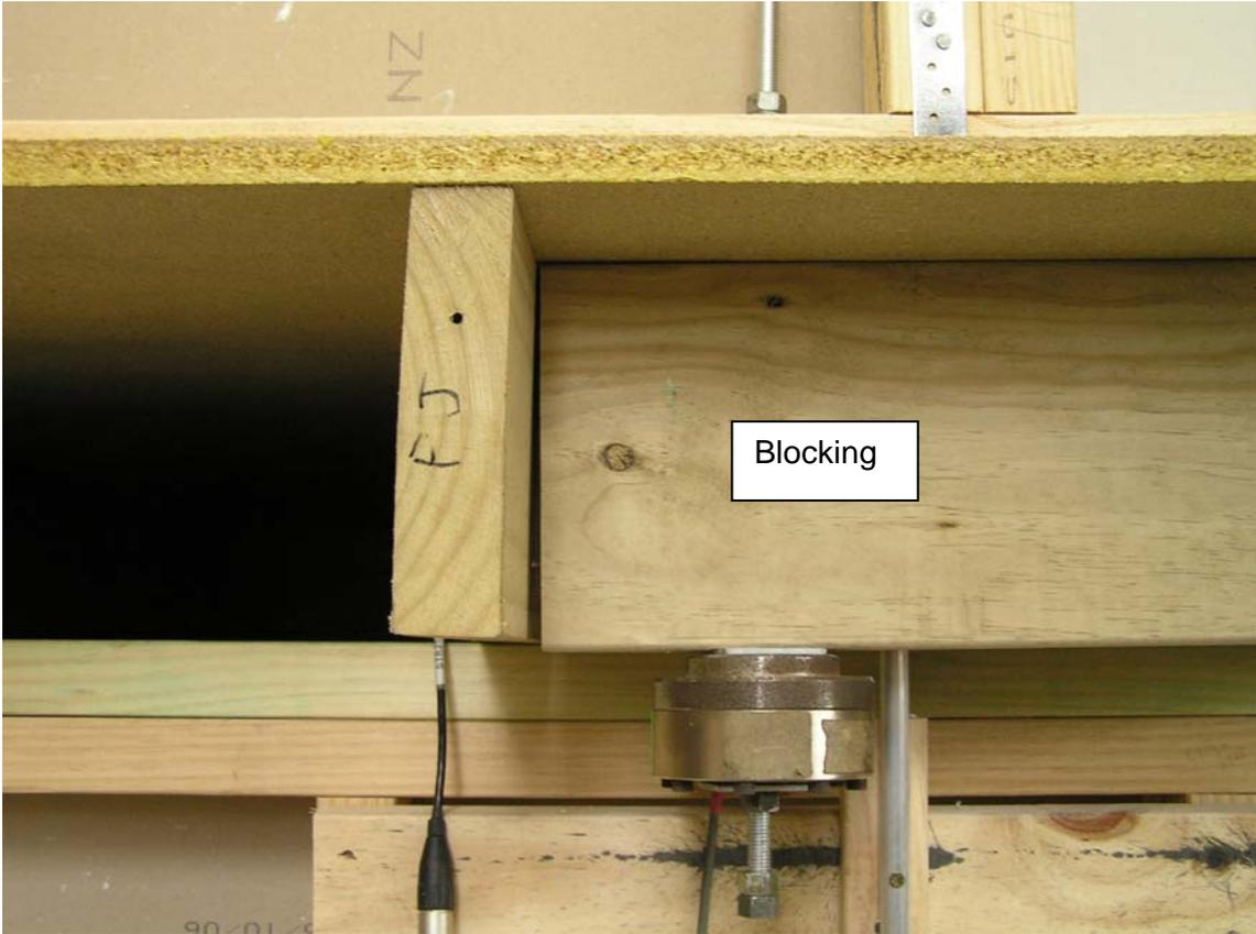
**Figure 18. Distortion of blocking and joists from racking loads in Side 1 for Test 1 of Stage I at +10 mm deflection**
