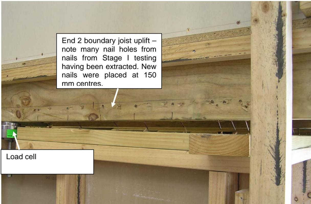
Figure 53. End 2 boundary joist uplift in latter stages of Stage III Test 1
