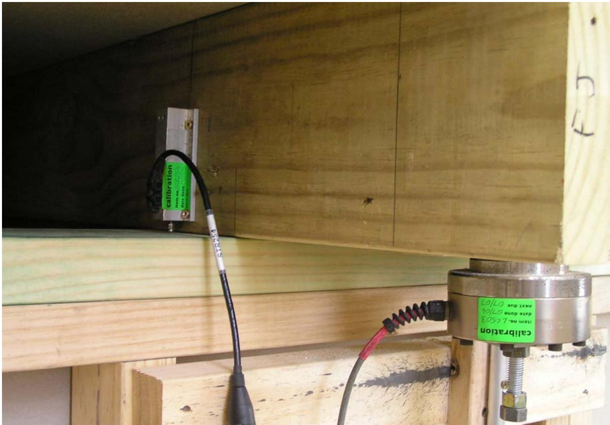
Figure 15. Measurement of floor joist uplift from the lower storey top plate
