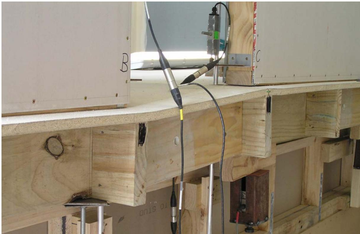
**Figure 21. Distortion from both upwards and downwards loads in Side 2 for Test 3 of Stage I at -40 mm deflection**
