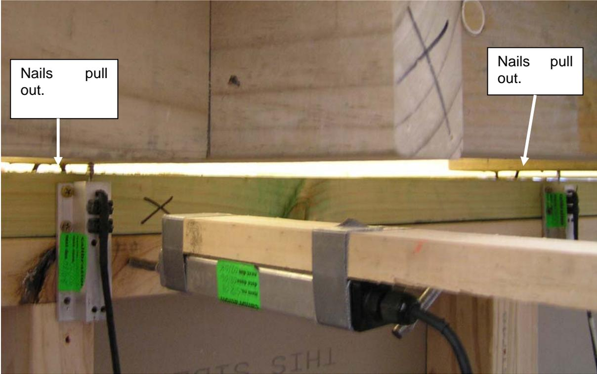
Figure 36. Joist uplift along Side 2 at joist ends for Stage II testing
