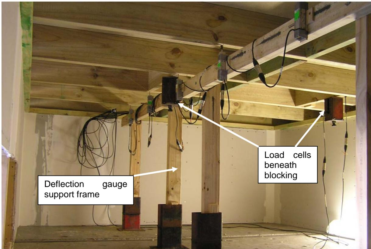
Figure 34. View under floor for Stage II testing
