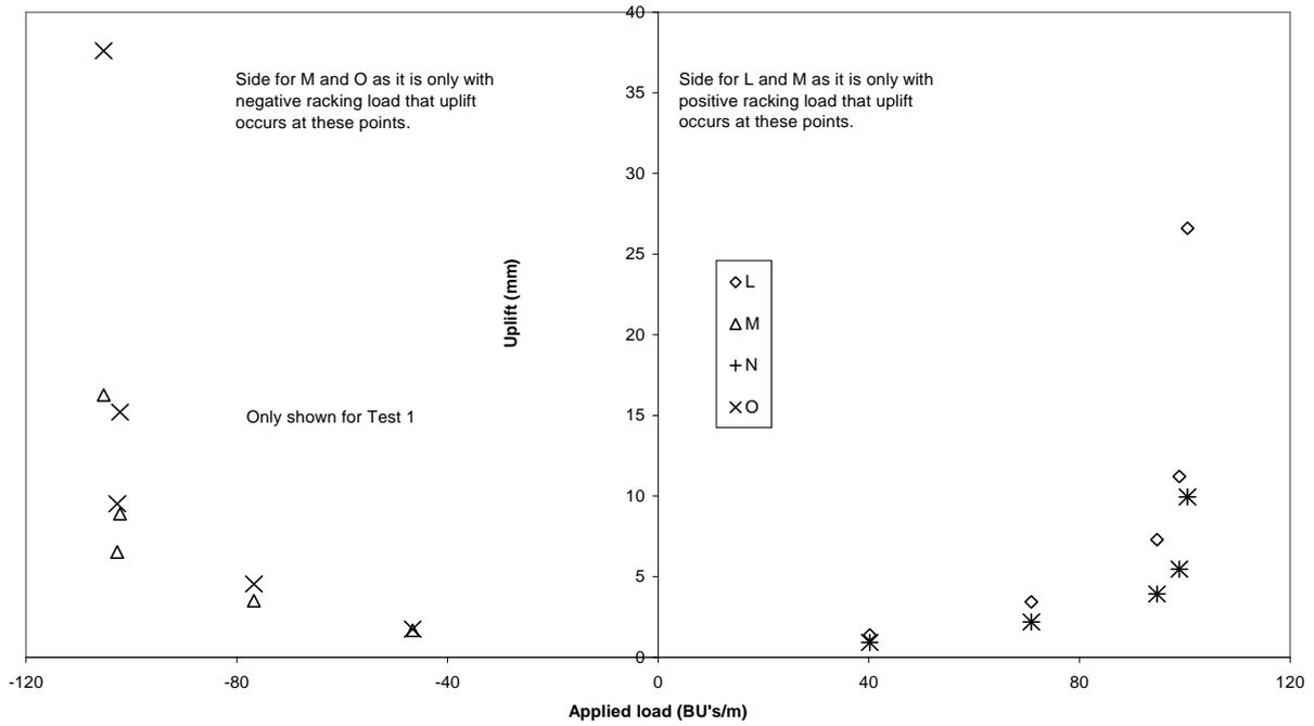
**Figure 62. Uplift of upper storey studs from lower storey studs versus racking load at End 2 for Stage III**
