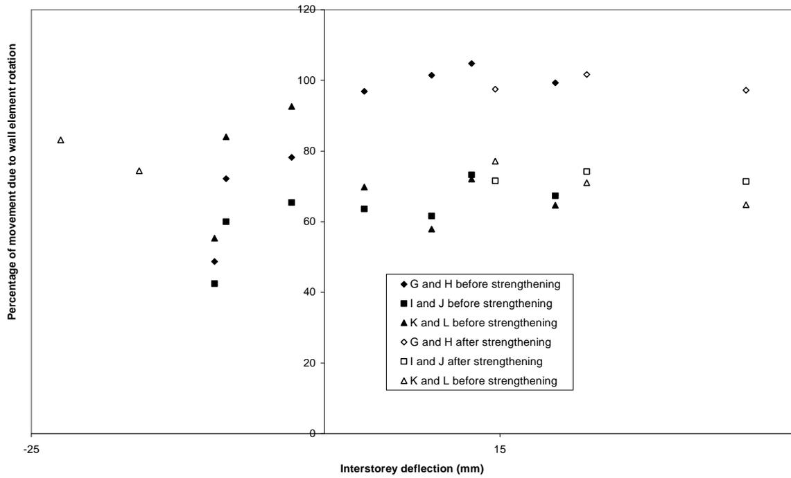
**Figure 30. Percentage of wall horizontal movement due to vertical movement at G, H, I, J, K and L measured during Stage I**
