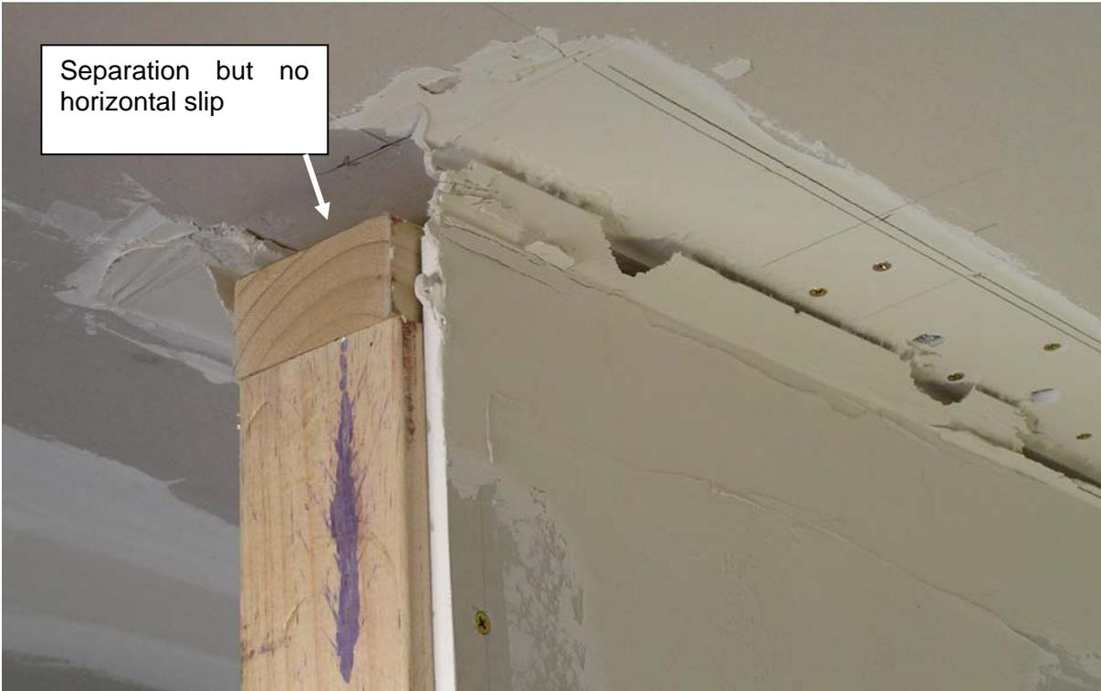
**Figure 40. Separation of internal wall top corner from ceiling in Stage II testing**
