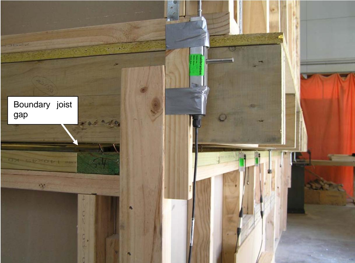
Figure 37. Joist uplift at corner for Stage II testing
