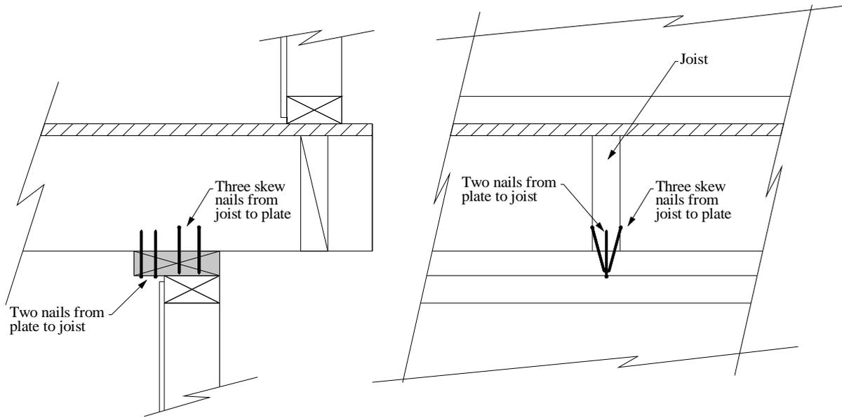
**Figure 50. Nailing of internal floor joists to top plate supports used in Stage III testing**
