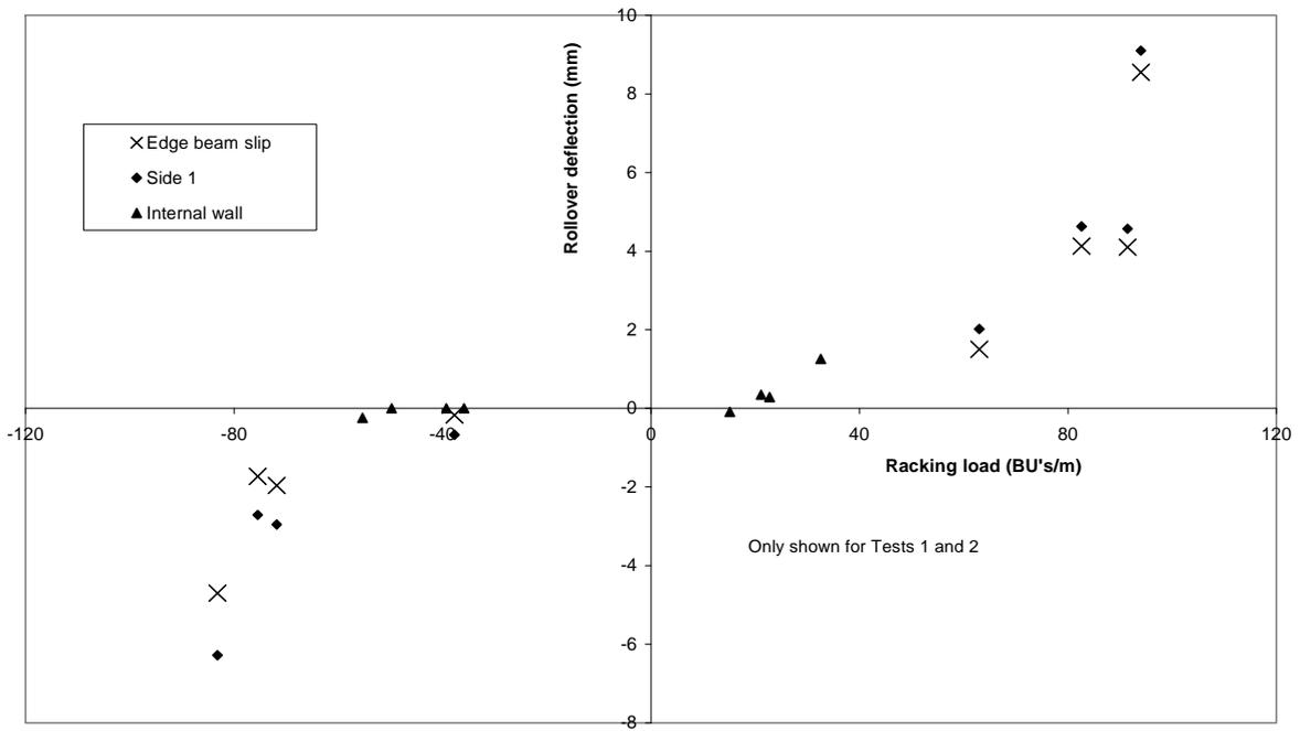
**Figure 43. Joist roll-over versus racking load for Stage II**
