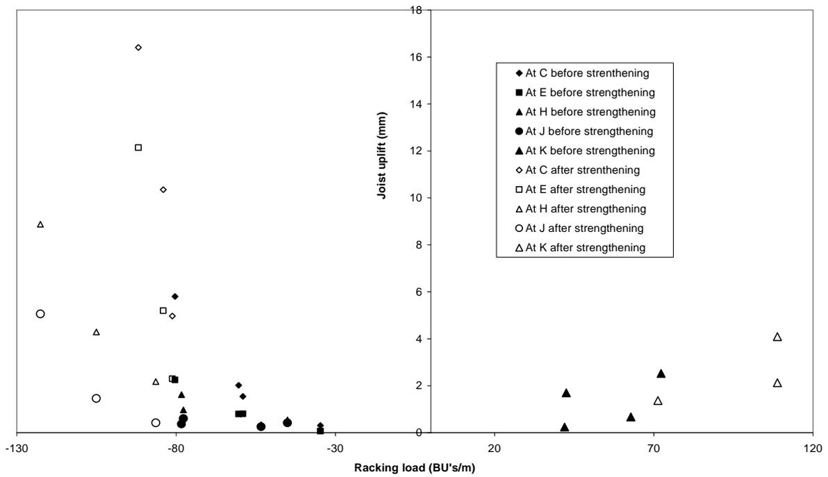
Figure 25. Joist uplift versus racking load on each side wall for Stage I
