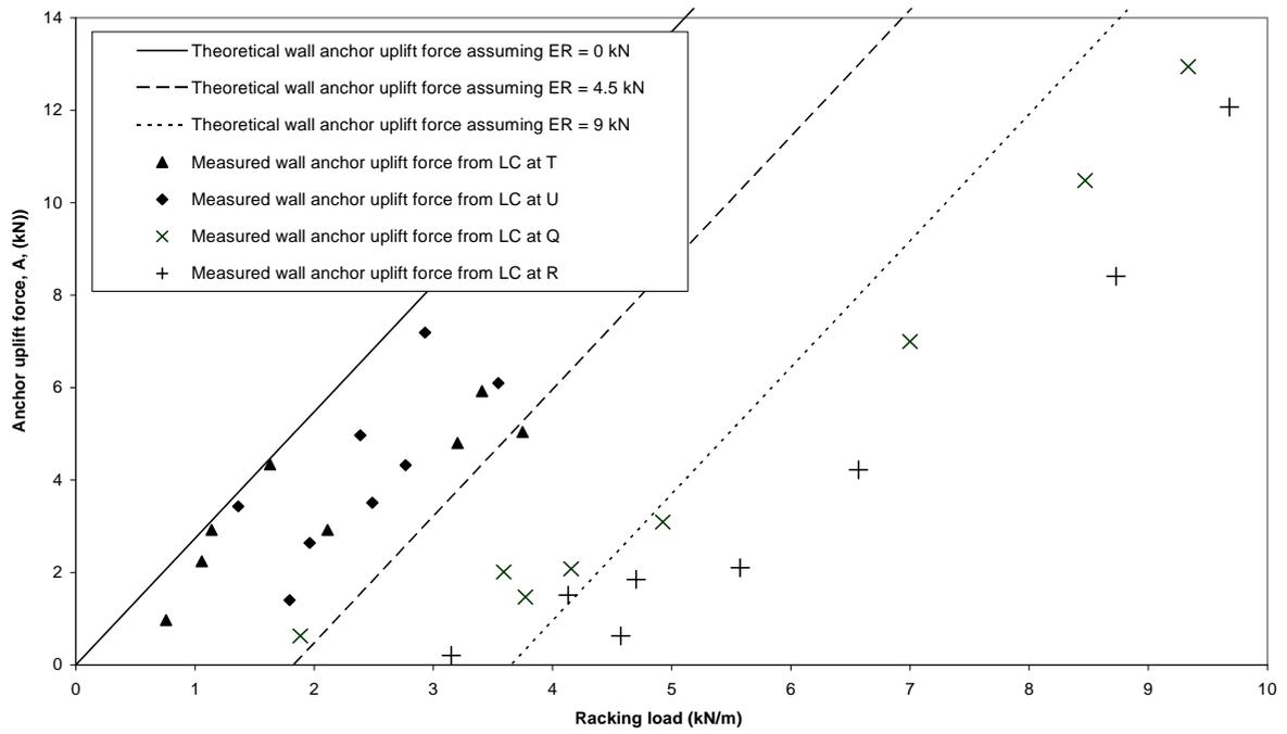
**Figure 48. Comparison of theoretical and measured uplift forces on bracing walls for Stage II**
