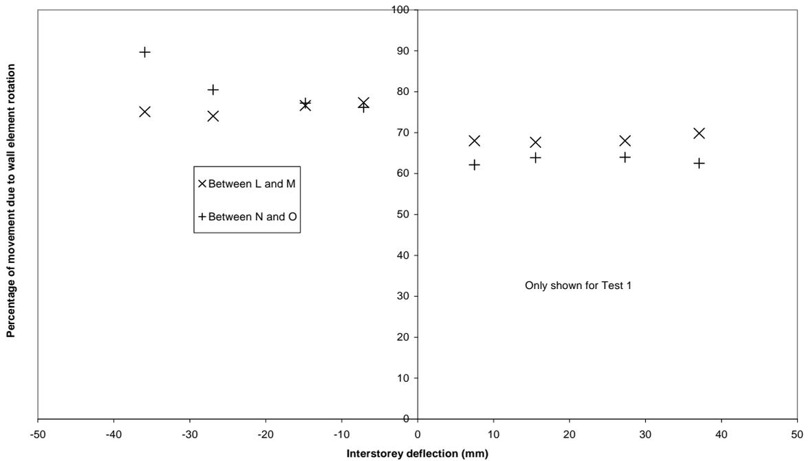
**Figure 63. Percentage of wall horizontal deflection due to 'rocking' versus racking load at End 2 for Test 1 of Stage III**
