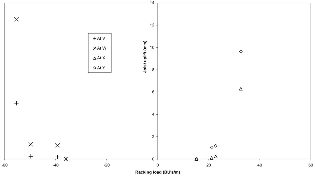
**Figure 42. Joist uplift from wall below versus racking load near the internal wall for Stage II**
