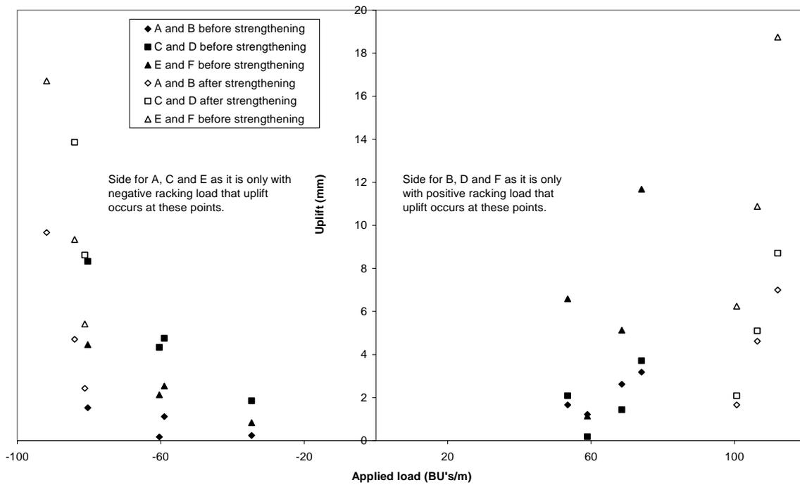
Figure 27. Inter-storey uplift movement at A, B, C, D, E and F measured during Stage I
