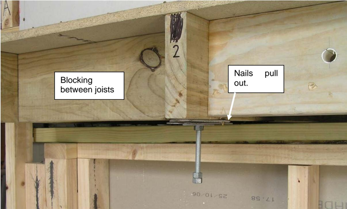
Figure 55. Joist uplift on side walls during Stage III testing
