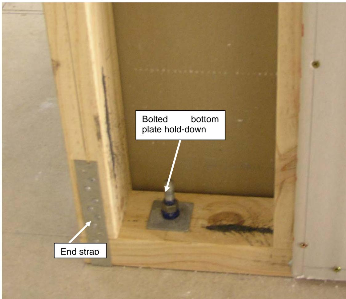
**Figure 51. Internal wall used for Stage III testing**
