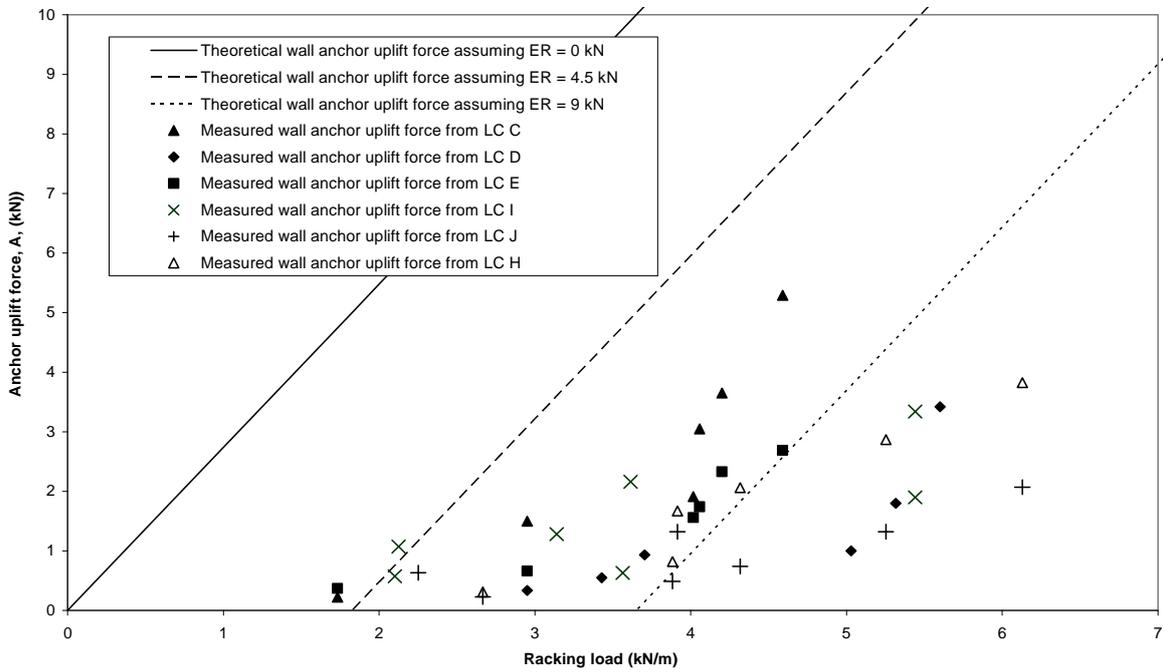
**Figure 31. Comparison of theoretical and measured uplift forces on bracing walls for Stage I**
