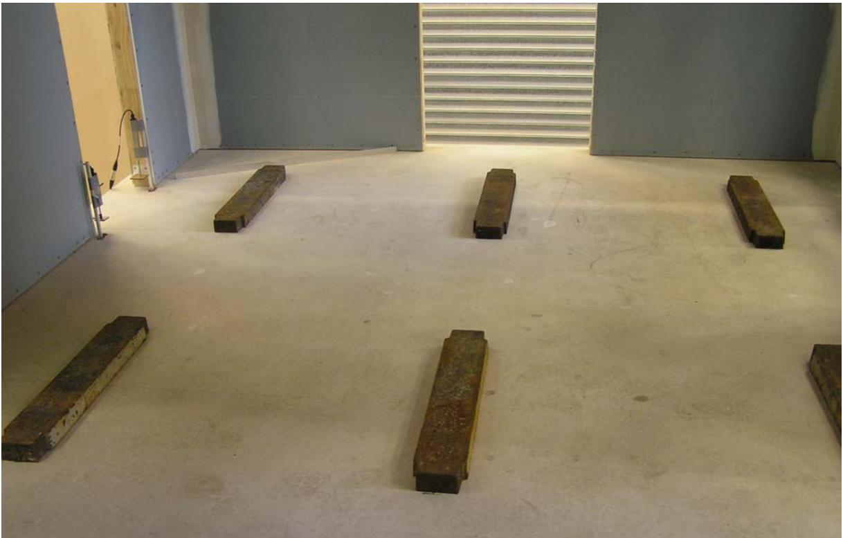
**Figure 12. Photograph of weights added to interior floor**
