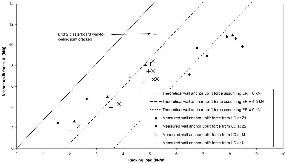
**Figure 69. Comparison of theoretical and measured uplift forces on bracing walls for Stage III**
