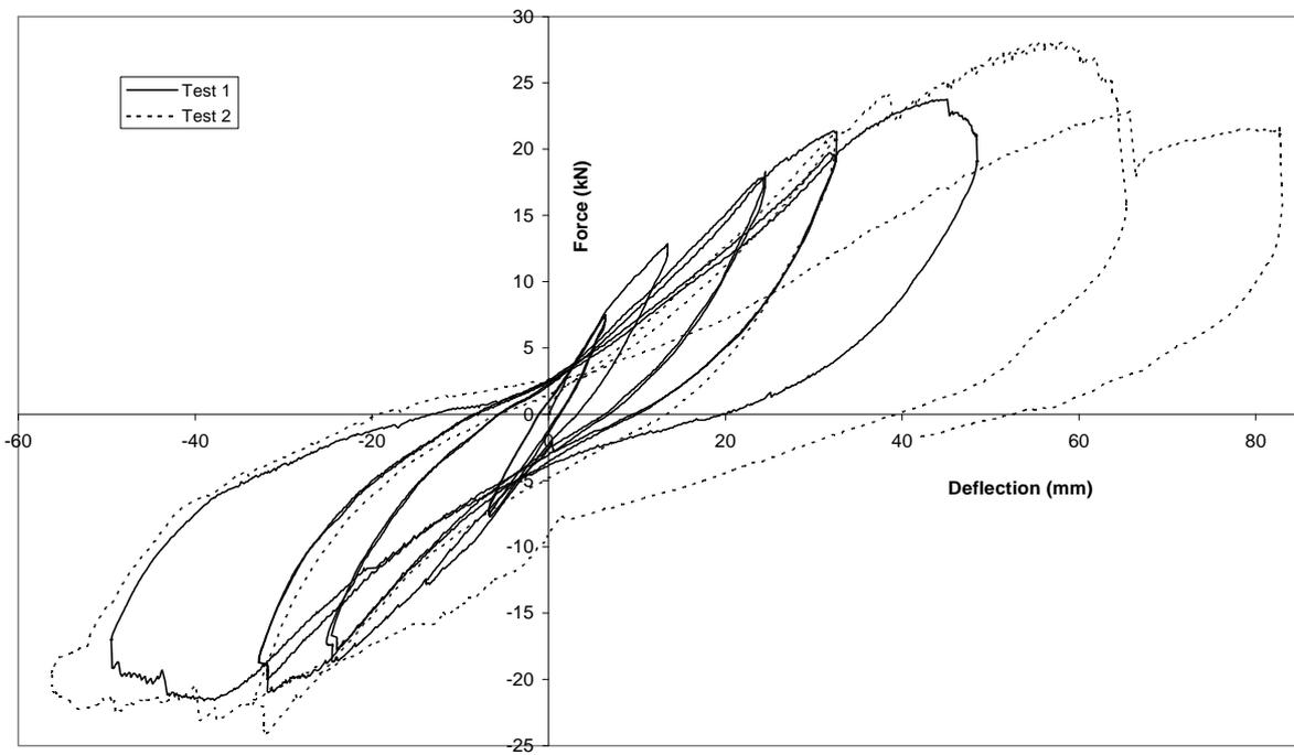
Figure 59. Total racking force versus average deflection for Stage III
