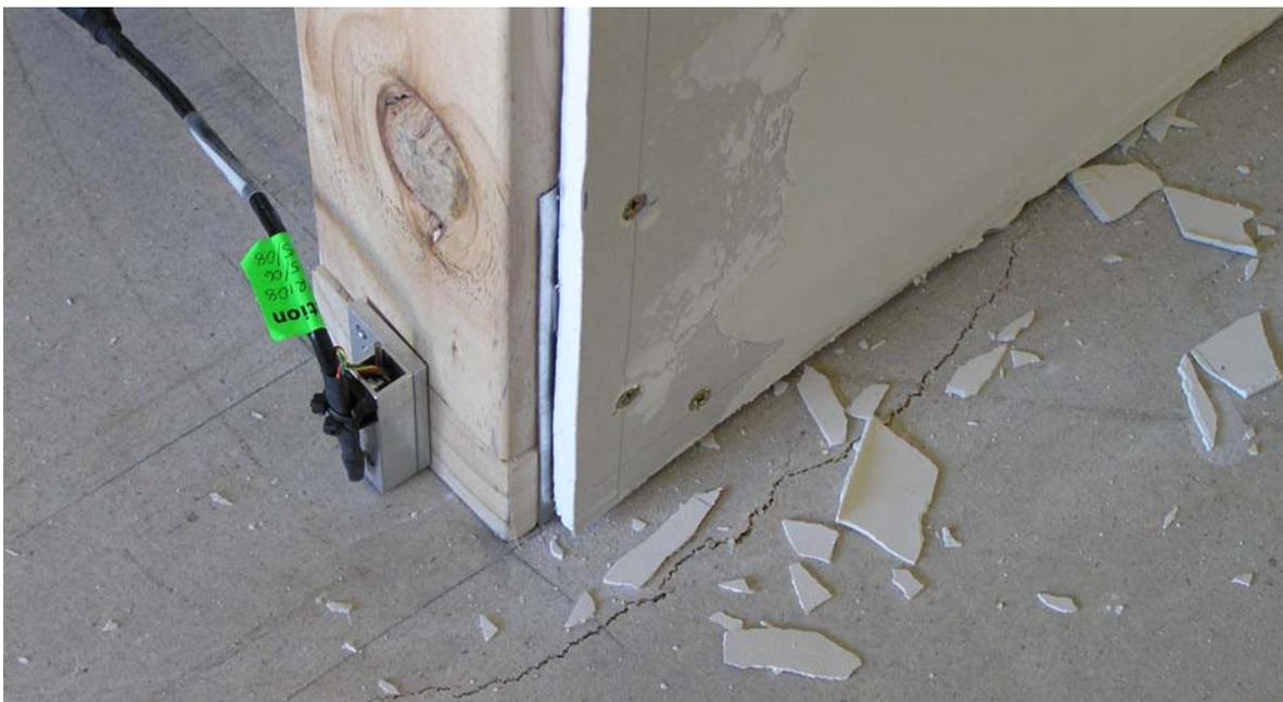
Figure 39. Flooring breakage due to blocking vertical movement at the internal wall for Stage II testing
