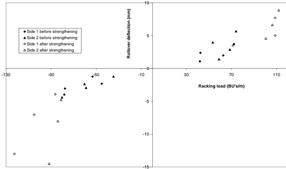
Figure 26. Joist roll-over deflections versus racking load on each side wall for Stage I
