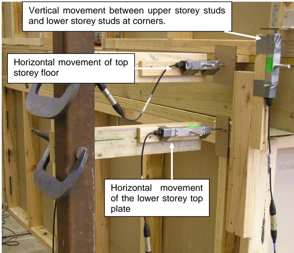
Figure 16. Measurement of horizontal deflections and inter-storey uplift of Side 1 in Stage I
