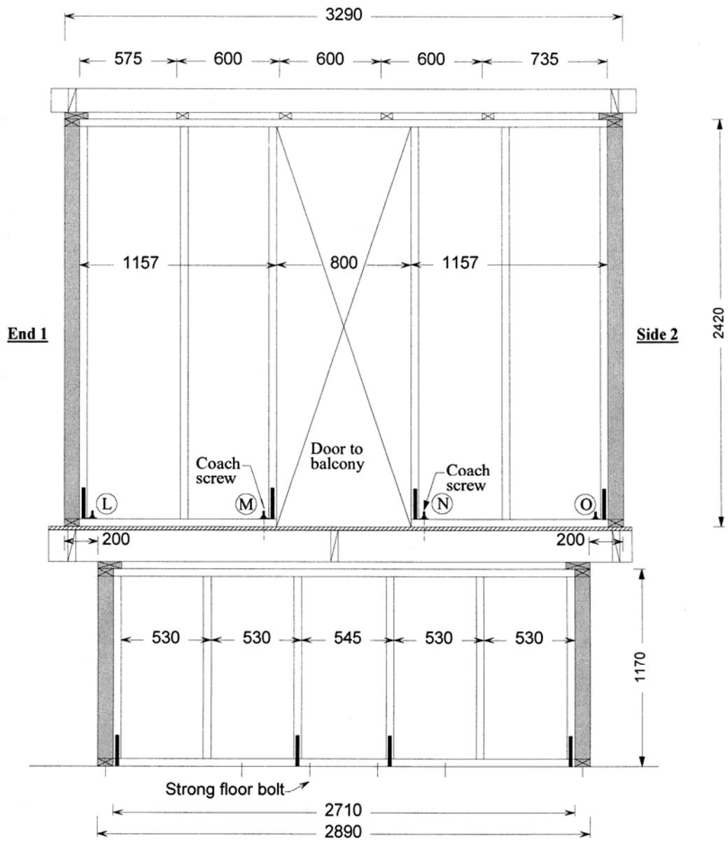
**Figure 6. End 2 wall framing**
