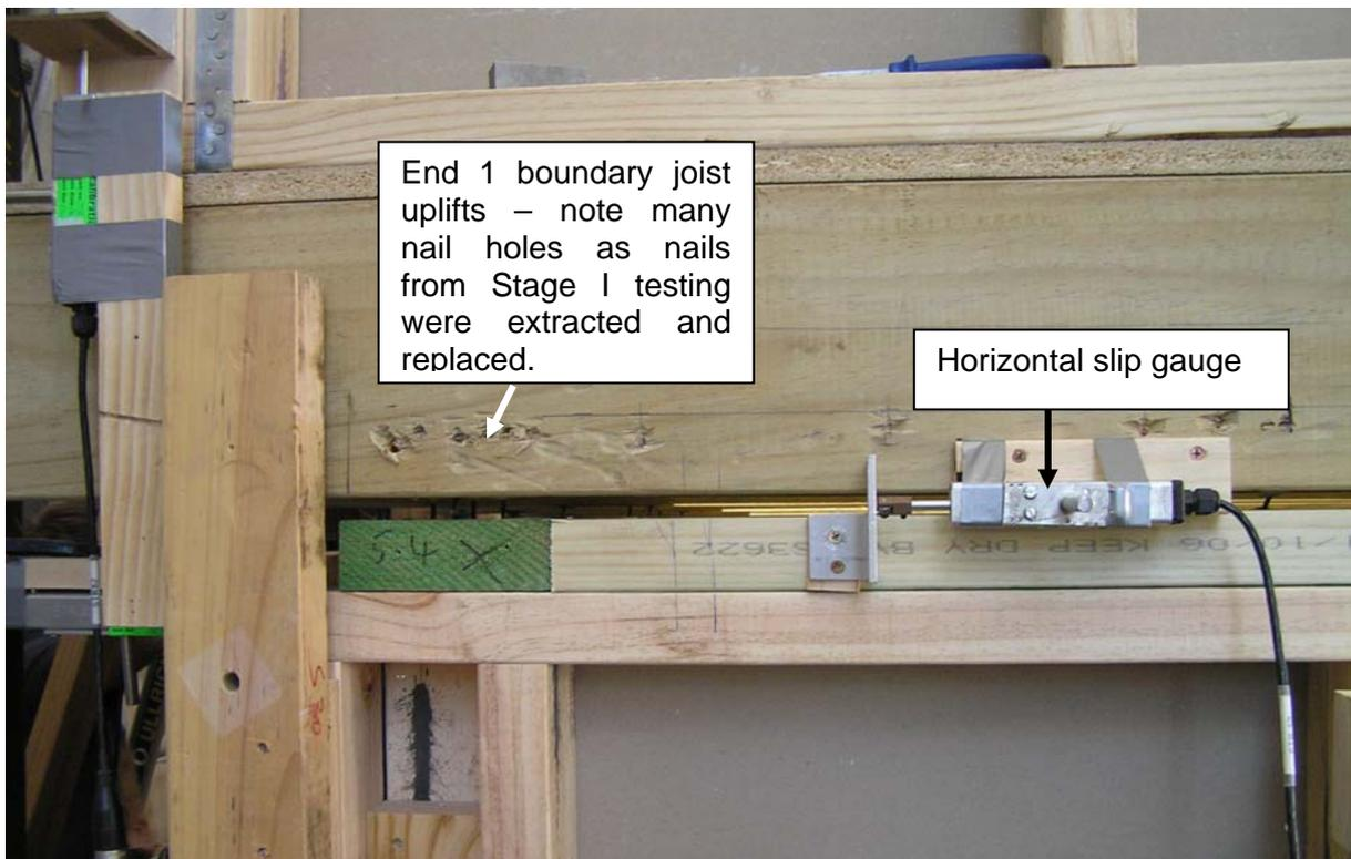
Figure 35. End 1 boundary joist uplift for Stage II testing
