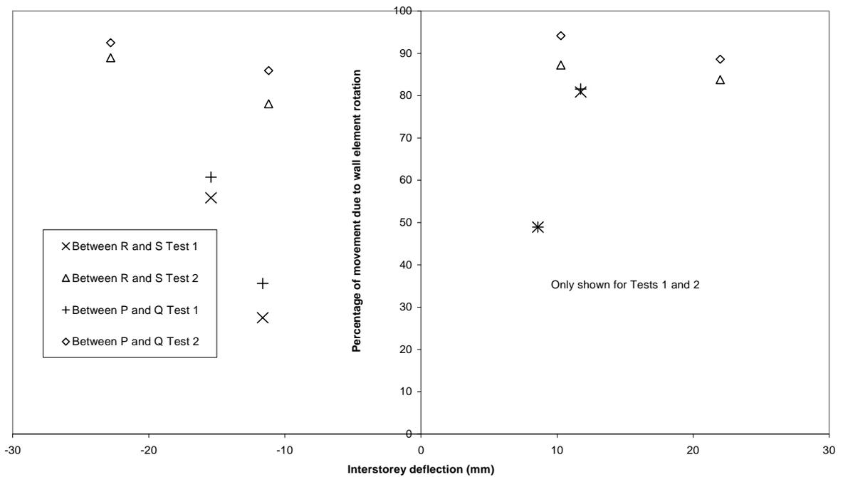
**Figure 45. Percentage of deflection due to 'rocking' versus racking load at End 1 for Stage II**
