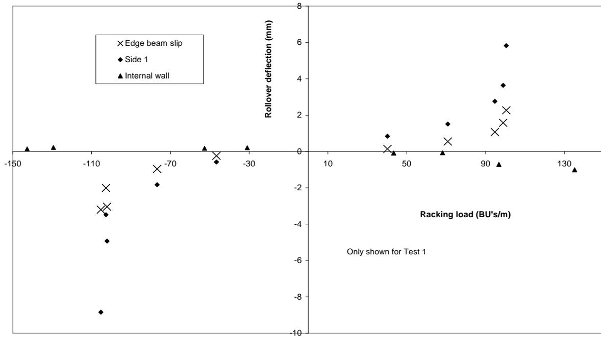
**Figure 61. Joist roll-over versus racking load for Test 1 of Stage III**
