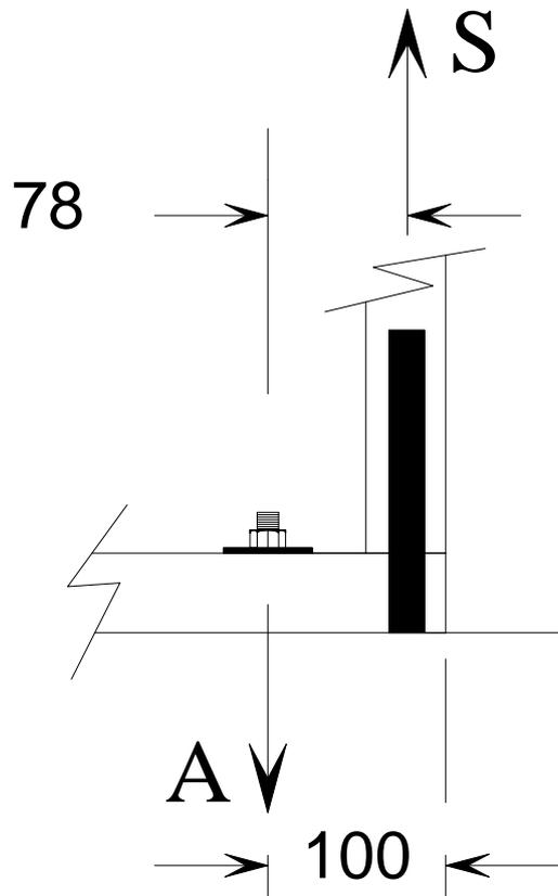
Figure 67. Flexural loading of bottom plate
