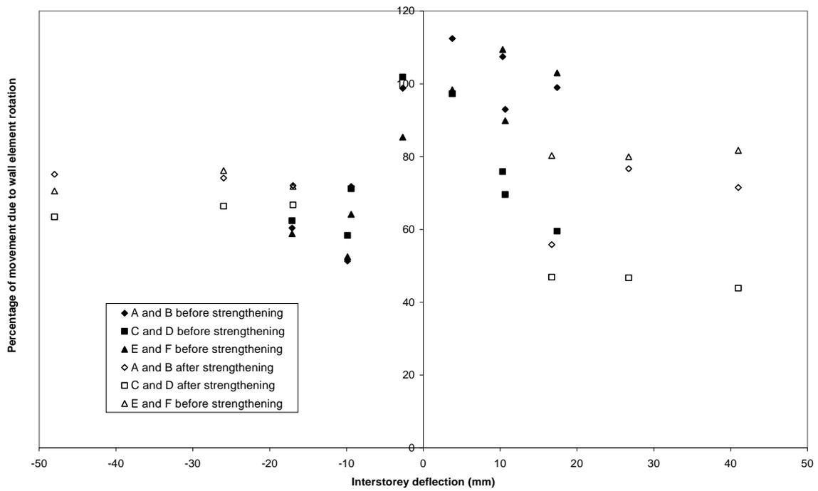
Figure 29. Percentage of wall horizontal movement due to vertical movement at A, B, C, D, E and F measured during Stage I
