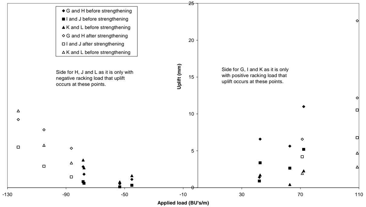
Figure 28. Inter-storey uplift movement at G, H, I, J, K and L measured during Stage I
