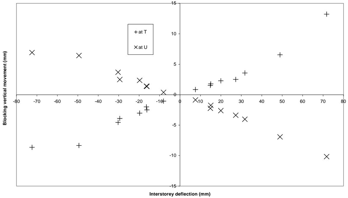
**Figure 46. Blocking vertical movement versus wall deflection at the internal wall for Stage II**
