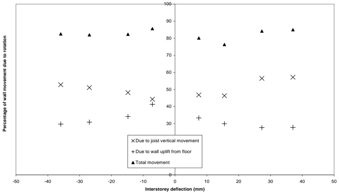
Figure 66. Percentage of deflection due to 'rocking' versus racking load at the internal wall for Stage III
