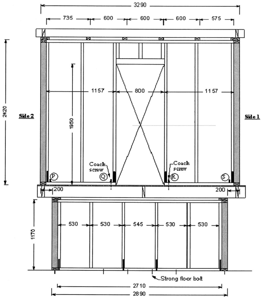
Figure 5. End 1 wall framing
