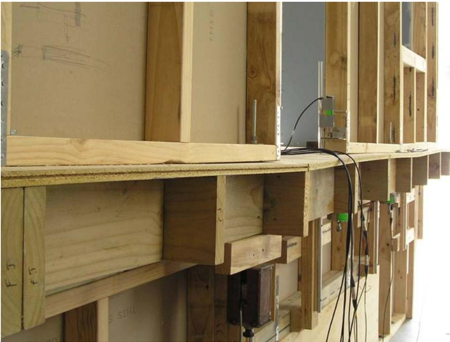
**Figure 19. Distortion of floor and blocking due to racking loads in Side 1 for Test 3 of Stage I at +25 mm deflection**
