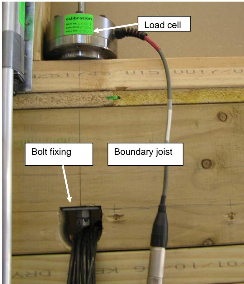
Figure 38. Measurement of axial load transferred to End 1 boundary joist for Stage II testing
