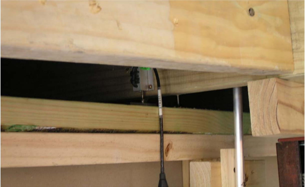
Figure 22. Joist uplift from wall below in Test 3 of Stage I at 40 mm deflection
