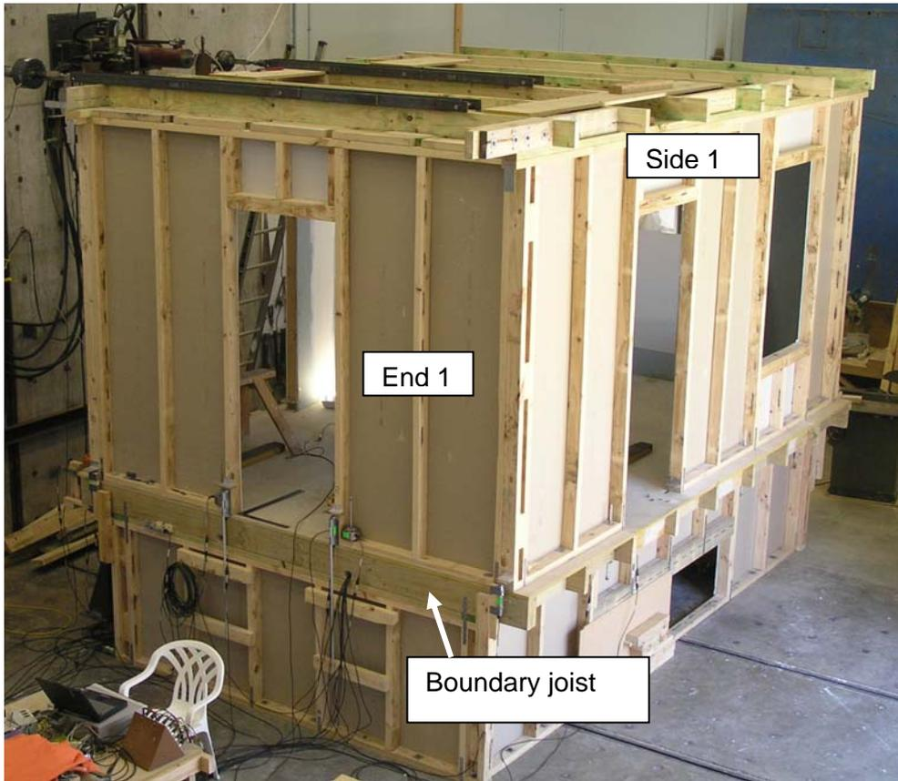
Figure 32. Test set-up for Stage II testing
