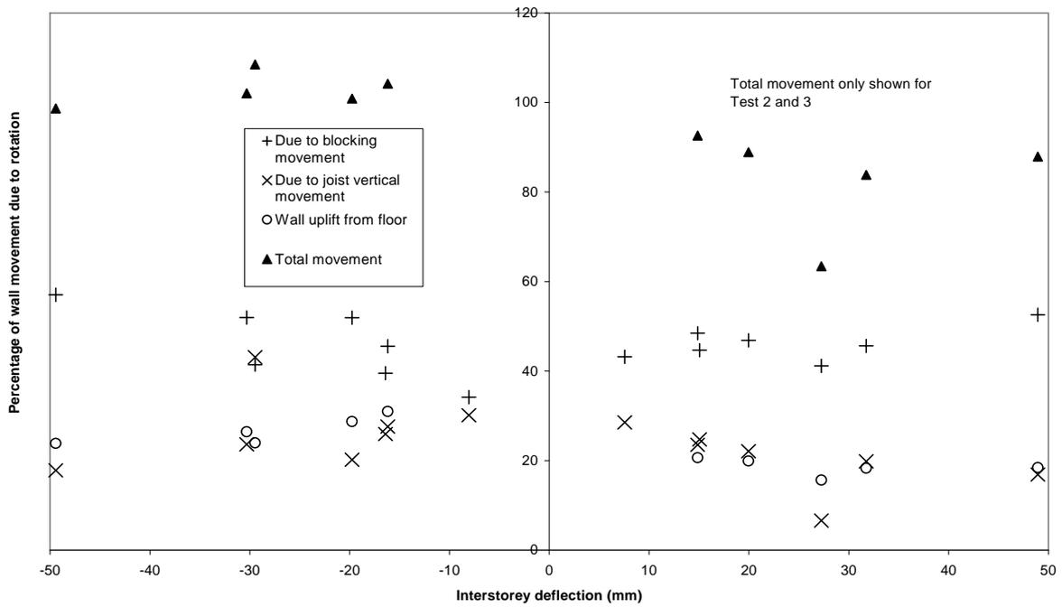
**Figure 47. Percentage of deflection due to 'rocking' versus racking load at the internal wall for Stage II**
