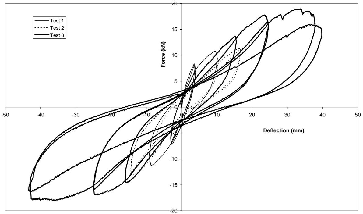
Figure 24. Total racking force versus average side wall deflections for Stage I
