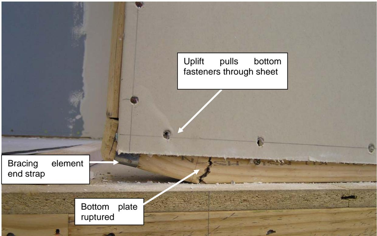
Figure 57. A second bottom plate failure late in Test 2 of Stage II at End 2
