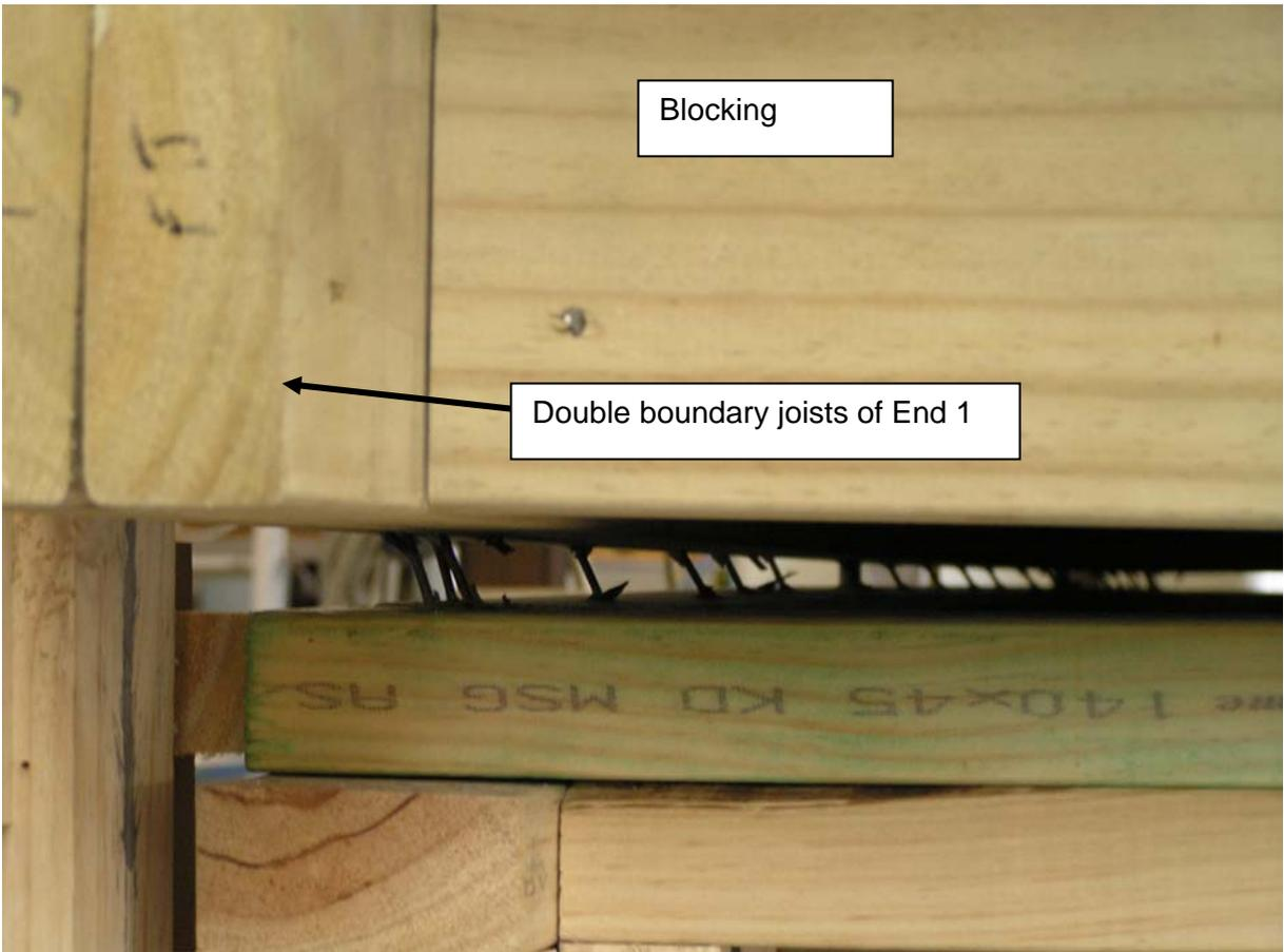
Figure 23. Close-up view of boundary joist uplift from wall below in Test 3 of Stage I at +40 mm deflection
