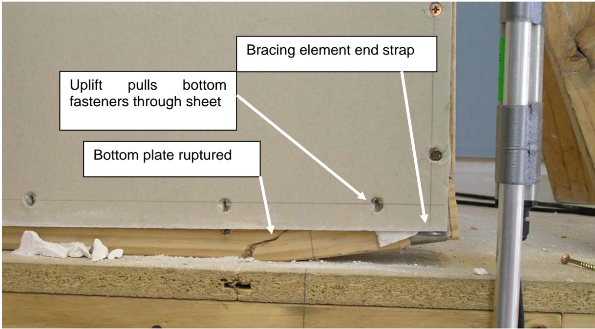
Figure 56. Bottom plate failure late in Test 2 of Stage II at End 2
