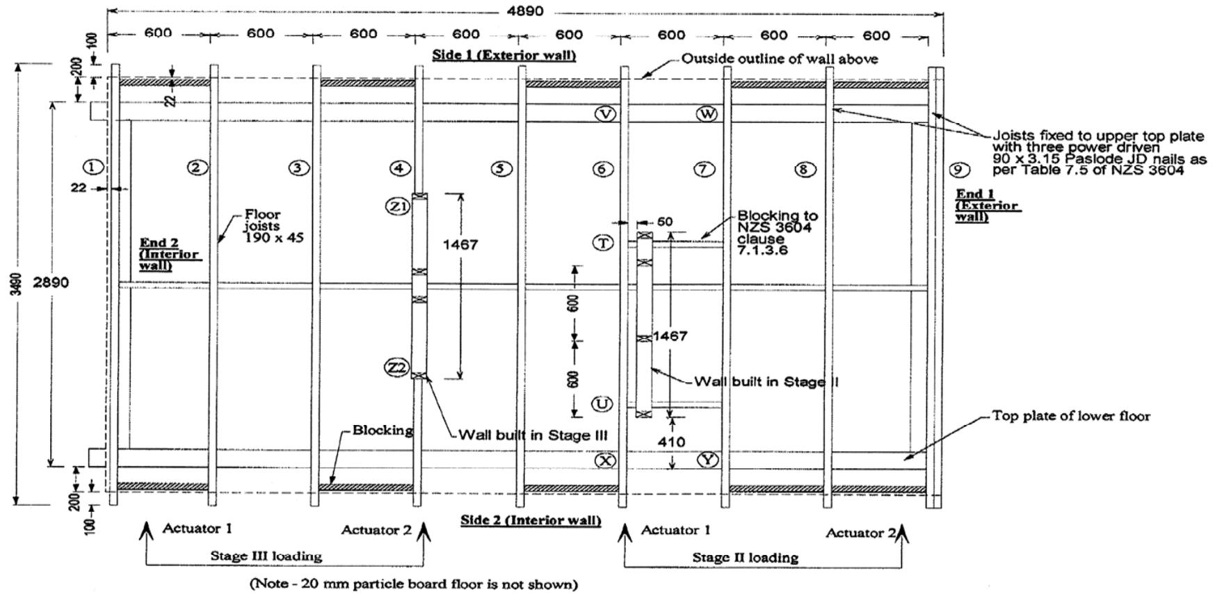
Figure 1. Plan view of floor framing
