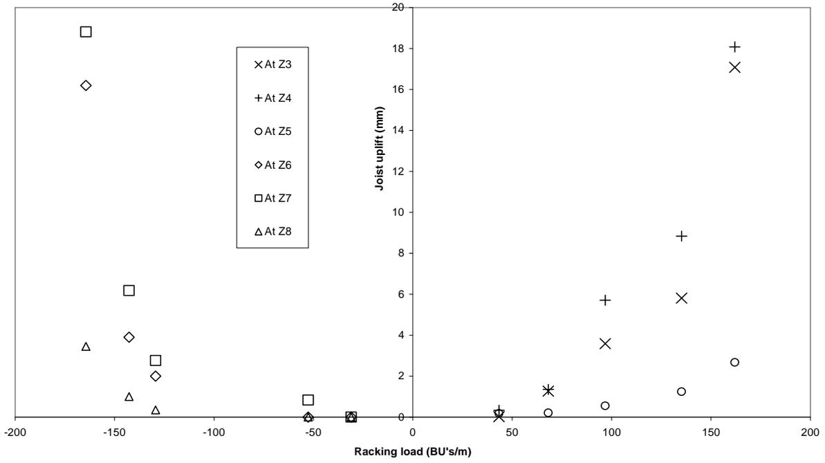
**Figure 60. Joist uplift from wall below versus racking load near the internal wall for Test 1 of Stage III**
