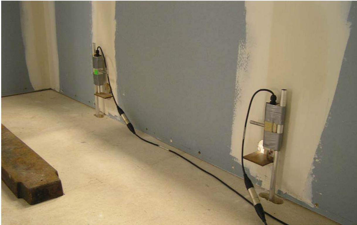
Figure 14. Measurement of inter-storey uplift
