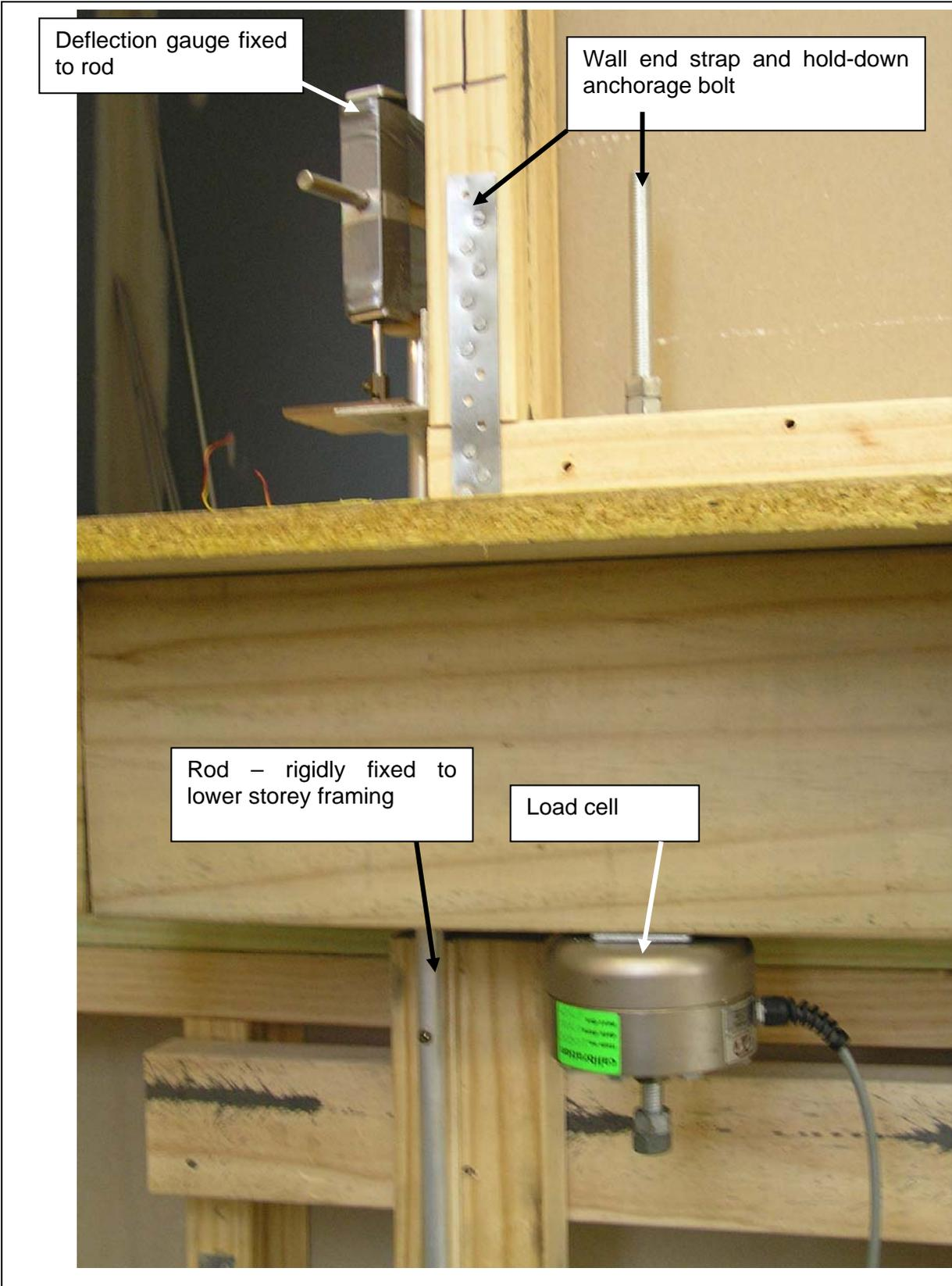
Figure 13. Measurement of inter-storey uplift and vertical load transfer
