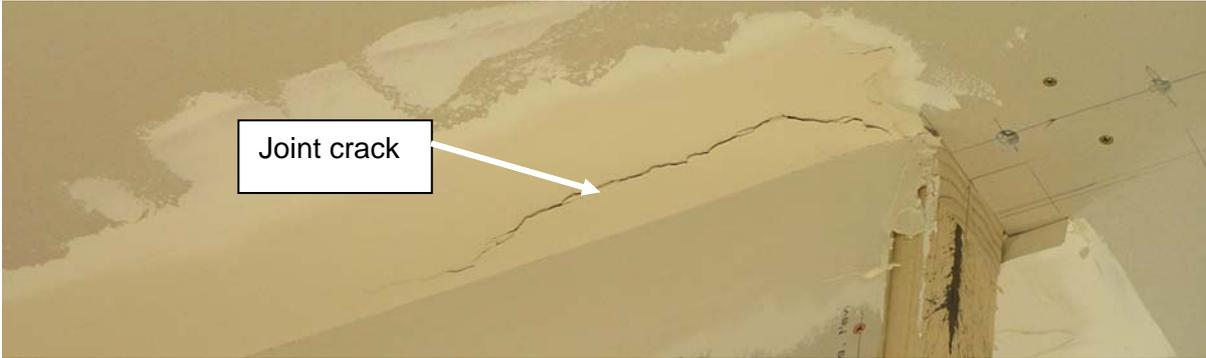
(a) Cracking from Test 1
