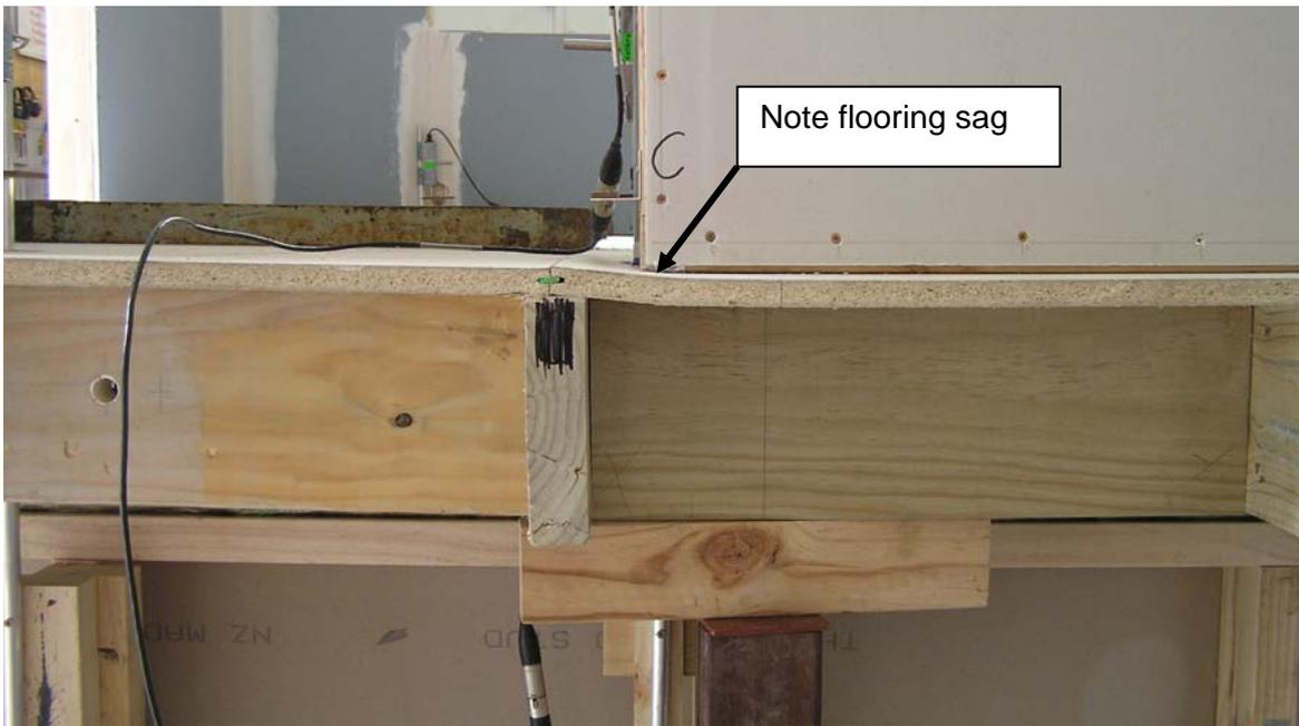
**Figure 20. End of bracing element compressing floor below in Side 2 for Test 3 of Stage I at +40 mm deflection**
