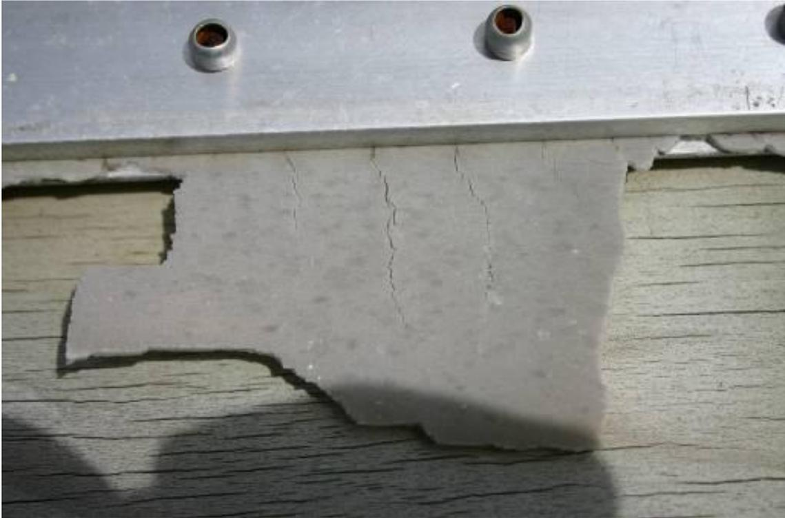
**Figure 13. Typical appearance of the PP sheet after three years of outdoor exposure**
