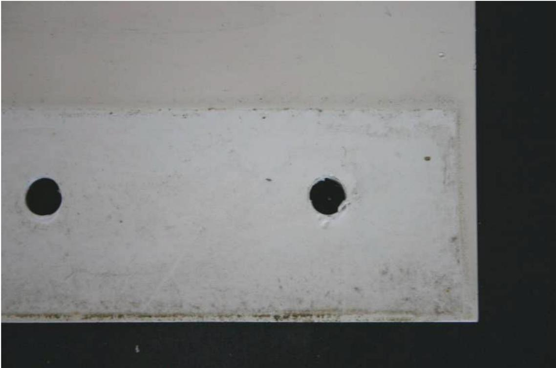
**Figure 30. uPVC sample from the Kaitaia exposure site collected in 2005 – the bottom of the sample was covered by the stress rack clamp during exposure and is markedly lighter than the exposed area of the sample**
