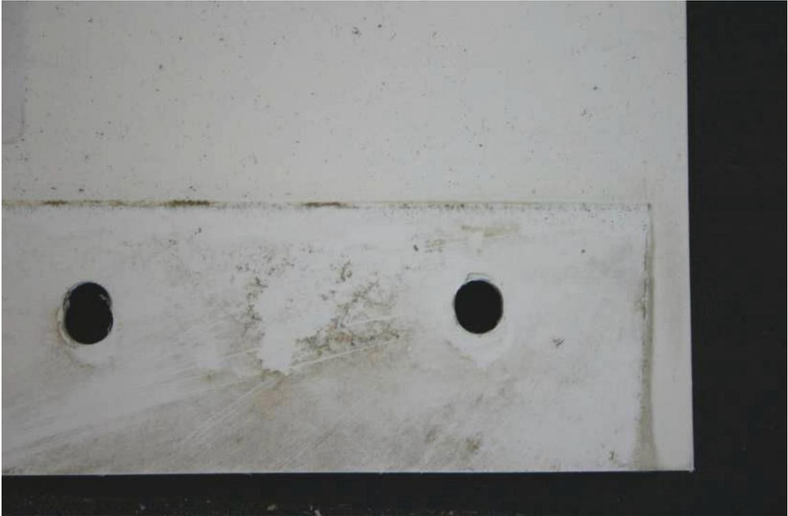
**Figure 31. uPVC sample from the Kaitaia exposure site collected in 2006 – the bottom of the sample, covered by the stress rack clamp during exposure, is now much more similar in appearance to the exposed area of the sample**
