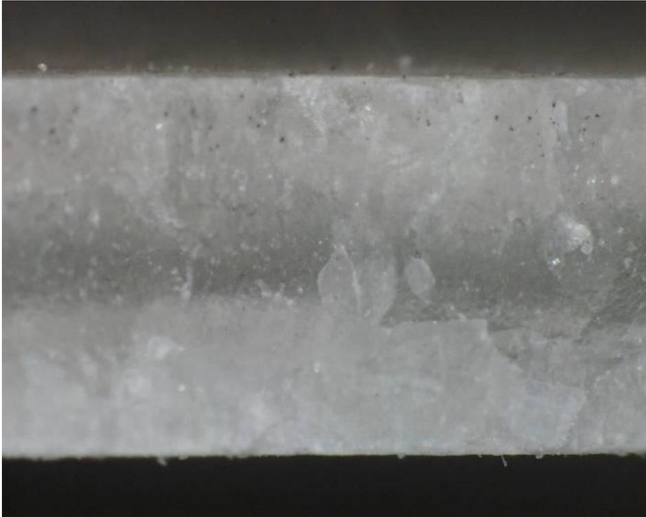
**Figure 15. Optical microscope image of PP sheet edge showing penetration of the microcracks into the sheet after three years of exposure**
