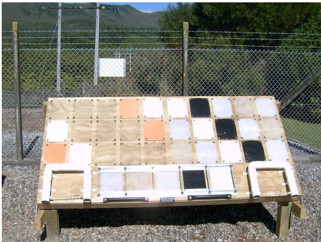
**Figure 8. Exposure rack configuration used on the additional exposure sites**
