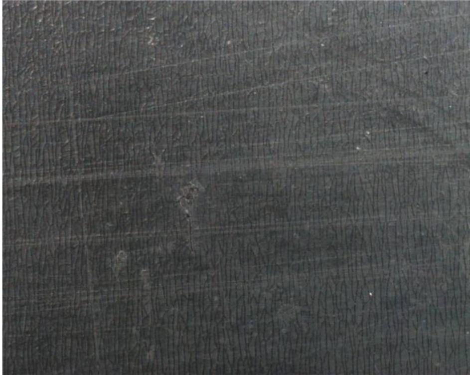
**Figure 20. Optical microscope image of micro-cracks in black PE sheet**
