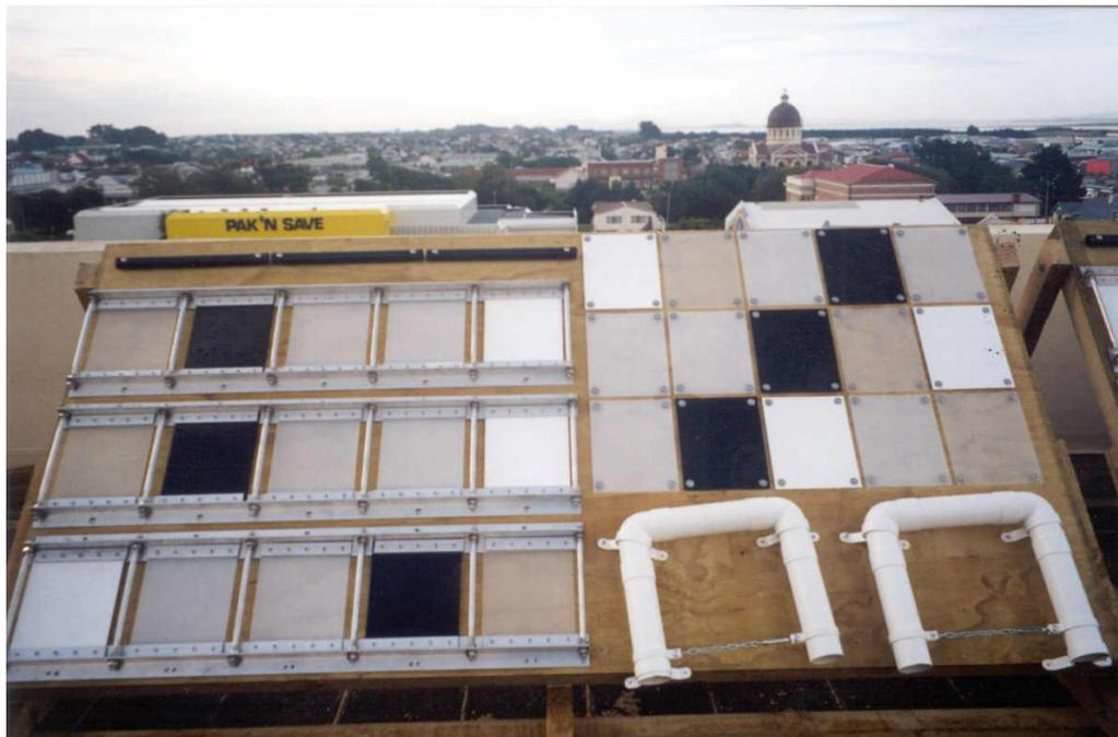
**Figure 7. BRANZ exposure rack configuration**
