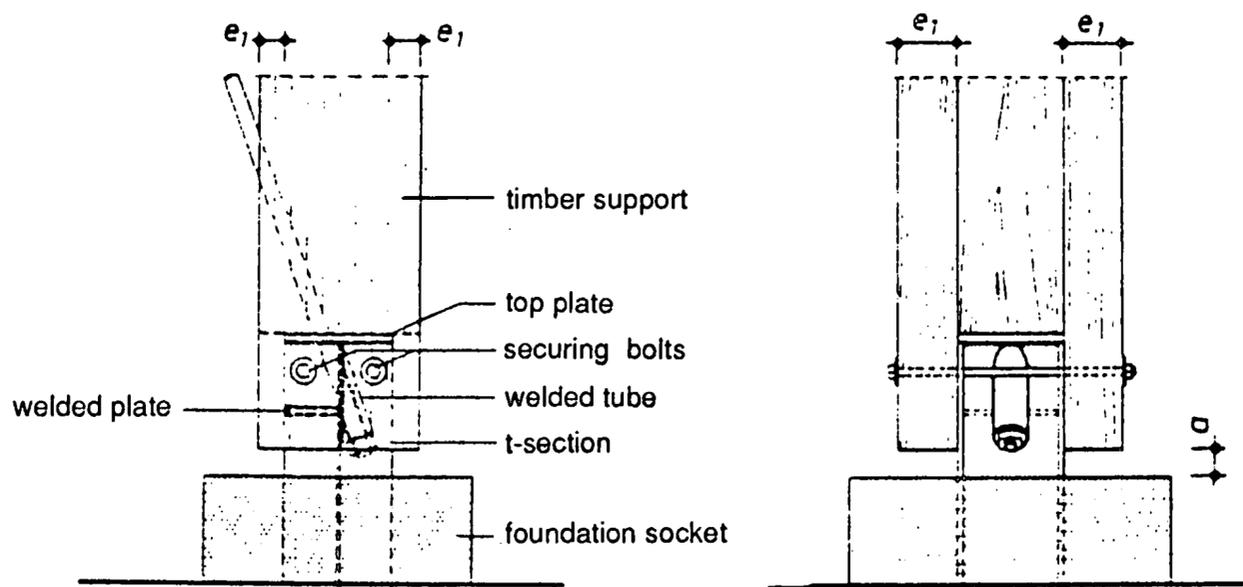
**Figure 8.4:** Column base joint [8.1] which satisfies the requirements of F30 if  $50 \leq a \leq 100$  mm and  $e_1 \geq 40$  mm. The bracing and its anchorage must be suitably protected.
