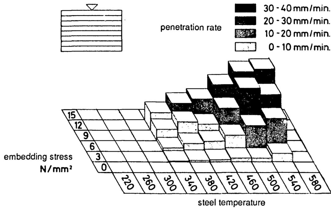
**Figure 4.12:** Penetration rates at force-fibre angle 90°. Each column represents average initial rate measured by four tests, regardless of the two dowel diameters [4.10].
