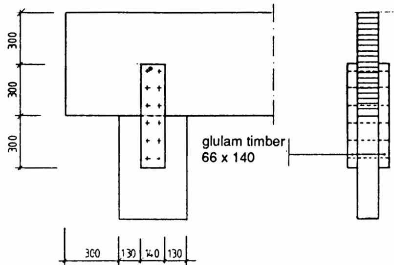
Figure 8.7: Fire tested beam-to-column joint with glulam timber gussets.
