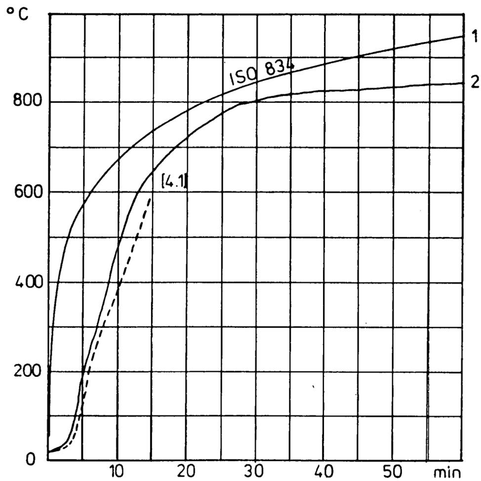
**Figure 4.2:** Temperature of flat plates during fire testing of beam-to-column joints in Figure 4.1 [4.1], [4.4]
