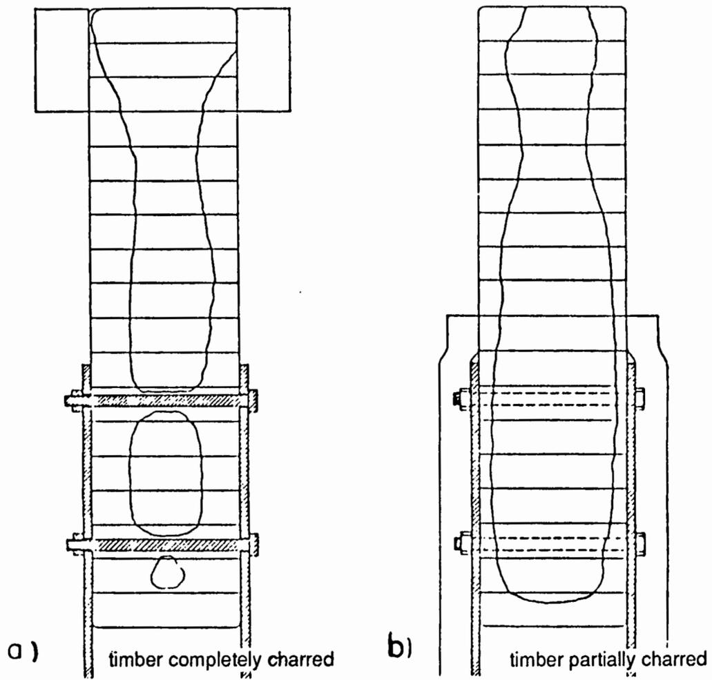
Figure 8.9: Vertical sections through the joint in Figure 7.5 after 60 minutes of standard fire [8.6], a) without protection, b) with fire protection.
