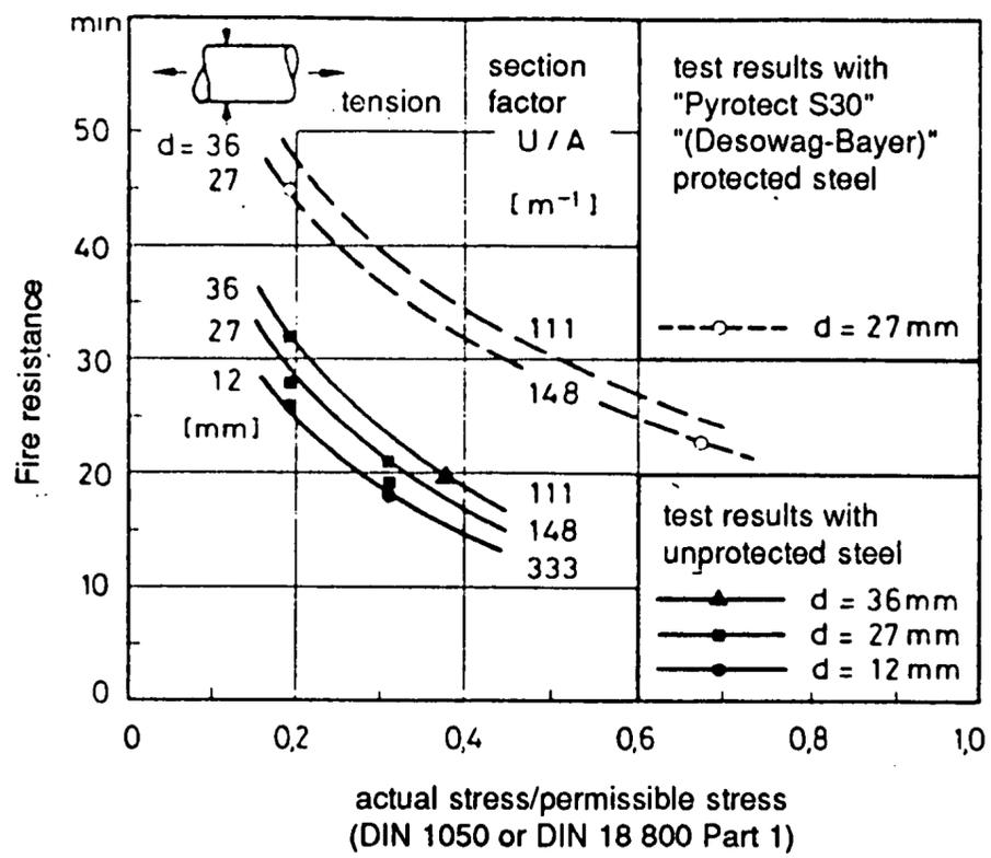
**Figure 7.1:** The fire resistance of round steel bars with and without fire resistant coatings as a function of the permissible stress and the bar diameter [7.5].
