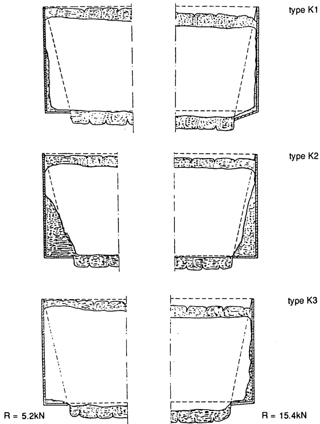
Figure 8.18: Vertical sections (along the beam) through the details in Figures 8.14 and 8.15 after 30 minutes of fire test [8.4].
