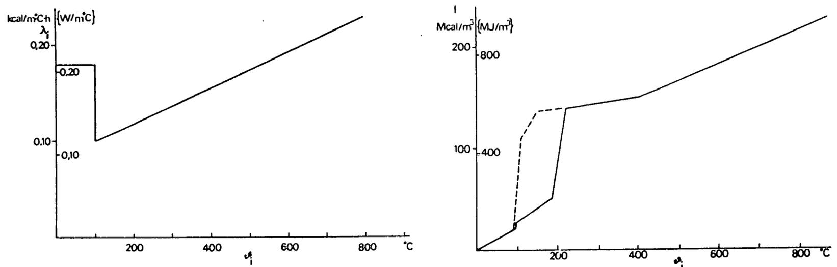
**Figure 7.9:** Conductivity and heat absorption characteristics of gypsum plasterboard ( $= 790 \text{ kg/m}^3$ ) as a function of the temperature in the board [7.1]. The full curve is for the board exposed to direct fire and the dotted curve is for the board which was not exposed directly to the fire.
