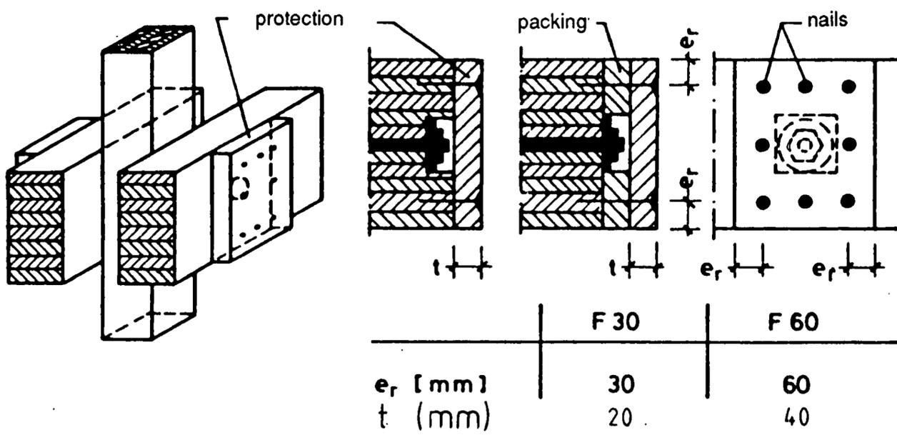
Figure 7.14: The required thicknesses of protections for bolted joints [7.5].
