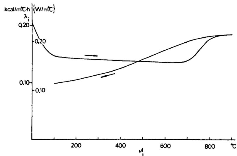
**Figure 7.2:** Conductivity of fire resistant plaster of the "Jimotherm" type as a function of the temperature in the plaster
