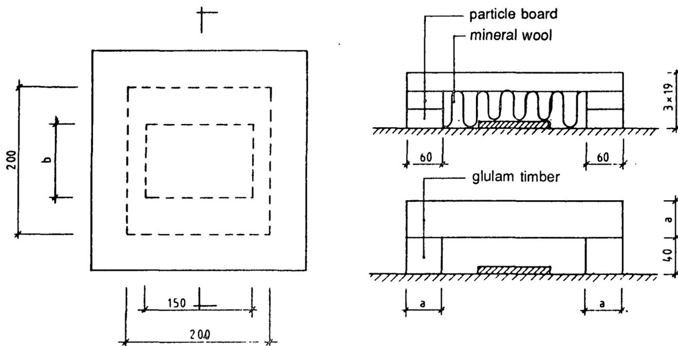
**Figure 7.12:** Samples for the study of temperature development during fire for steel gussets which have been protected with glulam timber or particle board [7.7].
