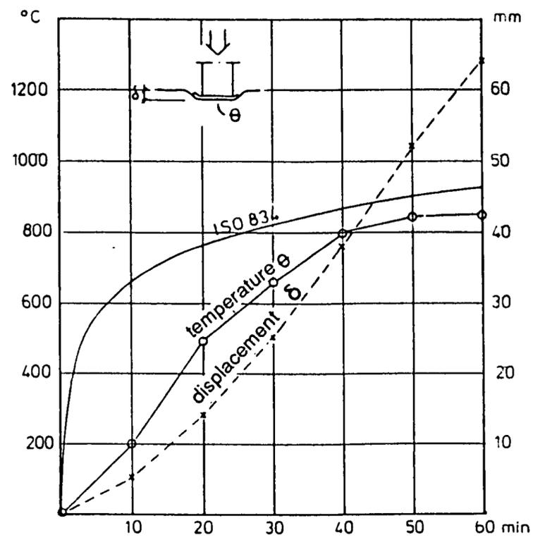
**Figure 4.3:** Temperature at the contact surface between the steel plate and the timber, and the displacement of the steel plate during the fire test in accordance with ISO 834.
