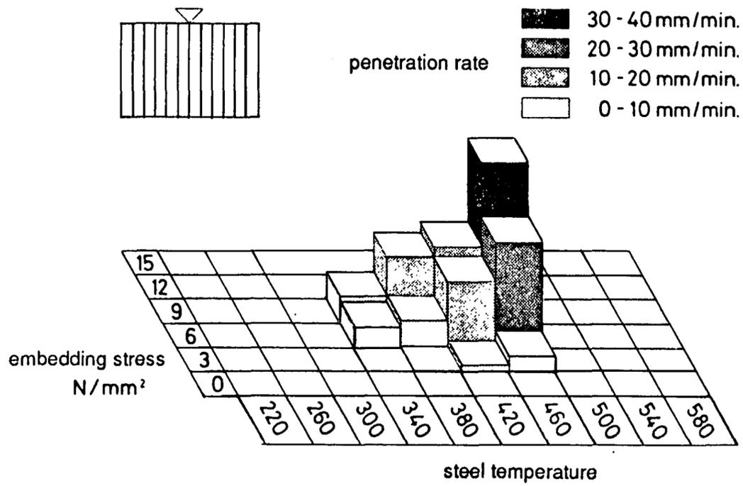
**Figure 4.11:** Penetration rates at force-fibre angle 0°. Each column represents average initial rate measured by four tests, regardless of the two dowel diameters [4.10].
