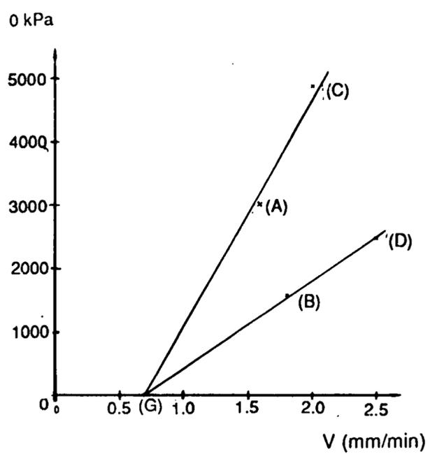
**Figure 4.6:** Empirical relationship between proof stress and the charring rate for the joints in Figure 4.4 [4.5].
