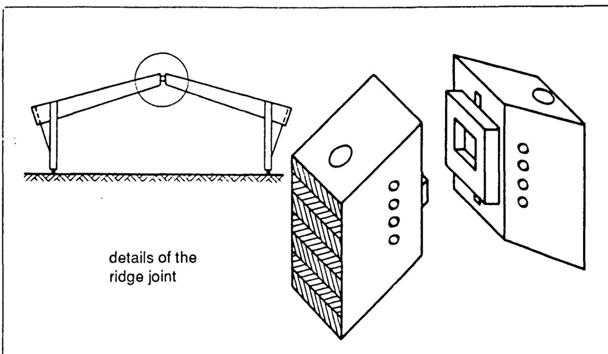
**Figure 8.22:** Fire tested hinged ridge joints which under certain conditions fulfill the requirements of F30 and F90 [8.1].
