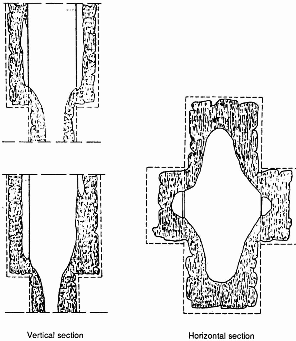
Figure 8.8: Vertical and horizontal sections through the beam-to-column joint as shown in Figure 8.7 after 60 minutes of standard fire [8.4].
