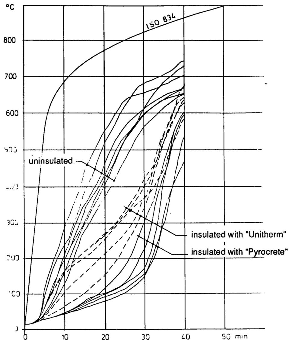
**Figure 4.7:** Temperature development in steel plates with or without insulation under fire tests in accordance with ISO 834 [4.6], [4.8].
