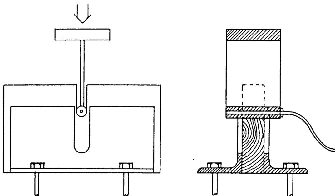
Figure 4.10: Test arrangements with an electrically heated dowel according to [4.10], and based on a photograph.
