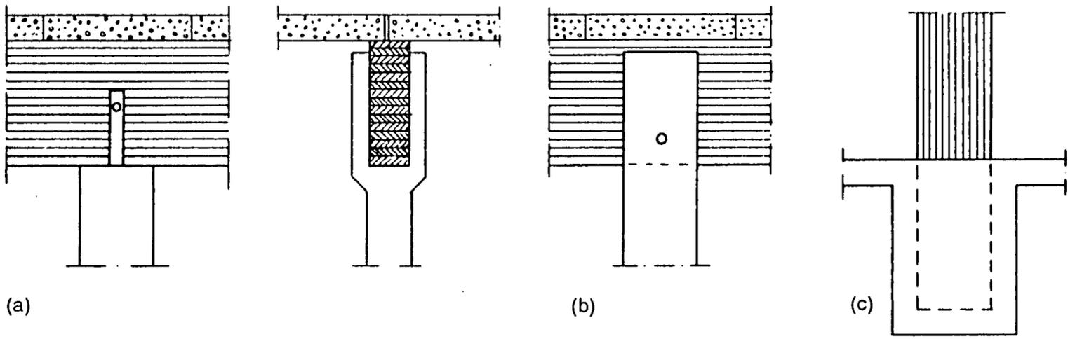
Figure 5.1: Examples of joints between concrete and glulam timber construction.
