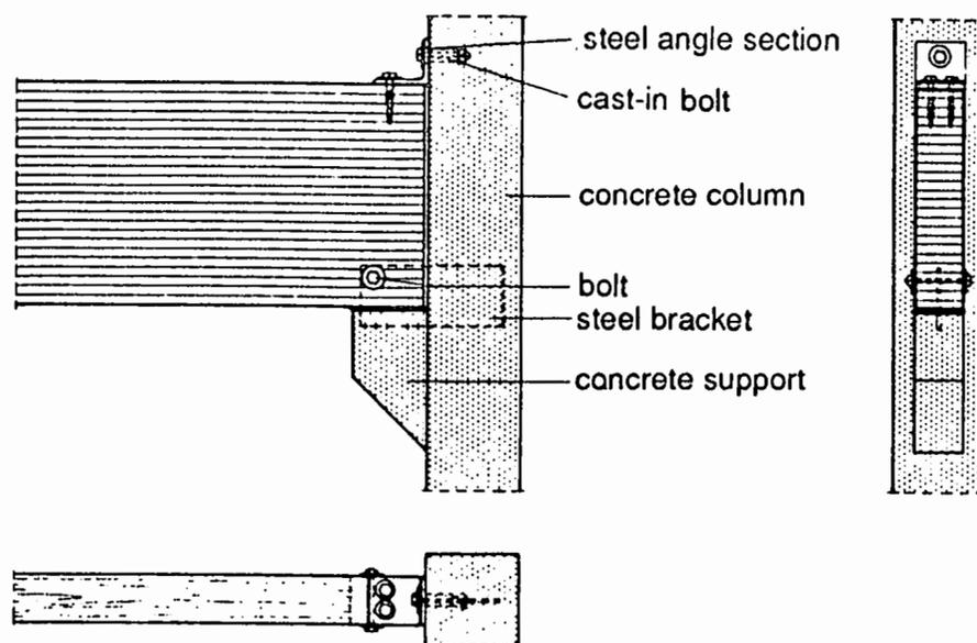
Figure 8.12: Beam-to-column joint with beam support made of concrete and side restraint of angle section is classified according to [8.7] as F30.
