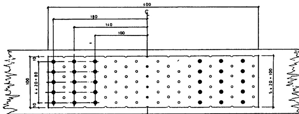
**Figure 4.8:** Fire tested timber joint with two nailed plates of 2.5 x 100 x 400 and 4 x 15 nails 40/60 [4.9].
