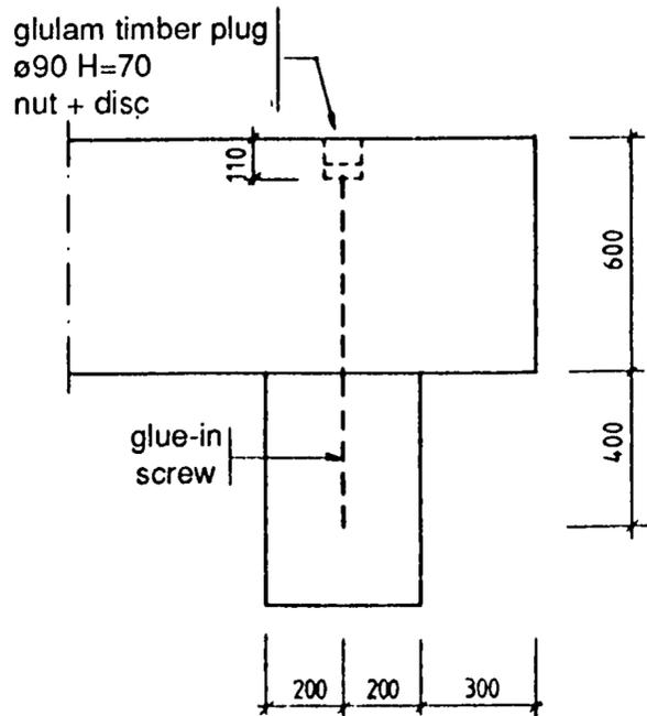
Figure 8.5: Fire tested beam-to-column joint with glue-in screw [8.4].
