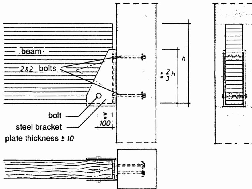
**Figure 8.13:** Beam-to-column joint with steel support bracket of minimum thickness of 10 mm, bolted to concrete or glulam timber columns which satisfies the requirements [8.1] for class F30.
