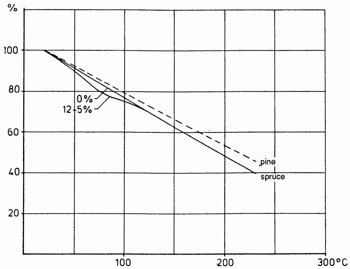
**Figure 1.3:** Relative shear strength as a function of temperature for spruce and pine [1.10].
