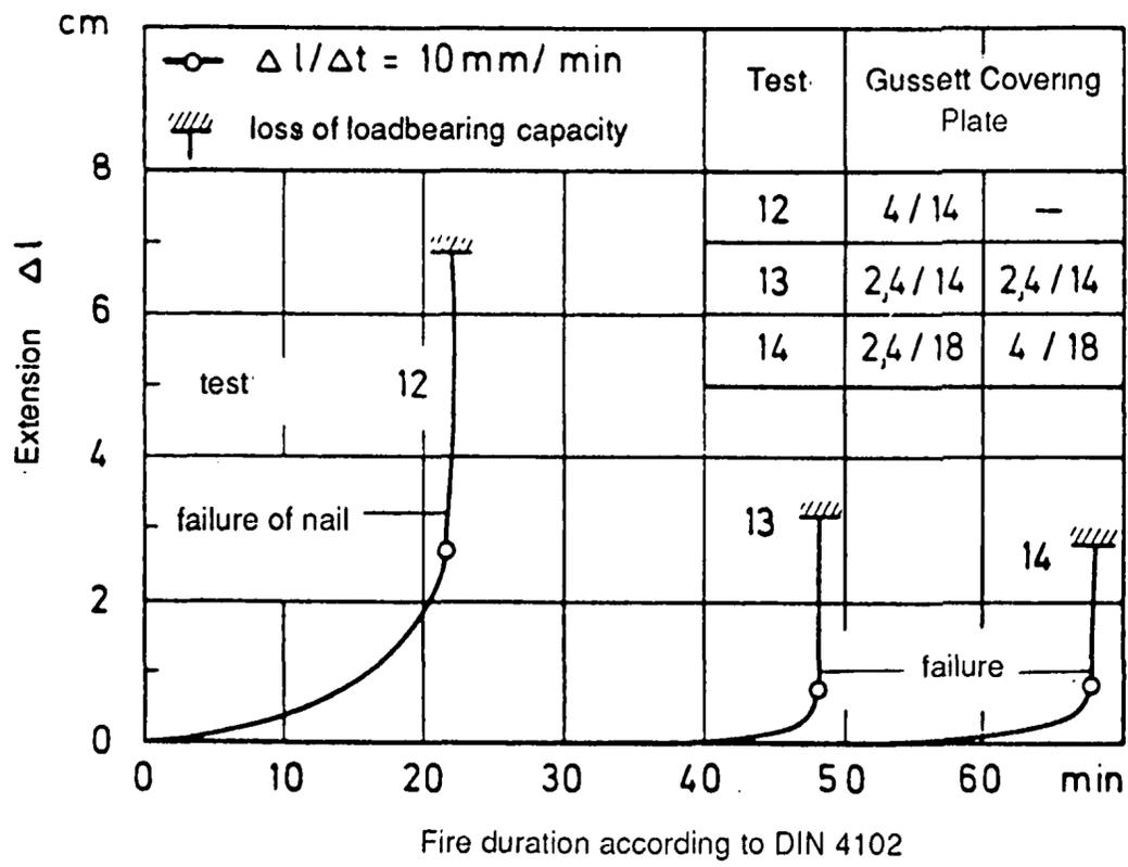
Figure 4.23: Deformations of joints shown in Figure 4.22 in the fire tests [4.14].
