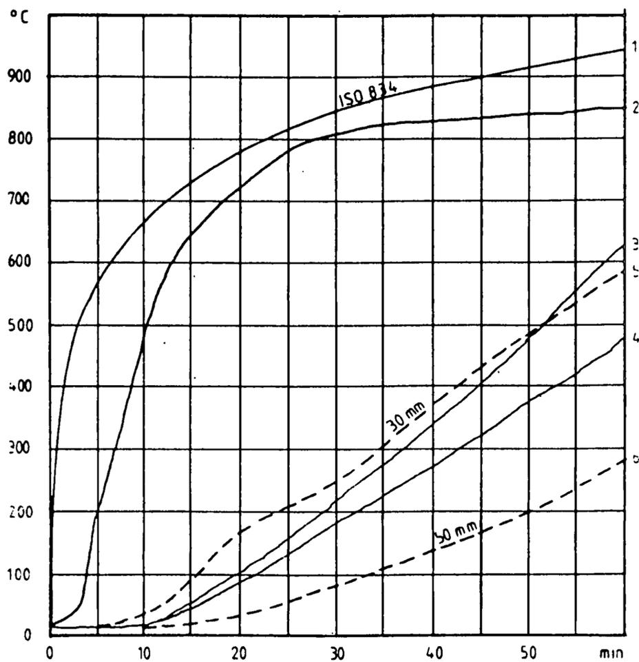
Figure 7.6: Temperature development in steel gusset without (curve 2) and with (curves 3 and 4) the mineral wool insulation as shown in Figure 7.5 [7.9]. Similar characteristics with mineral wool insulation are shown in Figure 7.7 (curves 5 and 6).
