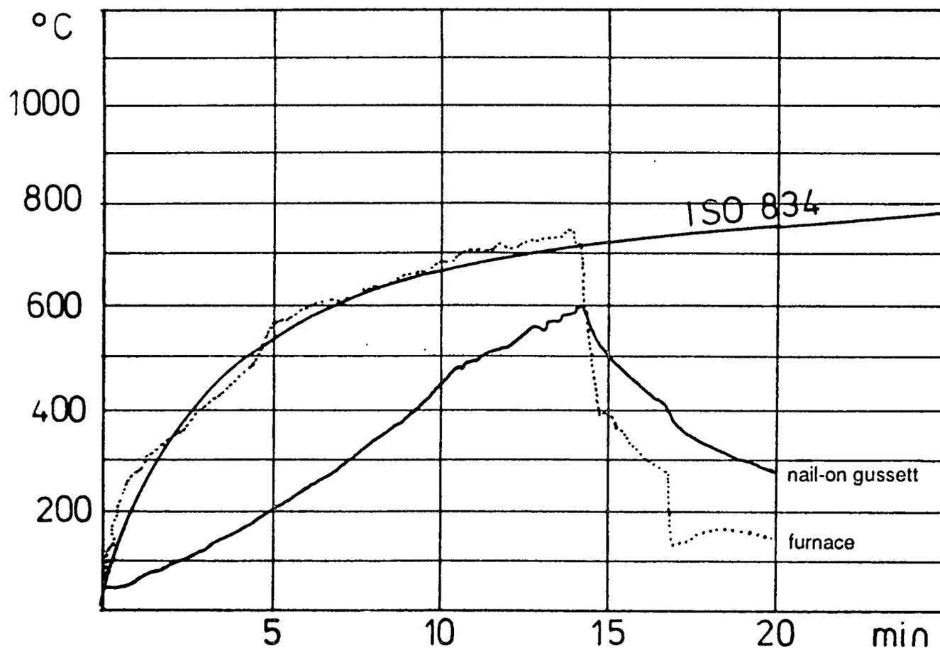
Figure 4.9: Temperature development in nail-on gussets as shown in Figure 4.8 [4.9].
