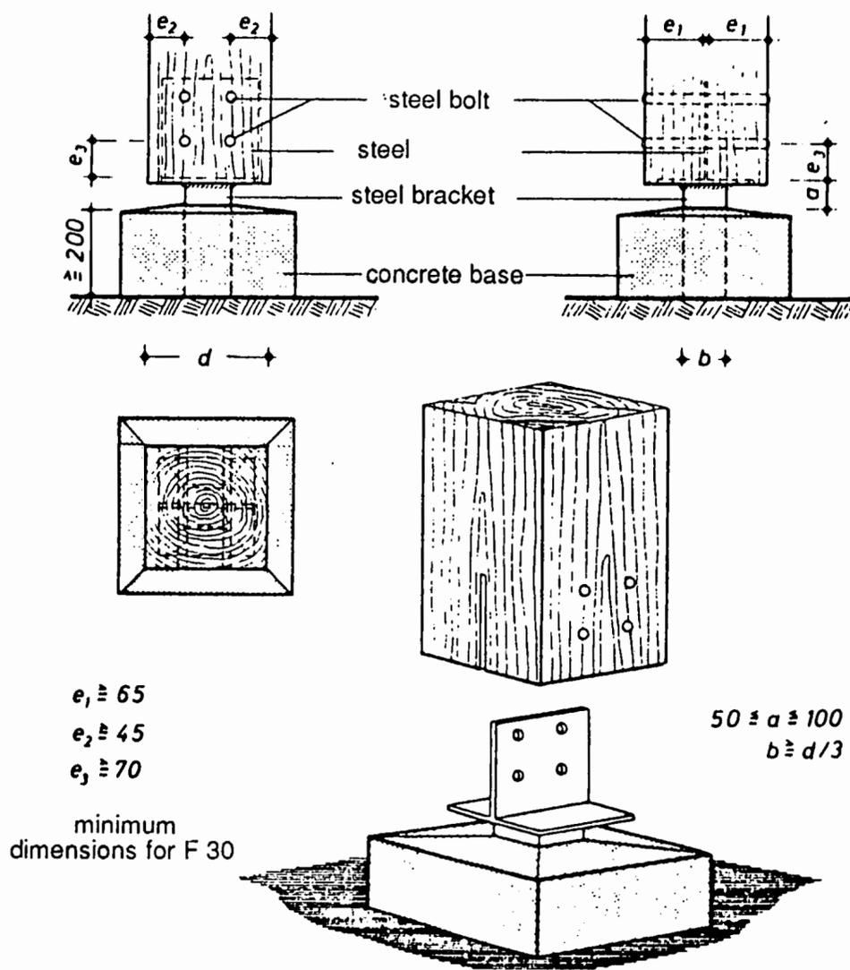
Figure 8.2: Column base for exterior use [8.1] in Fire Class F30.
