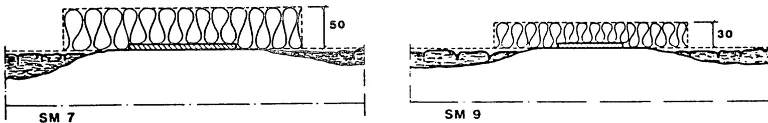
**Figure 7.8:** Sections through the mineral wool insulated plates as shown in Figure 7.7 after 60 minutes of standard fire [7.8].
