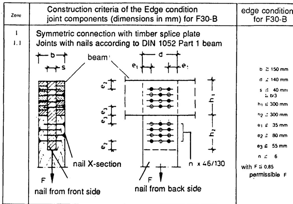
Figure 4.24: Fire tested beam-to-column joints in framework with timber spliced-in plate and double sided nailing [4.14], [4.16].
