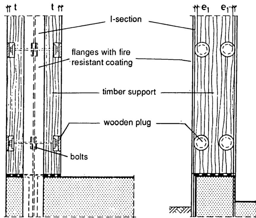
**Figure 8.3:** Fixed column in fire class F30. The flanges of the steel section had been treated with a fire-resistant coating [8.1].
