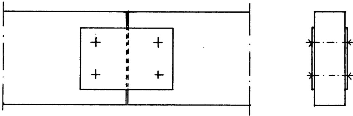
**Figure 9.1:** Fire resistances of a bolted timber joint and the principles for their calculation [9.4], [9.5].
