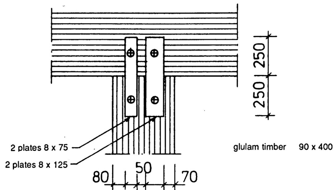
**Figure 4.1:** Fire tested beam-to-column joints with flat plates and bolts [4.1], [4.2]
