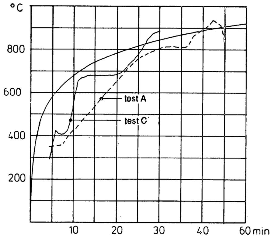
Figure 4.15: Temperature of the bolts 10 mm from the underside of the plate as a function of time [4.5].
