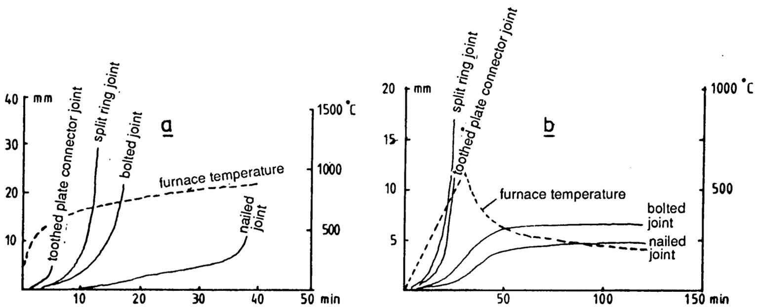
Figure 4.14: Deformation of timber joints under tension, as shown in Figure 4.13, in fire tests
