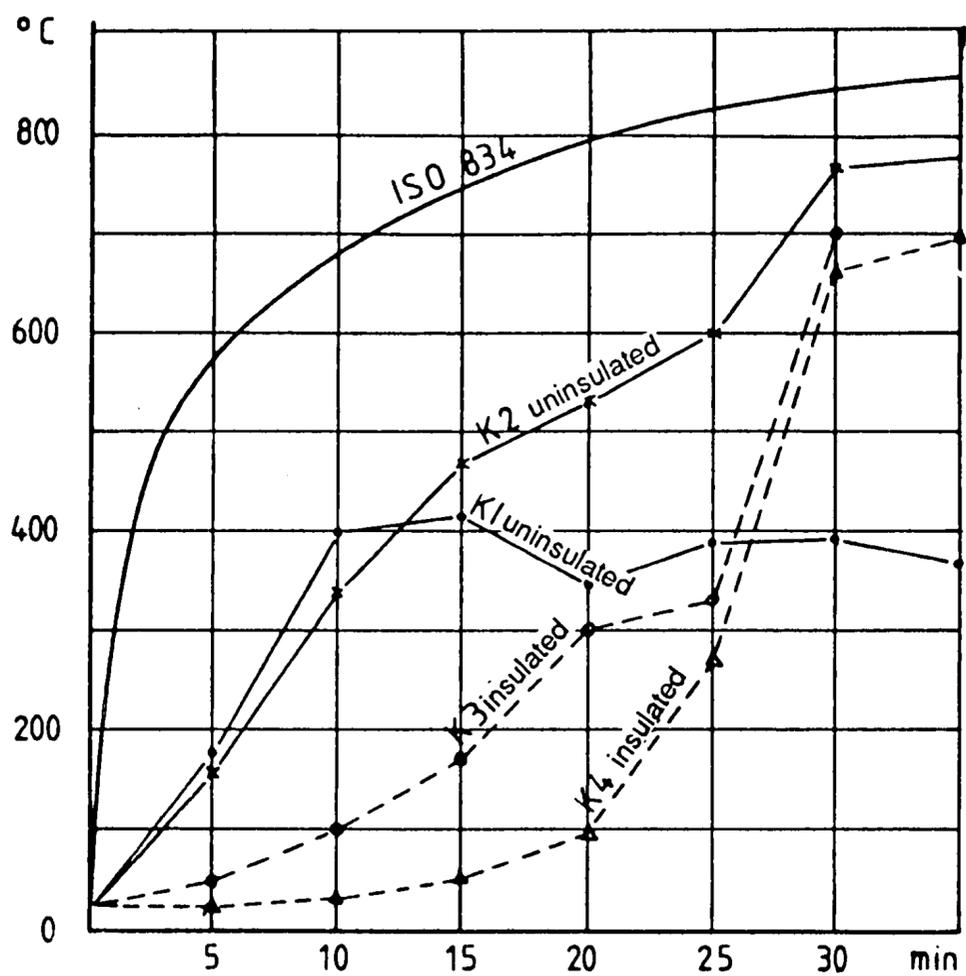
Figure 8.16: Temperatures at contact surface between secondary beam and support bracket in Figures 8.14 and 8.15 [8.3].
