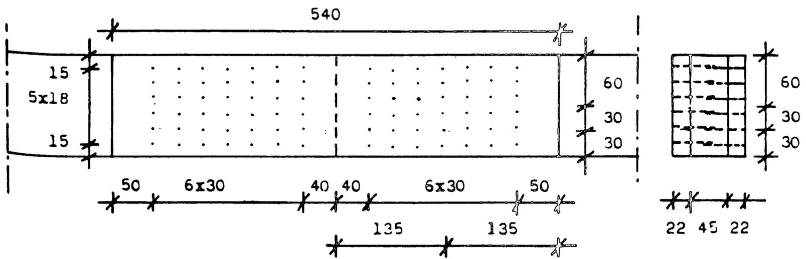
Figure 4.20: Fire tested timber joint with nailed timber gussets [4.13].
