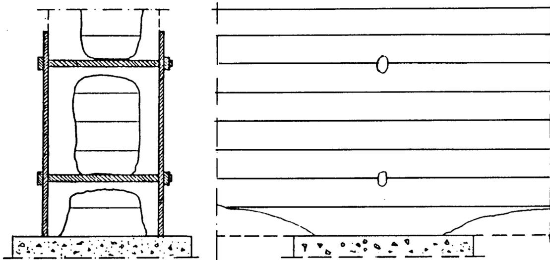
Figure 5.2: Fire tested beam-to-column joint in Figure 5.1a. Vertical sections across and along the beam after 60 minutes of standard fire.
