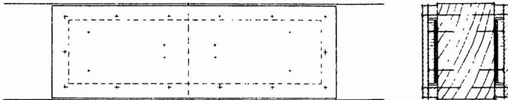
**Figure 7.10:** Fire tested timber joints with plywood protected nail-on gussets [7.10].
