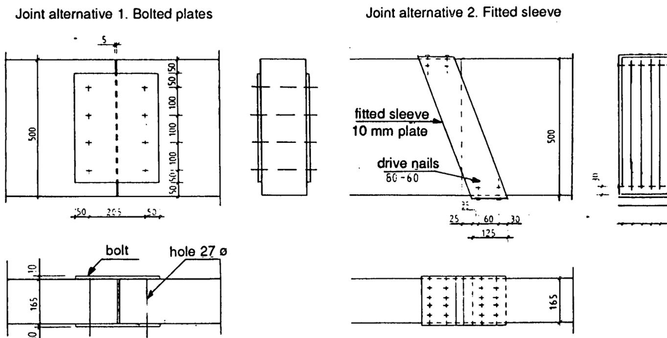
**Figure 4.4:** Fire tested beam joints with bolted plates (alternative 1) and fitted sleeve (alternative 2). Two load levels were investigated, which corresponded to 65% and 100% respectively of the permissible load [4.5].
