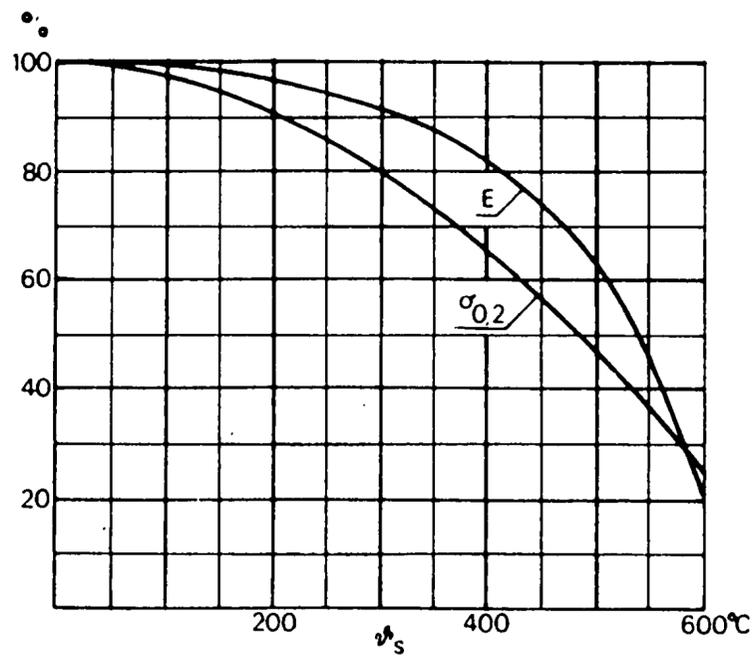
**Figure 1.1:** 0.2-limit and modulus of elasticity as a function of the steel temperature for mild steel [1.1].
