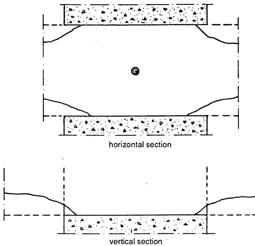
Figure 5.3: Fire tested beam-to-column joint in Figure 5.1b. Horizontal and vertical sections along the beam after 60 minutes of standard fire.
