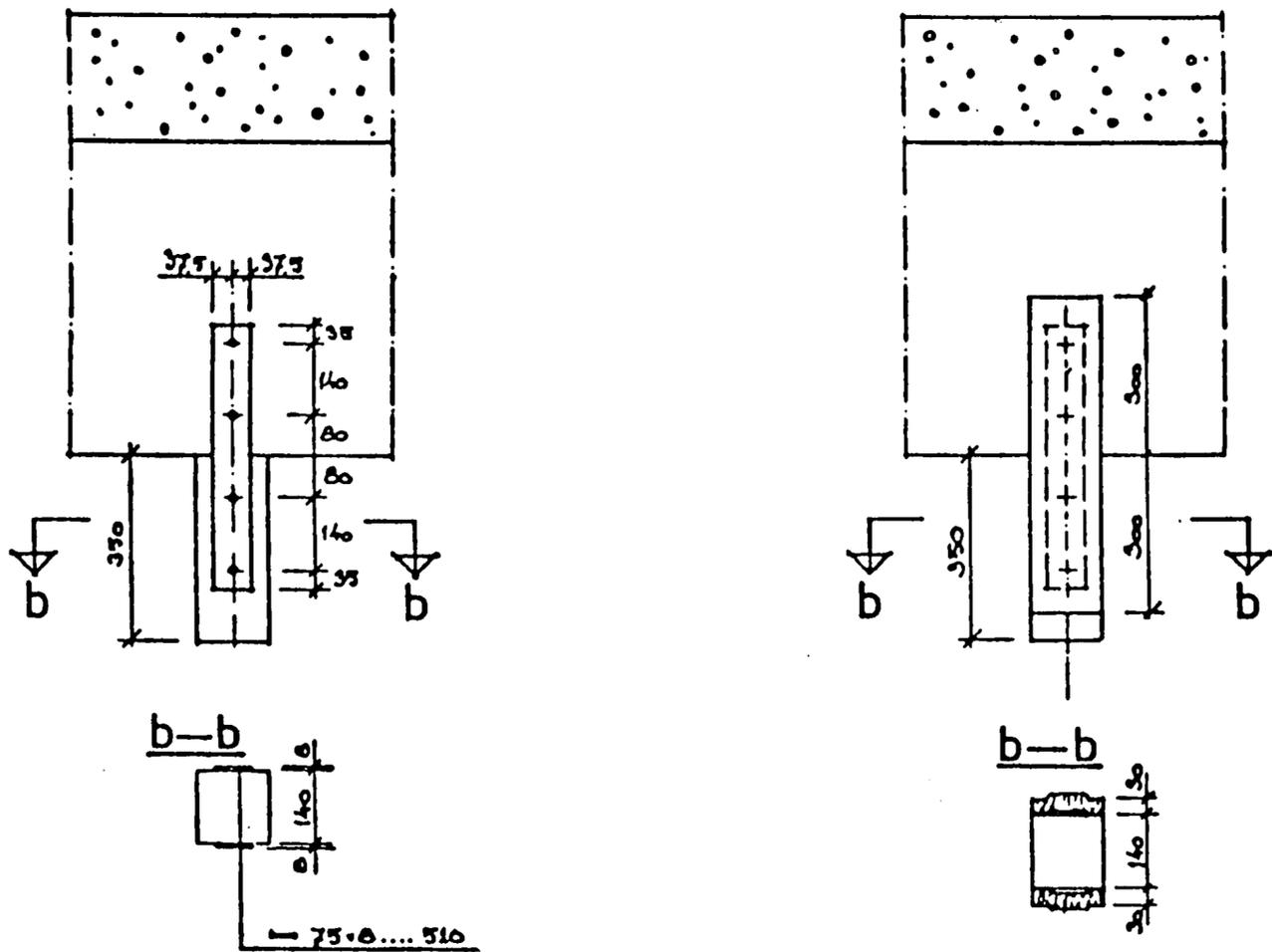
Figure 7.5: Fire tested beam-to-column joints of steel gussets and screws with or without mineral wool insulation.
