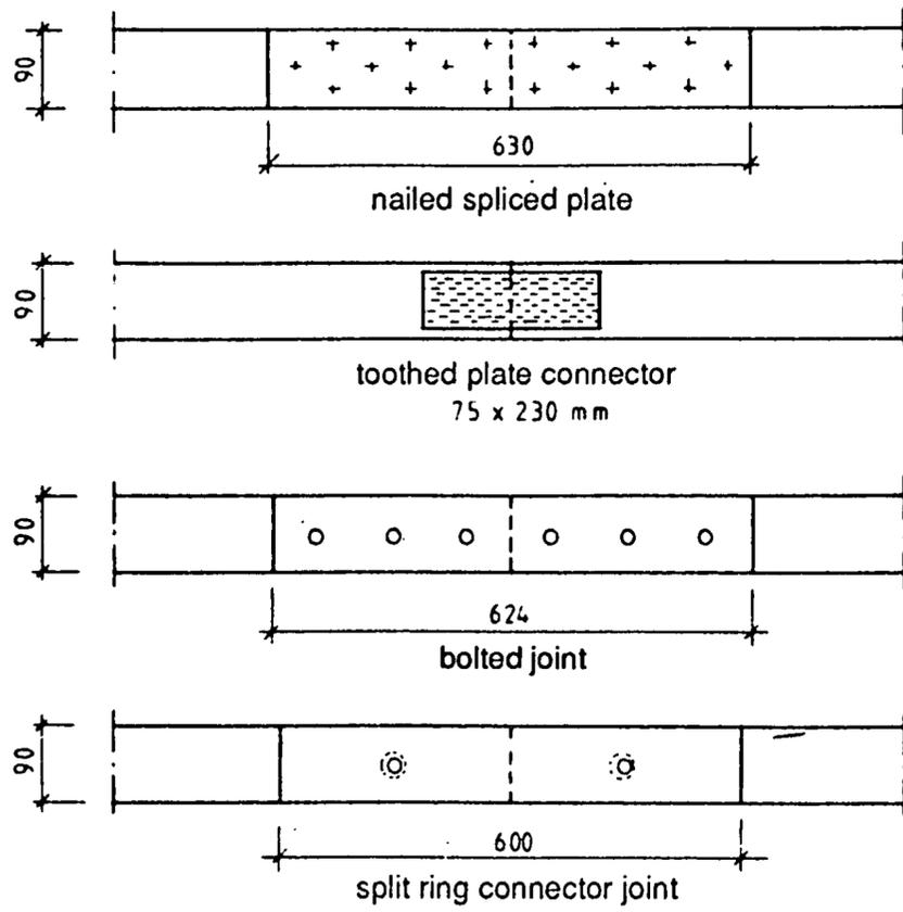
Figure 4.13: Timber joint samples under tension in Australian fire tests [4.12].
