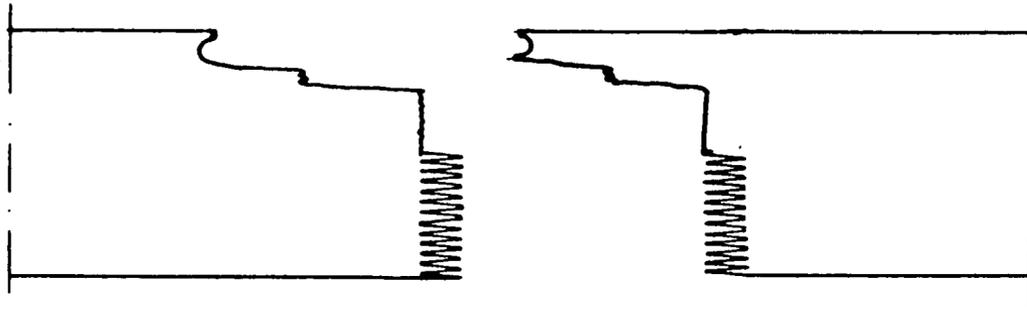
**Figure 6.1:** Typical failure of a finger joint which was a combination of fracture at the base of the fingers, the side of the fingers, adjoining knot or other natural defects in the timber.
