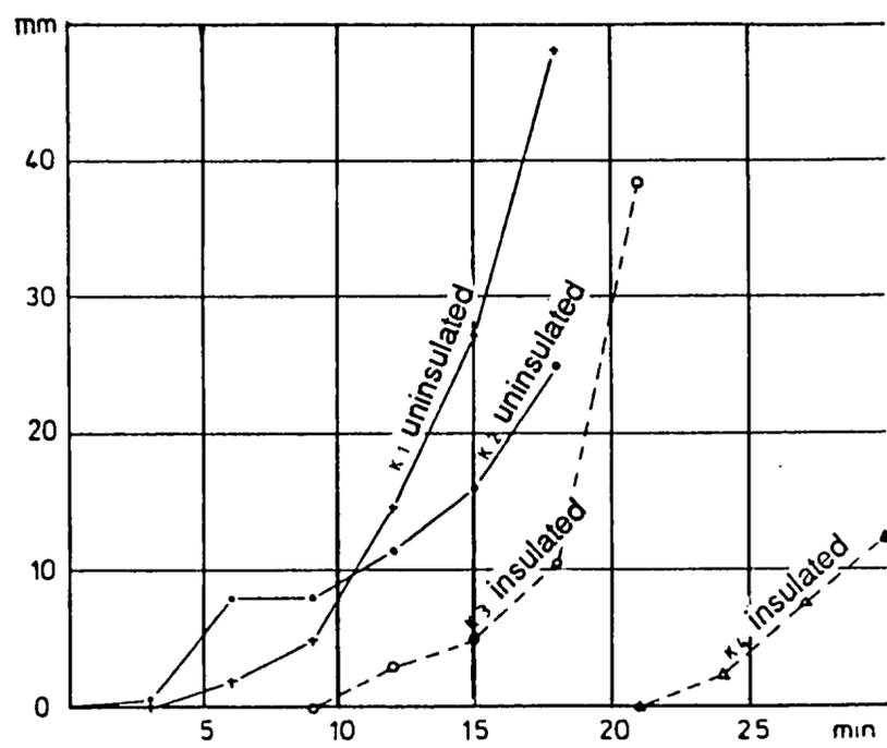
Figure 8.17: Downward displacement of secondary beam relative to primary beam in fire tests of support brackets in Figures 8.14 and 8.15 [8.3].
