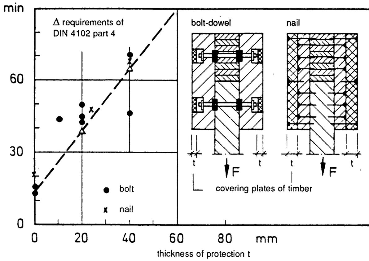
Figure 7.13: Experimental results of the relationship between fire resistance and thickness of the wooden plug or timber protection [7.5].
