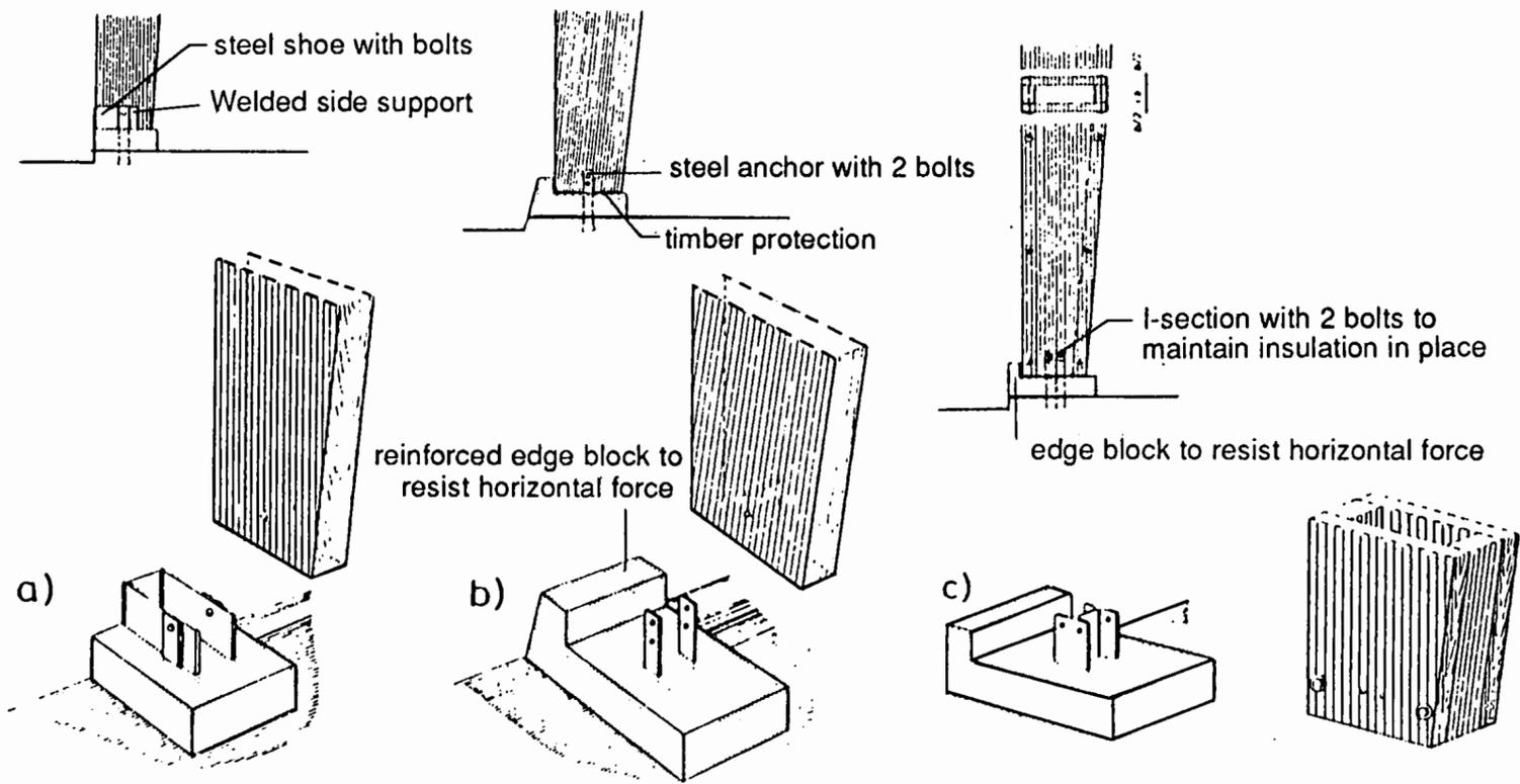
Figure 8.1: Hinged column bases, where the loads are transferred through bearing [8.1], present no problem even when high fire resistance is required.
