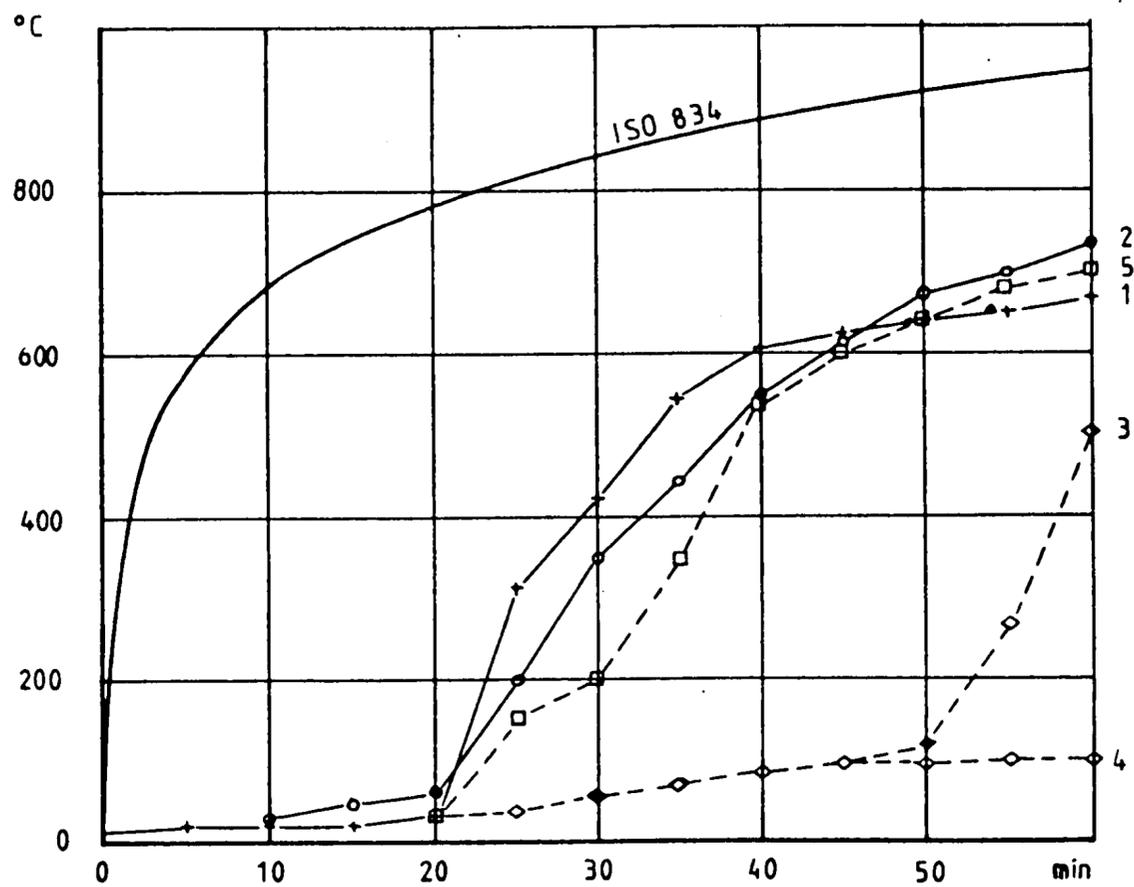
Figure 8.6: Temperature of the screw (curve 1) and at the bearing surface (curve 2) in the fire test of beam-to-column joint as shown in Figure 8.5. Temperature at the interface between the timber gusset and the side of the beam (curves 3 and 4) and the bearing surface (curve 5) in the fire test of beam-to-column joints as shown in Figure 8.7 [8.3].
