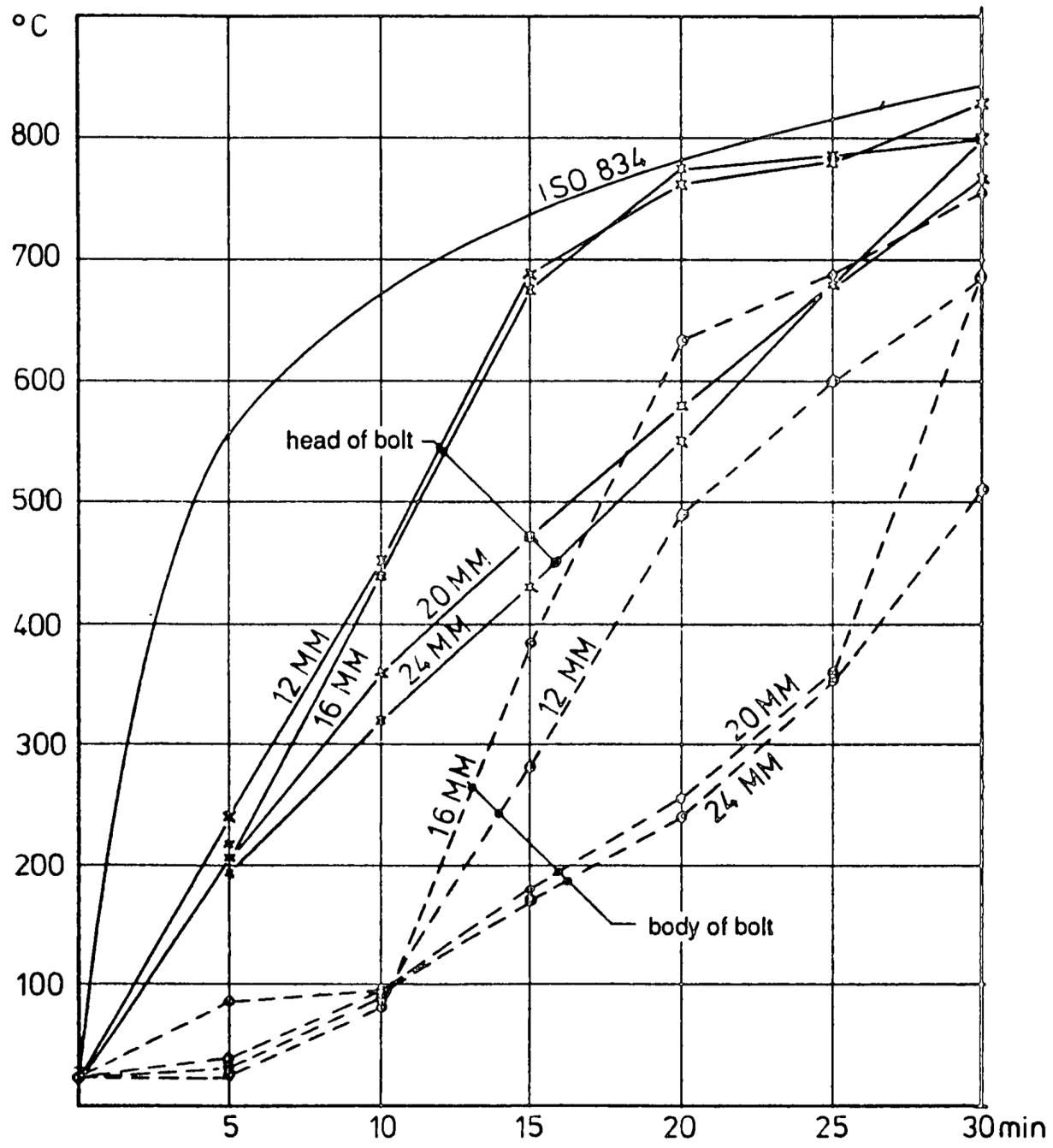
Figure 4.19: Temperature development in bolts of different diameters [4.1] [4.2].
