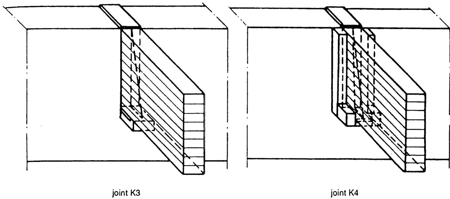
Figure 8.15: Fire tested alternative protections for fitting (type K2) of joints with secondary beams [8.4].
