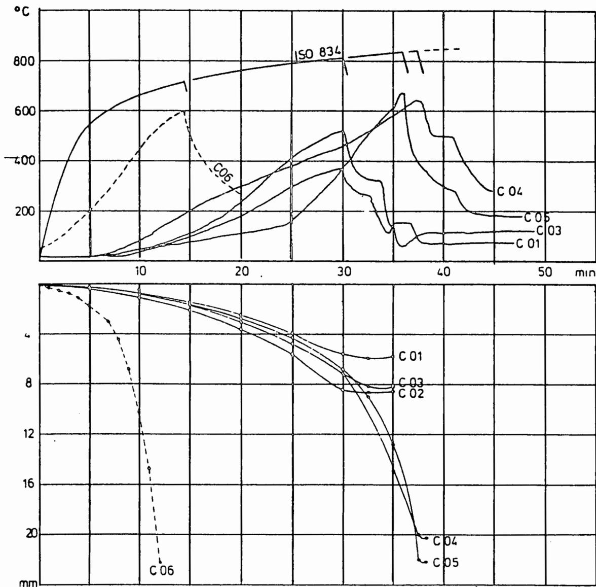
**Figure 7.11:** The temperature and deformation characteristics of the fire tested timber joint with plywood protected nail-on gussets as shown in Figure 7.10 [7.10].
