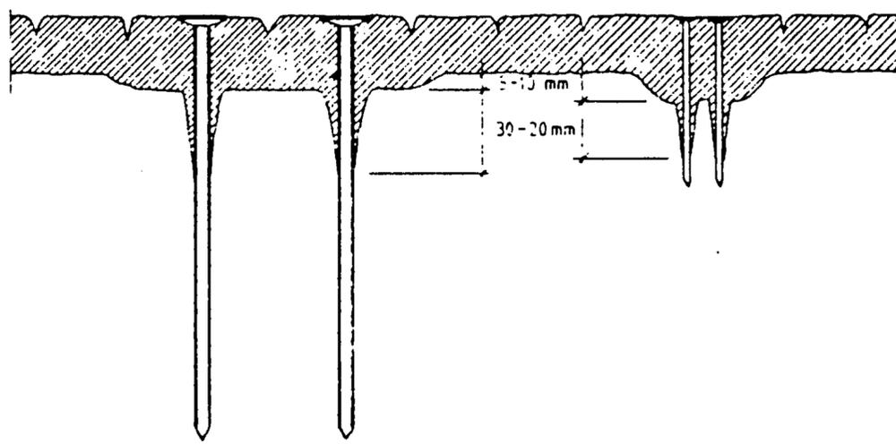
Figure 4.21: Schematic diagram of the penetration of the charred zone in the vicinity of large and small nails respectively [4.1], [4.2].
