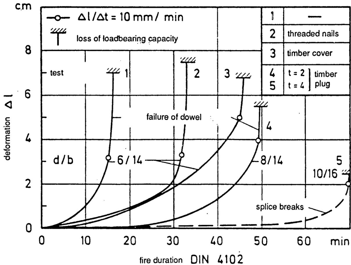
Figure 4.17: Deformation of bolted joints in Figure 4.16 during fire tests [4.14].
