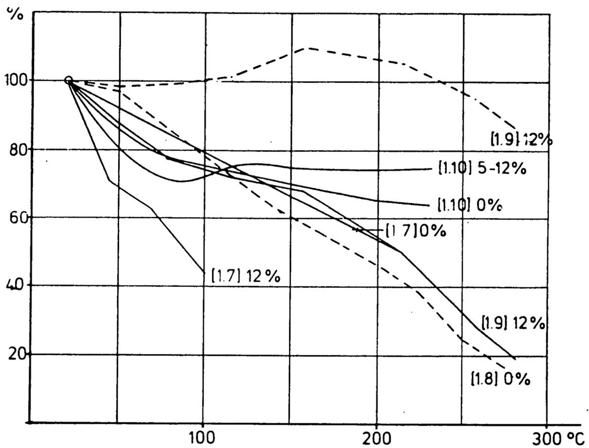
**Figure 1.2:** Relative compressive strength parallel to the grain direction as a function of temperature for Douglas fir [1.8], [1.9], spruce [1.7], [1.10] and pine [1.10].
