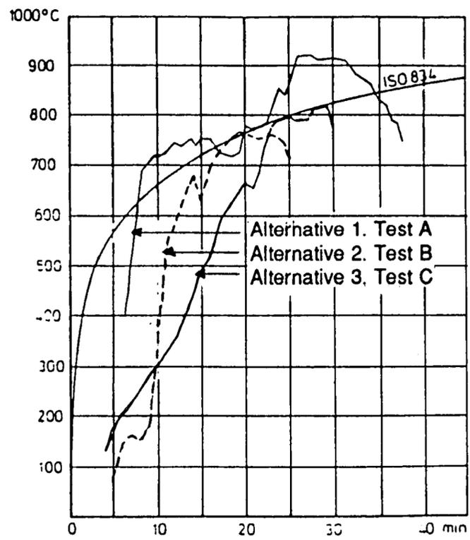
**Figure 4.5:** Temperature at the contact surfaces between glulam timber beam and the joint plates and side surfaces respectively as a function of time [4.5].
