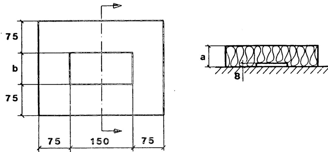
**Figure 7.7:** Test samples for studying the temperature development during fire in flat steel plate insulated with mineral wool [7.8] where  $a = 30$  or  $50$  mm and  $b = 75$  or  $125$  mm.
