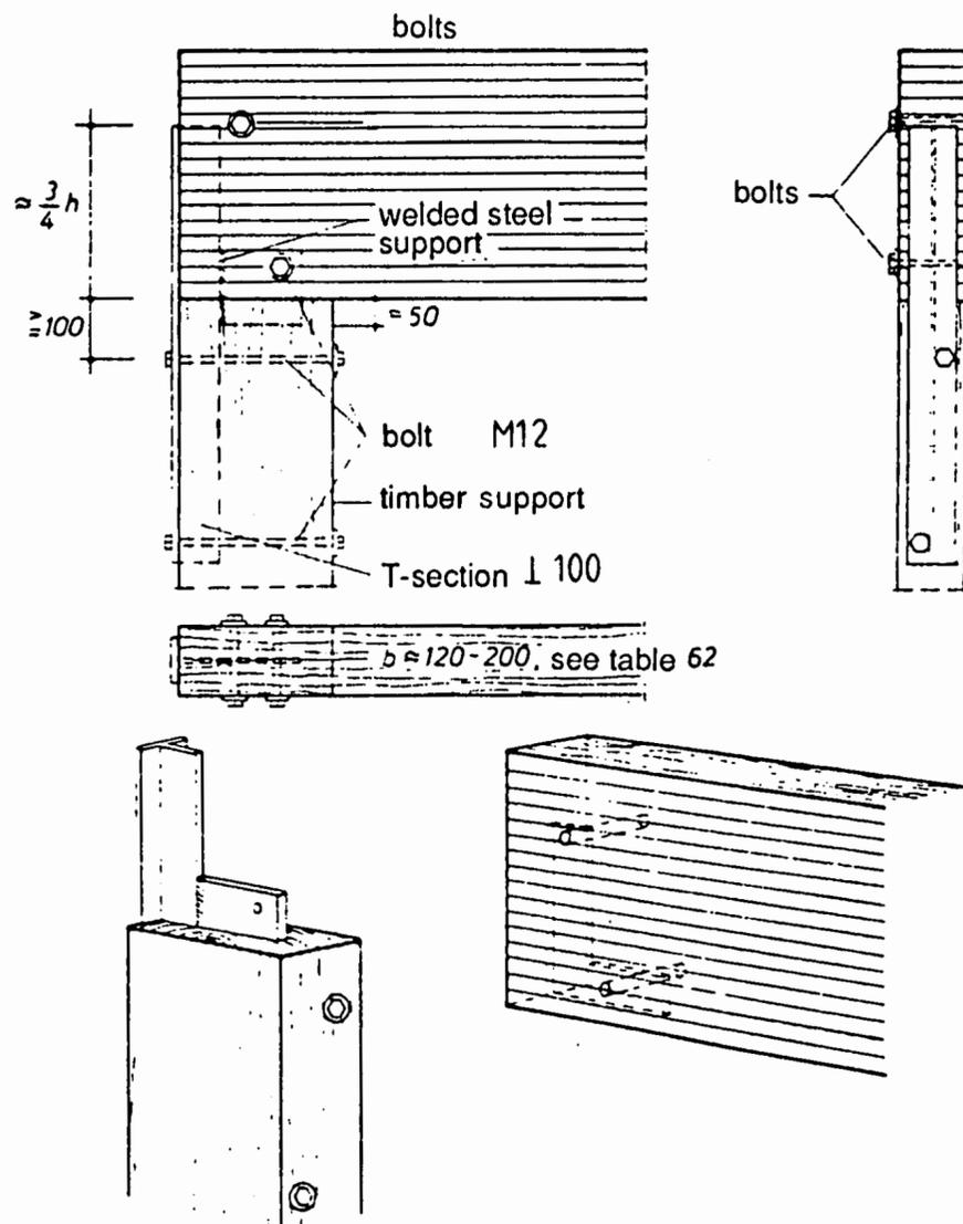
Figure 8.10: Beam-to-column joint with inserted steel T-section and classified according to [8.7] as F30 or F60 depending on the width of the beam. The column can be made of glulam timber or concrete.
