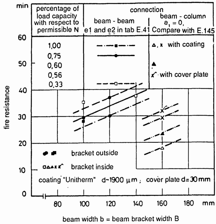
Figure 8.20: Summary of results from fire tests of beam support bracket type BMF [8.2].
