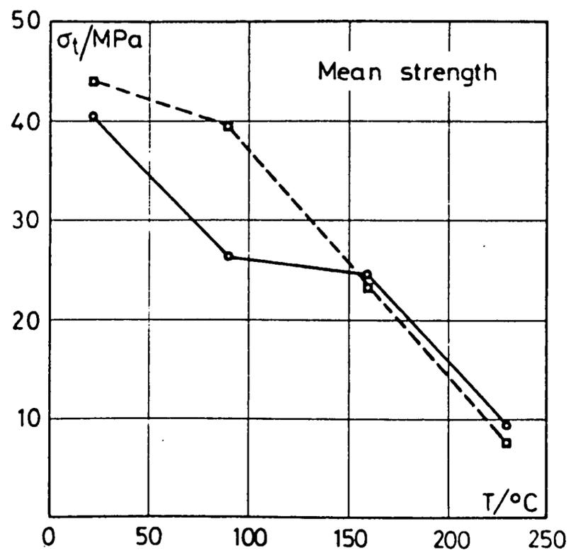
**Figure 6.2:** Experimental strength of timber with (□ ---) and without (o \_\_\_\_ ) finger joints at different temperatures [6.9].
