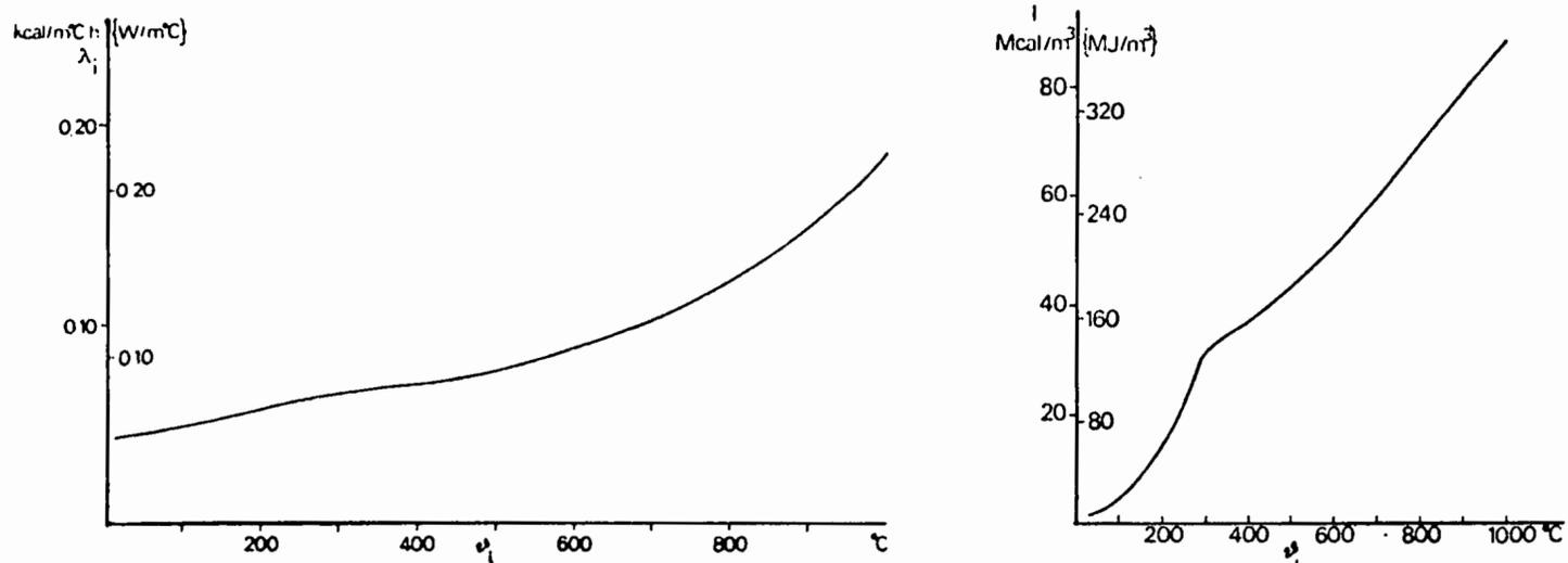
**Figure 7.3:** Conductivity and heat absorption characteristics of sprayed mineral wool of the type "Pyroguard 101" ( $T = 250 \text{ kg/m}^3$ ) as a function of the temperature in the insulation layer.
