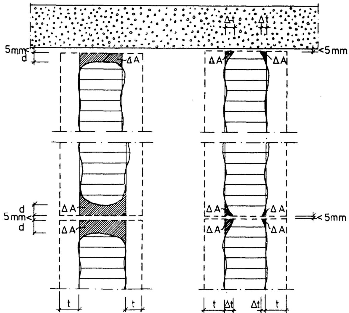
**Figure 3.1:** The effect of the width of a gap, between two glulam timber beams or between a glulam timber beam and a lightweight concrete slab, on the extent of the charred zone in the vicinity of the gap.
