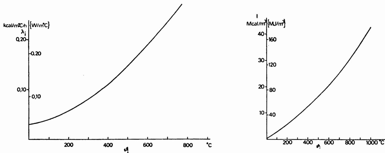
**Figure 7.4:** Conductivity and heat absorption characteristics in mineral wool boards ( $T = 150 \text{ kg/m}^3$ ) as a function of the material temperature [7.1].
