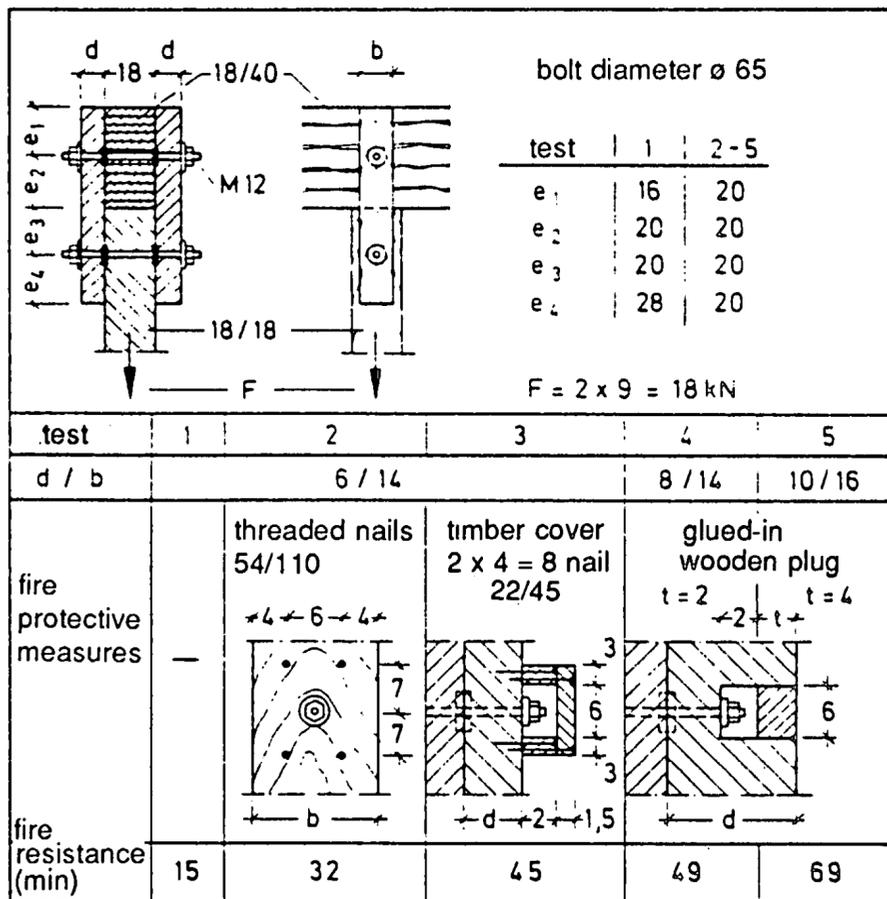
Figure 4.16: Fire tested beam or beam-to-column bolted joints in structural framework. External bolted timber joints with washers [4.14].
