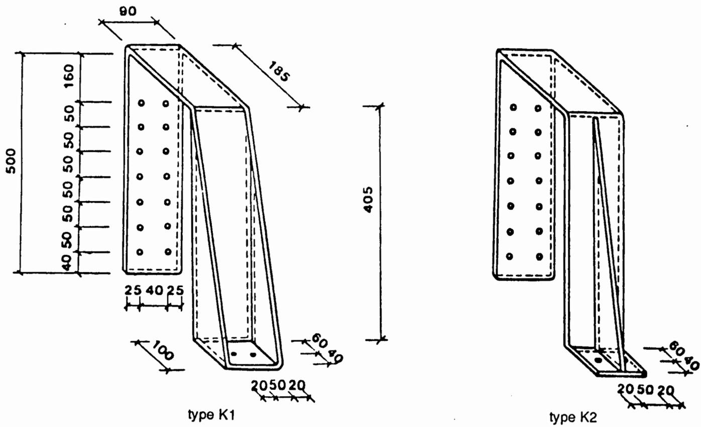
**Figure 8.14:** Fire tested fittings for joints between secondary glulam timber beam and primary glulam timber beam [8.4].
