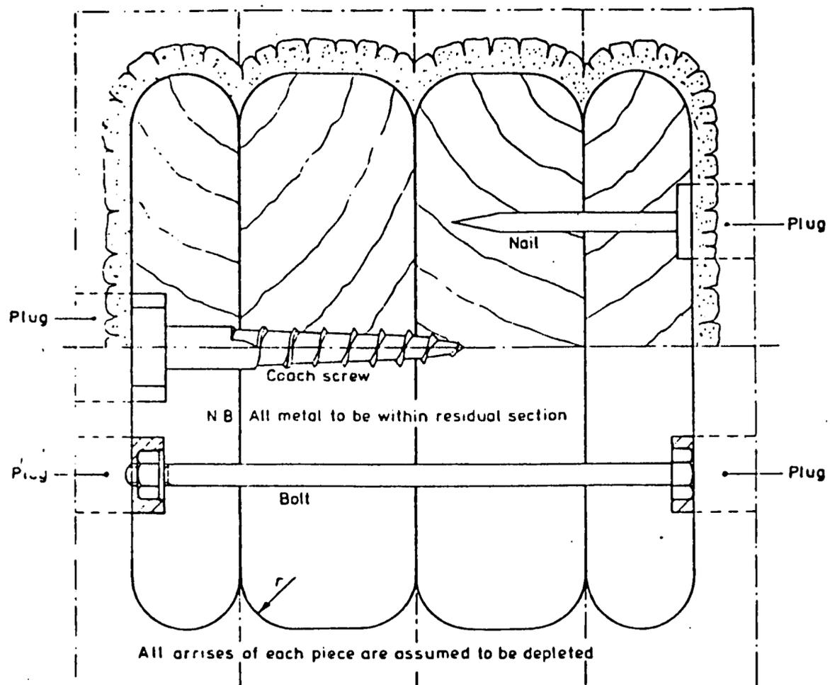
**Figure 10.1:** According to BS 5268, a metal connection should be buried into the timber so that it is completely within the residual section.
