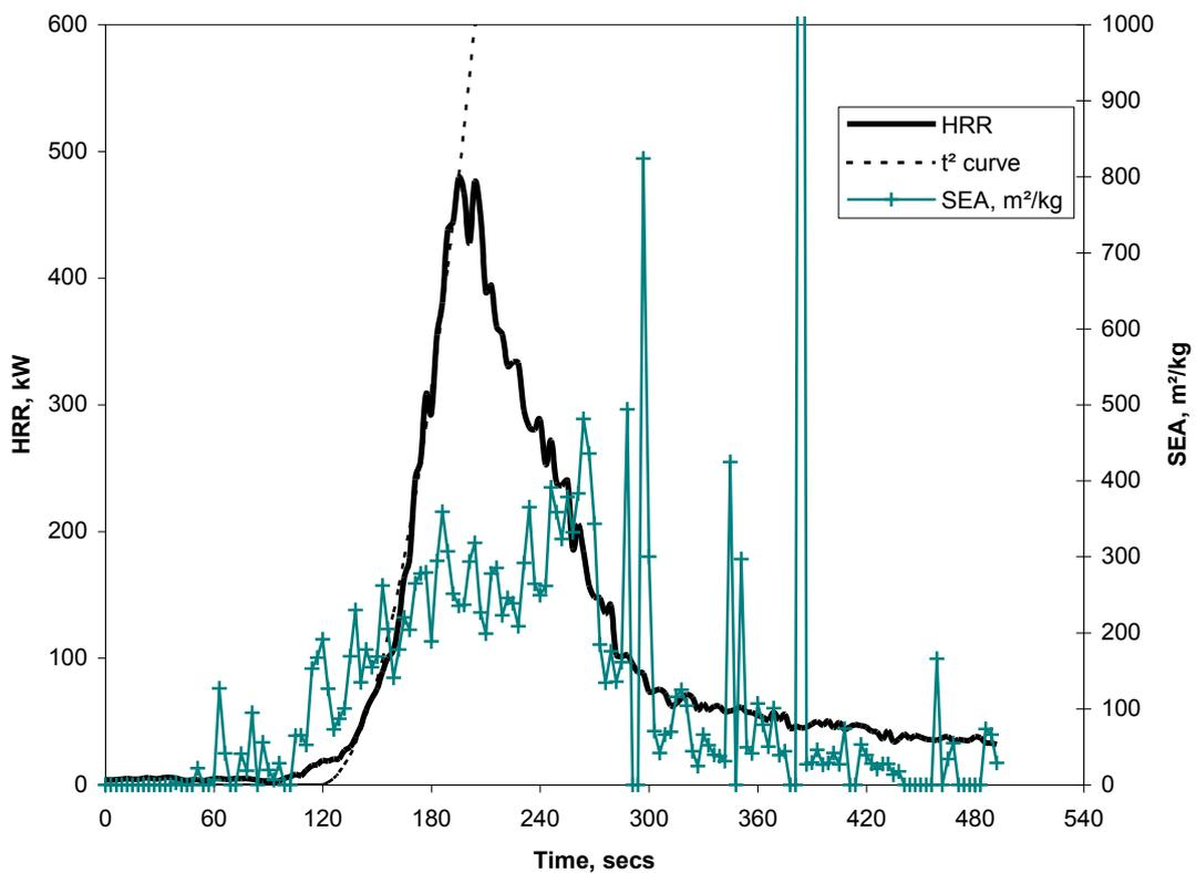
**Figure 27. Comparison of HRR and SEA for purpose-built seat burn with fire starter ignition and incipient fire development time of 135 seconds (30 kW)**
