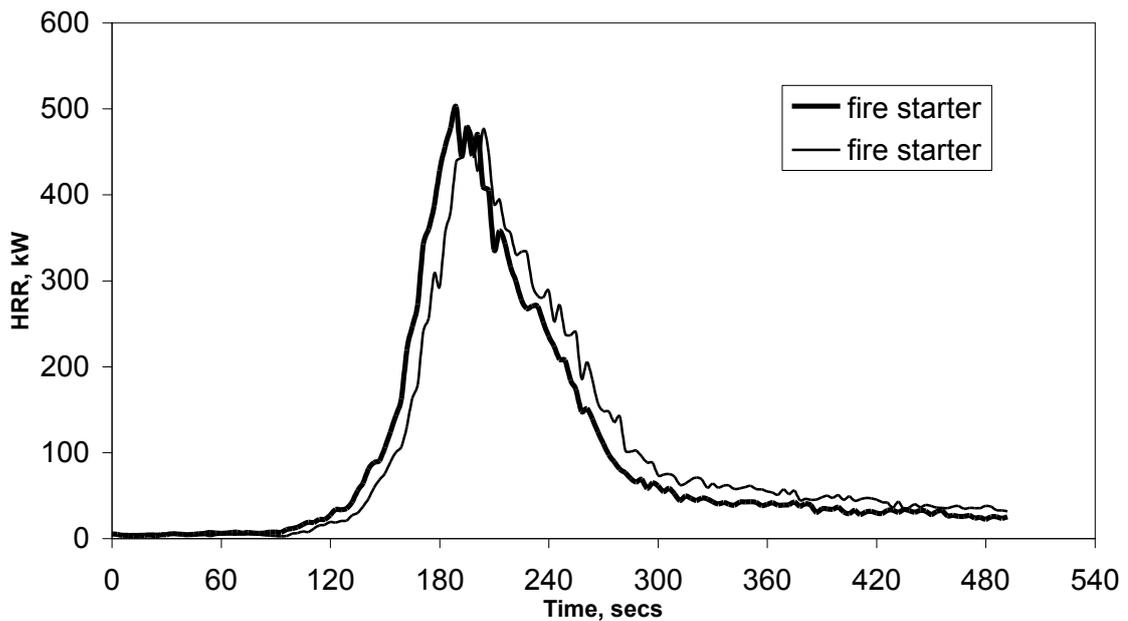
**Figure 16. HRR with ignition source on front edge of seat**
