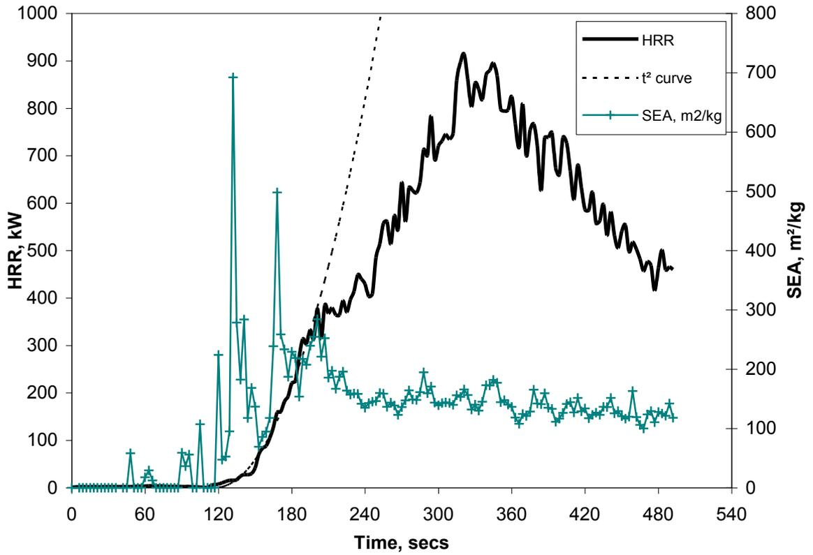
**Figure 28. Comparison of HRR and SEA for sofa burn with match ignition and incipient fire development time of 146.7 seconds (30 kW)**
