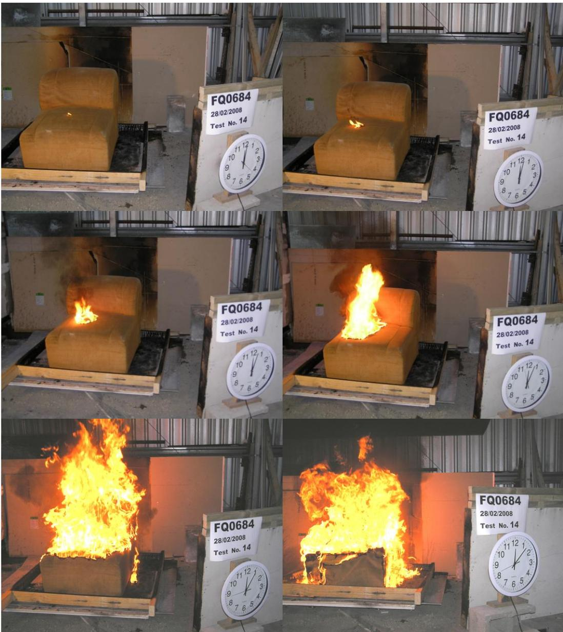
Figure 24. Fire growth with match in centre of sofa seat, 30 kW was exceeded at 172 seconds, fourth photo in sequence
