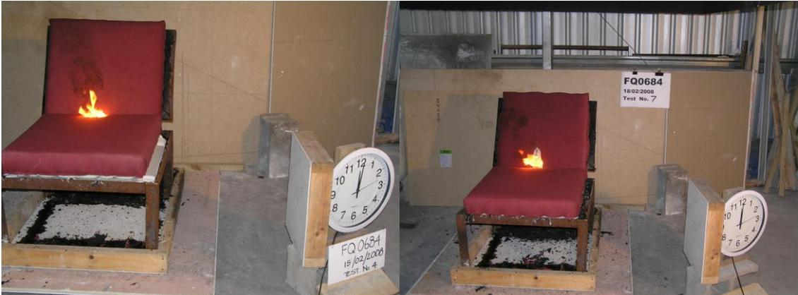
Equivalent flame size after 72 seconds from ignition with match vs 14 seconds from ignition with fire starter
