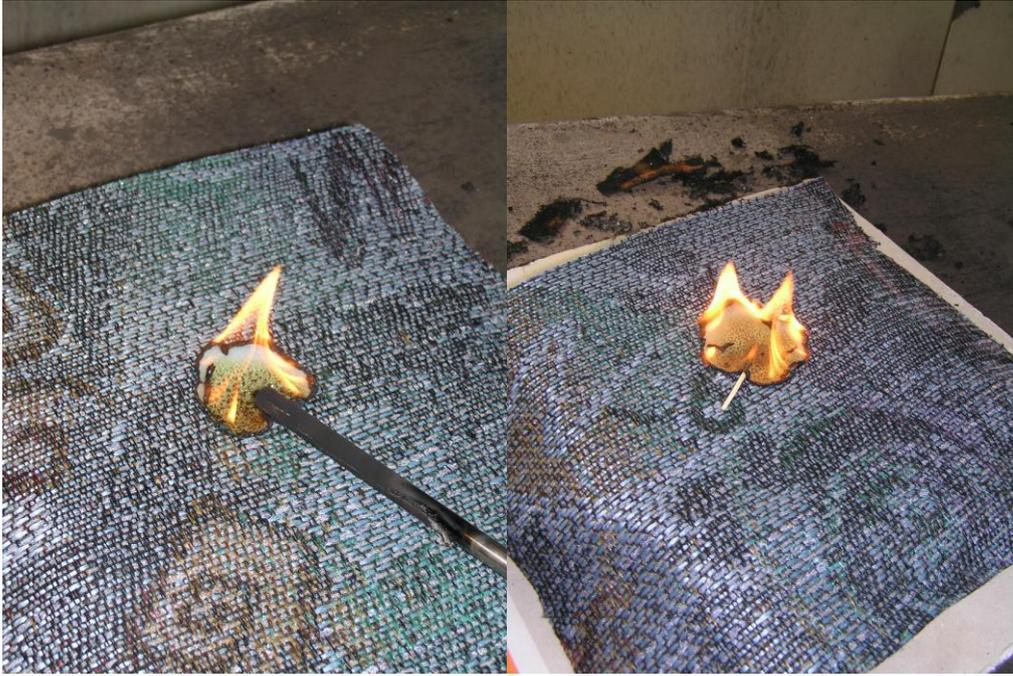
Figure 7. Gas flame and match ignition of olefin-covered PU foam
