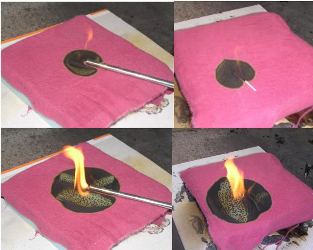
Figure 8. Gas flame and match ignition of cotton fabric-covered PU foam
