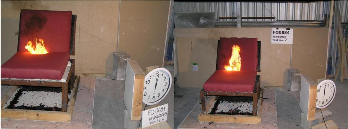
Flame development at approximate  $t_0$  times of 91 and 30 seconds respectively
