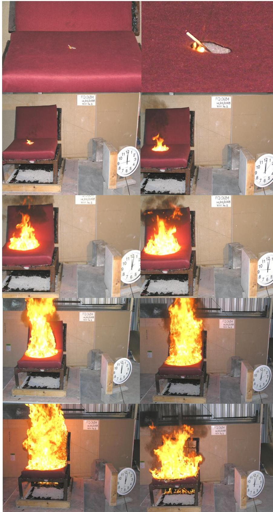
Figure 13. Fire growth with match in centre of seat cushion in Test 3,  $t^2$  rate of fire growth begins after approximately 69 seconds (fourth photo), and 30 kW was exceeded at 102 seconds, between fifth and sixth photos in sequence
