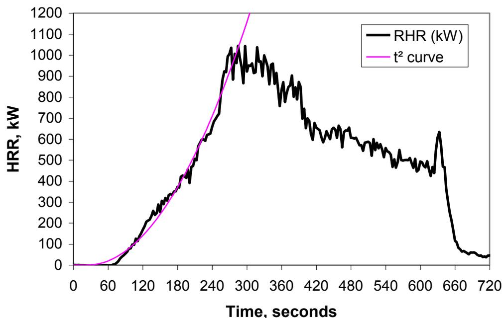
Figure 6. Example of sofa burn with delay time  $t_0$  of 24 seconds to  $t^2$  (medium+)
