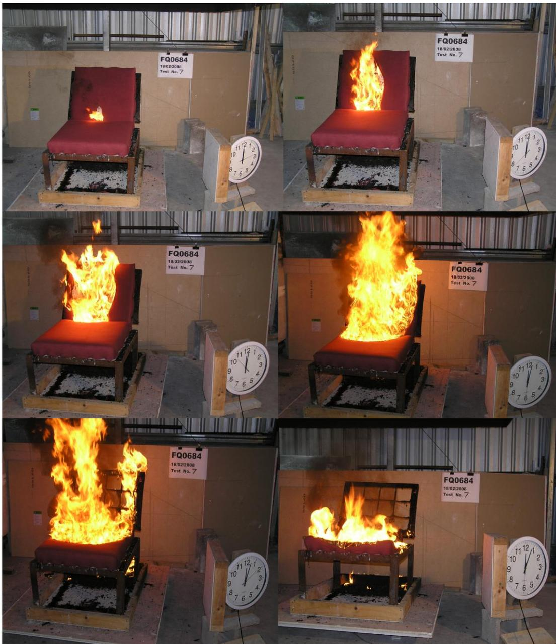
Figure 14. Fire growth with fire lighter at junction of seat base and back in Test 7,  $t^2$  fire growth rate was reached after 26 seconds, and 30 kW was exceeded at 53 seconds, third photo in sequence
