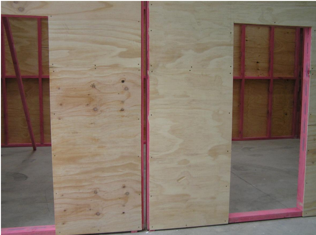
Figure 6. The 20 mm gap separating Chamber 1 from Chamber 2 and Chamber 3 from Chamber 4
