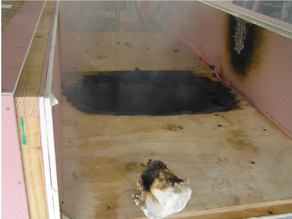
Figure 60. Area of Integrity failure on floor surface in Pilot Fire Test 1
