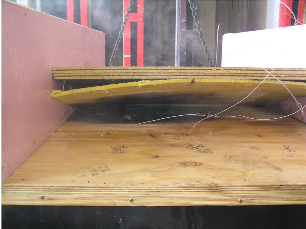
Figure 66. Area of Integrity failure on floor surface in Pilot Fire Test 2
