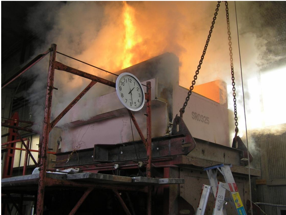
Figure 51. Pilot Fire Test Specimen 1 when fire broke through the floor
