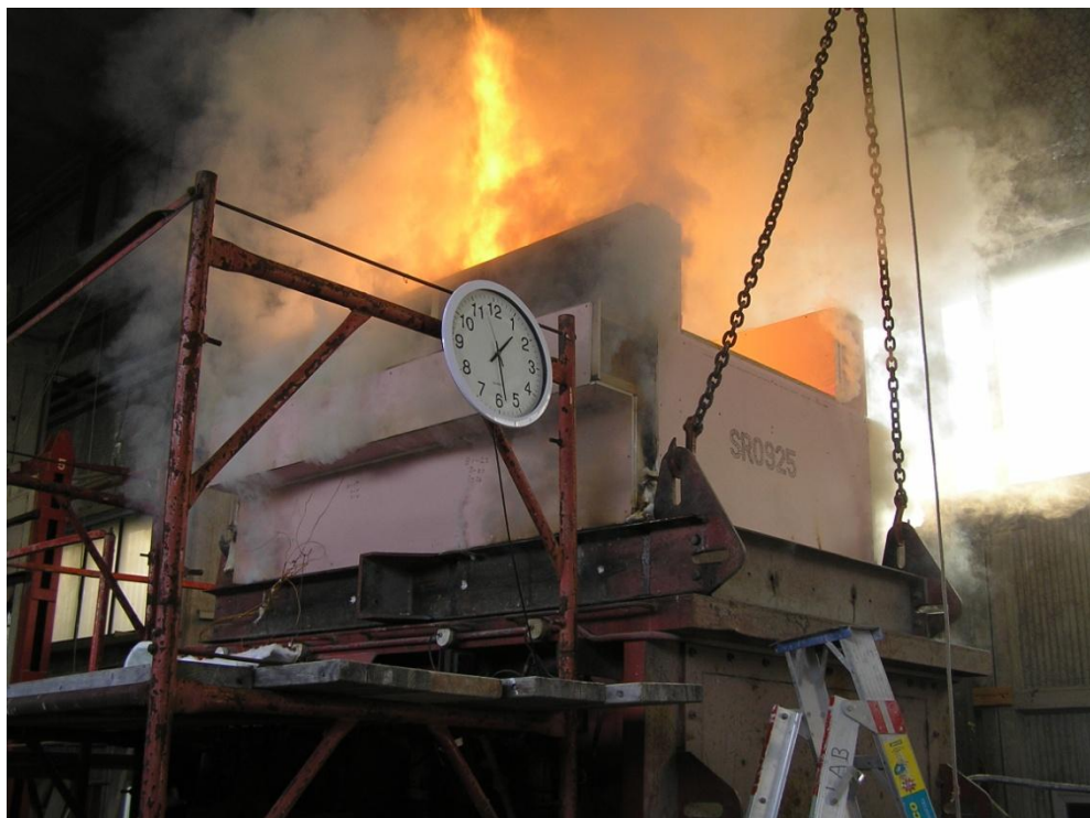
Figure 59. Pilot Fire Test 1 when fire broke through the floor at about 89 minutes
