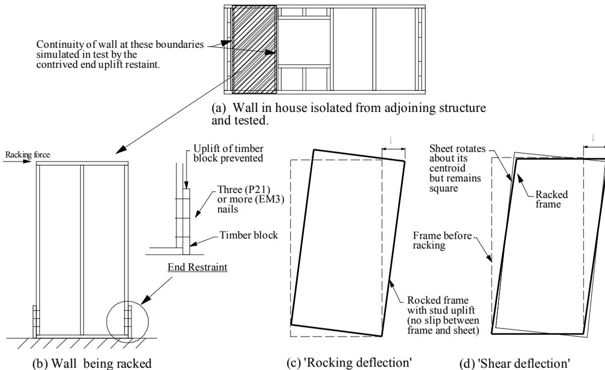
**Figure 4. Components of racking wall deflection and sketch of the BRANZ P21 uplift restraints**
