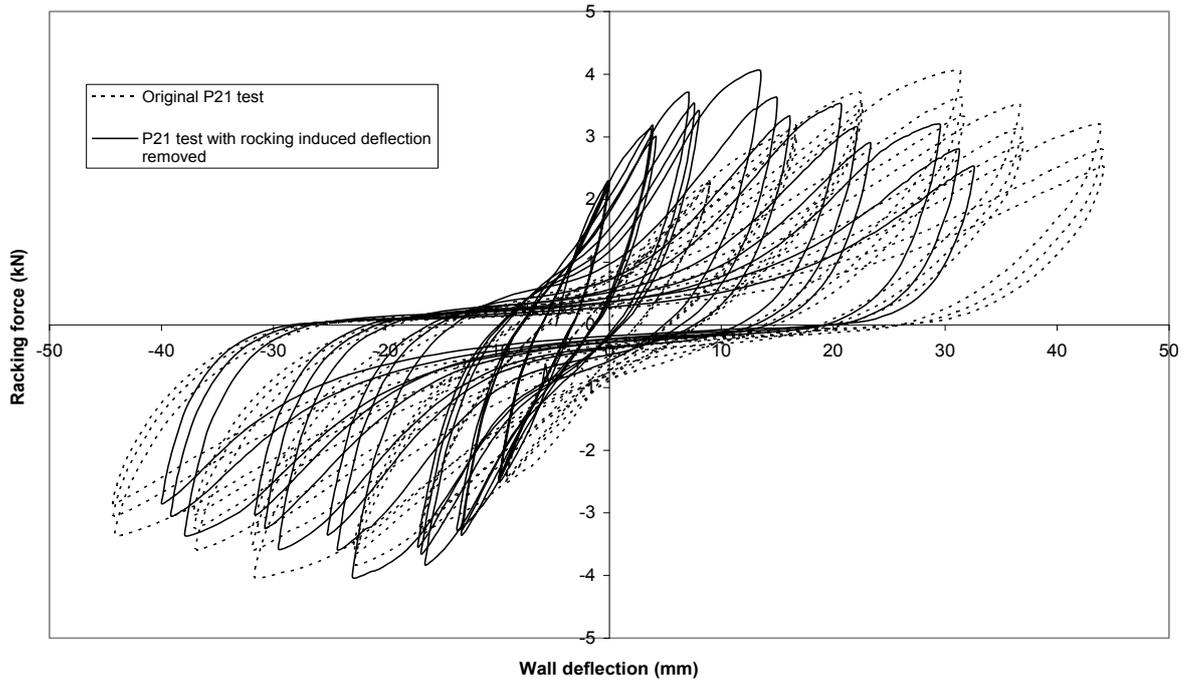
**Figure 31. Wall 1 – 0.6 m long wall lined with plasterboard on one face with end straps**
