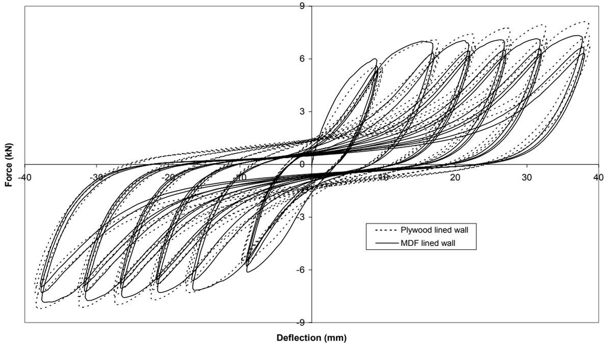
Figure 8. Comparison of test hysteresis loops for MDF and plywood-lined walls
