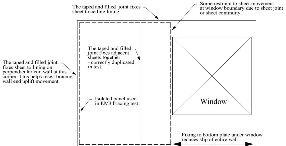
Figure 3. Restraint of wall lining in real buildings
