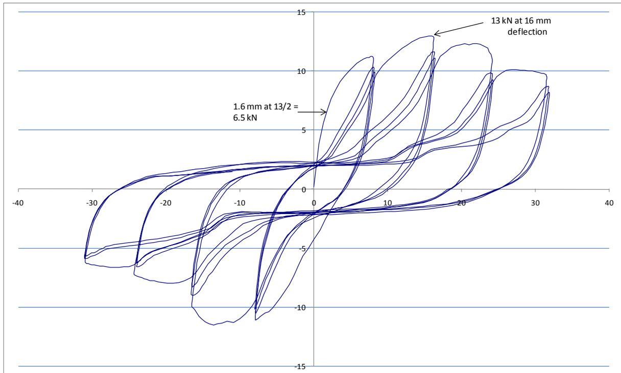
Figure 1. Sample P21 test result giving an apparent ductility of 8.9
