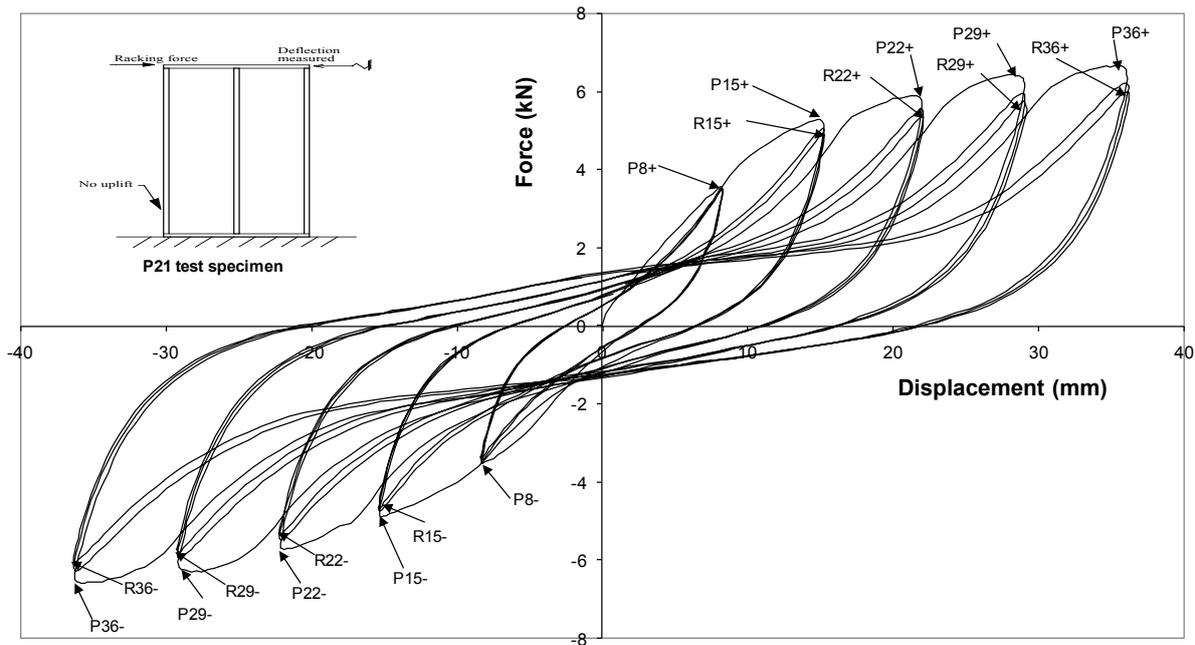
**Figure 2. Hysteresis loops from a typical EM3-V3 test**
