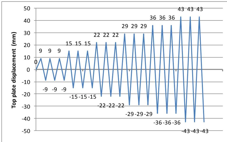
Figure 3. Cyclic load protocol. (example shown for a 2,400 mm high specimen)
