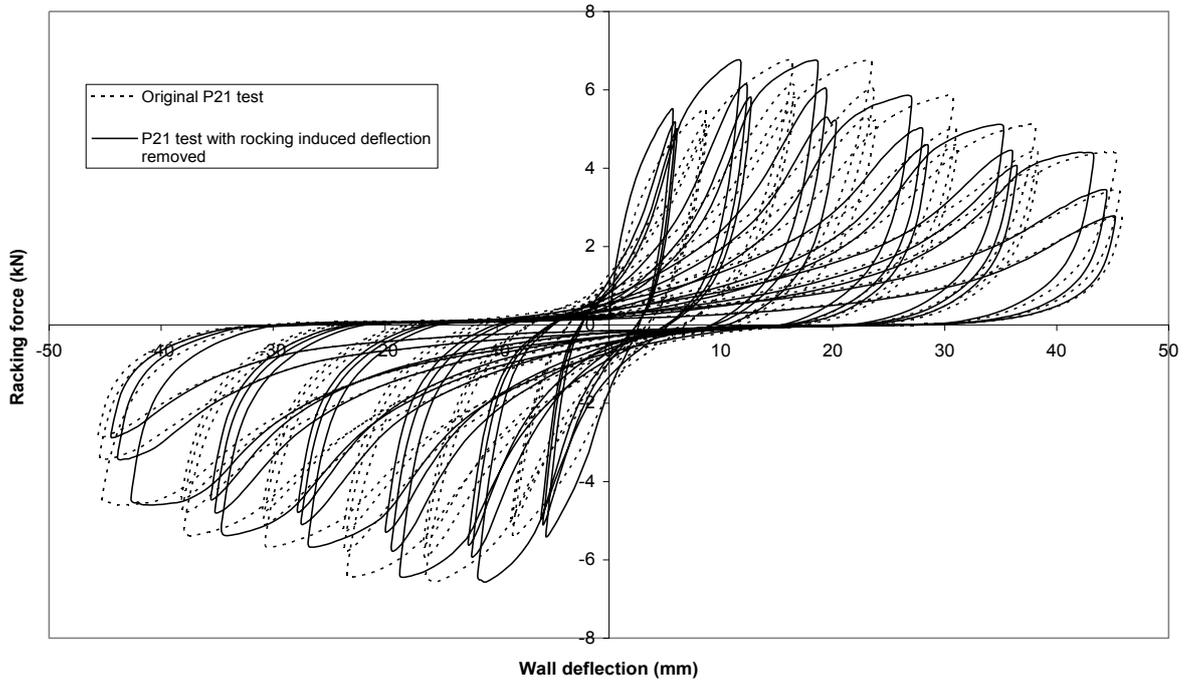
Figure 33. Wall 3 – 1.2 m long wall lined with plasterboard on one face without end straps
