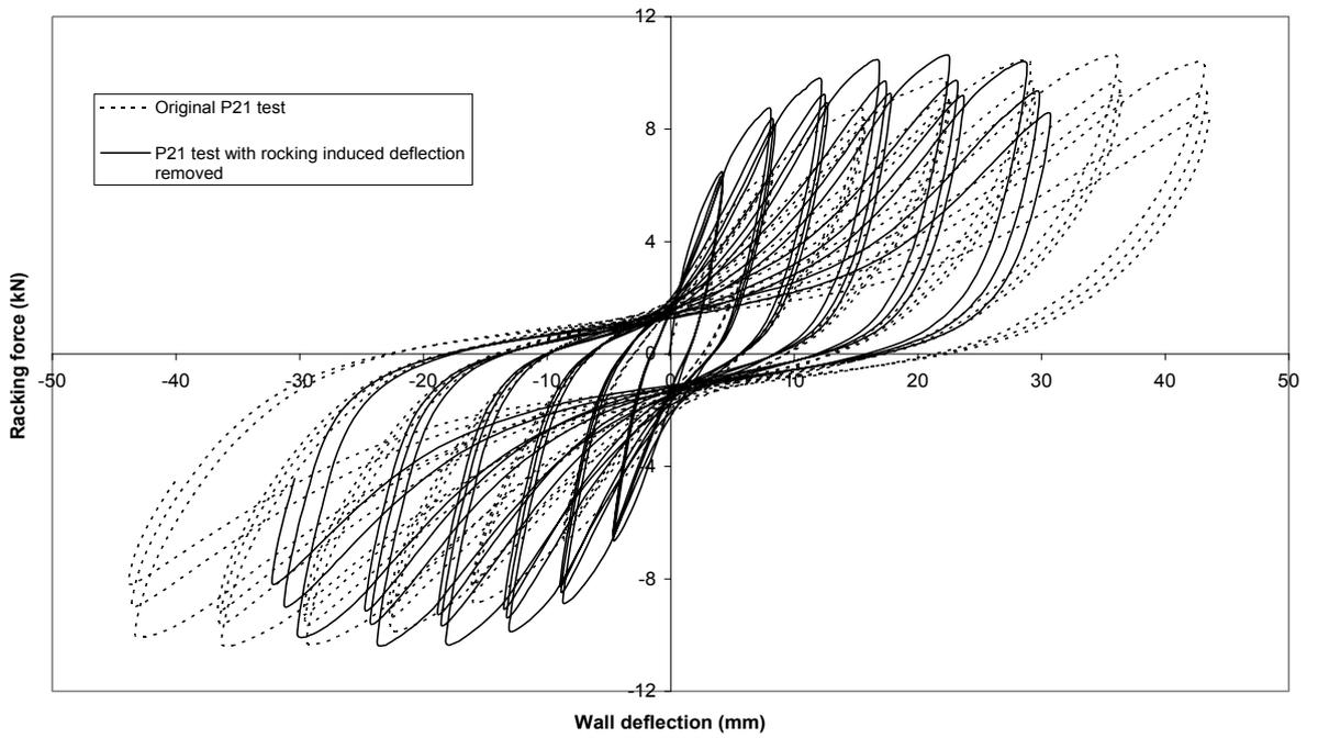
**Figure 39. Wall 9 – 1.2 m long wall lined with fibre-cement sheet on one face with end straps**
