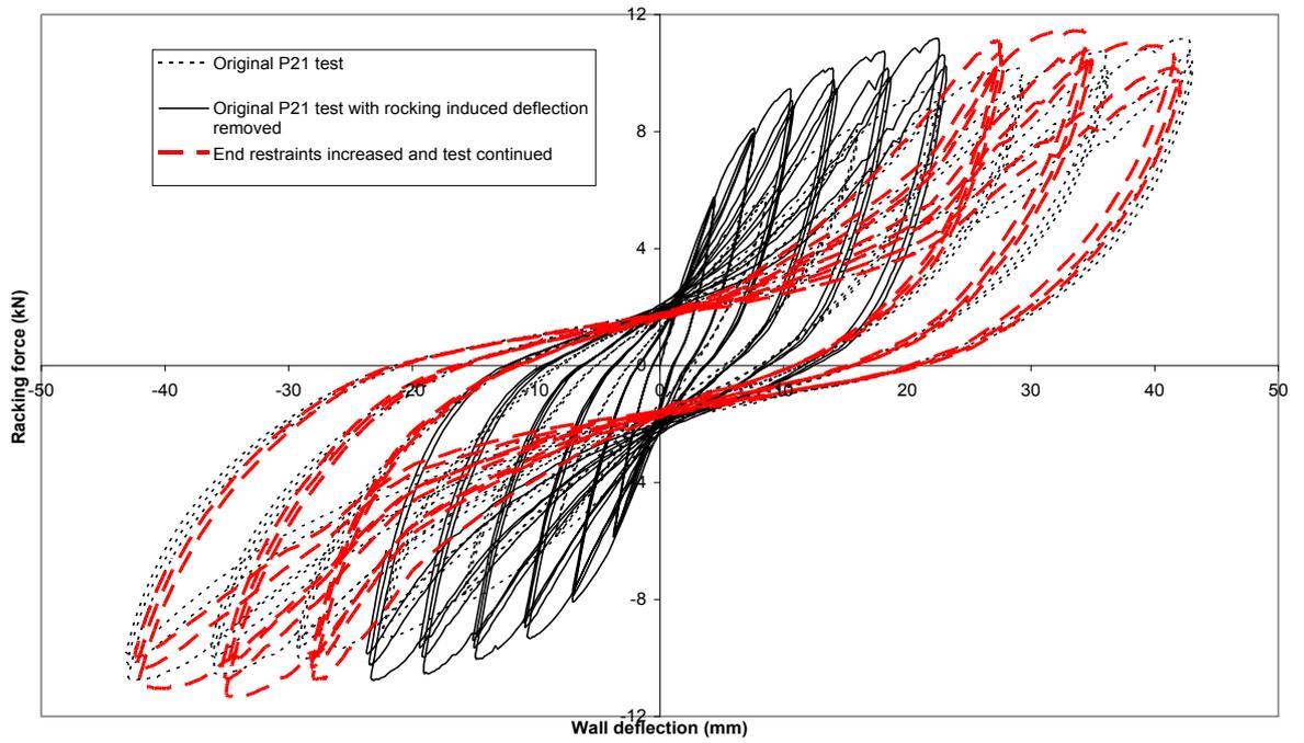
**Figure 41. Wall 11 – 1.2 m long wall lined with MDF on one face with end straps**
