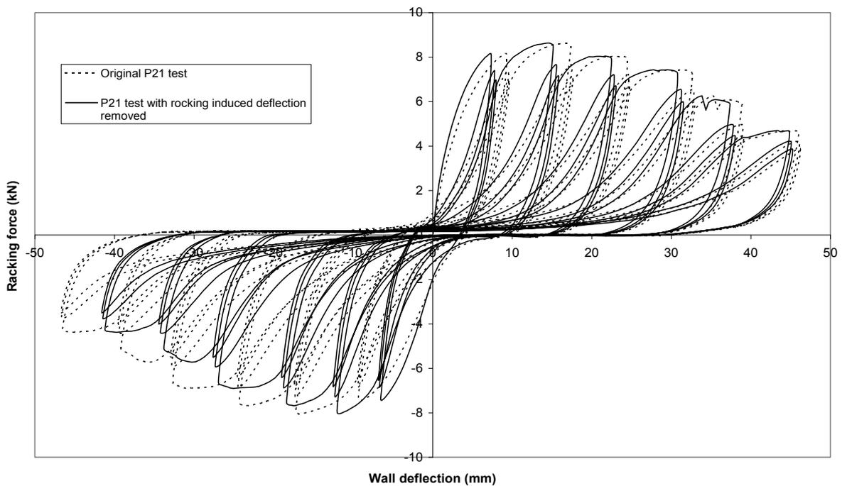
**Figure 36. Wall 6 – 1.8 m long wall lined with plasterboard on one face without end straps**
