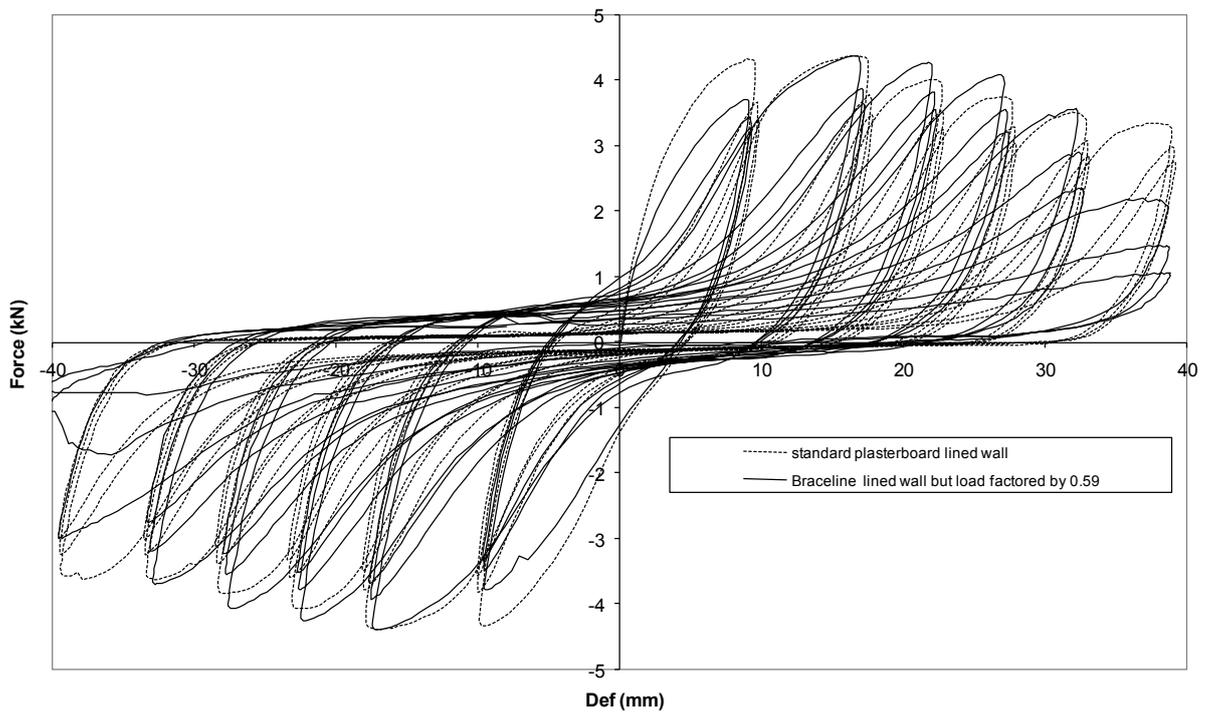
**Figure 7. Comparison of hysteresis loops for standard plasterboard and Braceline-lined walls**
