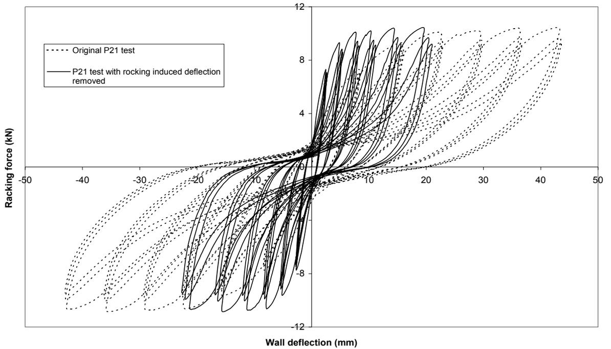
Figure 34. Wall 4 – 1.2 m long wall lined with plasterboard on both faces with end straps
