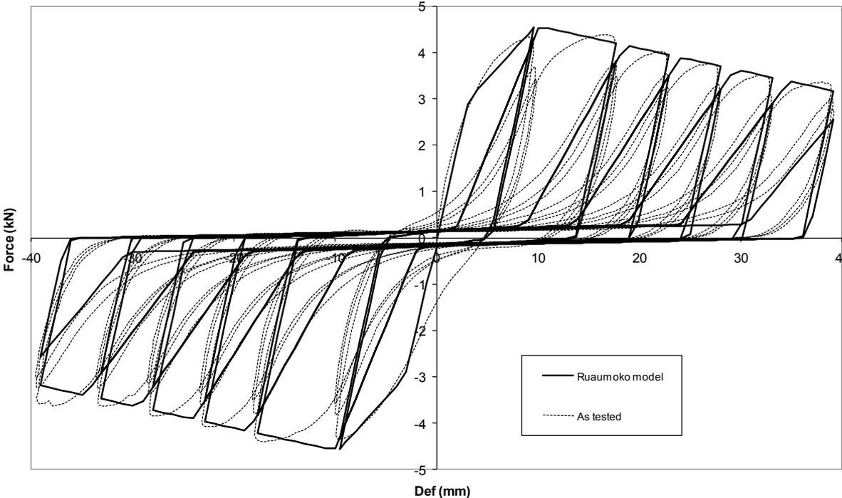
Figure 5. Comparison of test and matched hysteresis loops for standard plasterboard-lined walls
