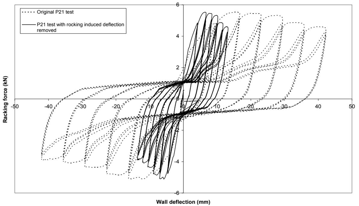
**Figure 35. Wall 5 – 1.2 m long wall lined with plasterboard on one face with end straps**
