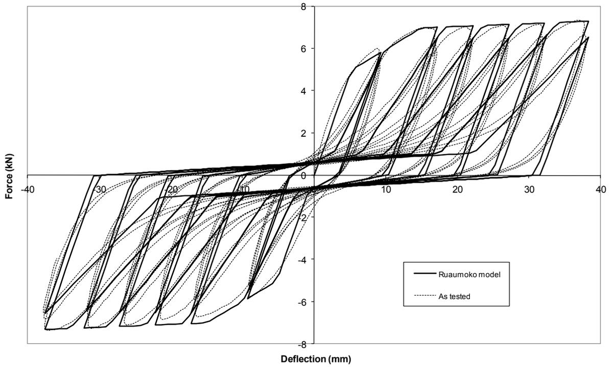
**Figure 6. Comparison of test and matched hysteresis loops for MDF-lined walls**
