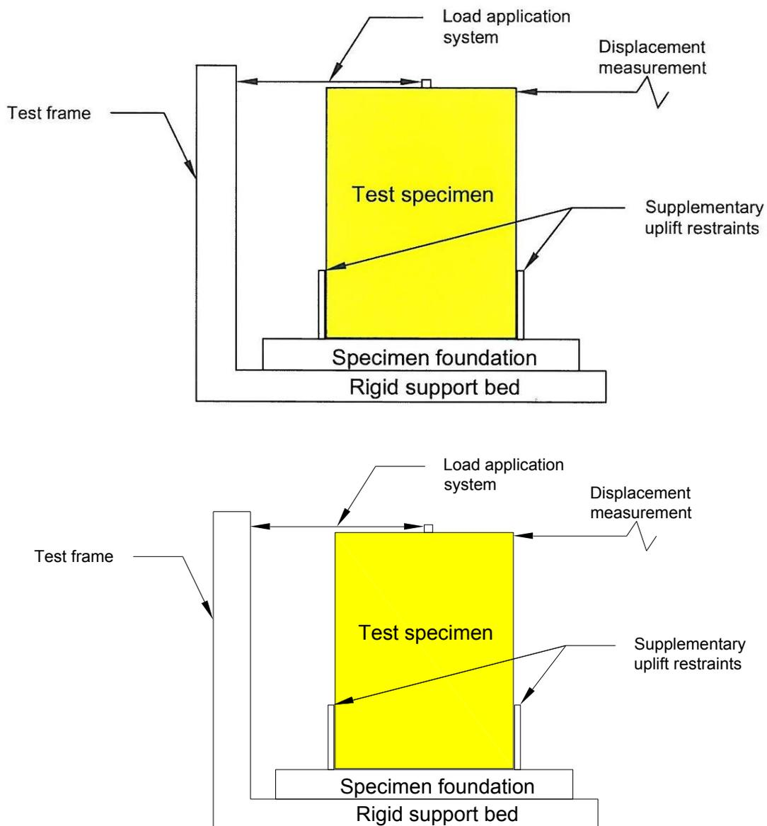
Figure 1. Test arrangement
