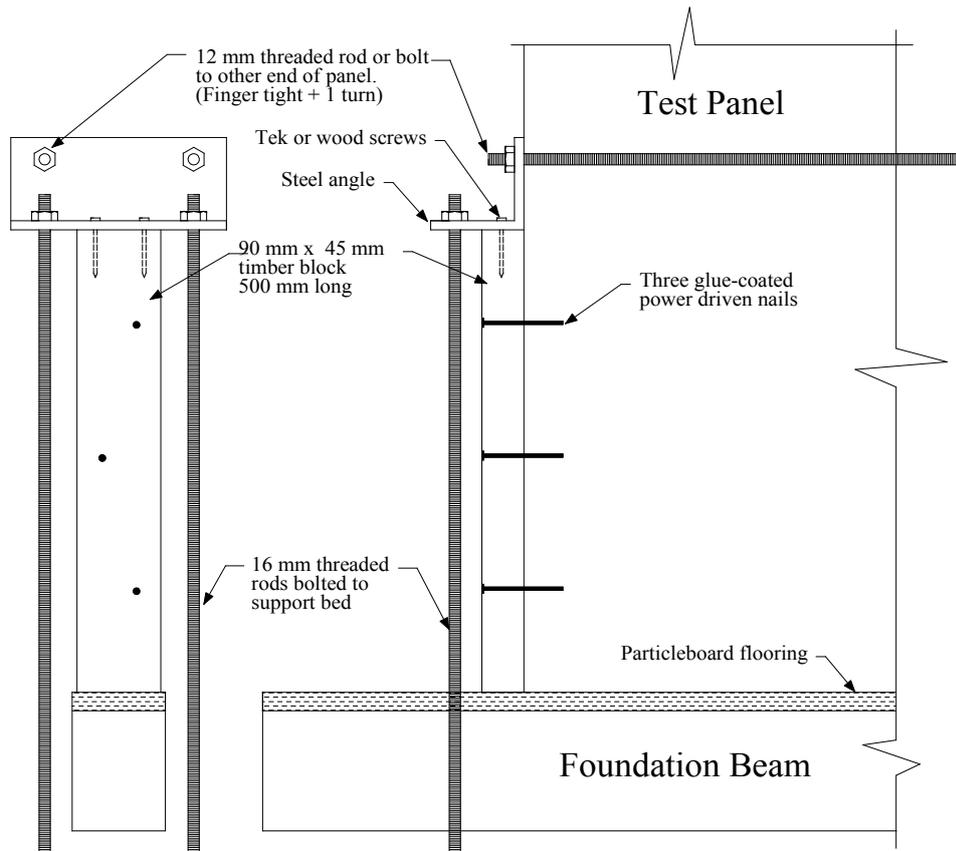
Figure 2. Supplementary uplift restraint
