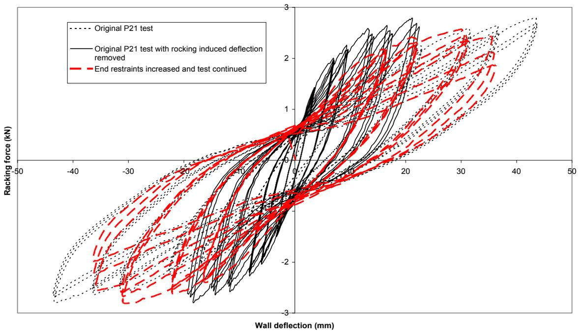
**Figure 40. Wall 10 – 0.4 m long wall lined with plasterboard on one face with end straps**
