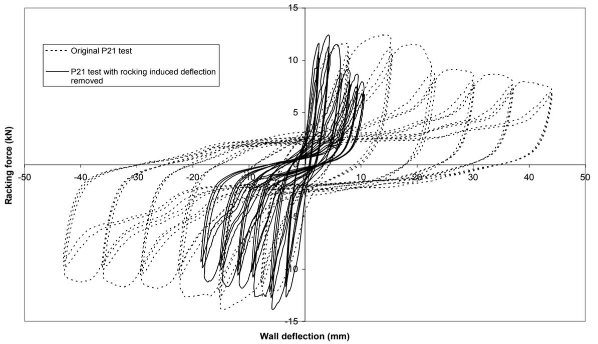
**Figure 37. Wall 7 – 2.4 m long wall lined with plasterboard on one face without end straps**
