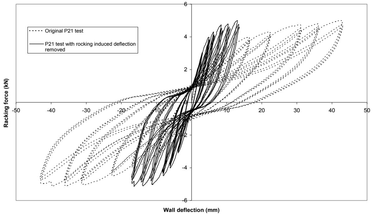
**Figure 32. Wall 2 – 0.6 m long wall lined with plasterboard on both faces with end straps**
