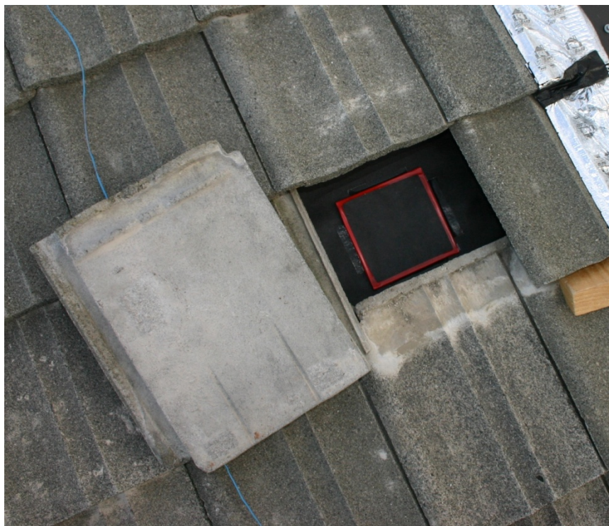
Figure 3: Picture of the condensation apparatus for roofs clad with tiles
