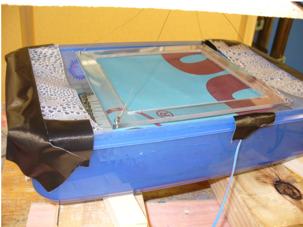
Figure 41: Detail of the Plexiglas frame supporting the underlay. The specimen is attached simply using double tape
