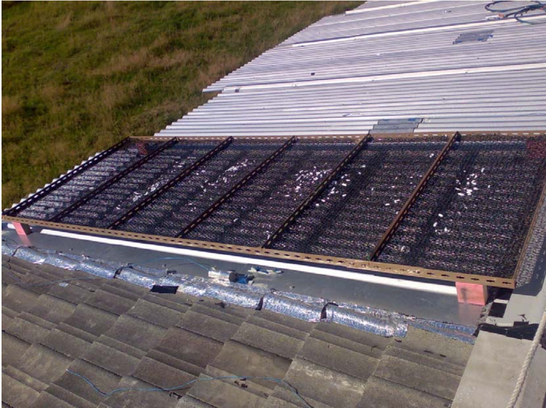
Figure 9: Metallic frame used to support the dry ice pellets in the dry ice experiment.
