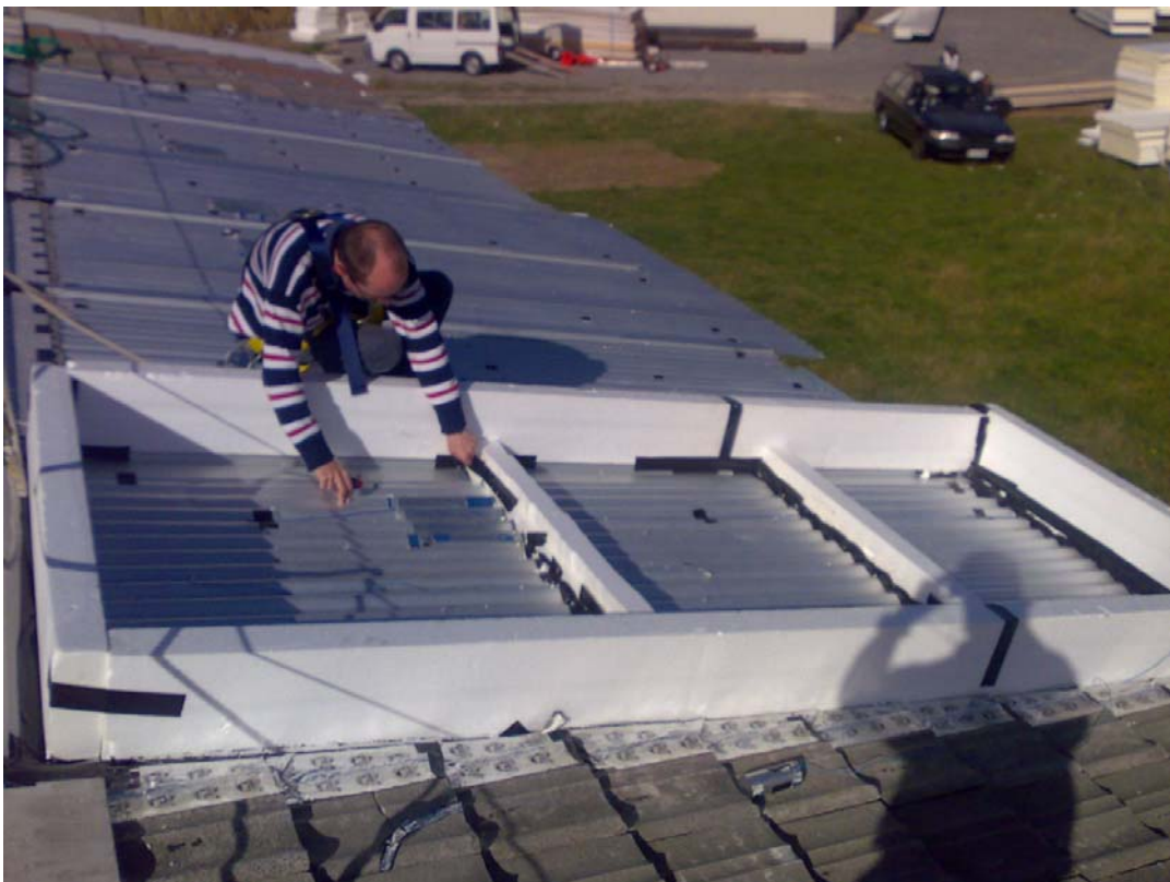
Figure 10: Polystyrene enclosure surrounding the metallic frame during the dry ice experiment. During the experiment thick polystyrene sheets sit on the polystyrene enclosure and cover the metallic frame in order to create an insulated cavity above the metal cladding.
