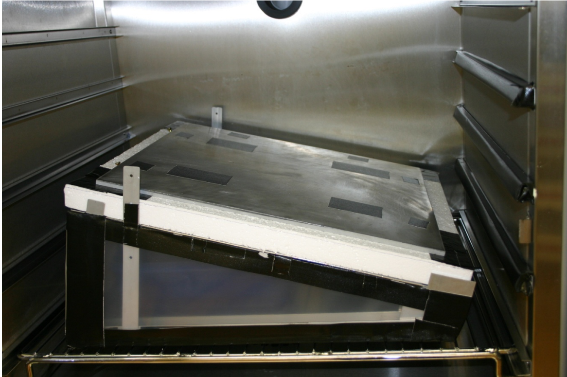
Figure 33: Metal plate simulating a metal cladding installed above the underlay specimen
