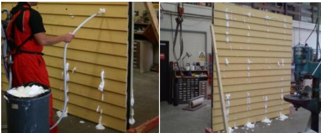
Figure 13a & b: Installation of Airfoam in large scale test wall (D4861) at BRANZ
