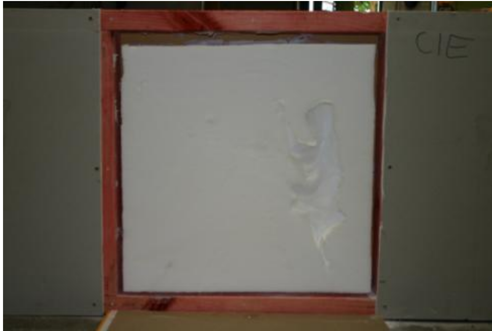
Figure 24: : Shrinkage in low wall C1, specimen C1D.
