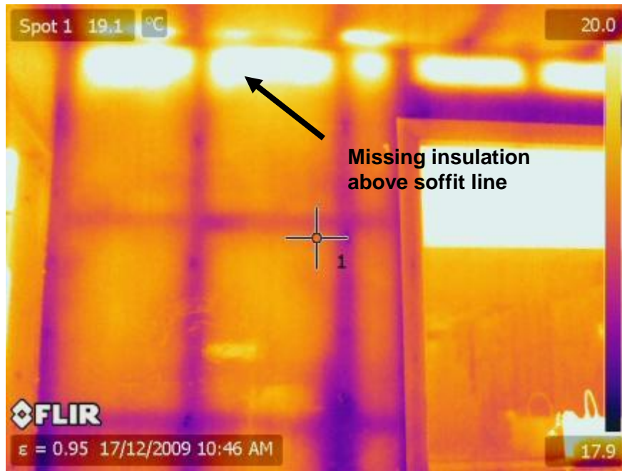
Figure 4: Thermal image identifying missing insulation in another upper wall above the soffit line (House C7)
